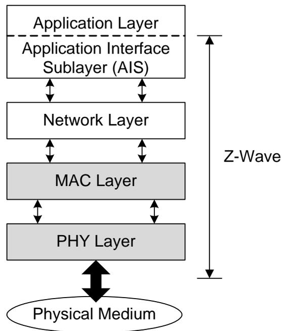
**Figure A.2 – Z-Wave layers**
