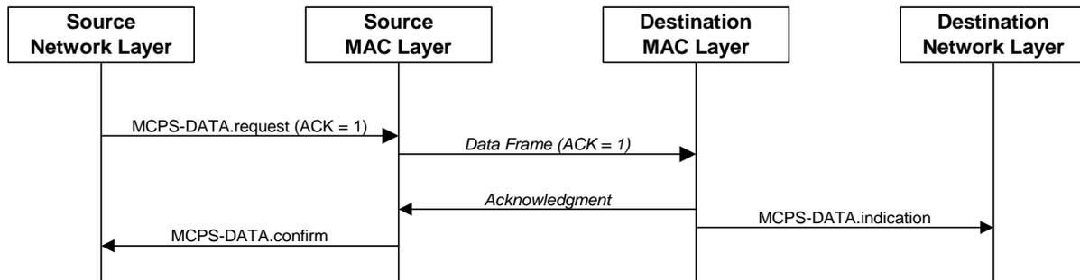
**Figure 8-23 – Successful data transmission with an acknowledgment frame**
