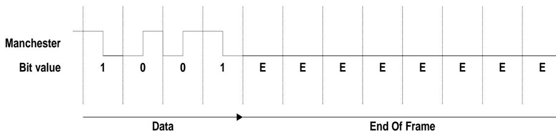
**Figure A.10 – End of frame delimiter (EFD) pattern (R2/R3)**
