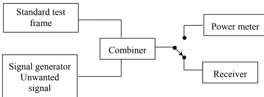
**Figure A.6 – Receiver blocking test definitions**
