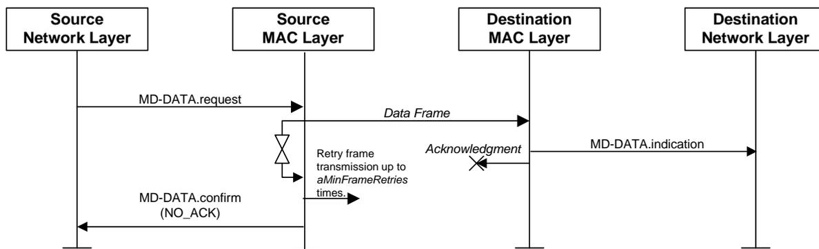
**Figure A.35 – Lost acknowledgment frame transmission scenario**
