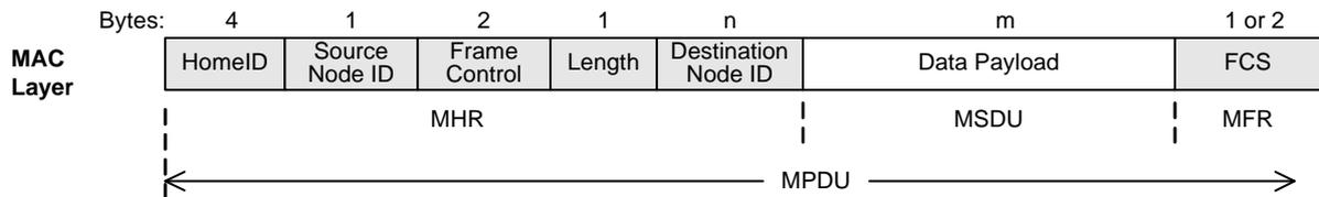
**Figure A.14 – General MAC frame format (Channel Configurations 1, 2 only)**
