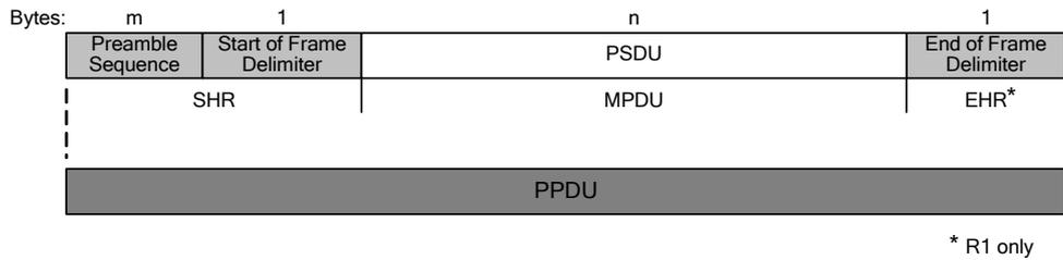
**Figure 7-4 – PPDU packet format**
