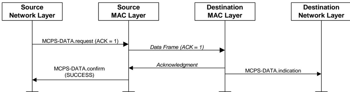
**Figure A.34 – Lost frame transmission scenario**
