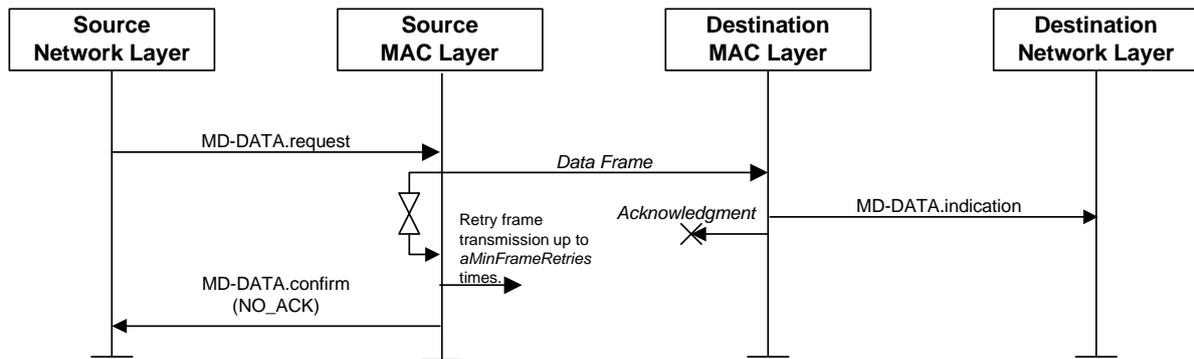
**Figure 8-26 – Lost acknowledgment frame transmission scenario**
