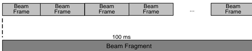
**Figure 8-19 – Format of the beam fragment**
