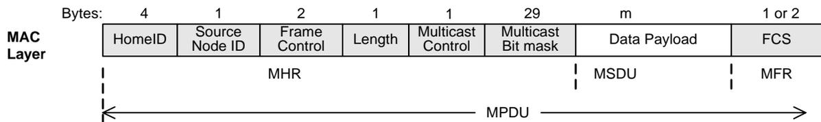
**Figure A.16 – Multicast MAC frame format (channel configurations 1, 2 only)**
