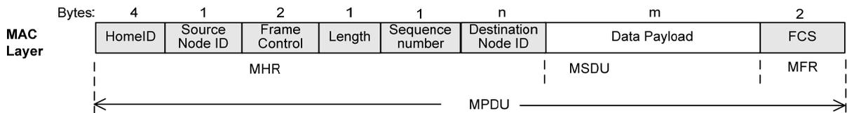
**Figure A.15 – General MAC frame format (channel configuration 3 only)**
