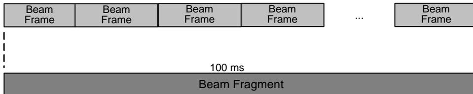
Figure A.28 – Format of the beam fragment
