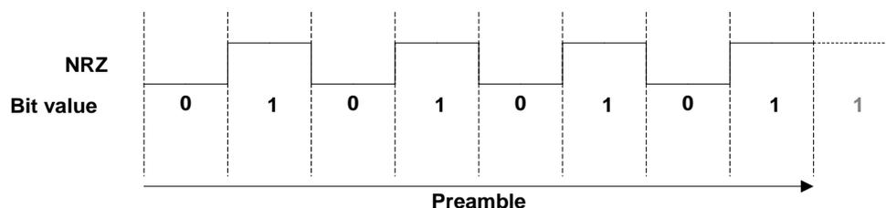
Figure A.9 – NRZ encoded preamble pattern (R2/R3)
