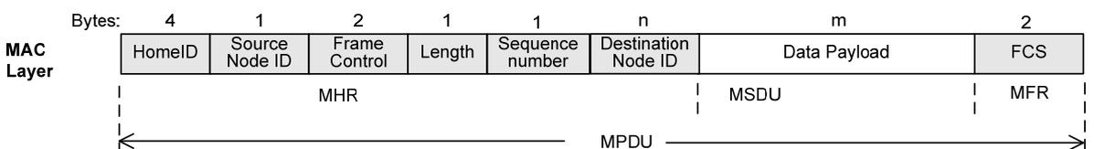
**Figure 8-6 – General MAC frame format (channel configuration 3)**
