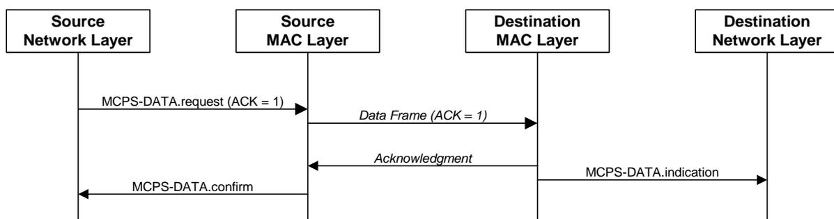
Figure A.32 – Successful data transmission with an acknowledgment frame
