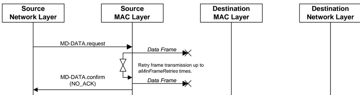
Figure 8-25 – Lost frame transmission scenario
