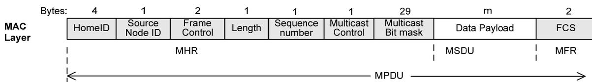
**Figure A.17 – Multicast MAC frame format (channel configuration 3)**
