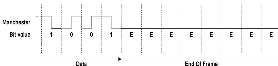
**Figure 7-7 – End of frame delimiter pattern**
