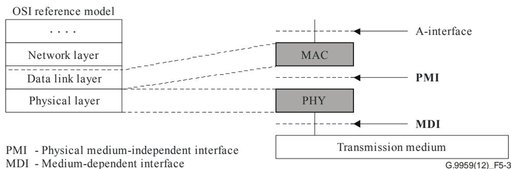
**Figure 5-3 – Protocol reference model of an ITU-T G.9959 transceiver**
