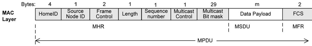
**Figure 8-8 – Multicast MAC frame format (channel configuration 3)**
