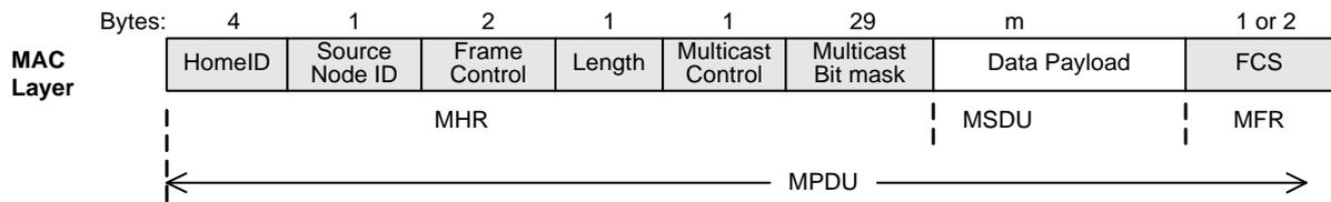
**Figure 8-7 – Multicast MAC frame format (channel configurations 1, 2)**
