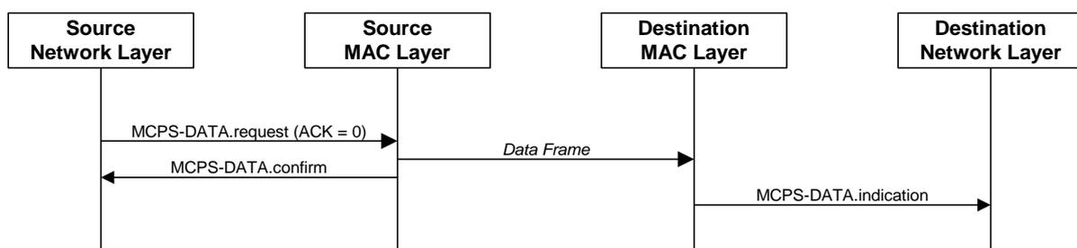
Figure 8-22 – Successful data transmission without an acknowledgment
