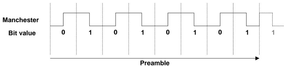
**Figure 7-5 – Manchester encoded preamble pattern (R1)**
