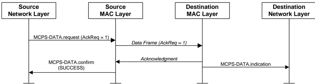
**Figure A.33 – Successful frame transmission scenario**
