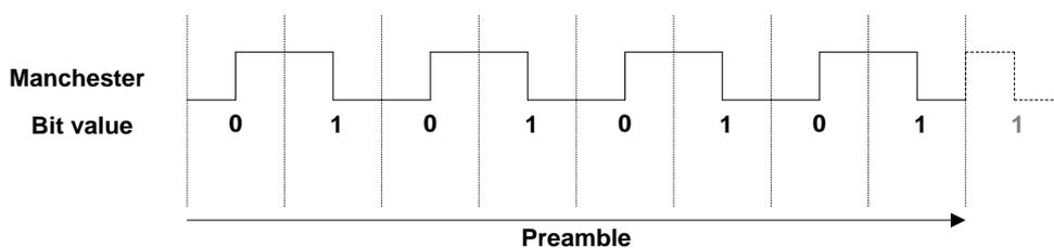
Figure A.8 – Manchester encoded preamble pattern (R1)
