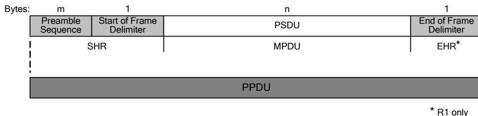
Figure A.7 – PPDU packet format
