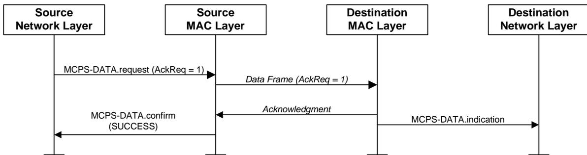
Figure 8-24 – Successful frame transmission scenario
