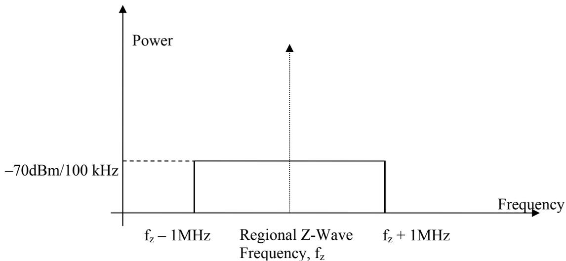
**Figure A.5 – Receiver spurious requirements**
