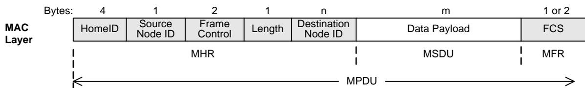
**Figure 8-5 – General MAC frame format (channel configurations 1, 2)**
