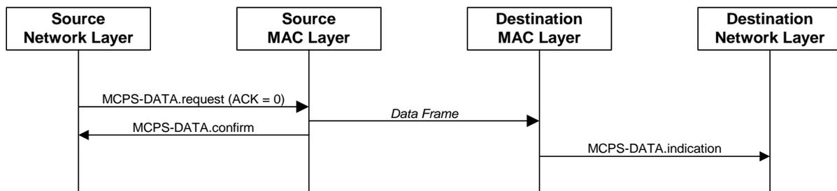
Figure A.31 – Successful data transmission without an acknowledgment
