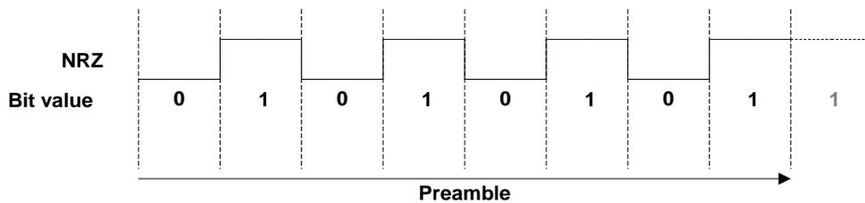
**Figure 7-6 – NRZ encoded preamble pattern (R2/R3)**
