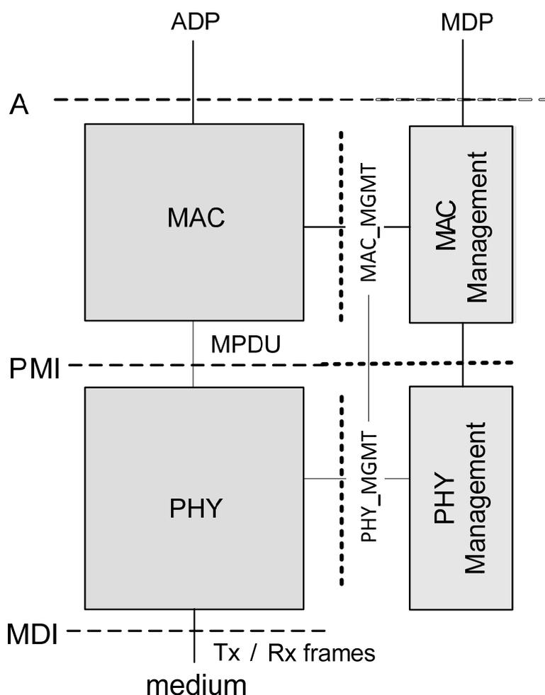
**Figure 5-5 – Functional model of an ITU-T G.9959 transceiver**
