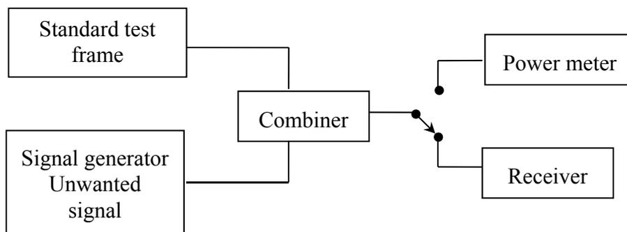
**Figure 7-3 – Receiver blocking test definition**
