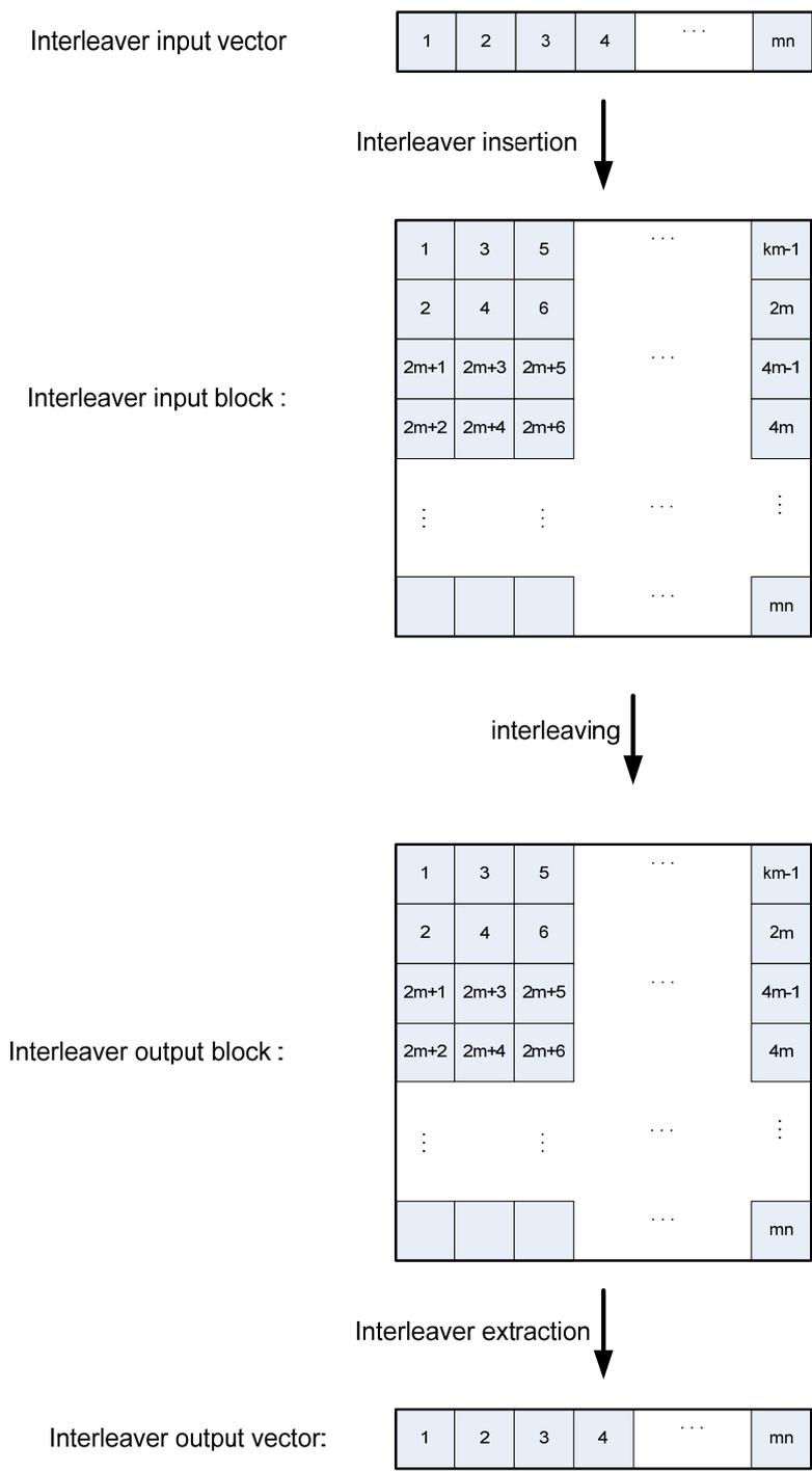
**Figure 7-14 – Order of writing in and reading out of the permutation matrix**
