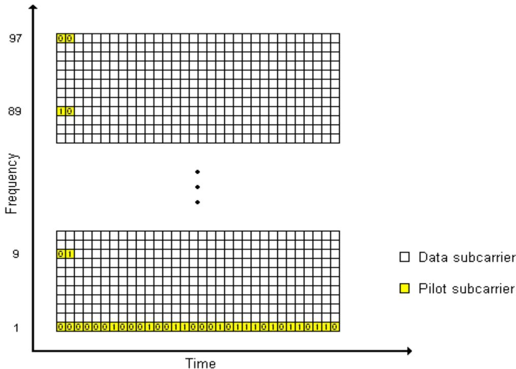
**Figure B.4 – Pilot and data subcarrier allocation (OFDM symbols vs subcarriers)**
