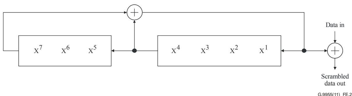
**Figure E.2 – LFSR used to generate the data bits that are used to modulate the pilot tones**
