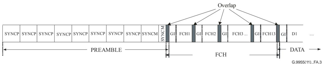
**Figure A.3 – Typical data frame structure**
