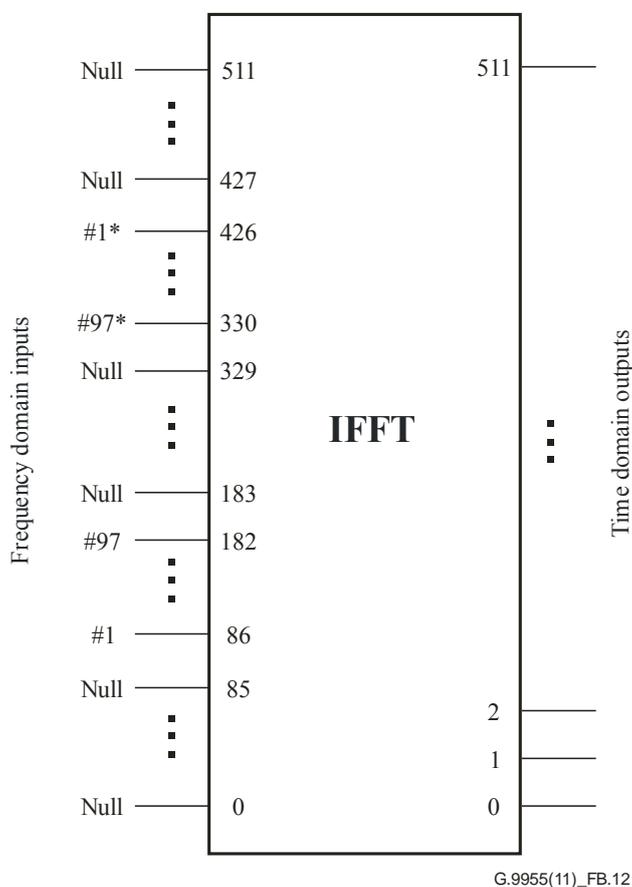
**Figure B.12 – Subcarrier mapping**
