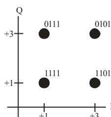
**Figure E.1 – 16-QAM constellation diagram**
