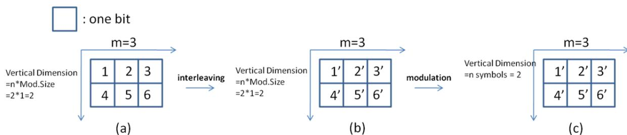
**Figure A.11 – Example of interleaving with DBPSK**
