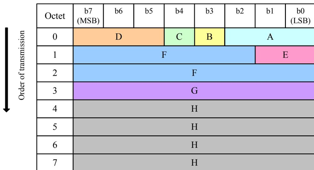
**Figure 6-1 – Example of mapping fields onto groups of octets**
