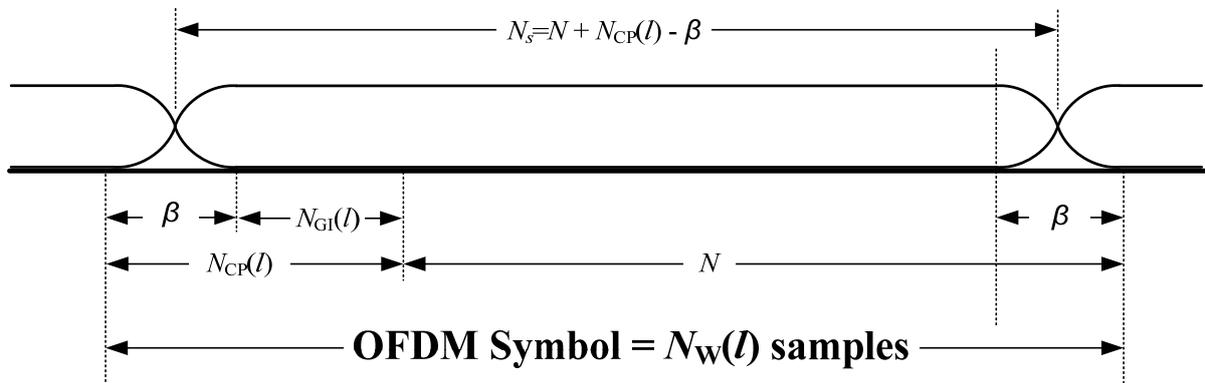
Figure 7-22 – Structure of an OFDM symbol
