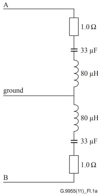
**Figure I.1a – The adaptative network for the frequency range 3 kHz-148.5 kHz**
