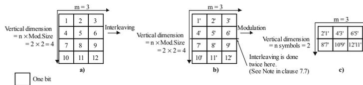
**Figure A.12 – Example of interleaving with DQPSK**
