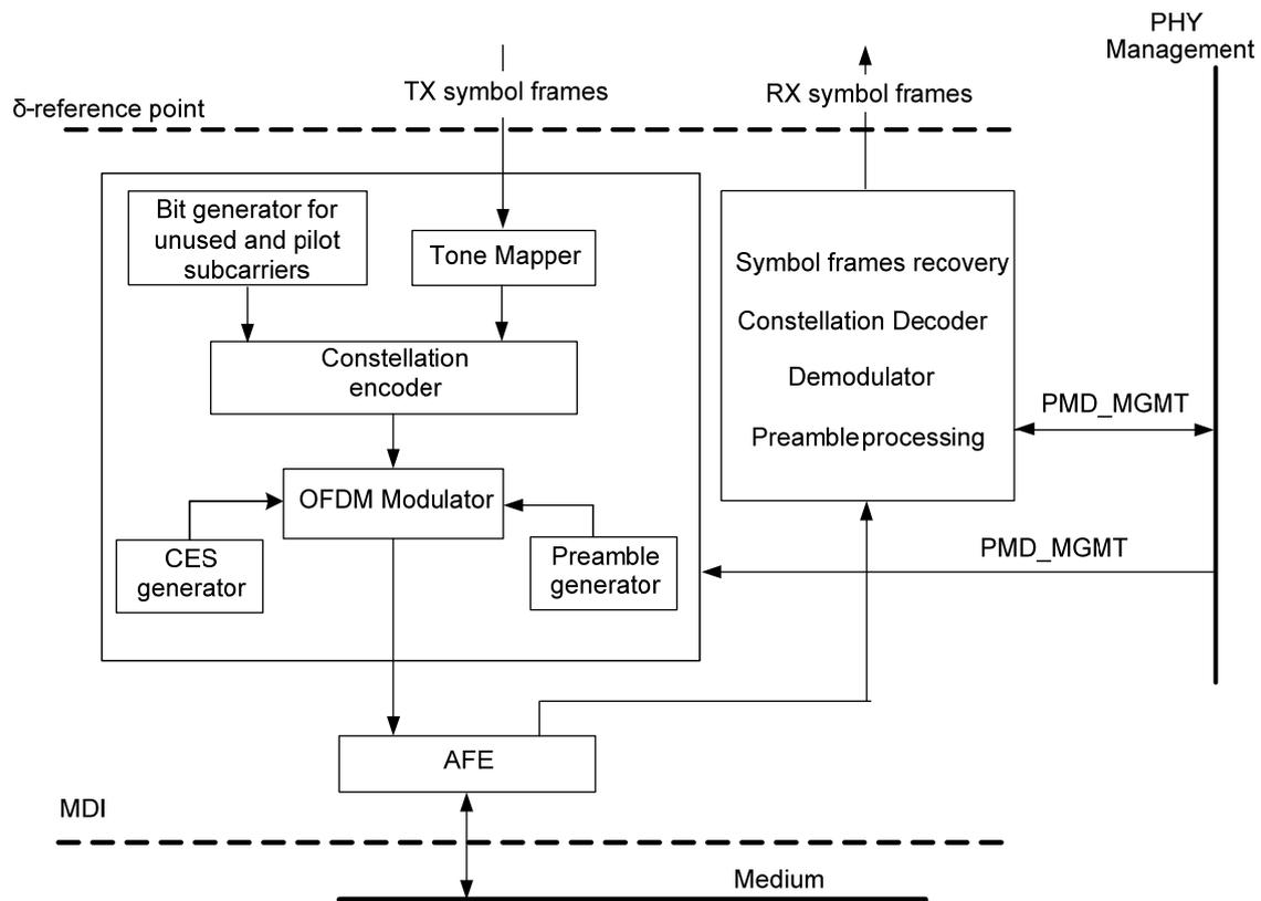
**Figure 7-16 – Functional model of PMD**
