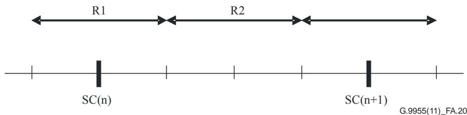
**Figure A.20 – Frequency notching**
