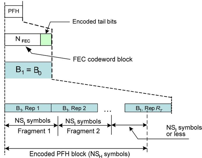
**Figure 7-13 – Generation of the encoded PFH block**
