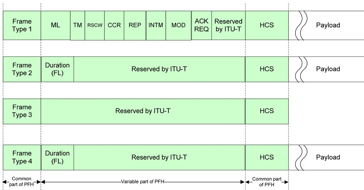
**Figure 7-4 – Content of the PFH depending on the Frame Type field**
