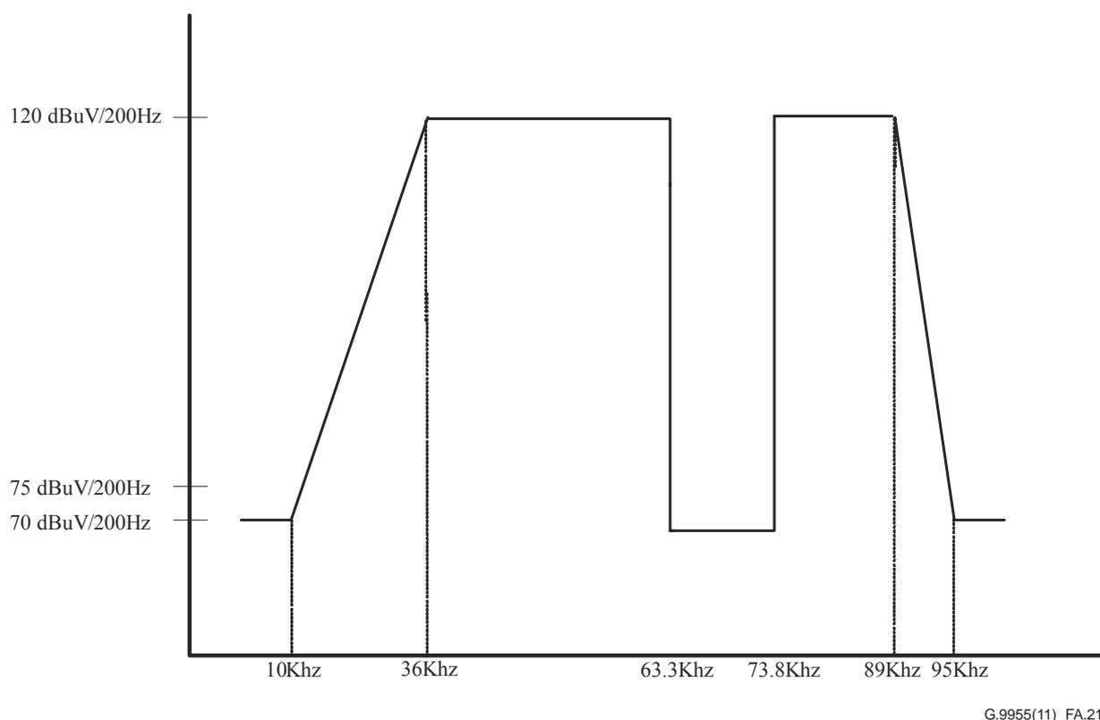
**Figure A.21 – Spectrum with two notches inserted to cohabitate with S-FSK PLC modem**
