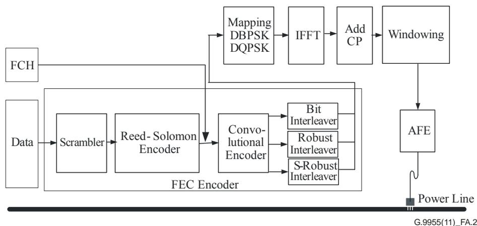
Figure A.2 – Block diagram of OFDM transceiver
