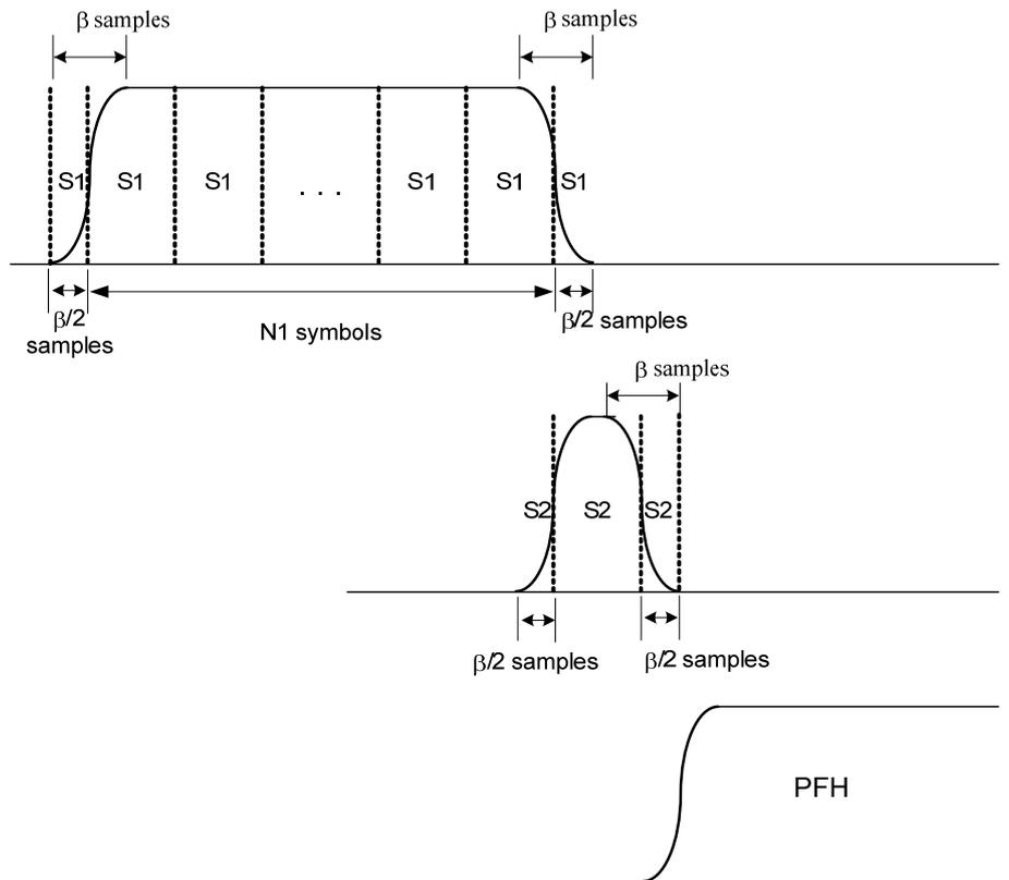
**Figure 7-25 – Preamble time-domain generation**
