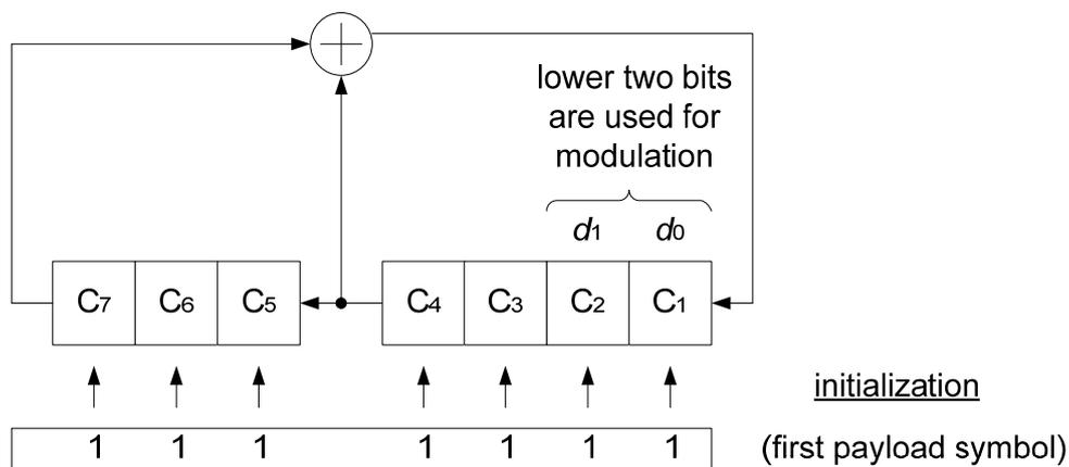
**Figure 7-17 – LFSR for modulation of inactive subcarriers**
