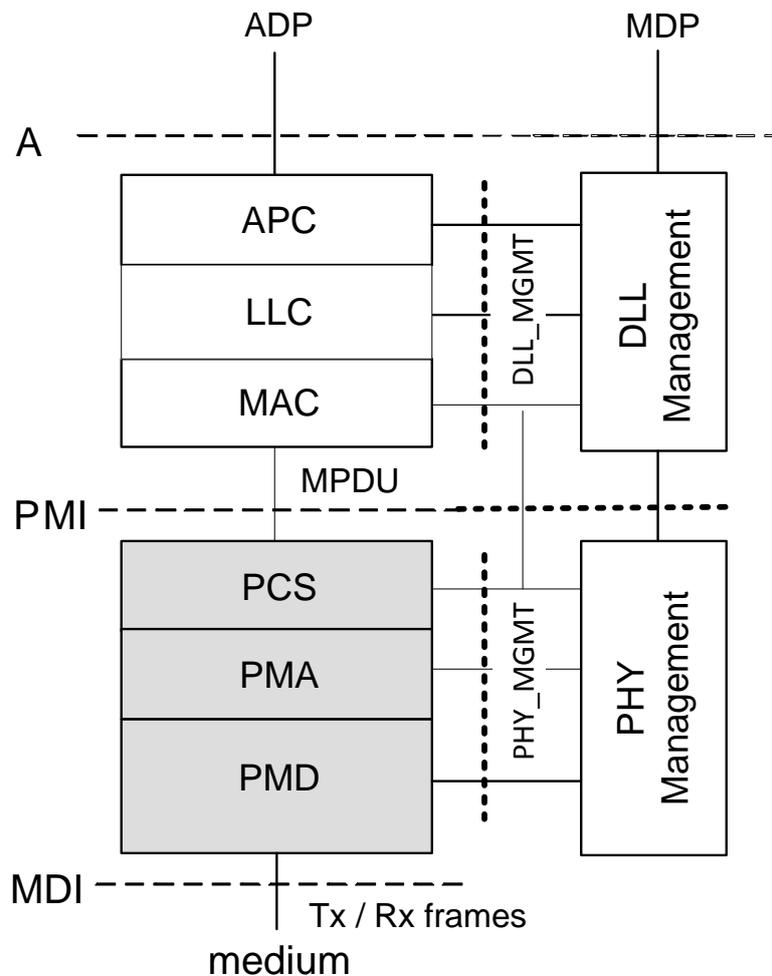
**Figure 5-7 – Functional model of ITU-T G.9955 transceiver**
