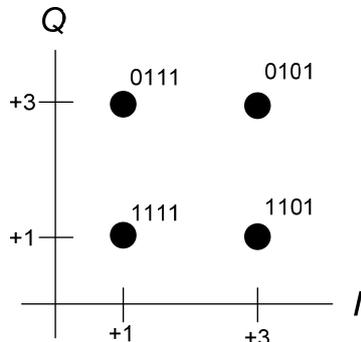
**Figure 7-19 – Constellation mapping for  $b = 4$  ( $d_3d_2d_1d_0$ , first quadrant)**
