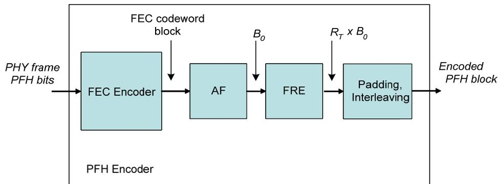
**Figure 7-12 – Functional diagram of the PFH encoder**
