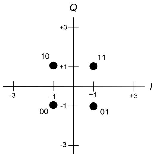
**Figure 7-18 – Constellation mapping for  $b = 2$  ( $d_1d_0$ )**
