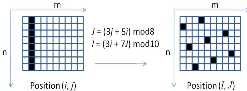
**Figure A.10 – Example of spreading behaviour**
