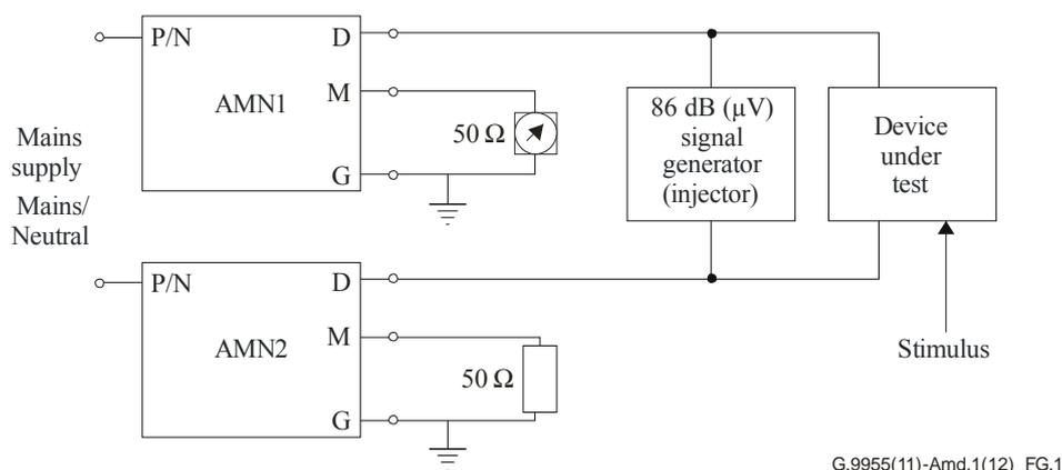
NOTE – AMN1 to AMN2 are artificial mains networks conforming to subclause 11.2 of [CISPR 16-1] (example Figure 5 / 9-148.5 kHz)
