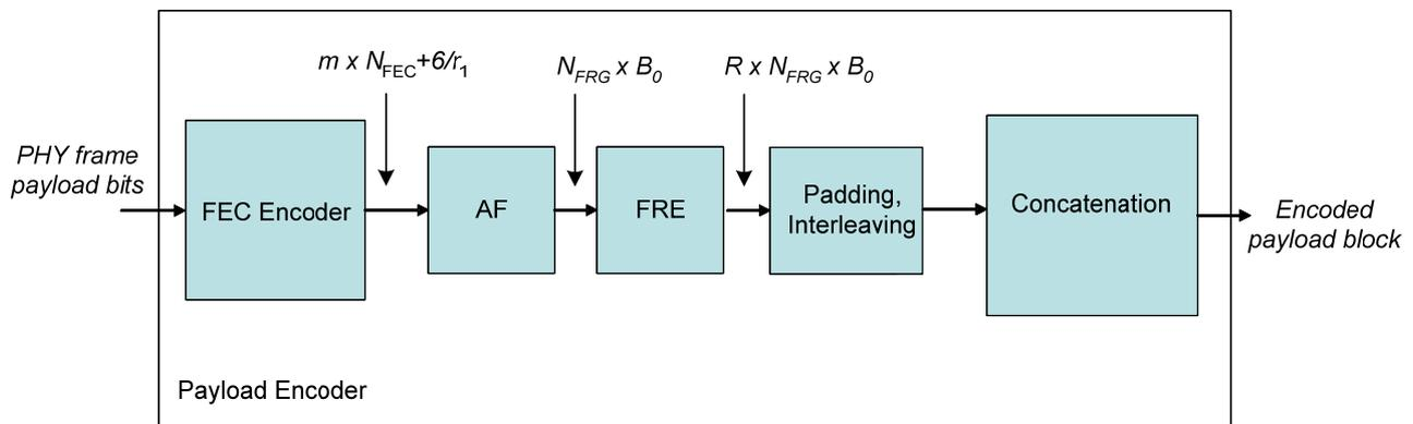
**Figure 7-9 – Functional diagram of the payload encoder**
