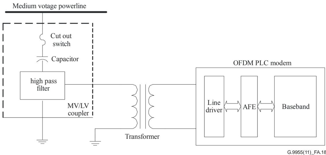
**Figure A.18 – Proposed coupling circuit**
