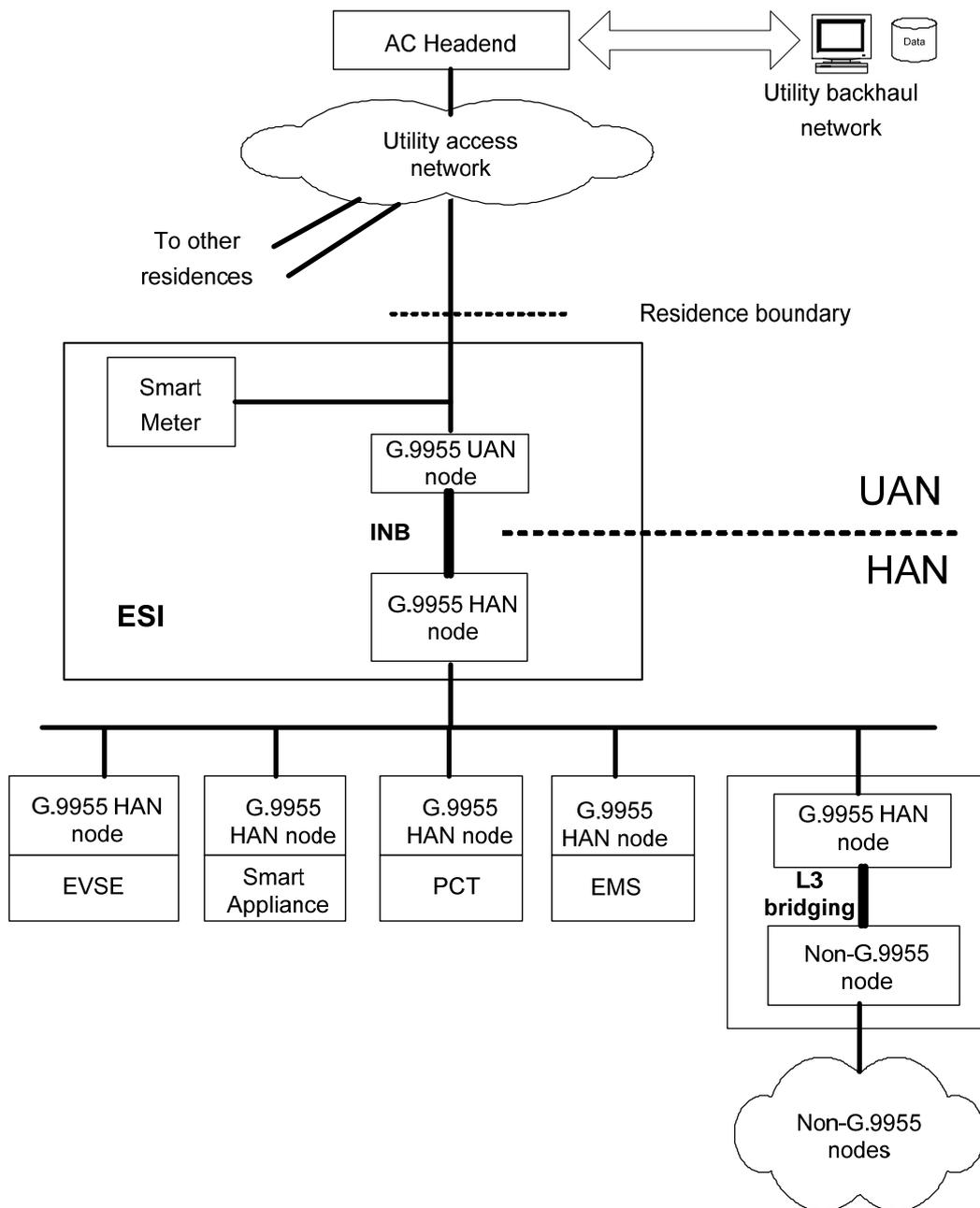
**Figure 5-4 – Example of functional diagram of an EM-HAN connected to utility**
