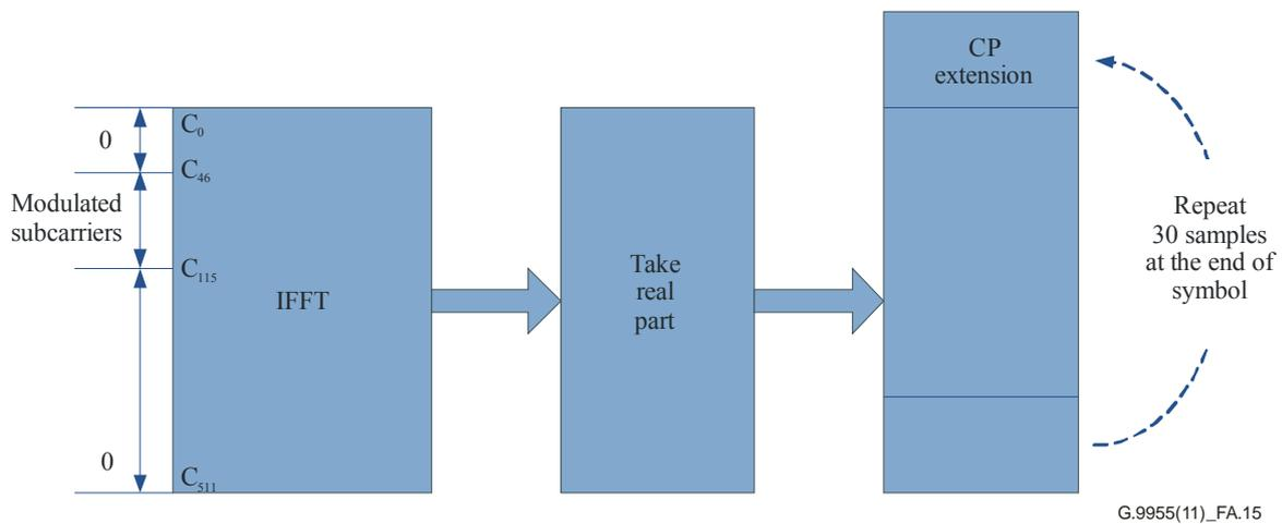
**Figure A.15 – IFFT input/output and CP addition**
