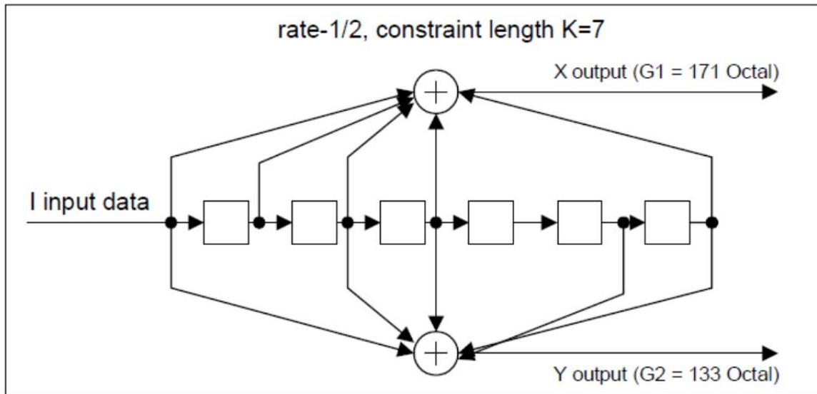
**Figure 7-8 – Inner convolutional code encoder**
