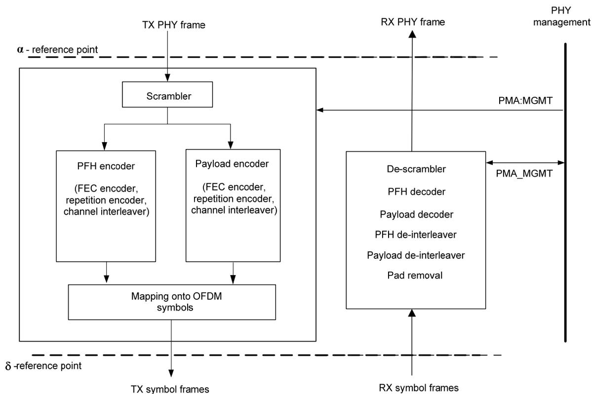
**Figure 7-5 – Functional model of PMA**
