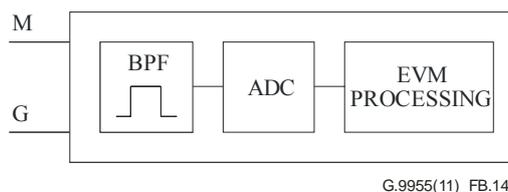
**Figure B.14 – EVM meter (block diagram)**
