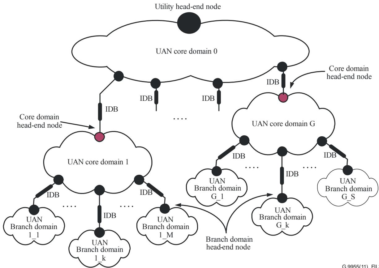
**Figure II.3 – Example of UAN with multiple domains**
