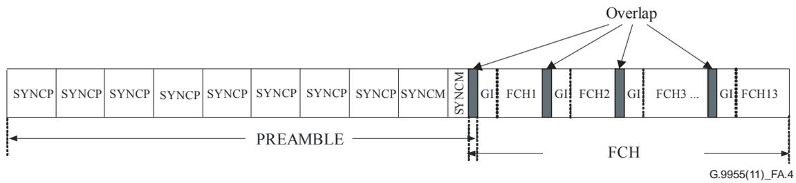
**Figure A.4 – ACK/NACK frame structure**
