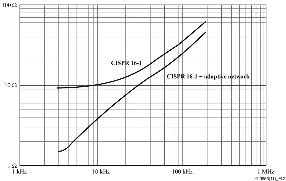
**Figure I.2 – The nominal CISPR 16-1 impedance (doubled) and the calculated impedance between points A and B (Figure I.1b) when the adaptive network is added to the CISPR 16-1 network**
