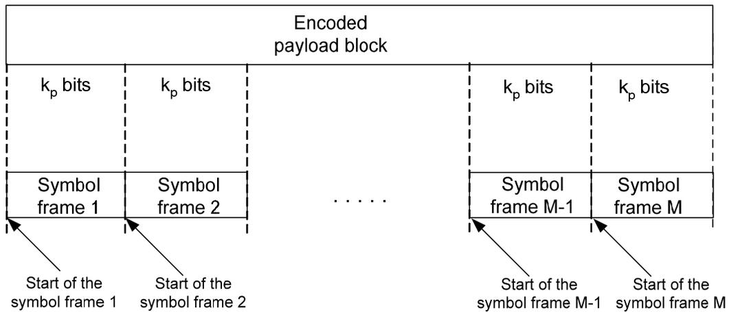
**Figure 7-15 – Payload mapping**
