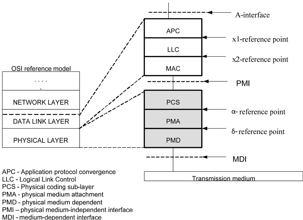
**Figure 5-5 – Protocol reference model of ITU-T G.9955 transceiver**
