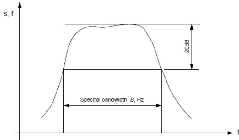
**Figure 7-27 – Measurement of spectral bandwidth**
