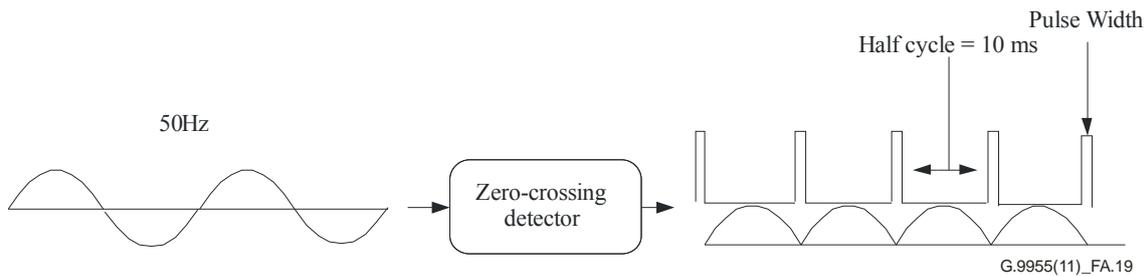
**Figure A.19 – Zero crossing detector**
