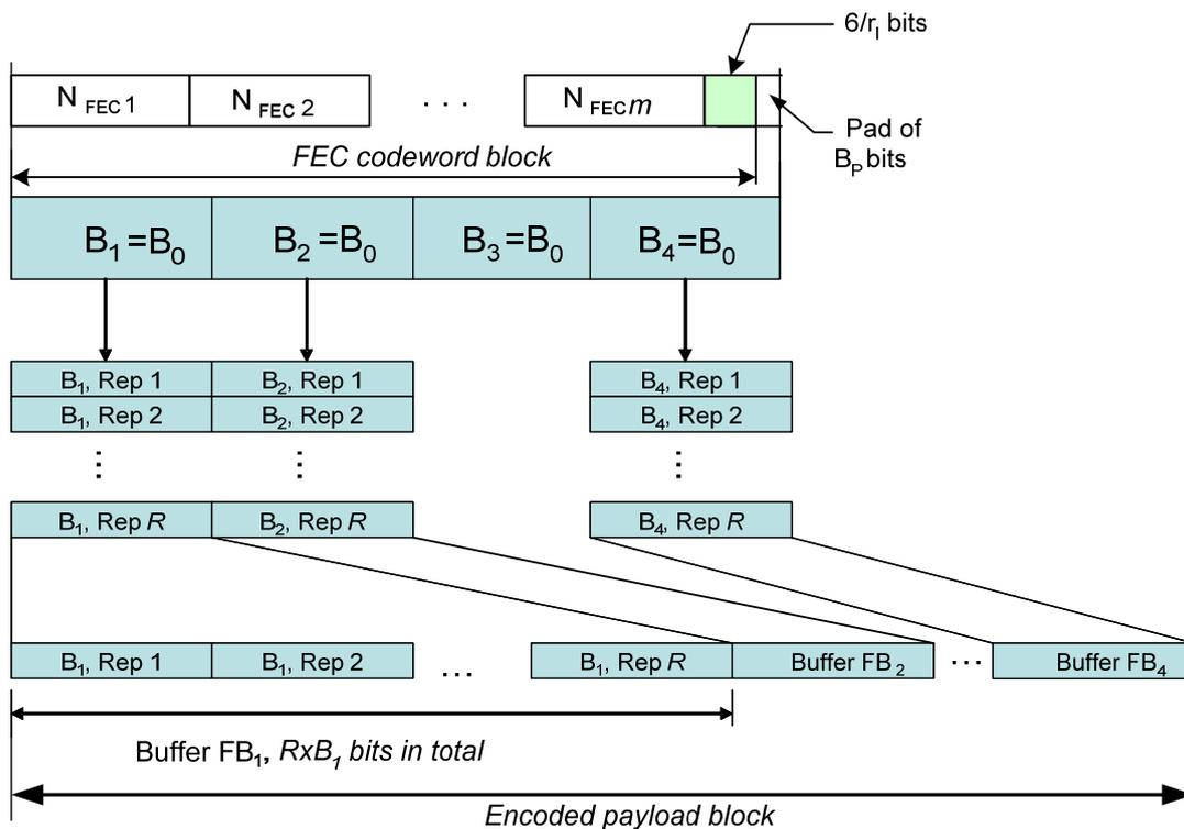
**Figure 7-10 – Generation of the encoded payload block (case  $N_{\text{frg}} = 4$ , cyclic shifting, interleaving and padding of fragments when in IoAC mode is not shown)**
