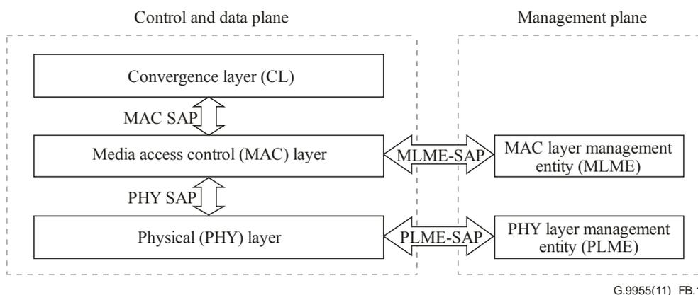
**Figure B.1 – Reference model of PRIME protocol layers**
