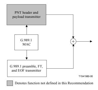
Figure 9/G.989.1 – Basic structure of a G.989.1 transmitter
