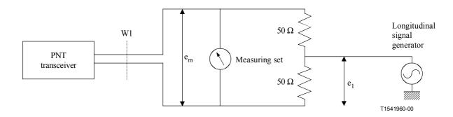
NOTE – When performing the measurement of this parameter, in order to ensure meaningful results, resistance values must be within 0.1% of the values specified here.
