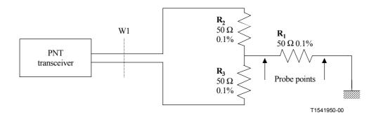
NOTE – The specified value of no more than –55 dBVrms considers that the measurement across resistor  $R_1$  measures 2/3 of the actual longitudinal voltage. Therefore, when performing a measurement of this parameter, in order to ensure meaningful results, the resistance values of  $R_1$ ,  $R_2$  and  $R_3$  as depicted in this figure must be well matched and the values of the resistors must be within 0.1% of the values specified here.
