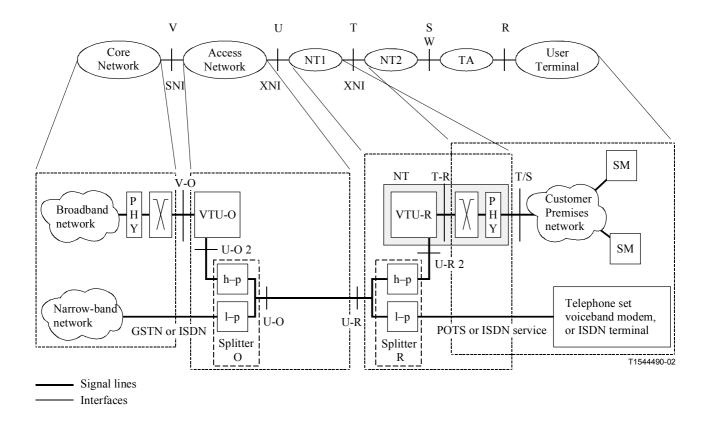
Figure 8 bis/G.995.1 – G.993.1 system reference model and its alignment with the generic reference configuration
