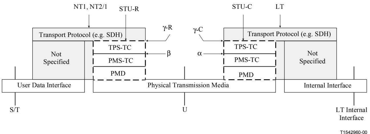
**Figure 12/G.995.1 – User plane protocol reference architecture for ITU-T G.991.2**
