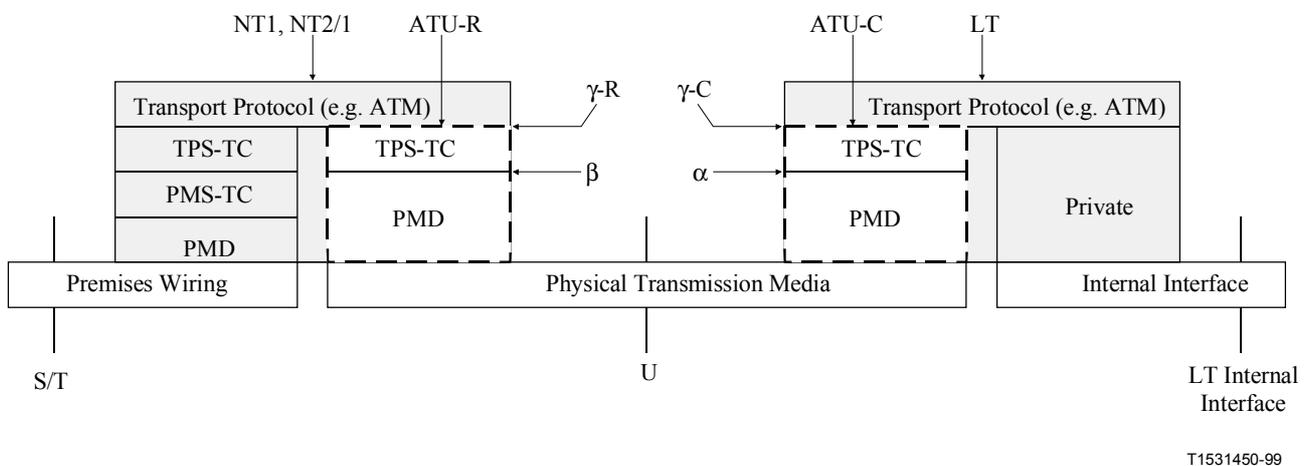
**Figure 10/G.995.1 – User plane protocol reference architecture for ITU-T G.992.1 and G.992.2**
