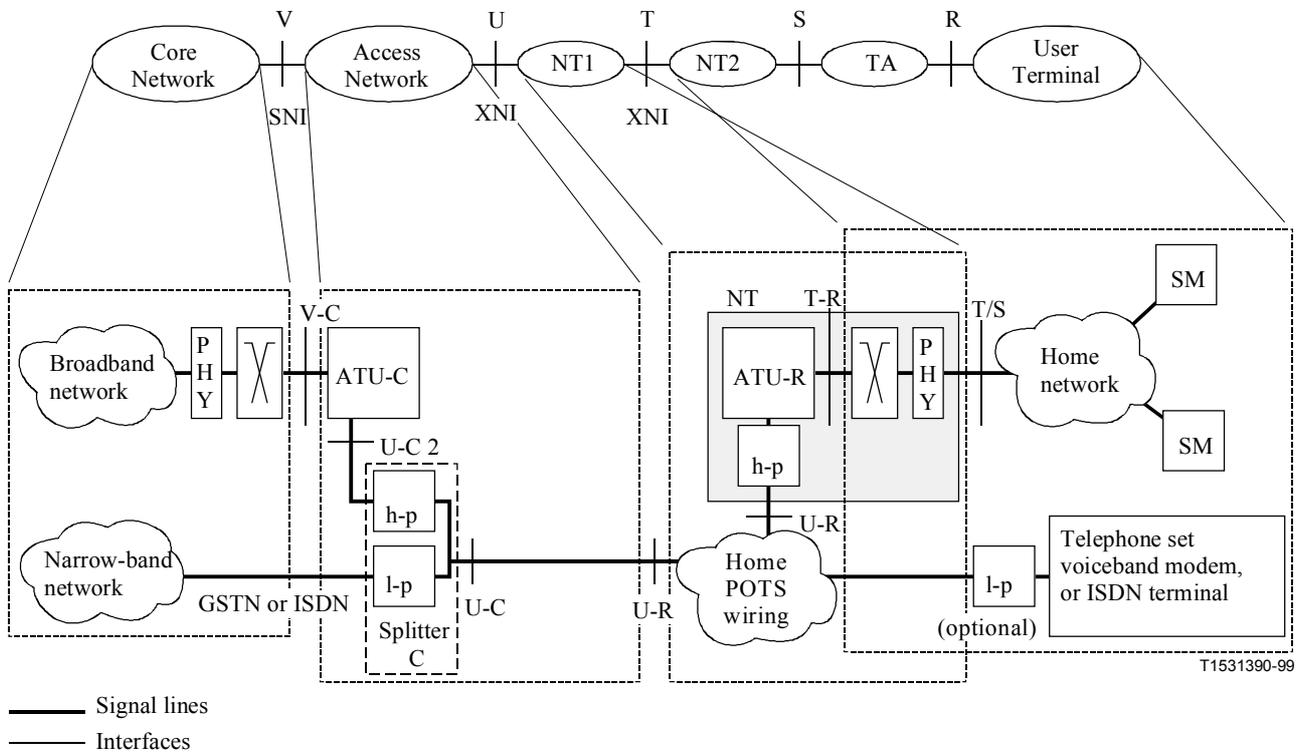
**Figure 3/G.995.1 – G.992.2 system reference model and its alignment with the generic reference configuration**
