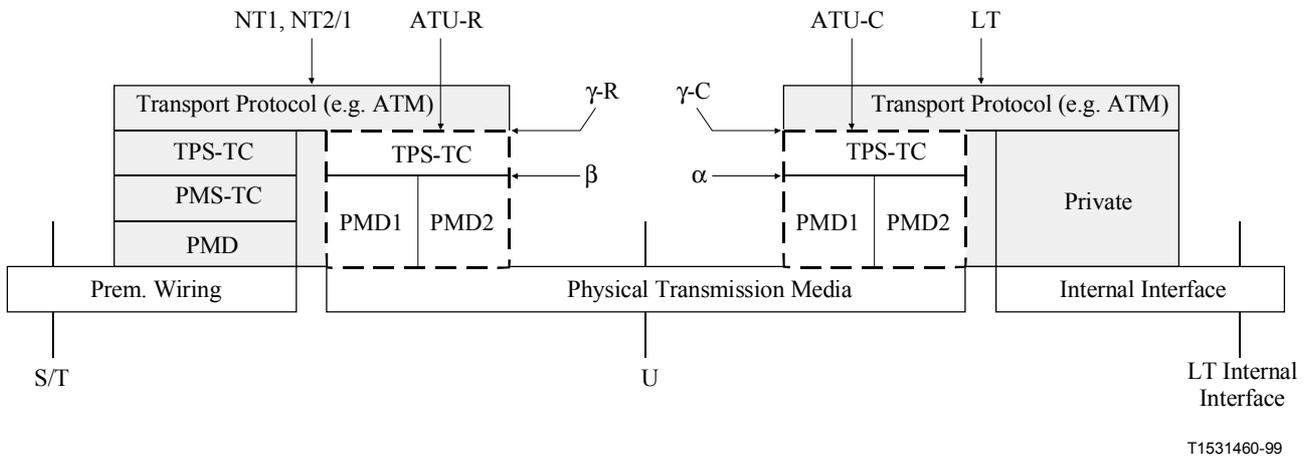
**Figure 11/G.995.1 – User plane protocol reference architecture for ITU-T G.991.1**
