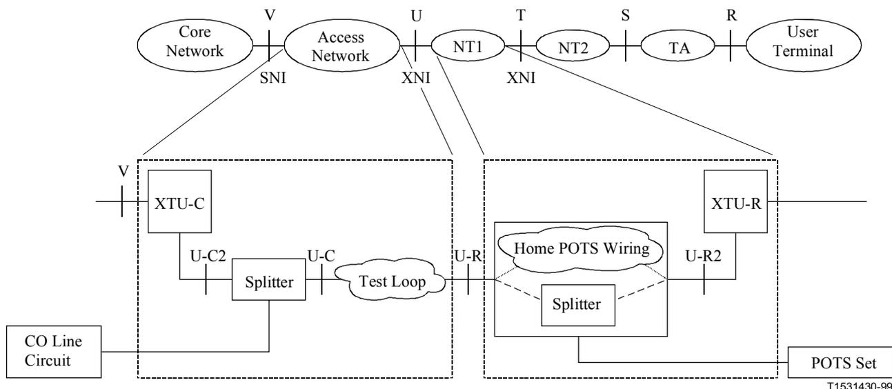
**Figure 8/G.995.1 – G.996.1 system reference model and its alignment with the generic reference configuration**
