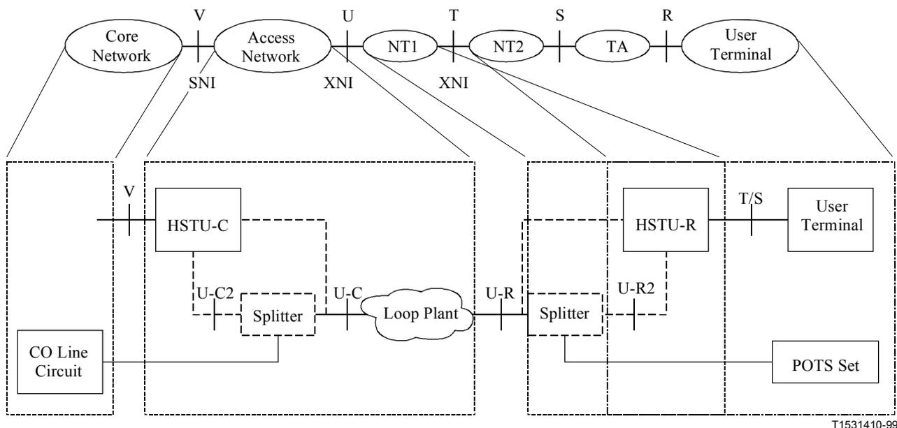
**Figure 6/G.995.1 – G.994.1 system reference model and its alignment with the generic reference configuration**
