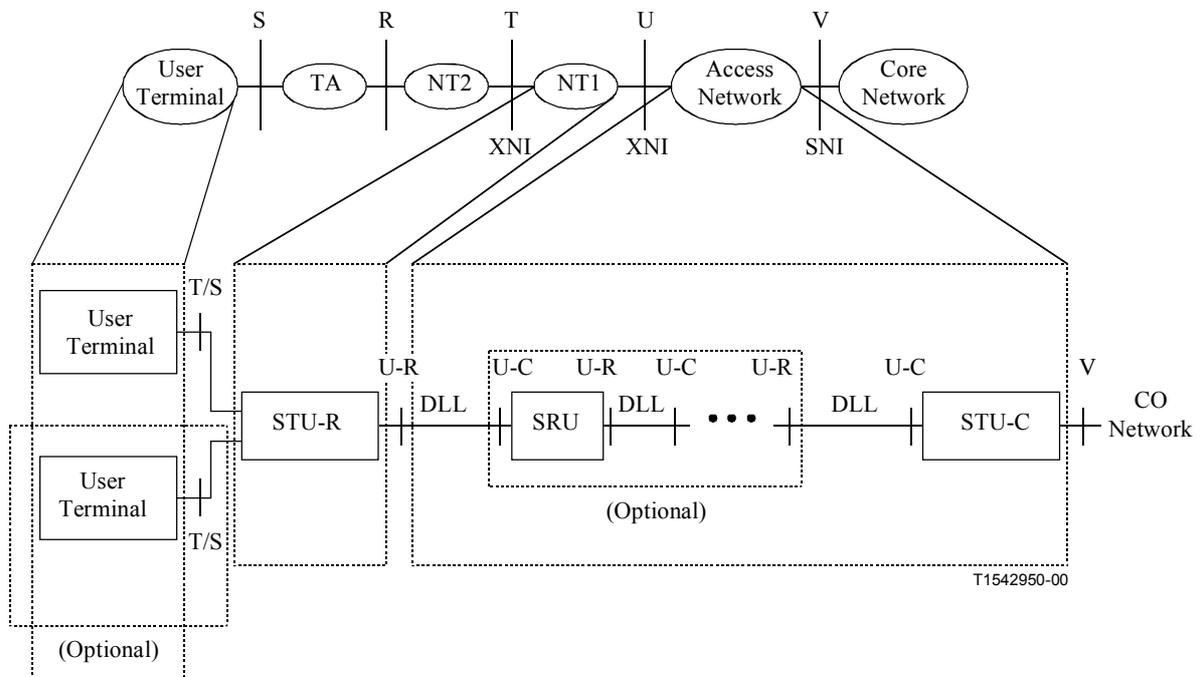
**Figure 5/G.995.1 – G.991.2 system reference model and its alignment with the generic reference configuration**
