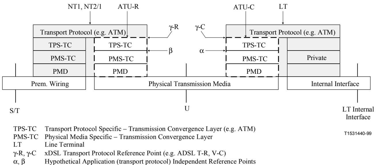
**Figure 9/G.995.1 – User plane protocol reference architecture**
