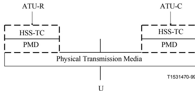
**Figure 13/G.995.1 – User plane protocol reference architecture for ITU-T G.994.1**
