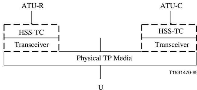
**Figure 11/G.995.1 – User plane protocol reference architecture for G.994.1**
