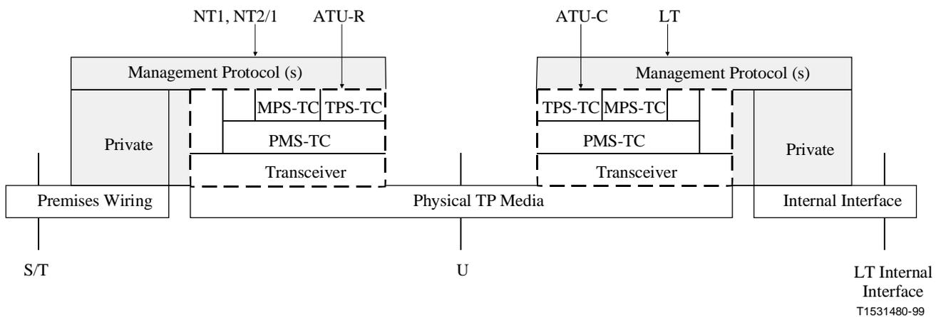
**Figure 12/G.995.1 – Management plane protocol reference architecture for G.99x-series Recommendations**
