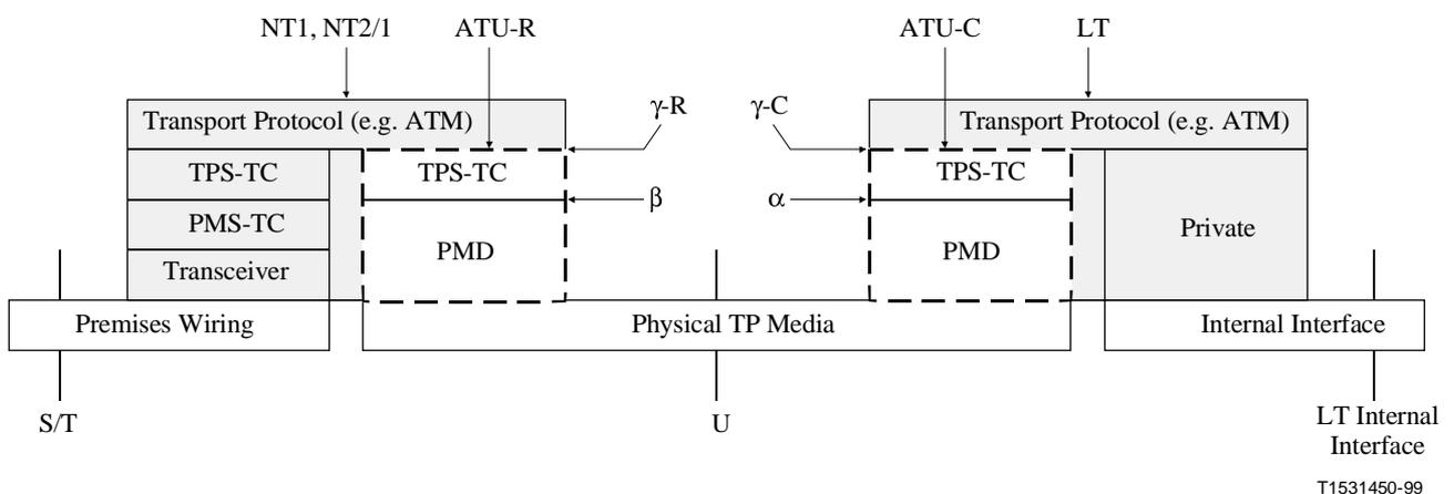
**Figure 9/G.995.1 – User plane protocol reference architecture for G.992.1 and G.992.2**
