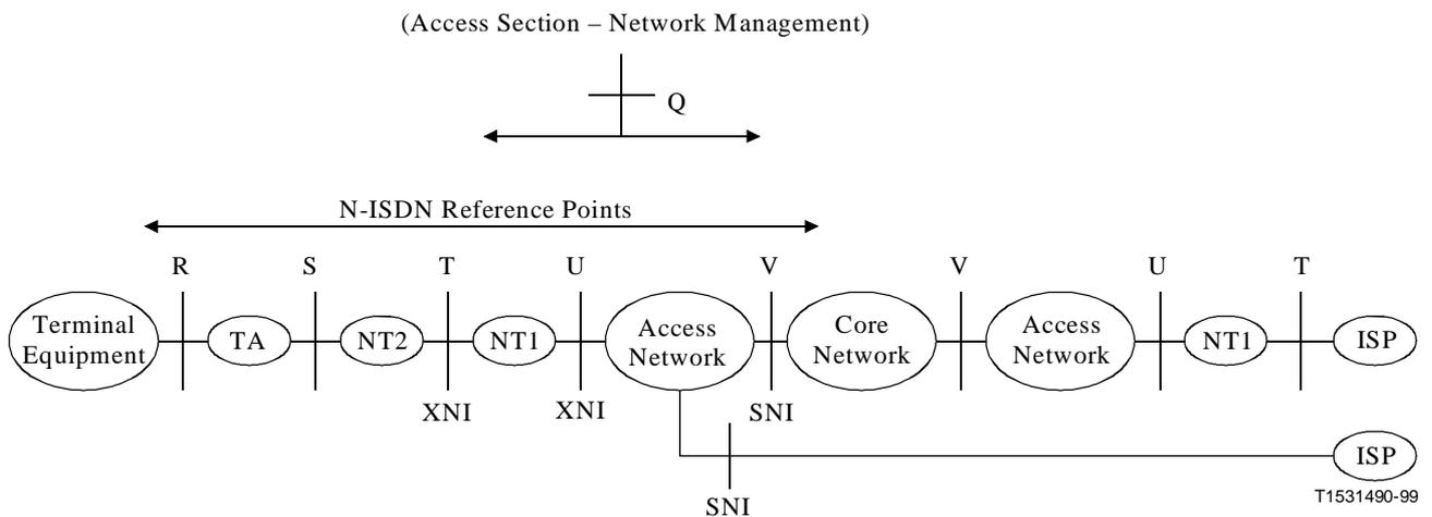
**Figure 13/G.995.1 – Illustration of a generic xDSL data Connection**
