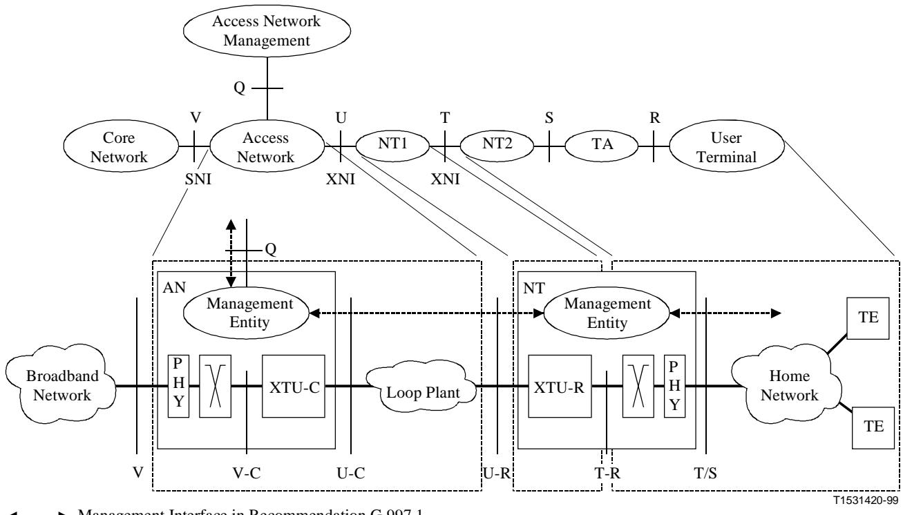
**Figure 6/G.995.1 – G.997.1 system reference model and its alignment with the generic reference configuration**
