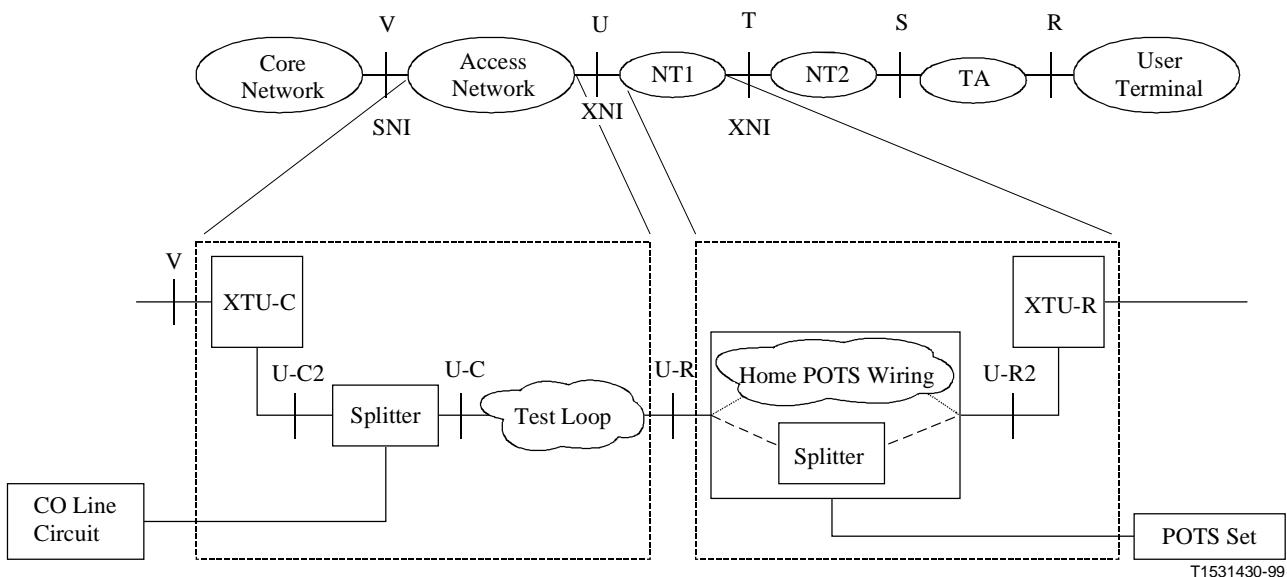
**Figure 7/G.995.1 – G.996.1 system reference model and its alignment with the generic reference configuration**
