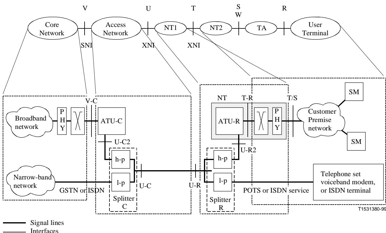
**Figure 2/G.995.1 – G.992.1 system reference model and its alignment with the generic reference configuration**
