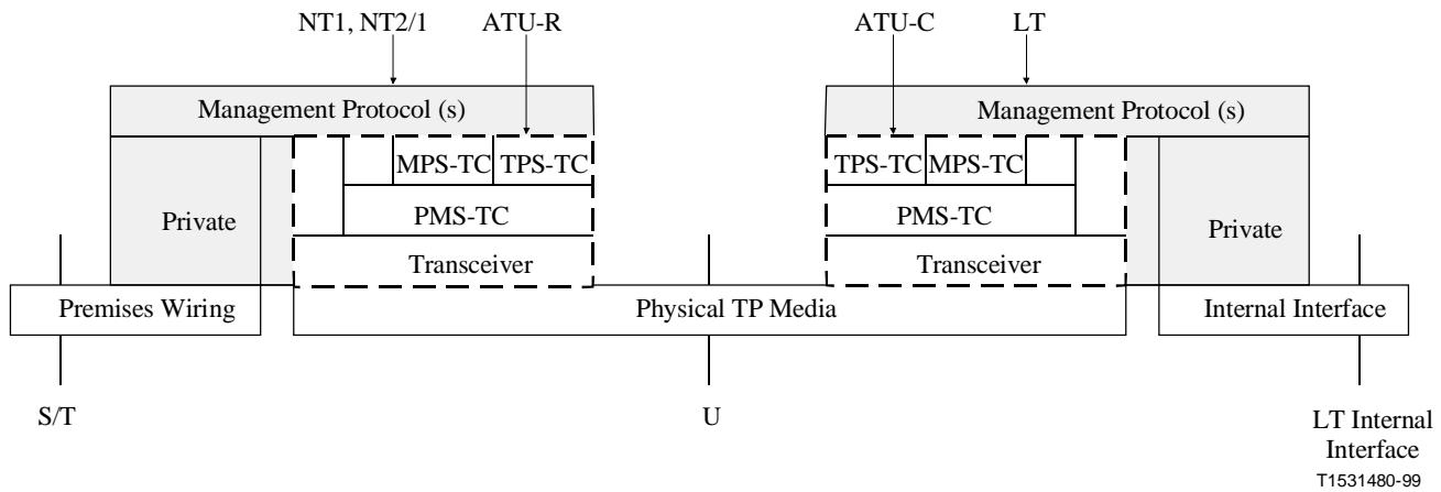
**Figure 12/G.995.1 – Management plane protocol reference architecture for G.99x-series Recommendations**
