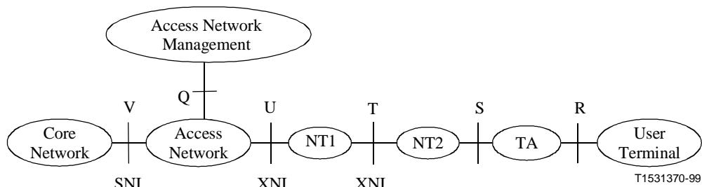
**Figure 1/G.995.1 – A reference configuration for a generic G.99x system**
