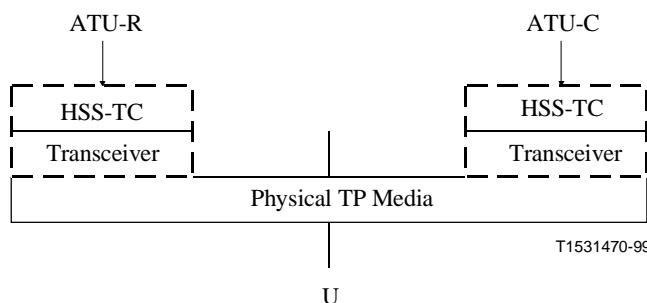
**Figure 11/G.995.1 – User plane protocol reference architecture for G.994.1**
