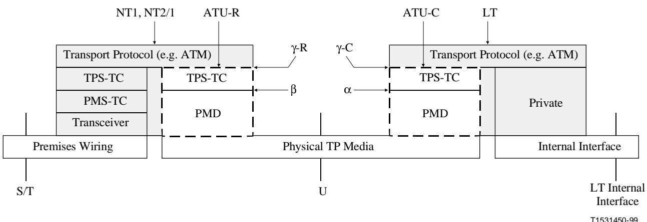
**Figure 9/G.995.1 – User plane protocol reference architecture for G.992.1 and G.992.2**
