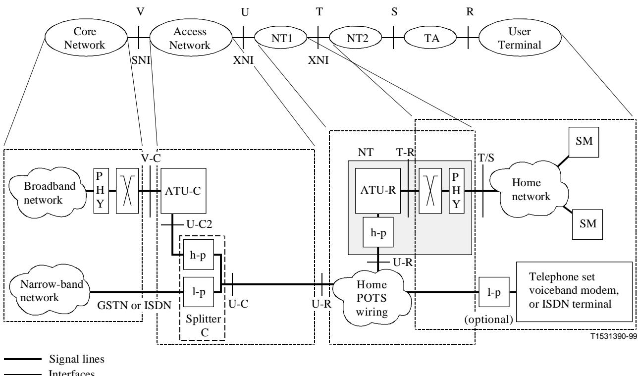
The G.992.2 system reference model shows the functional blocks useful to illustrate a G.992.2 transmission system. When comparing Figure 3 to the Figure 2 in 6.1.1.1, it may be observed that the main difference in the system reference model pertains to the absence of a separate POTS splitter functionality. The POTS splitter functionalities have now been distributed. The high-pass filter
