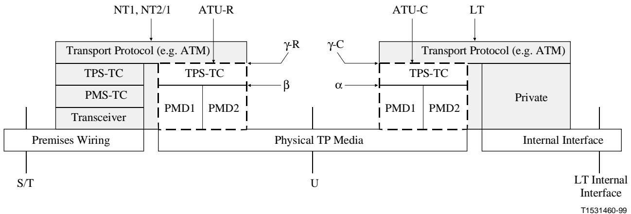
**Figure 10/G.995.1 – User plane protocol reference architecture for G.991.1**
