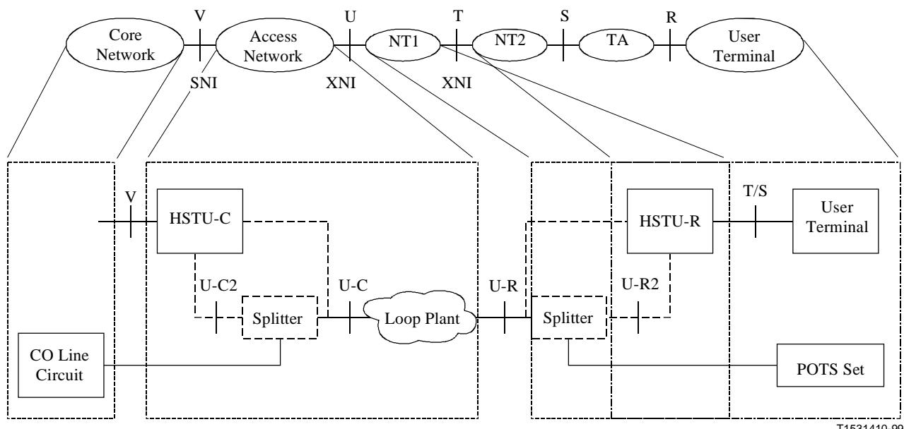
**Figure 5/G.995.1 – G.994.1 system reference model and its alignment with the generic reference configuration**
