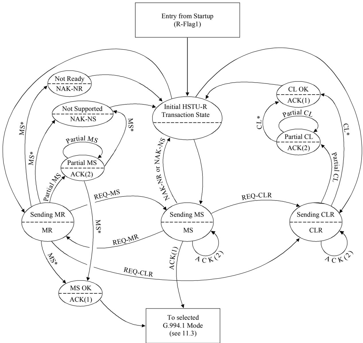
[Any State, including the Initial HSTU-R Transaction State]  $\xrightarrow{\text{(errored frame)}}$  Restart NAK-EF  $\rightarrow$  To R-Silent0, the Initial G.994.1 State for an HSTU-R (see clause 12)
