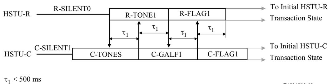
**Figure 15/G.994.1 – HSTU-C initiated duplex start-up procedure**
