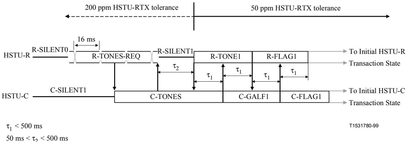
**Figure 14/G.994.1 – HSTU-R initiated duplex start-up procedure**
