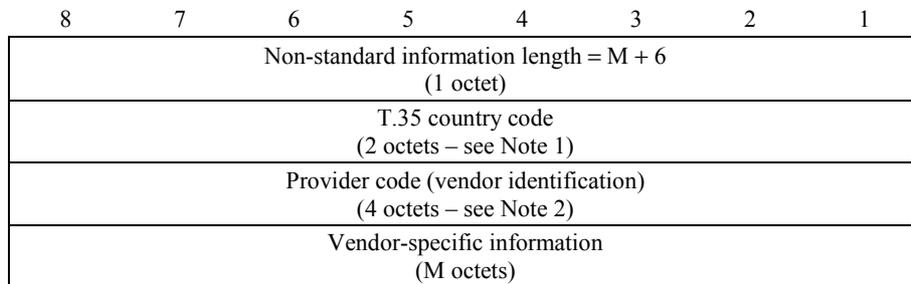
NOTE 1 – If the bits in the first octet are not all set to binary ONE, the bits in the second octet shall be set to binary ZERO by the transmitter and ignored by the receiver.
