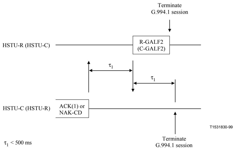
**Figure 19/G.994.1 – Half-duplex clear-down procedure**
