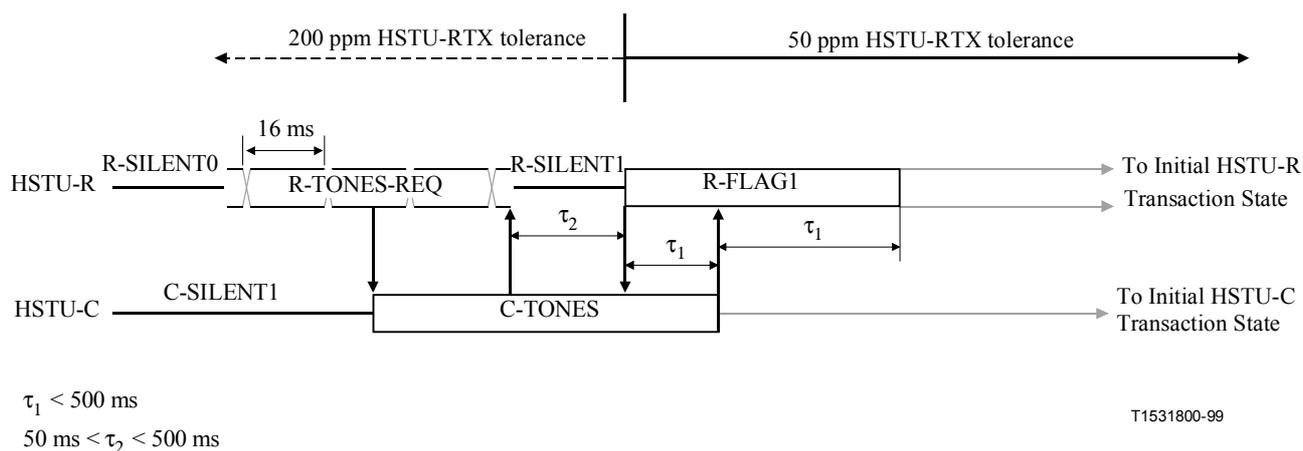
**Figure 16/G.994.1 – HSTU-R initiated half-duplex start-up procedure**
