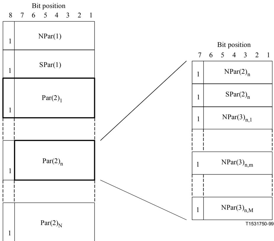
**Figure 8/G.994.1 – Order of transmission of NParS and SParS**
