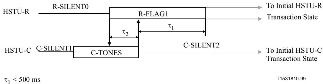
**Figure 17/G.994.1 – HSTU-C initiated half-duplex start-up procedure**
