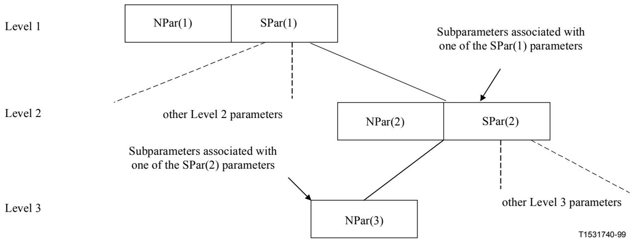
NPar(n) indicates a set of NPar parameters at level n in the tree.
