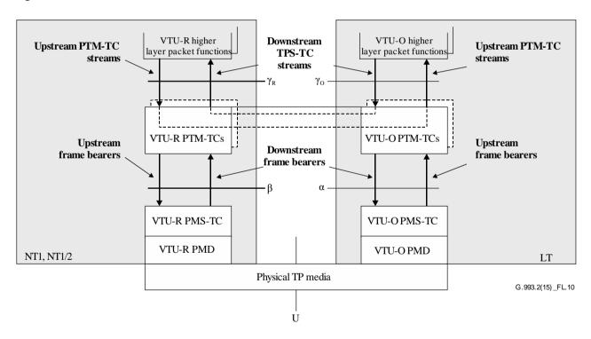
Figure L.10 – PTM-TC transport capabilities within the user plane
