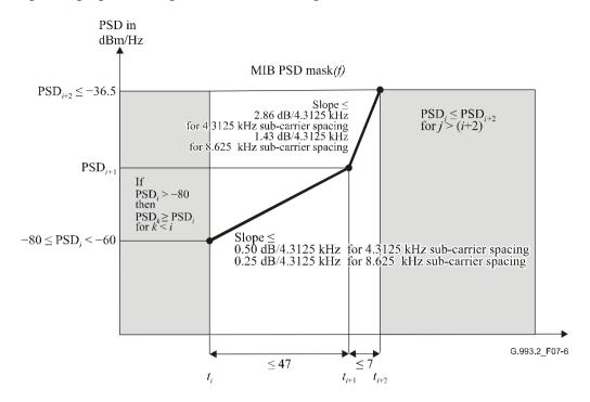
Figure 7-6 – Illustration of the two-slope steep upward shape
