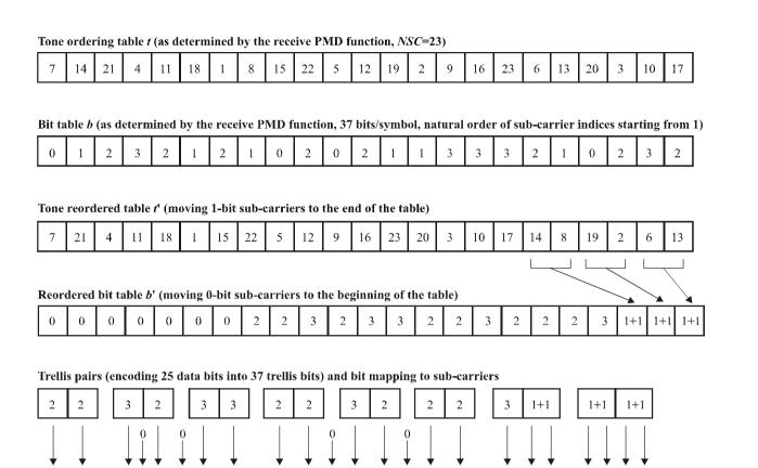
Figure 10-3 – Example of tone ordering and pairing of one-bit subcarriers
