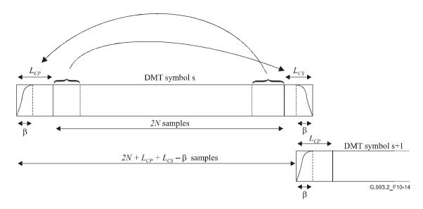
Figure 10-14 – Cyclic extension, windowing and overlap of DMT symbols
