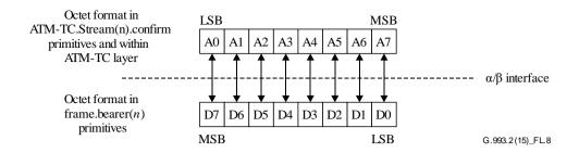
Figure L.8 – Bit mapping of the user plane transport function of the ATM-TC function
