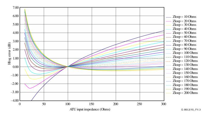
Figure II.3 – Hlog(f) error in dB as a function of loop and VTU impedance variations
