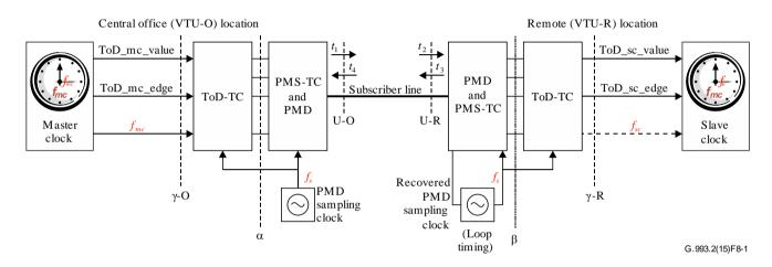
Figure 8-1 – End-to-end system reference model for time-of-day transport in VDSL2
