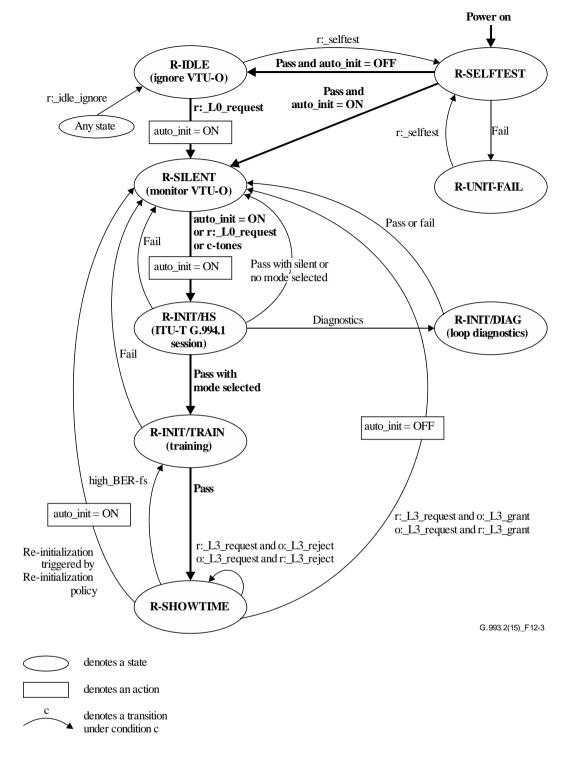
Figure 12-3 – State diagram for the VTU-R
