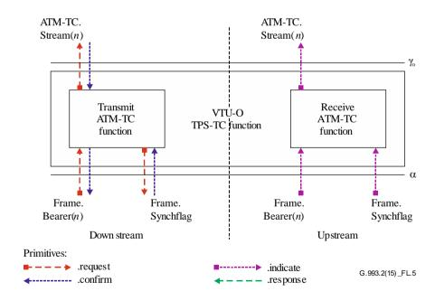
Figure L.5 – Signals of the VTU-O ATM-TC function
