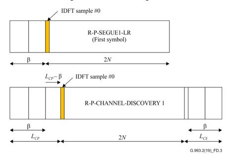
Figure D.3 – Reference samples for alignment of upstream symbols between the VDSL2-LR TRAINING stage and ITU-T G.993.2 channel discovery phase
