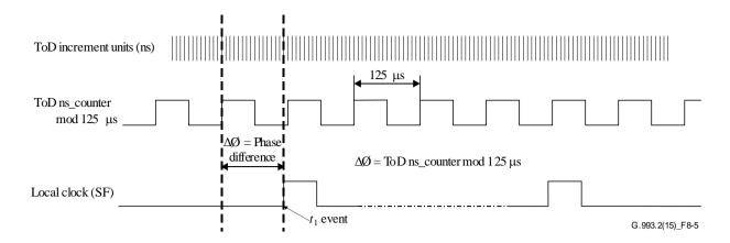
Figure 8-5 – ToD phase difference ( $\Delta \phi$ ) computation
