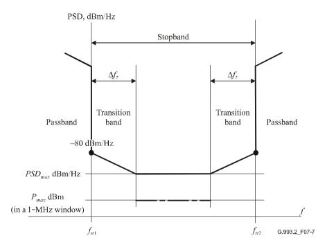
Figure 7-7 – Limit PSD mask and wide-band power limit in the stopbands
