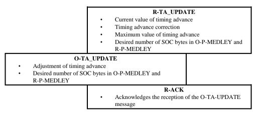
Figure 12-9 – SOC message exchange during the training phase
