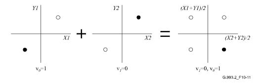
Figure 10-11 – Combination of a pair of 1-bit constellations to build a 2-bit constellation
