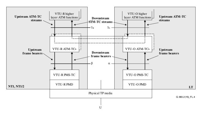
Figure L.4 – ATM-TC transport capabilities within the user plane
