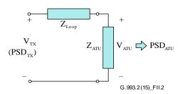
Figure II.2 – Measurement of PSD received by VTU
