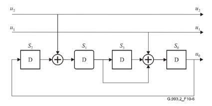
Figure 10-6 – Convolutional encoder: Finite state machine representation
