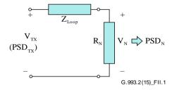
Figure II.1 – Measurement of received PSD by network or spectrum analyzer
