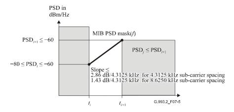
Figure 7-5 – Illustration of the one-slope steep upward shape
