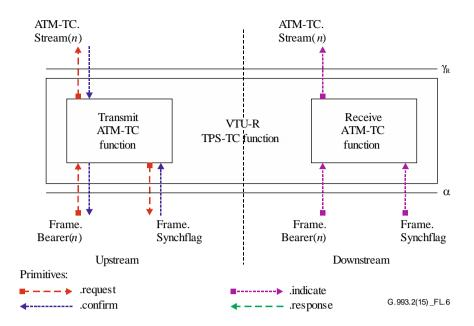
Figure L.6 – Signals of the VTU-R ATM-TC function
