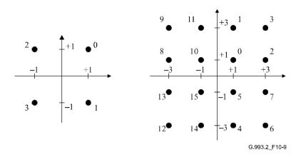
Figure 10-9 – Constellation labels for b=2 and b=4
