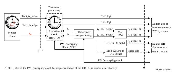
Figure 8-4 – Functional reference model for ToD-TC in the VTU-O
