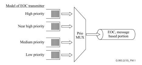
Figure M.1 – Model of the eoc transmitter
