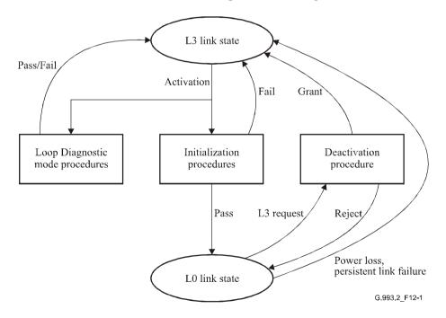
Figure 12-1 – VDSL2 link states and link state diagram
