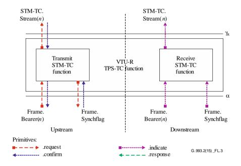
Figure L.3 – Signals of the VTU-R STM-TC function
