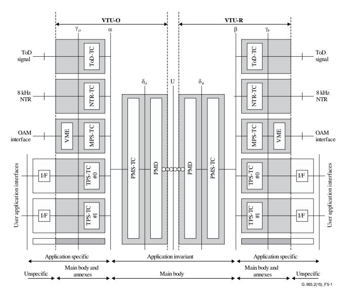
Figure 5-1 – VDSL2 and VTU functional model
