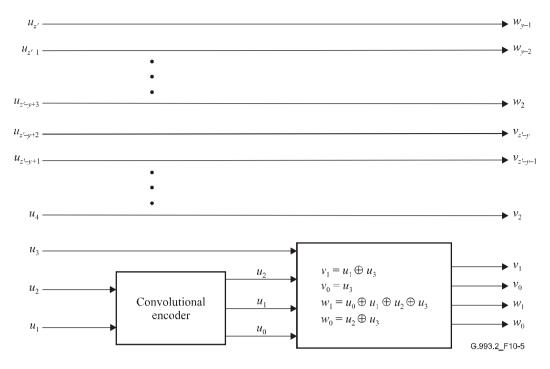
Figure 10-5 – Conversion of u to v and w
