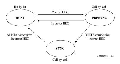
Figure L.9 – Cell delineation procedure state machine
