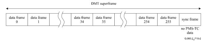
Figure 10-2 – DMT superframe structure
