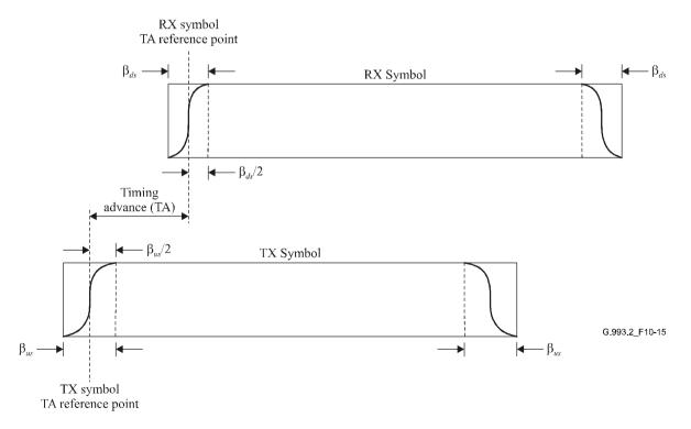
Figure 10-15 – Illustration of TA (VTU-R)
