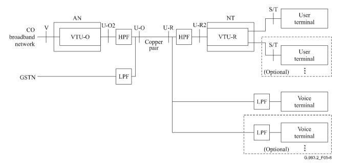
Figure 5-8 – Data with POTS service application model for splitterless remote deployment
