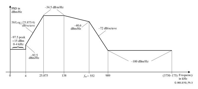
Figure A.3 – VTU-R EU-128 Limit PSD mask for operation over POTS
