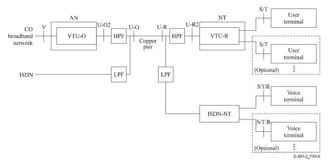
Figure 5-9 – Data with ISDN service application model
