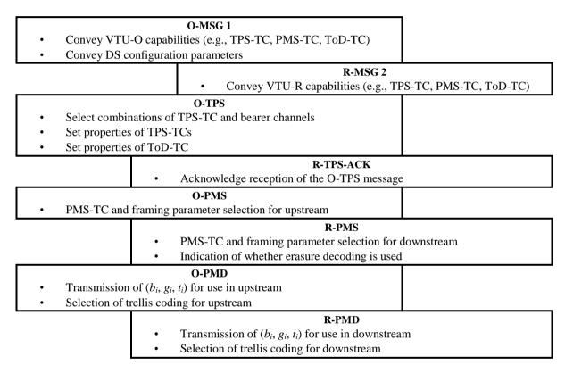
Figure 12-11 – SOC messages exchanged during the channel analysis and exchange phase
