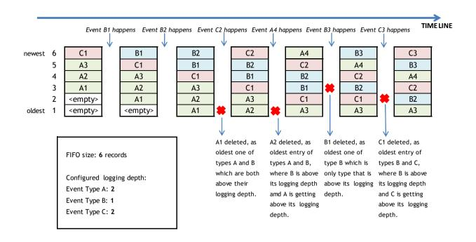
Figure 11-6 – Illustration of the buffer management rules
