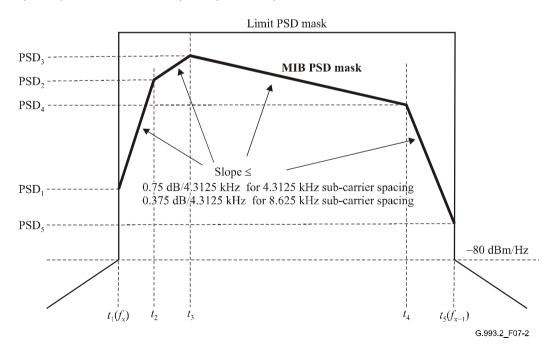
Figure 7-2 – Illustration of a MIB PSD mask in the case all breakpoint  $PSD_n$  values are greater than -80 dBm/Hz
