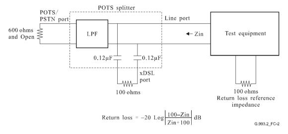
Figure C.2 – Impedance measurements in the band between 12 MHz and 30 MHz for the CO and remote POTS splitters
