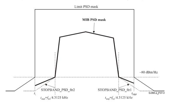
Figure 7-3 – Illustration of the restrictions on breakpoints for a case in which the MIB PSD mask lies below -80 dBm/Hz between two band separating frequencies ( $t_1$  and  $t_{NBP}$ ) but above -80 dBm/Hz for some frequency range inside the band
