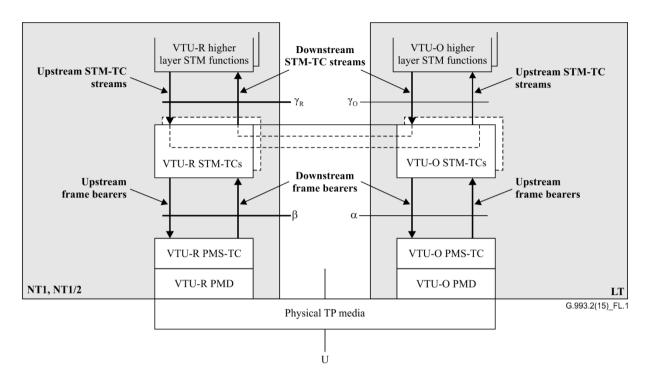
Figure L.1 – STM-TC transport capabilities within the user plane
