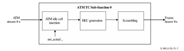
Figure L.7 – Block diagram of transmit ATM-TC function
