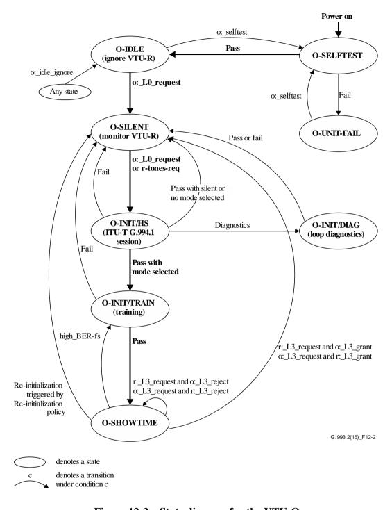
Figure 12-2 – State diagram for the VTU-O
