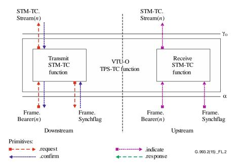
Figure L.2 – Signals of the VTU-O STM-TC function
