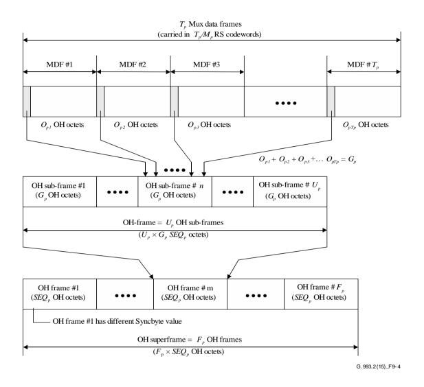
Figure 9-4 – Overhead subframe, frame, and superframe structure
