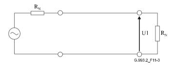
Figure 11-3 – Voltage across the load
