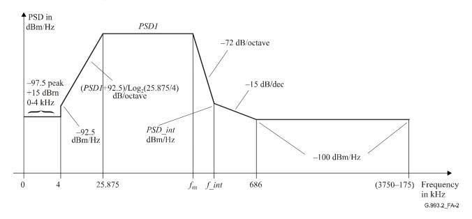
Figure A.2 – VTU-R US0 Limit PSD mask for operation over POTS
