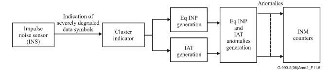
Figure 11-5 – Impulse noise monitor functional block diagram
