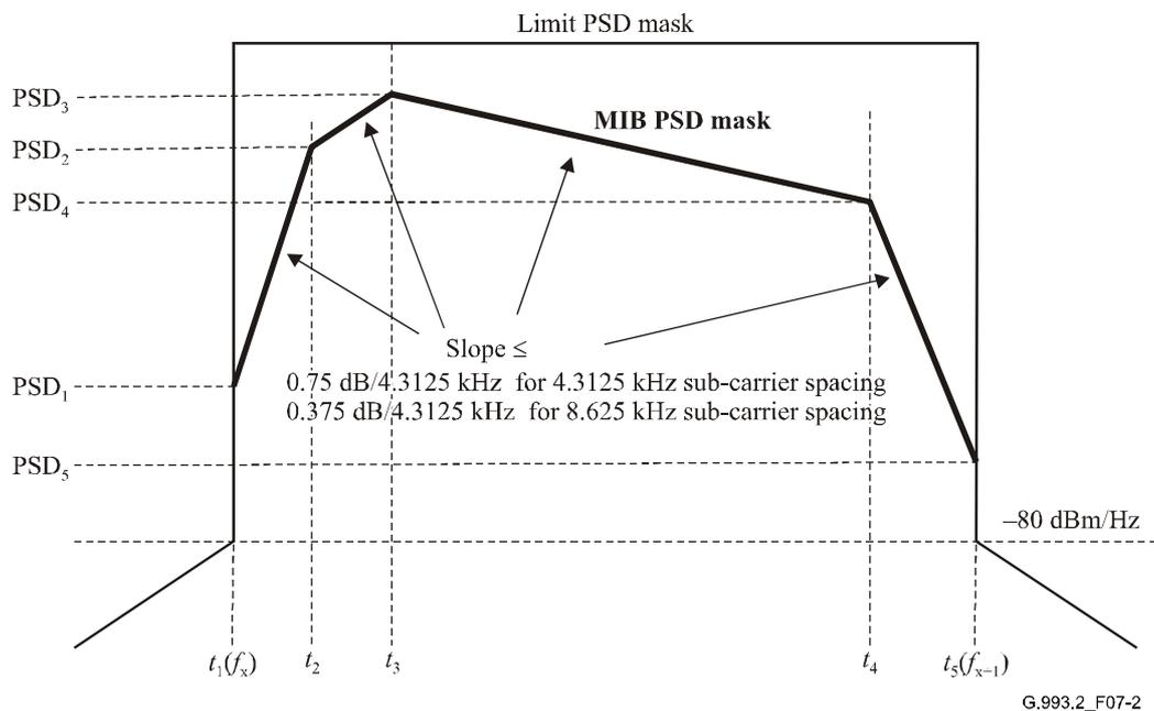
**Figure 7-2/G.993.2 – Illustration of a MIB PSD mask in the case all breakpoint PSD<sub>n</sub> values are greater than -80 dBm/Hz**
