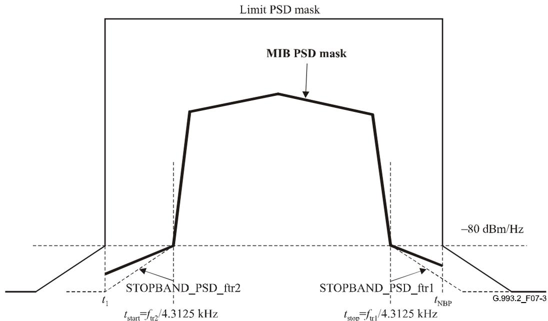
**Figure 7-3/G.993.2 – Illustration of the restrictions on breakpoints for a case in which the MIB PSD mask lies below  $-80$  dBm/Hz between two band separating frequencies ( $t_1$  and  $t_{NBP}$ ) but above  $-80$  dBm/Hz for some frequency range inside the band**
