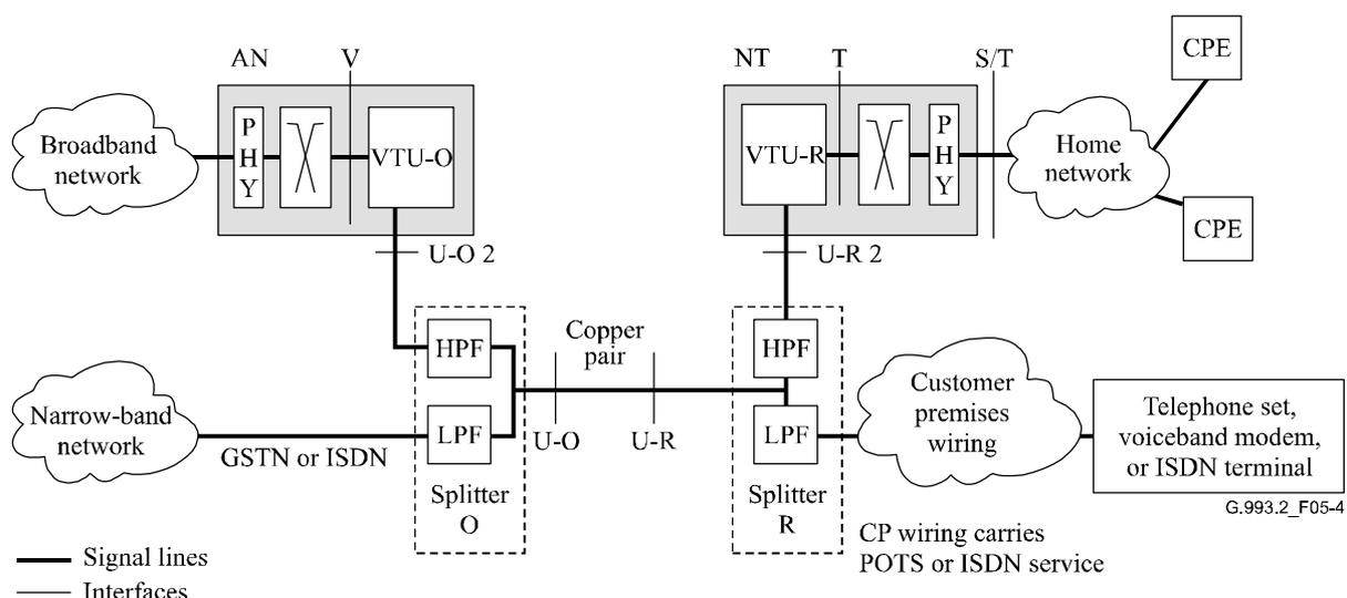
**Figure 5-4/G.993.2 – Generic application reference model for remote deployment with splitter**
