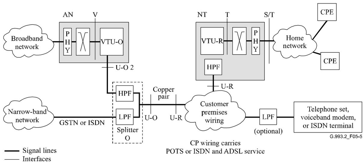
**Figure 5-5/G.993.2 – Generic application reference model for splitterless remote deployment**
