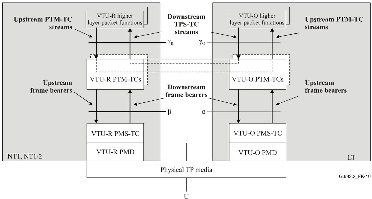
**Figure K.10/G.993.2 – PTM-TC transport capabilities within the user plane**
