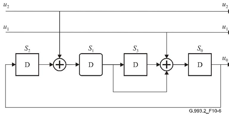
Figure 10-6/G.993.2 – Convolutional encoder: Finite state machine representation
