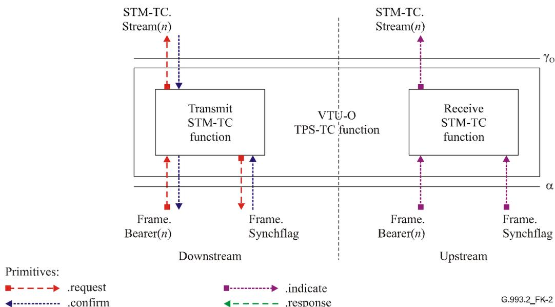
**Figure K.2/G.993.2 – Signals of the VTU-O STM-TC function**
