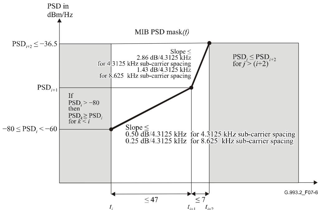
**Figure 7-6/G.993.2 – Illustration of the two-slope steep upward shape**
