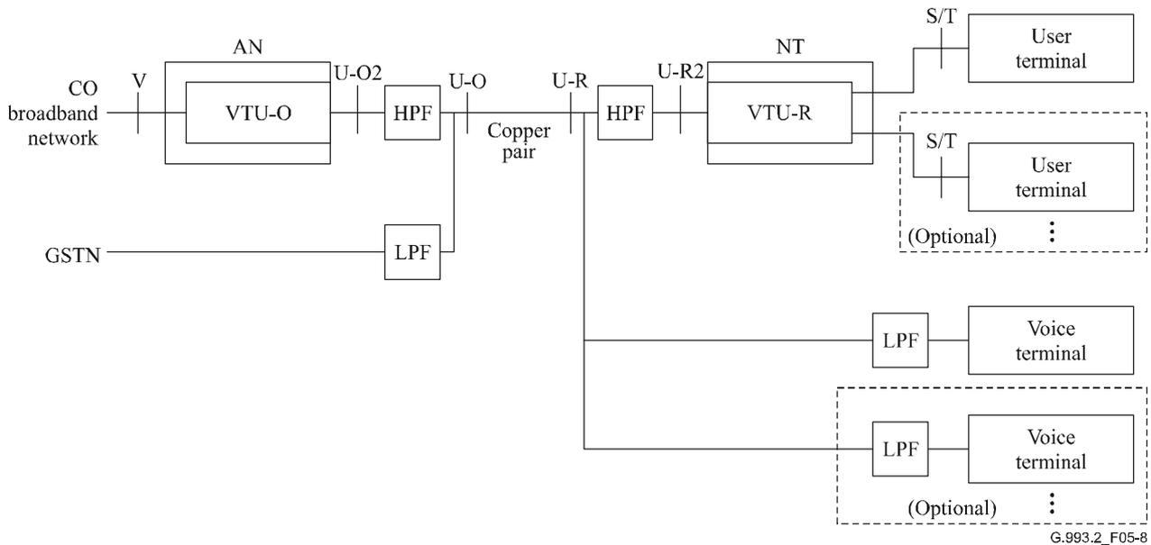
**Figure 5-8/G.993.2 – Data with POTS service application model for splitterless remote deployment**
