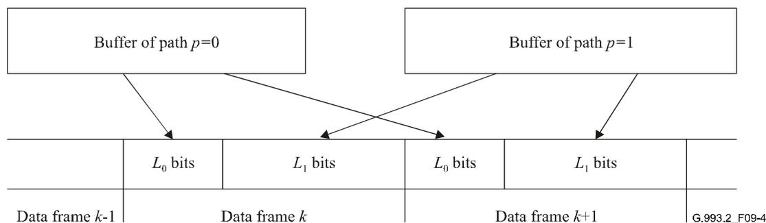
**Figure 9-4/G.993.2 – Multiplexing of two latency paths into data frames carried by DMT symbols**
