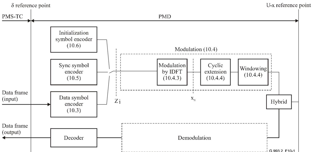
Figure 10-1/G.993.2 – Functional model of PMD sub-layer
