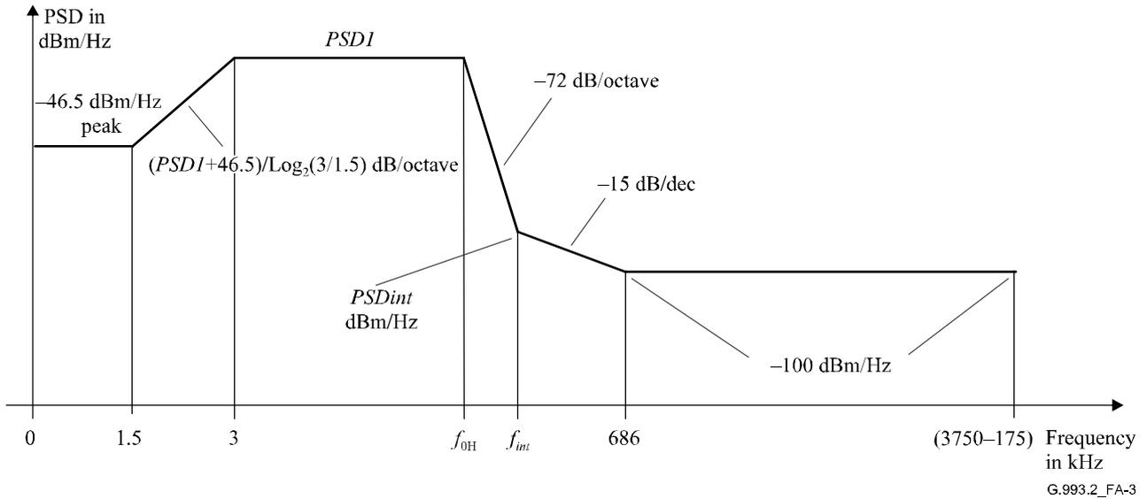
Figure A.3/G.993.2 – VTU-R US0 transmitter PSD mask for all-digital mode operation
