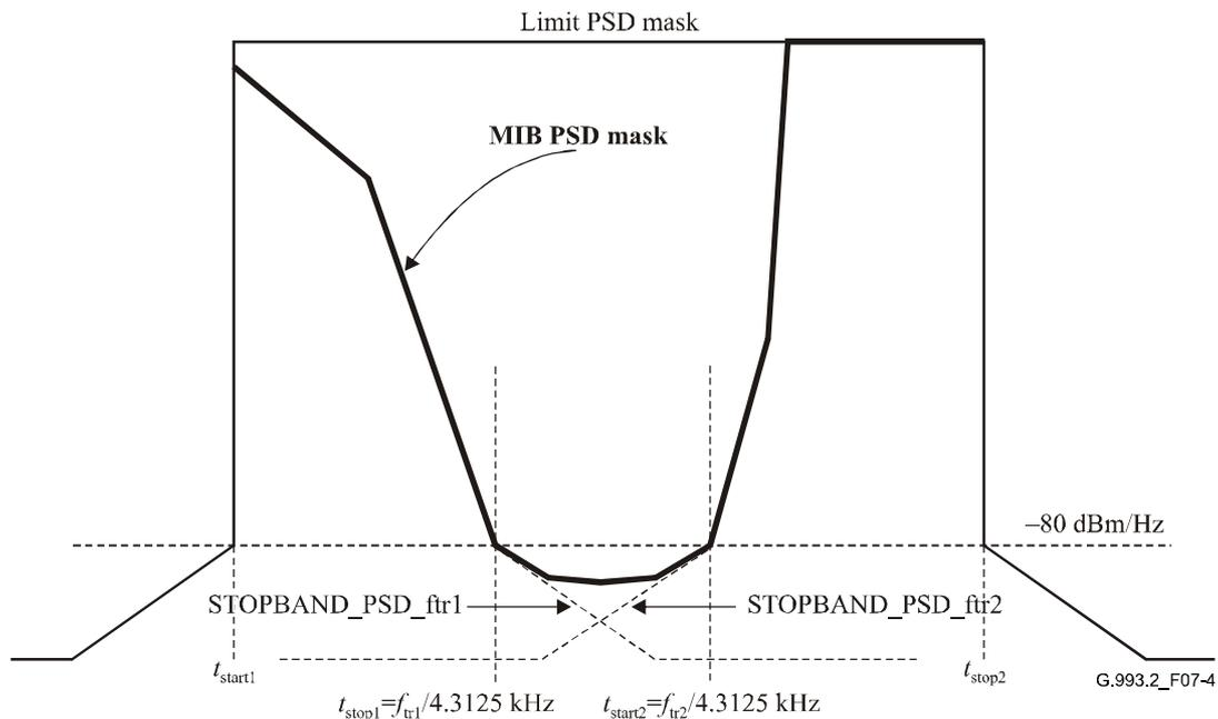
**Figure 7-4/G.993.2 – Illustration of the restrictions on breakpoints for a frequency band in which the MIB PSD lies below  $-80$  dBm/Hz between two frequency ranges where the PSD is above  $-80$  dBm/Hz**
