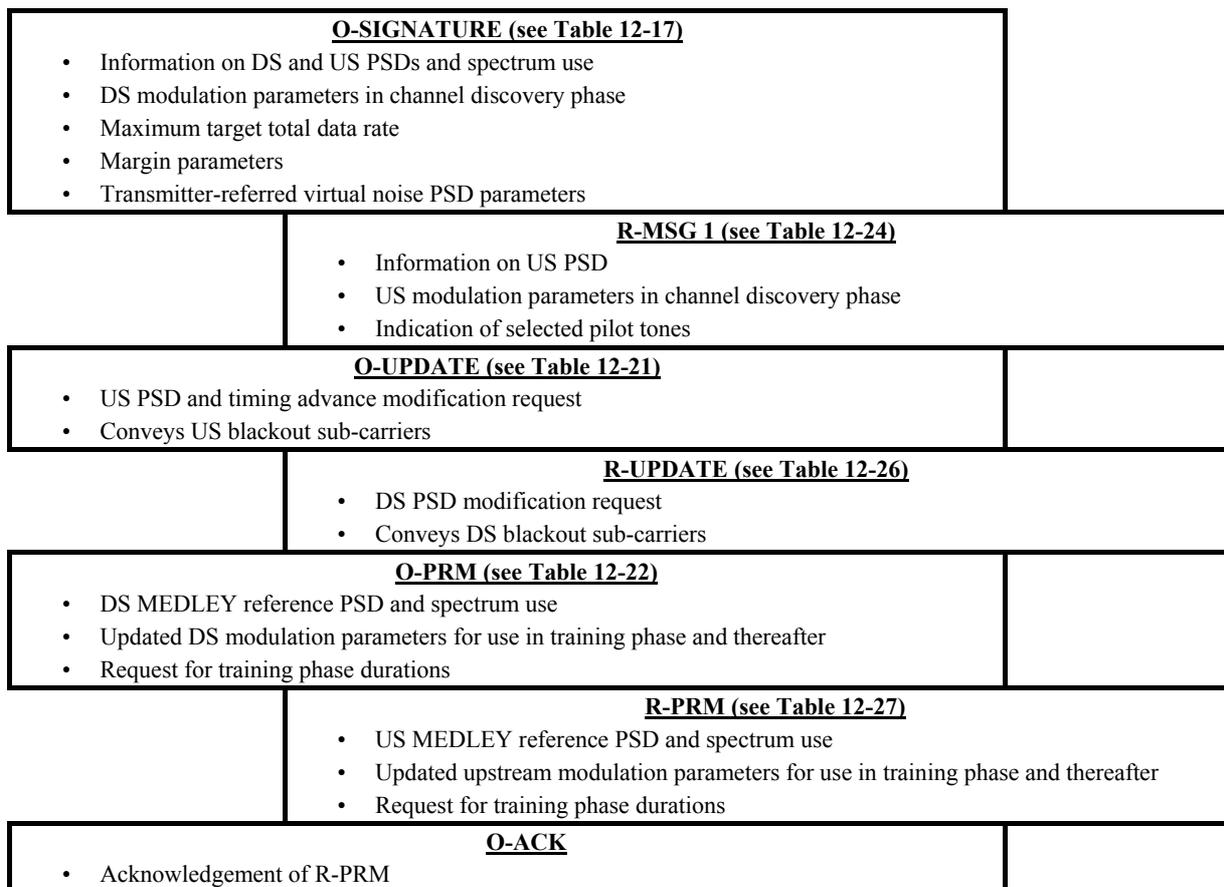
**Figure 12-5/G.993.2 – SOC message exchange during the channel discovery phase**
