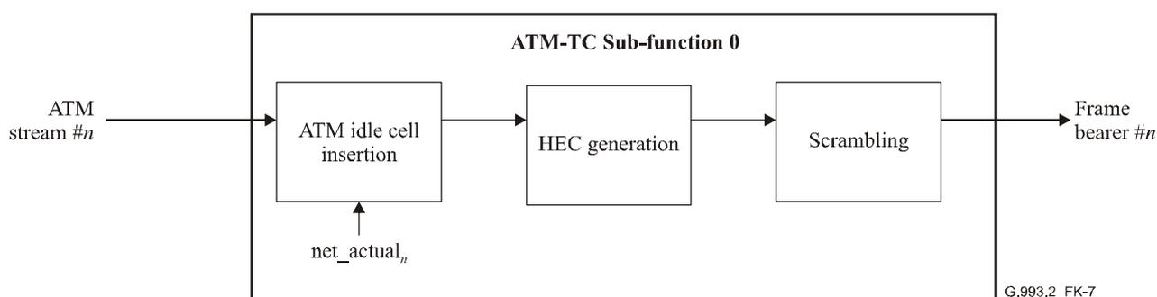
**Figure K.7/G.993.2 – Block diagram of transmit ATM-TC function**
