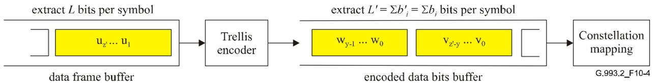
**Figure 10-4/G.993.2 – Relationship of trellis encoder and constellation mapping**
