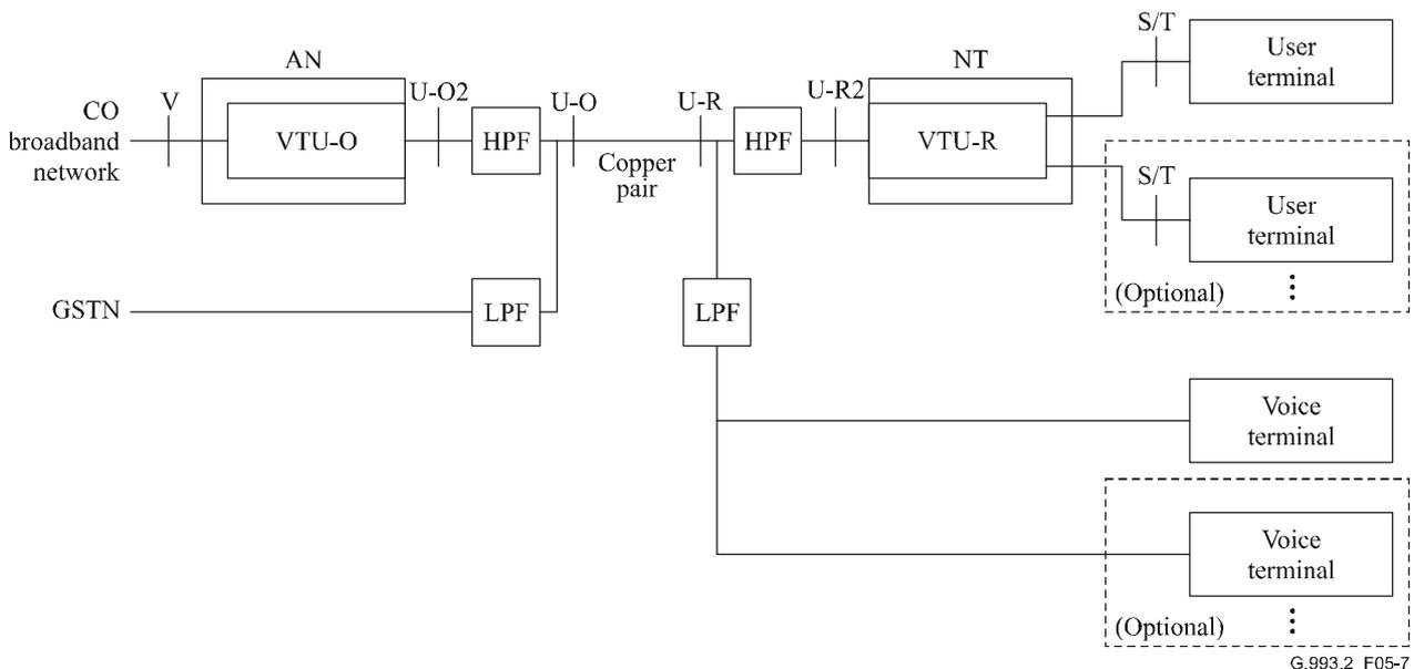
**Figure 5-7/G.993.2 – Data with POTS service application model for remote deployment with splitter**
