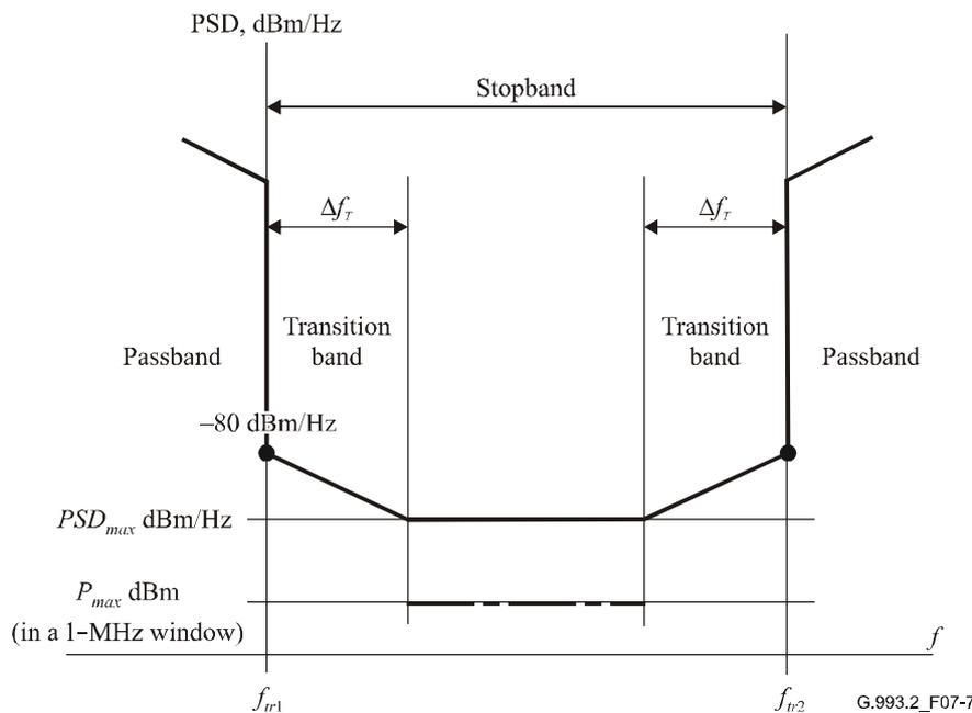
**Figure 7-7/G.993.2 – Limit PSD mask and wide-band power limit in the stopbands**
