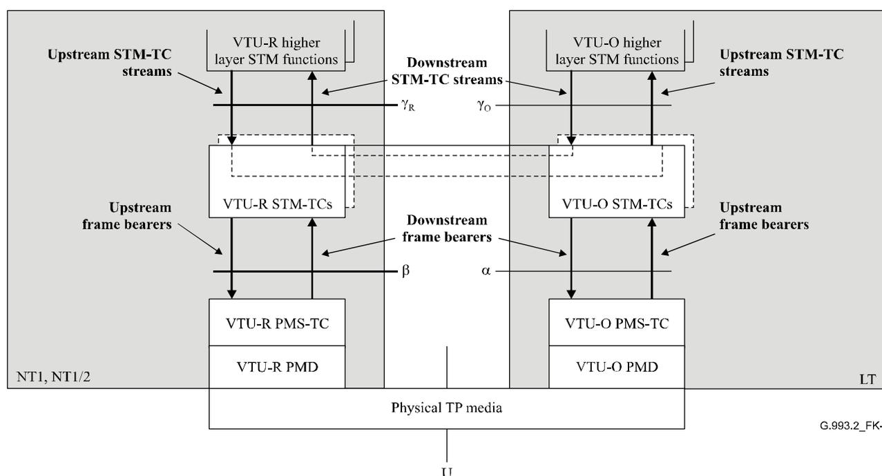
**Figure K.1/G.993.2 – STM-TC transport capabilities within the user plane**
