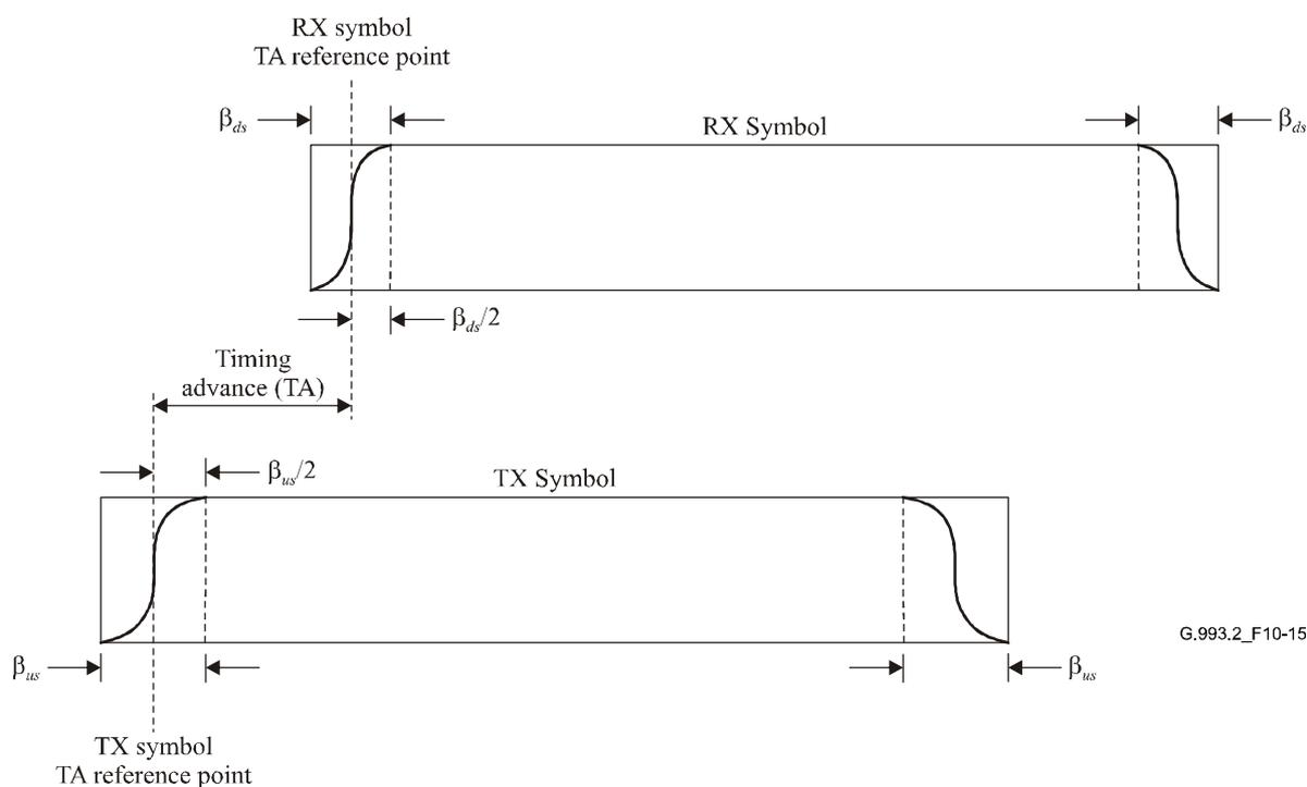
**Figure 10-15/G.993.2 – Illustration of TA (VTU-R)**
