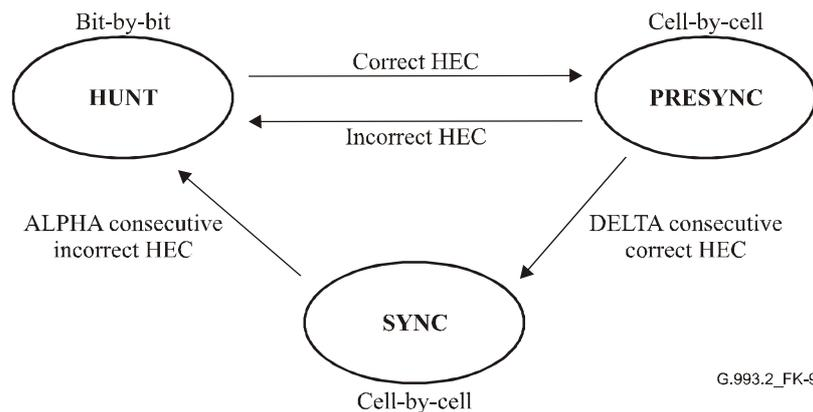
Figure K.9/G.993.2 – Cell delineation procedure state machine
