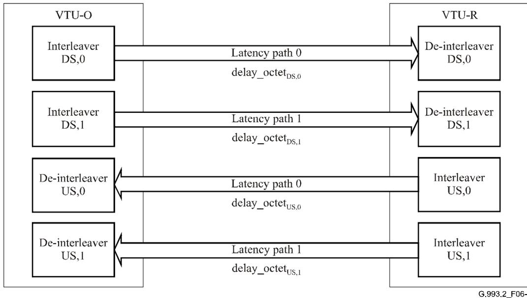
**Figure 6-1/G.993.2 – Illustration of all latency paths composing the aggregate interleave and de-interleave delay specified in each profile**
