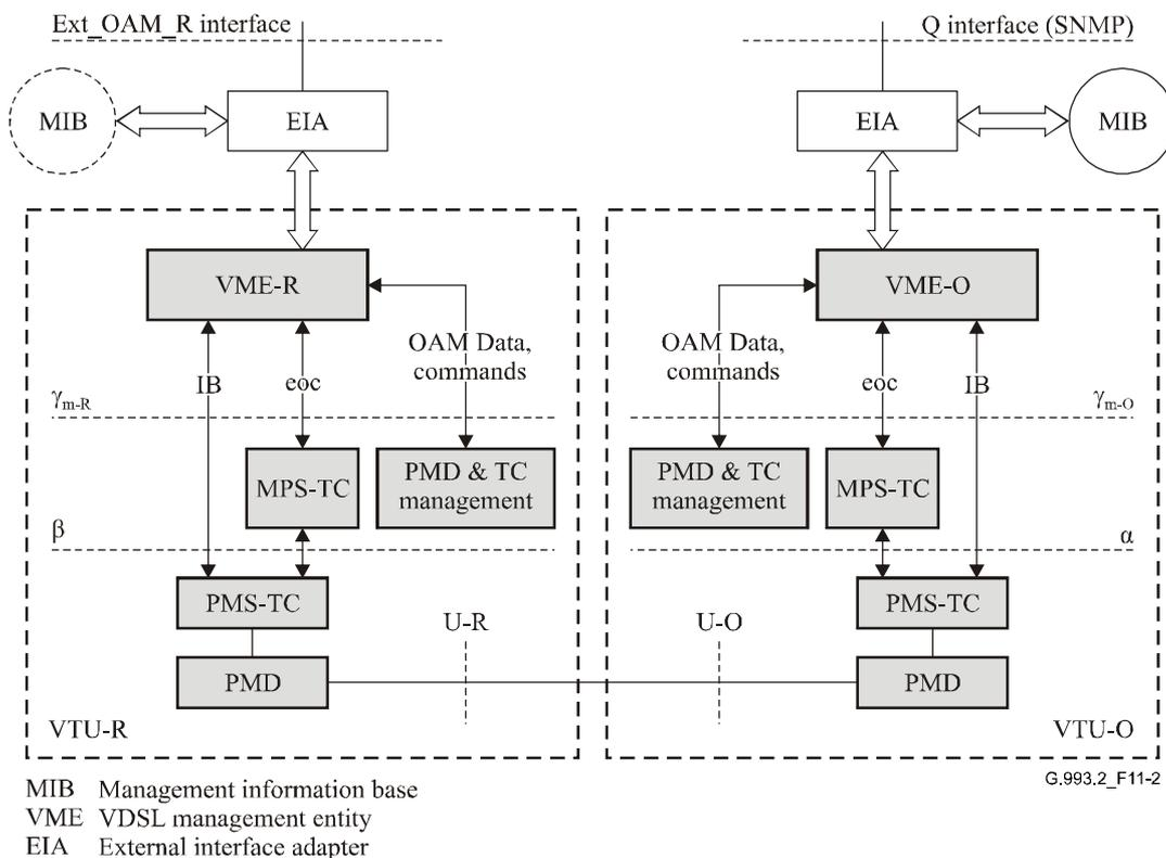
**Figure 11-2/G.993.2 – Functional model of OAM of the VDSL2 link**
