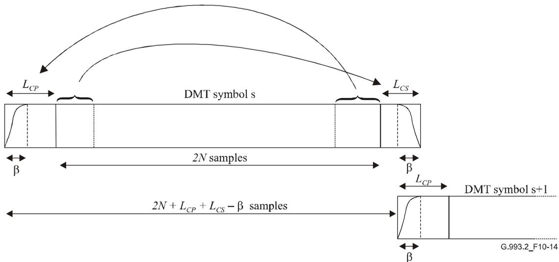
Figure 10-14/G.993.2 – Cyclic extension, windowing and overlap of DMT symbols
