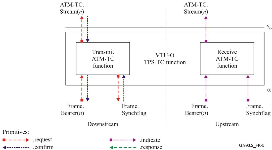
Figure K.5/G.993.2 – Signals of the VTU-O ATM-TC function
