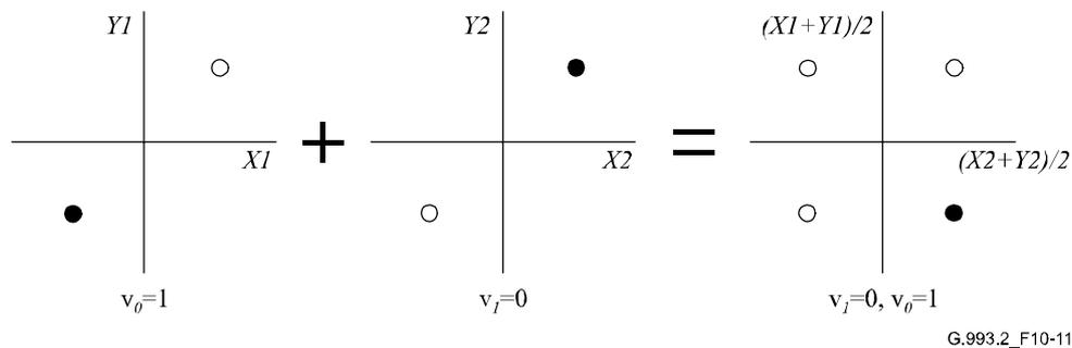
**Figure 10-11/G.993.2 – Combination of a pair of 1-bit constellations to build a 2-bit constellation**
