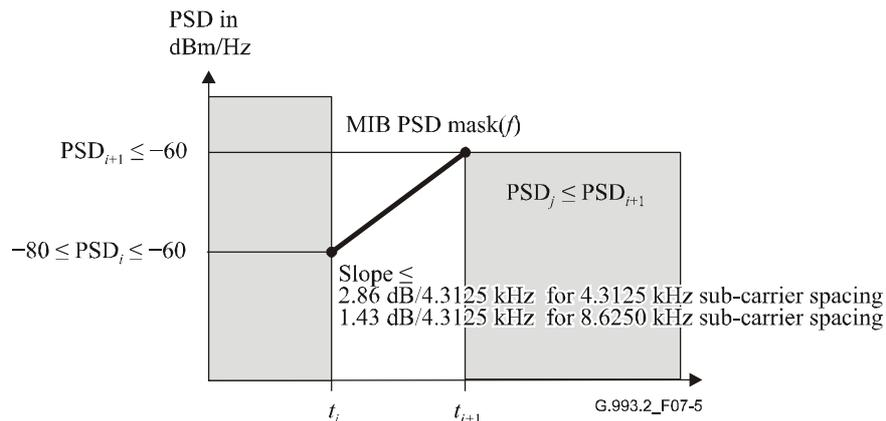
**Figure 7-5/G.993.2 – Illustration of the one-slope steep upward shape**
