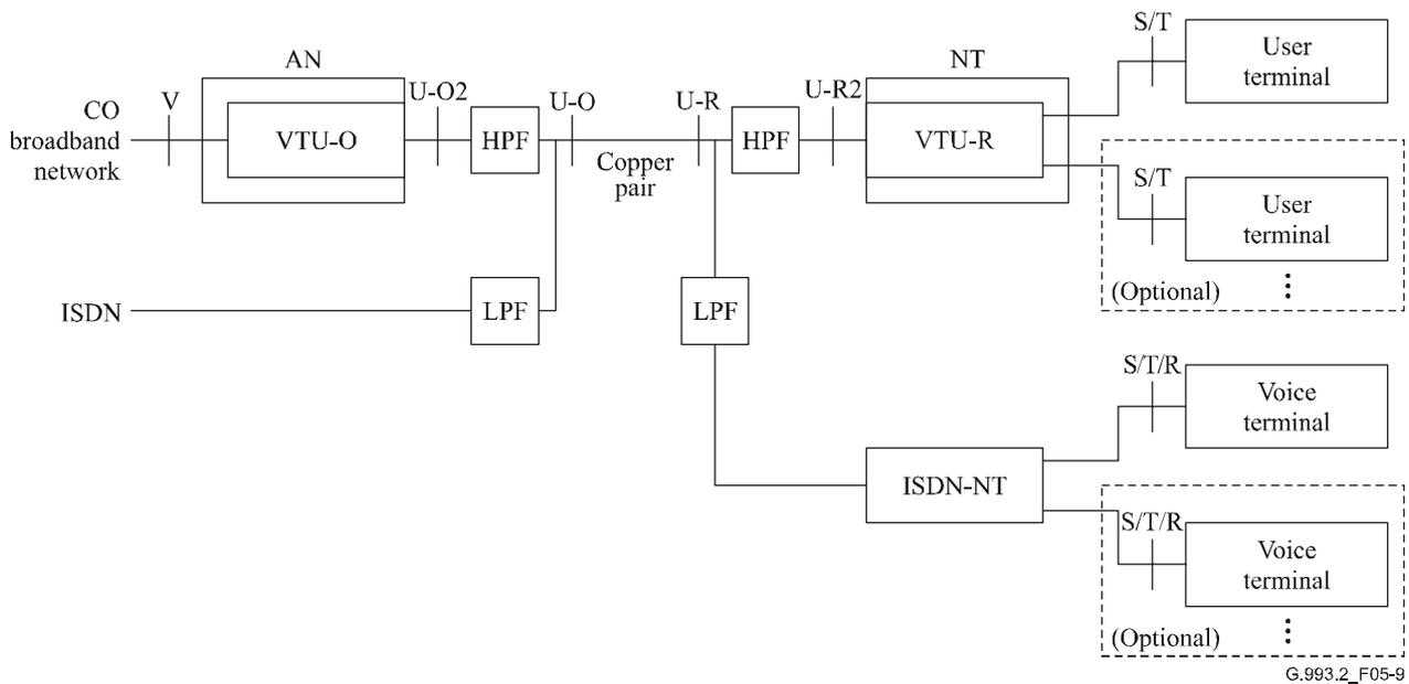
**Figure 5-9/G.993.2 – Data with ISDN service application model**
