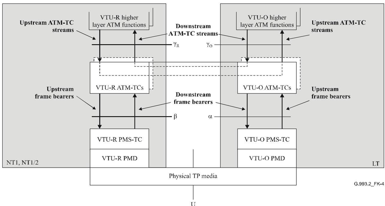
**Figure K.4/G.993.2 – ATM-TC transport capabilities within the user plane**
