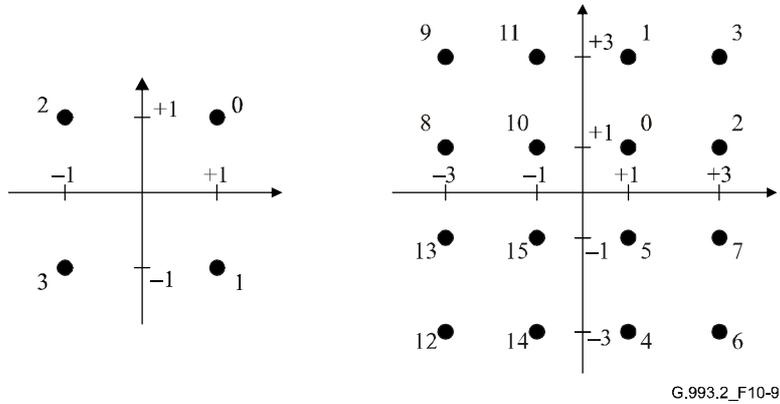
**Figure 10-9/G.993.2 – Constellation labels for  $b = 2$  and  $b = 4$**
