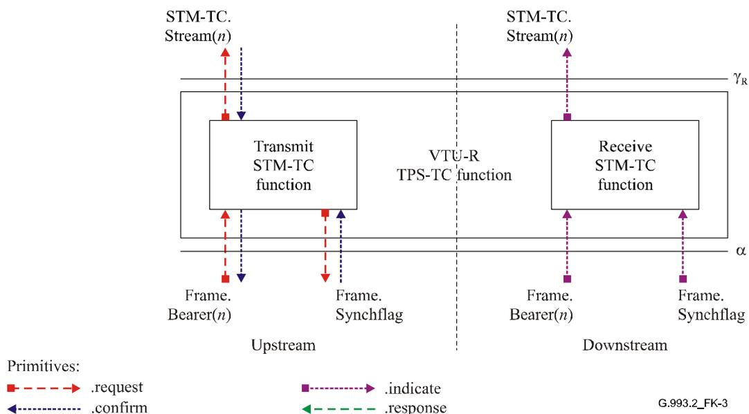
**Figure K.3/G.993.2 – Signals of the VTU-R STM-TC function**
