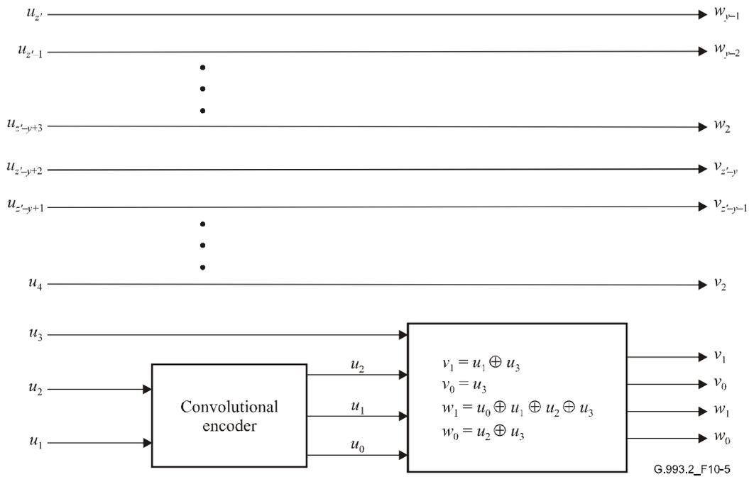
Figure 10-5/G.993.2 – Conversion of  $u$  to  $v$  and  $w$
