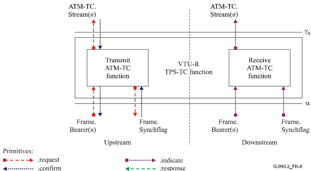
Figure K.6/G.993.2 – Signals of the VTU-R ATM-TC function
