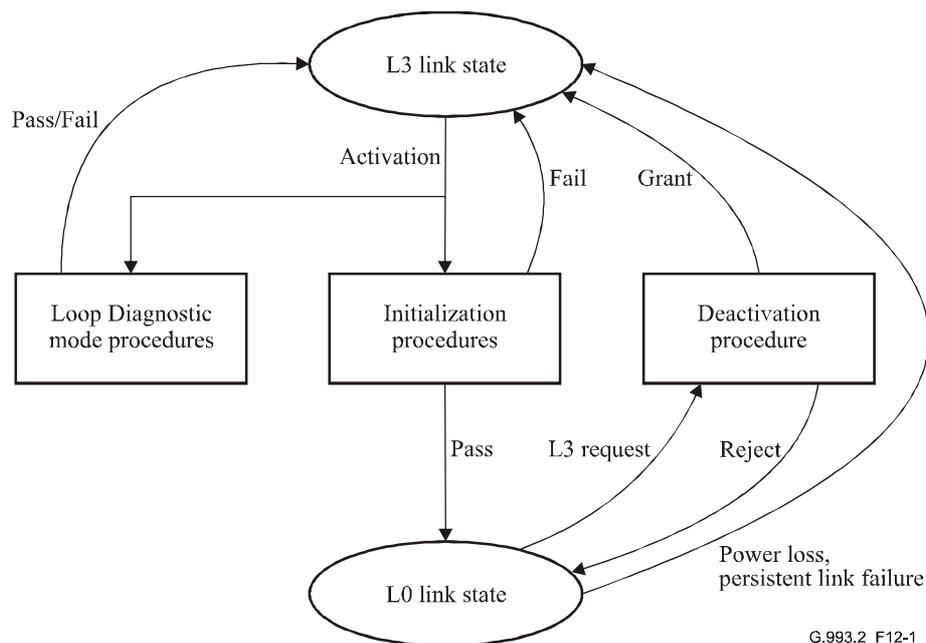
Figure 12-1/G.993.2 – VDSL2 link state and activation/deactivation procedures diagram
