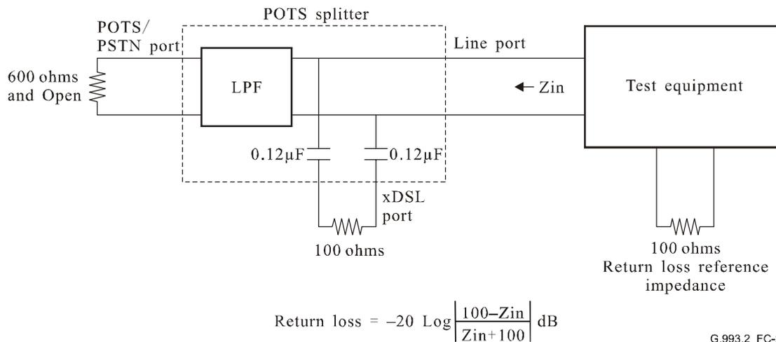
**Figure C.2/G.993.2 – Impedance measurements in the band between 12 MHz and 30 MHz for the CO and remote POTS splitters**
