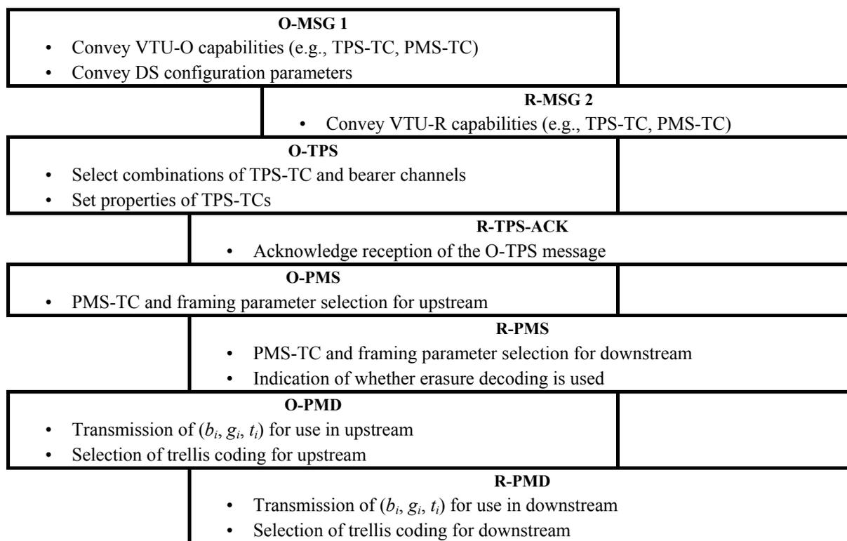
**Figure 12-9/G.993.2 – SOC messages exchanged during the channel analysis & exchange phase**
