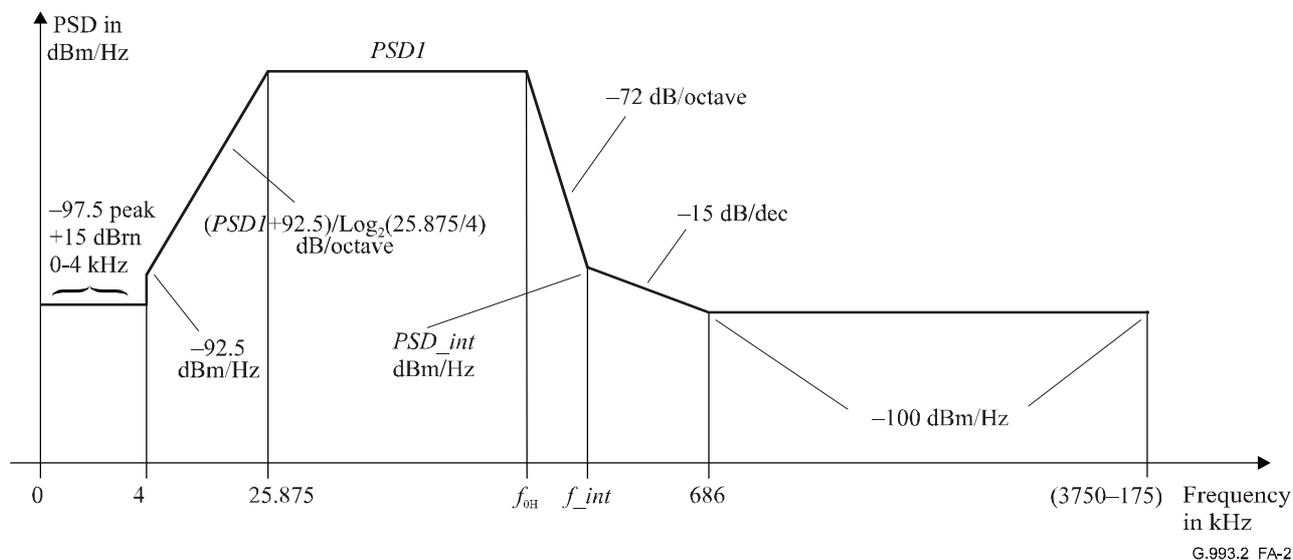
**Figure A.2/G.993.2 – VTU-R US0 transmitter PSD mask for operation over POTS**
