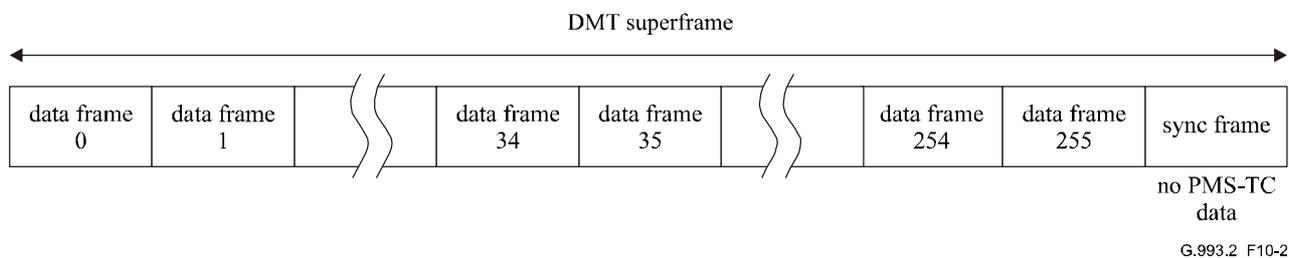
Figure 10-2/G.993.2 – DMT superframe structure
