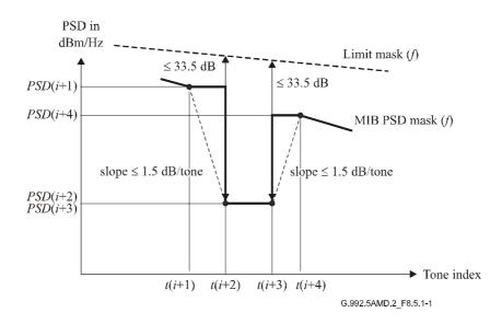
Figure 8.5.1-1/G.992.5 – Restrictions on breakpoints and MIB PSD mask (f)
