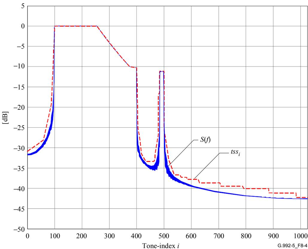
**Figure 8-4/G.992.5 – Example of the downstream  $\log_{10} tss_i$  values (in dB) as function of the subcarrier index**
