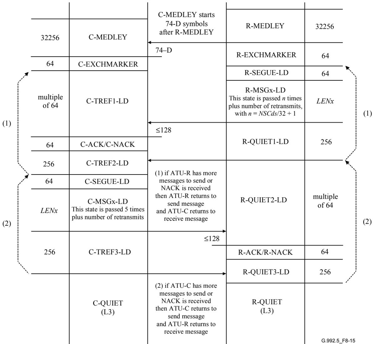
Figure 8-15/G.992.5 – Loop diagnostics timing diagram (part 2)
