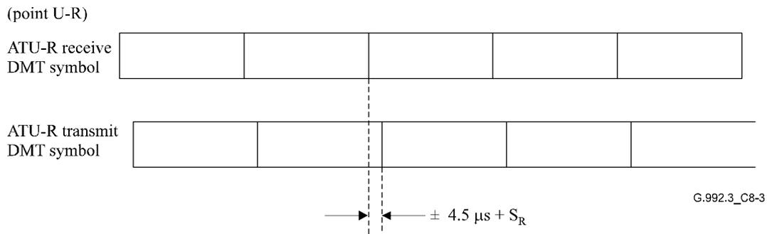
Figure C.8-3/G.992.3 – Loop timing for ATU-R
