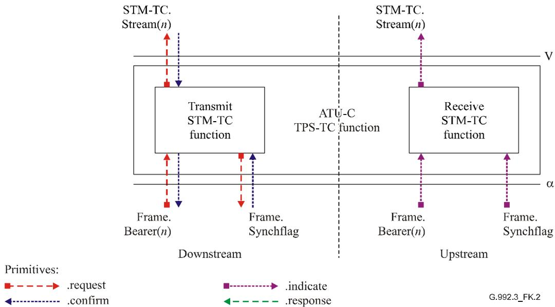
**Figure K.2/G.992.3 – Signals of the ATU-C STM-TC function**
