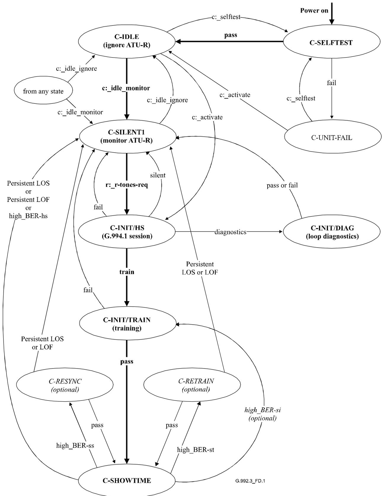
NOTE 1 – Events are received from the ATU-C host controller (c:\_) or from the ATU-R (r:\_).
