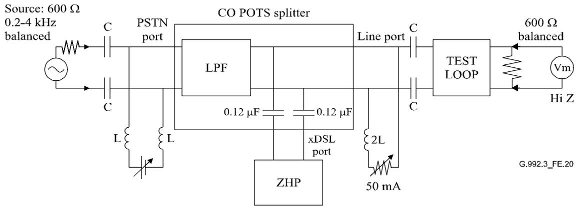
NOTE – The test loop is specified in Figure E.22.
