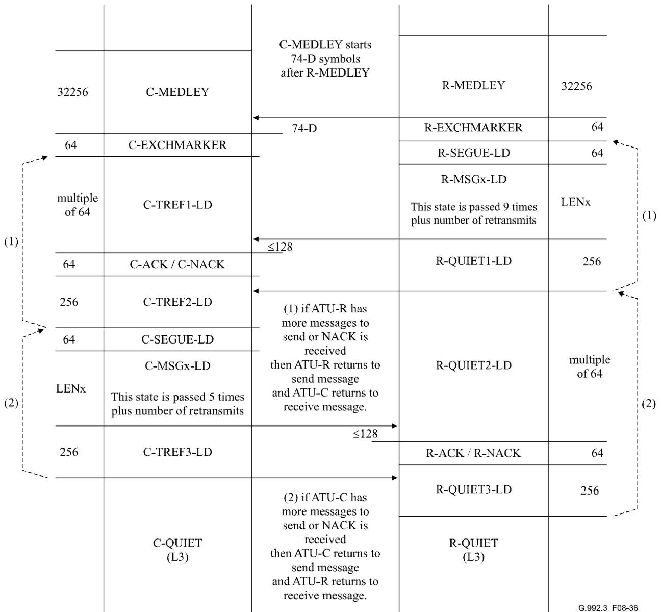
**Figure 8-36/G.992.3 – Loop diagnostics timing diagram (part 2)**
