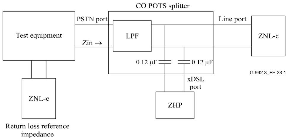
$$\text{ReturnLoss} = -20 \text{ Log} \left| \frac{\text{ZNL-c} - \text{Zin}}{\text{Zin} + \text{ZNL-c}} \right| \text{ dB}$$
