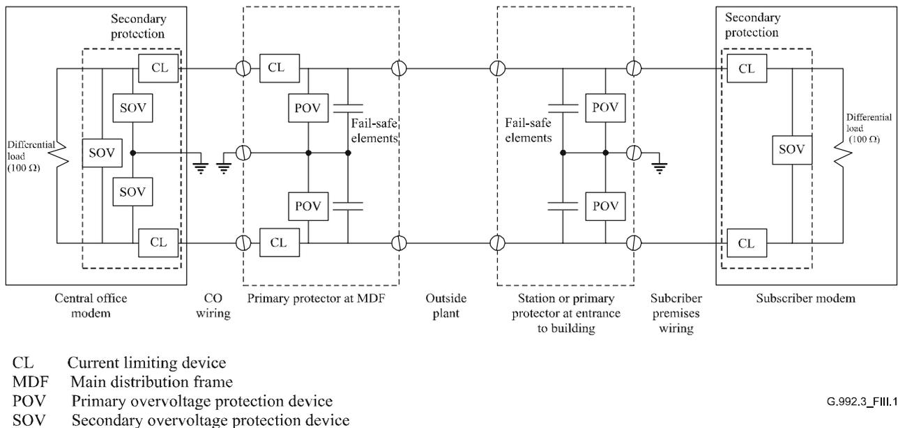
**Figure III.1/G.992.3 – Typical arrangement of protection devices**
