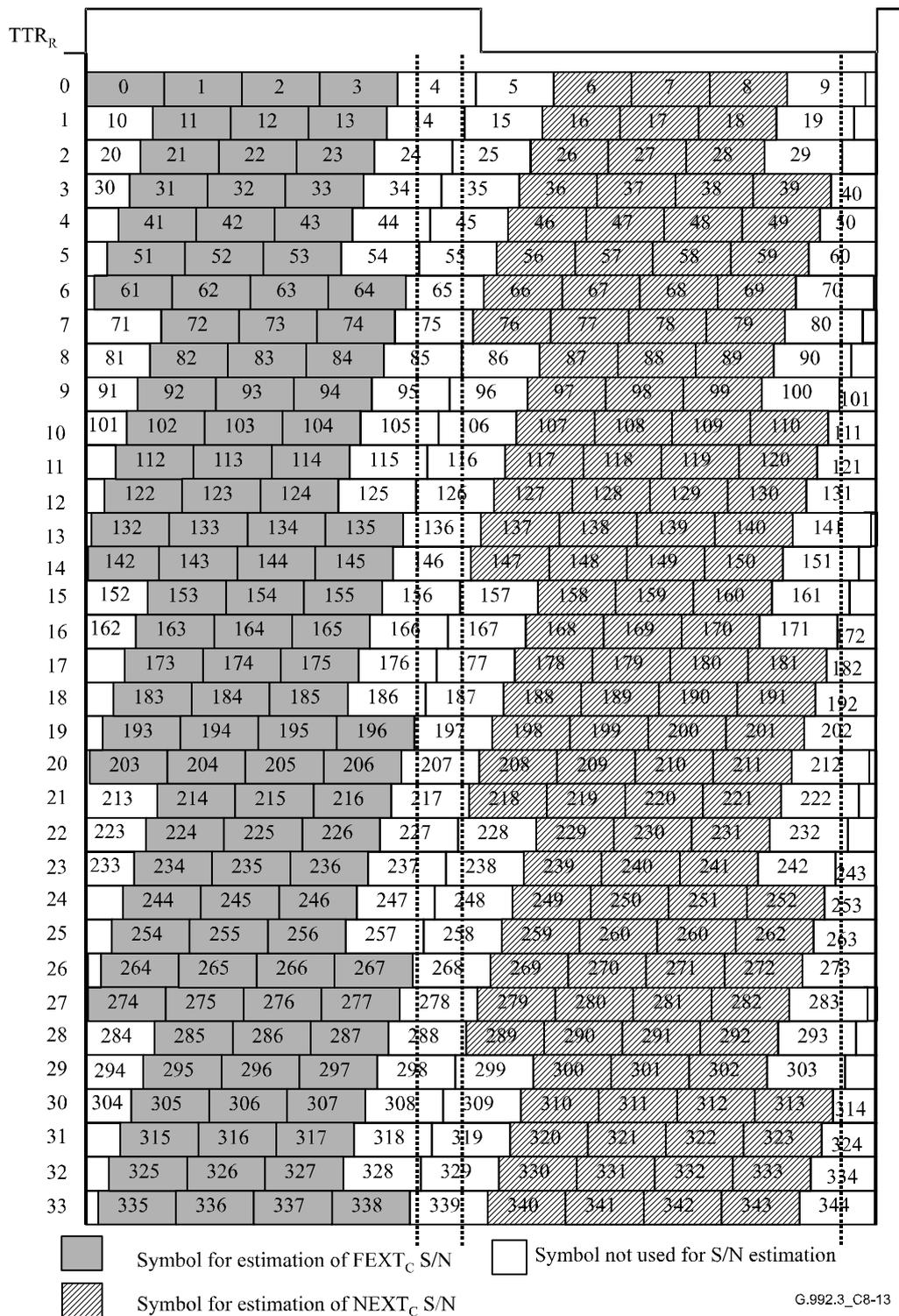
**Figure C.8-13/G.992.3 – Symbol pattern in a hyperframe for S/N estimation – Upstream**
