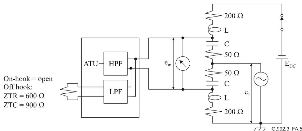
**Figure A.5/G.992.3 – Longitudinal balance above 30 kHz measurement method (HPF and LPF integrated)**
