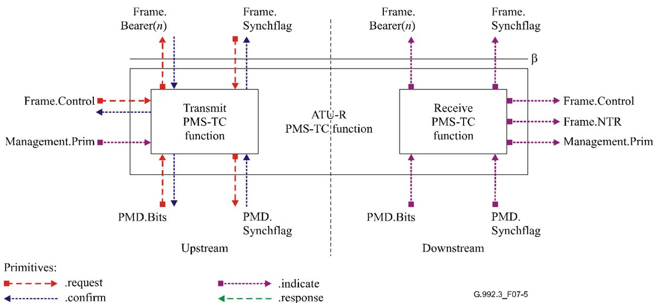
**Figure 7-5/G.992.3 – Signals of the ATU-R PMS-TC function**
