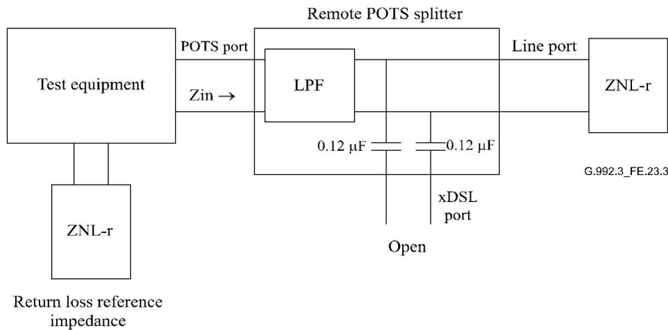
$$\text{ReturnLoss} = -20 \text{ Log} \left| \frac{Z_{\text{NL-r}} - Z_{\text{in}}}{Z_{\text{in}} + Z_{\text{NL-r}}} \right| \text{ dB}$$
