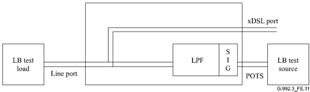
**Figure E.11/G.992.3 – Longitudinal balance remote test setup**
