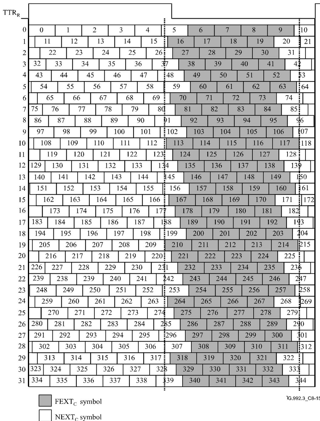
**Figure C.8-15/G.992.3 – Symbol pattern in a hyperframe without cyclic prefix – Upstream**
