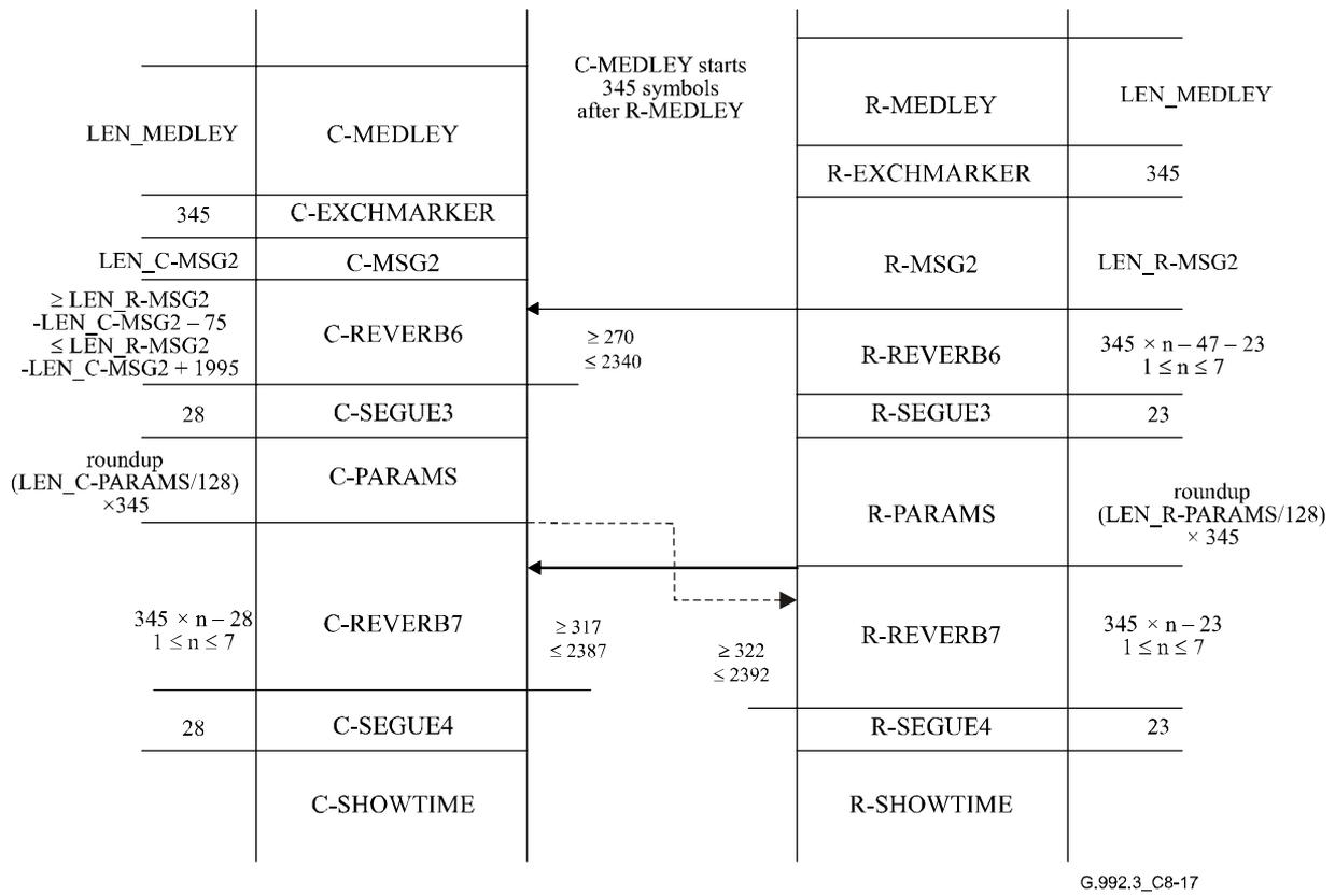
**Figure C.8-17/G.992.3 – Timing diagram of the initialization procedure (part 2) with C-PARAMS and with R-PARAMS states**
