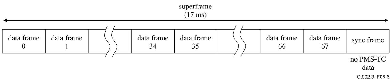
**Figure 8-6/G.992.3 – ADSL superframe structure – ATU-C transmitter**
