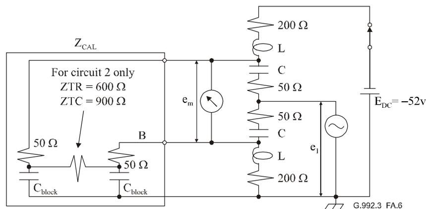
**Figure A.6/G.992.3 – Calibration circuit**
