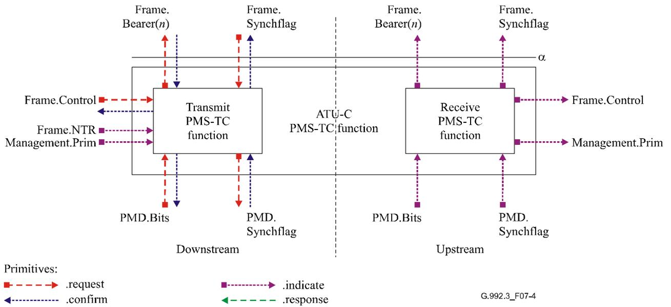
**Figure 7-4/G.992.3 – Signals of the ATU-C PMS-TC function**
