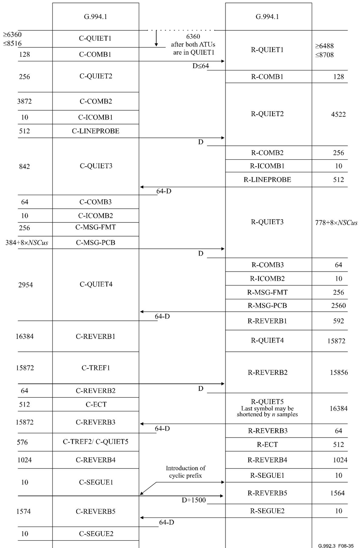
Figure 8-35/G.992.3 – Loop diagnostics timing diagram (part 1)
