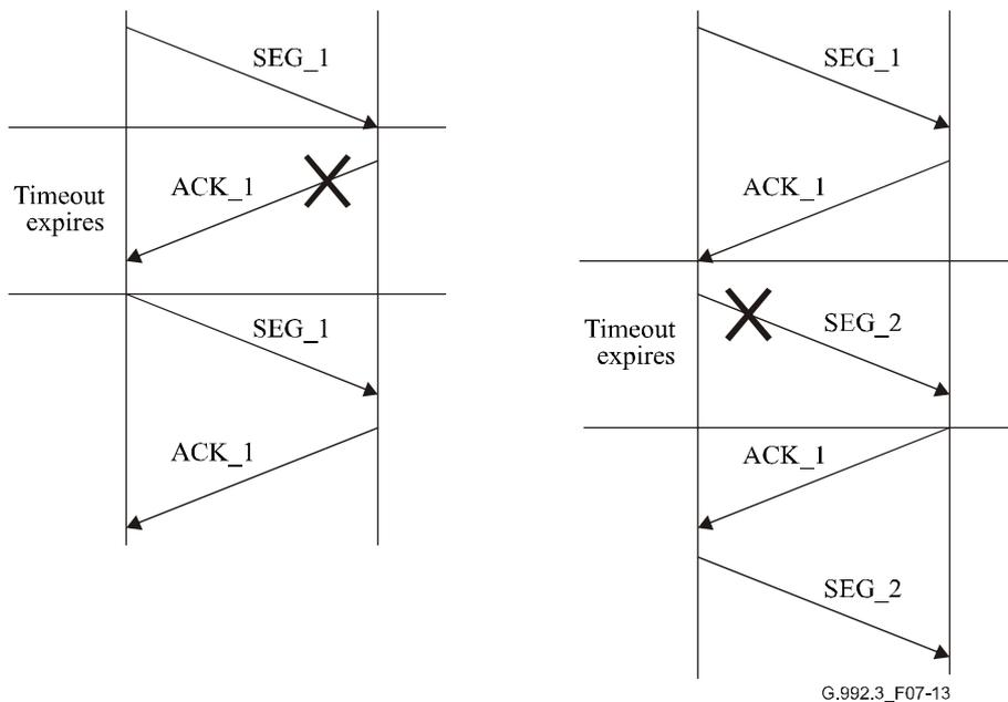
**Figure 7-13/G.992.3 – Example of retransmission of segment and acknowledgment**
