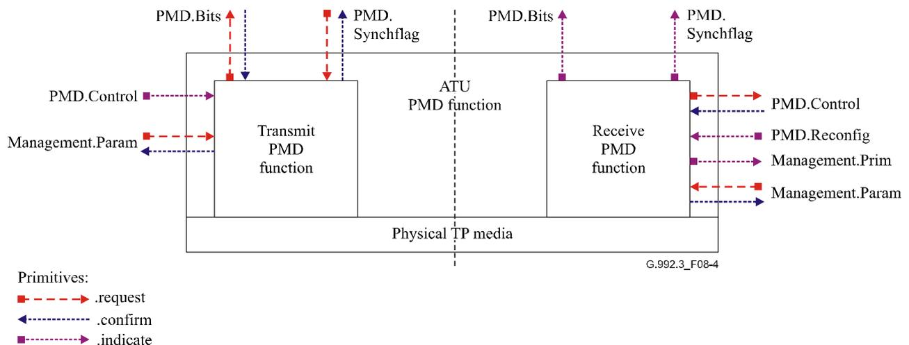
**Figure 8-4/G.992.3 – Signals of the ATU PMD function**
