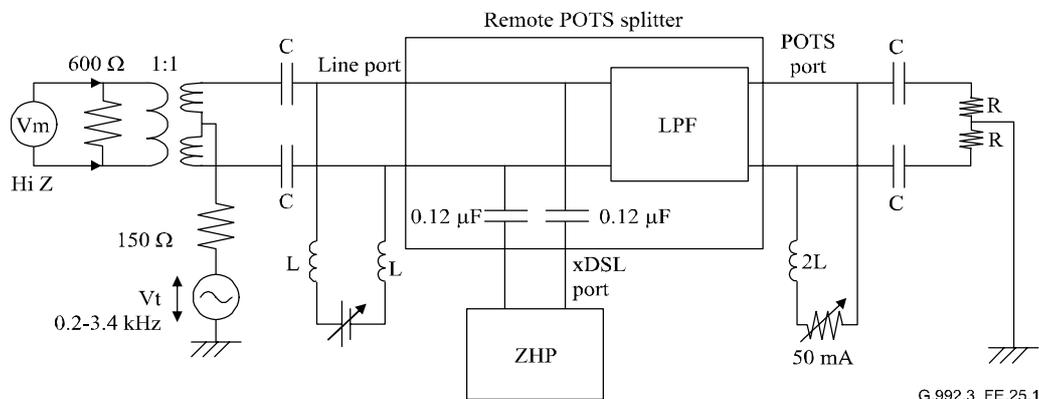
$$\text{Longitudinal Balance} = -20 \text{ Log } (V_m / V_t) \text{ dB}$$
