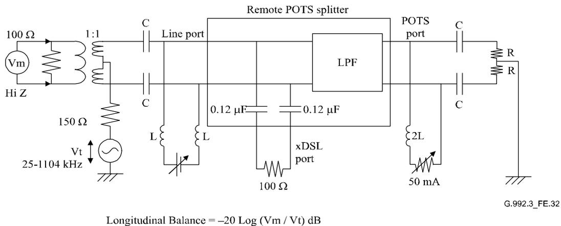
**Figure E.32/G.992.3 – Longitudinal balance remote test setup in the ADSL band**
