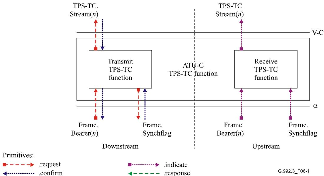
**Figure 6-1/G.992.3 – Signals of an ATU-C TPS-TC function**
