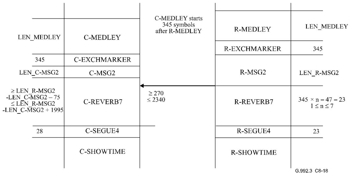
**Figure C.8-18/G.992.3 – Timing diagram of the initialization procedure (part 2) without C-PARAMS and without R-PARAMS states**
