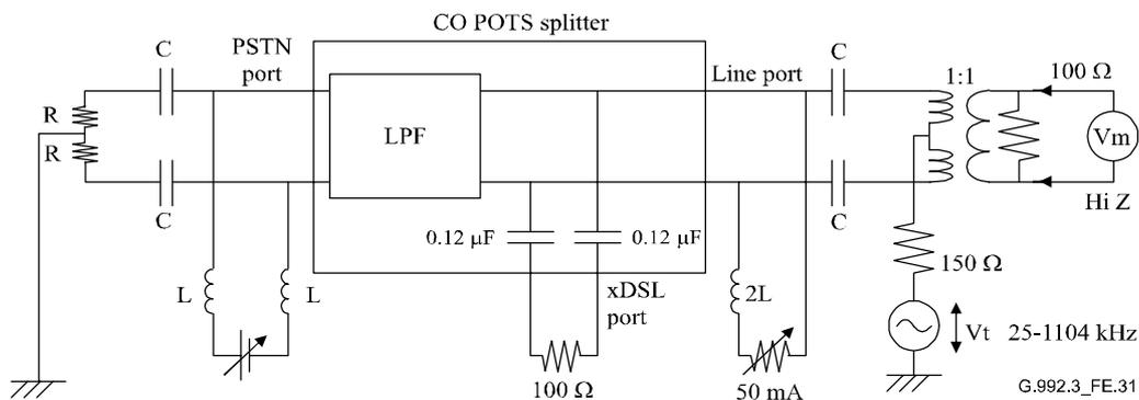
$$\text{Longitudinal Balance} = -20 \text{ Log} (V_m / V_t) \text{ dB}$$
