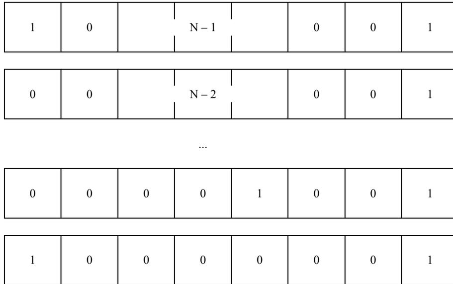
**Figure 7-11/G.992.3 – Example showing the control field in a segmented message of length  $N$**
