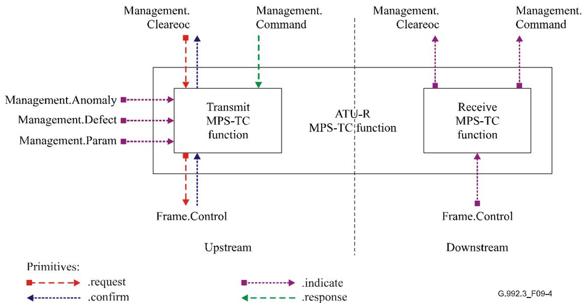
**Figure 9-4/G.992.3 – Signals of the ATU-R MPS-TC function**
