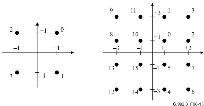
**Figure 8-13/G.992.3 – Constellation labels for  $b = 2$  and  $b = 4$**
