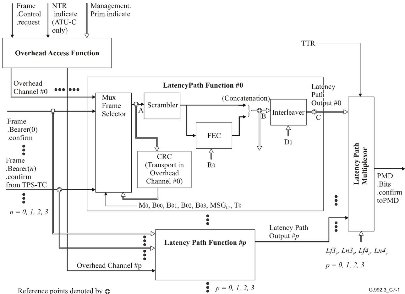
Figure C.7-1/G.992.3 – Block diagram of transmit PMS-TC function
