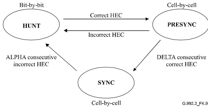
**Figure K.9/G.992.3 – Cell delineation procedure state machine**
