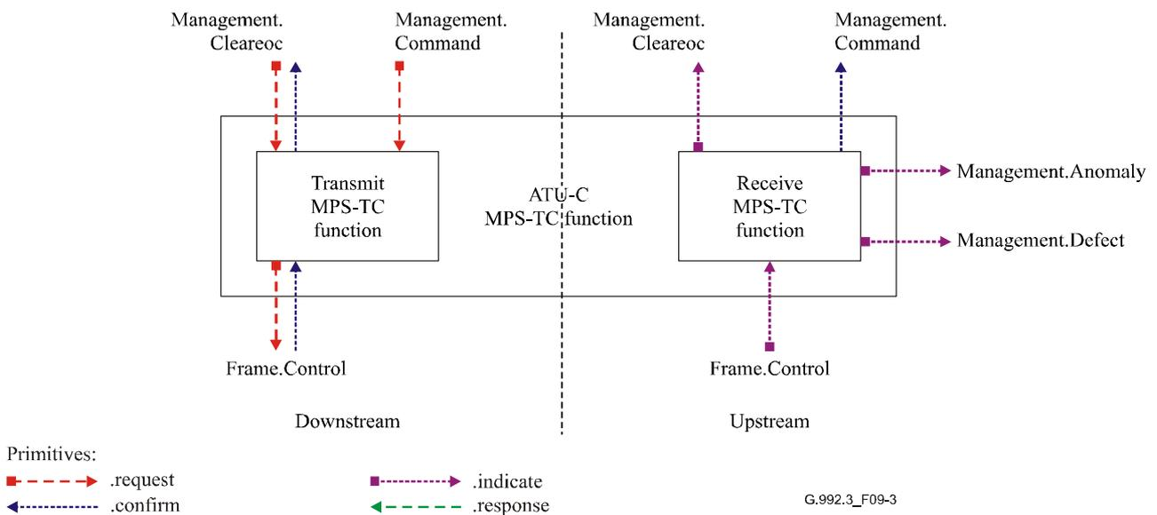
**Figure 9-3/G.992.3 – Signals of the ATU-C MPS-TC function**
