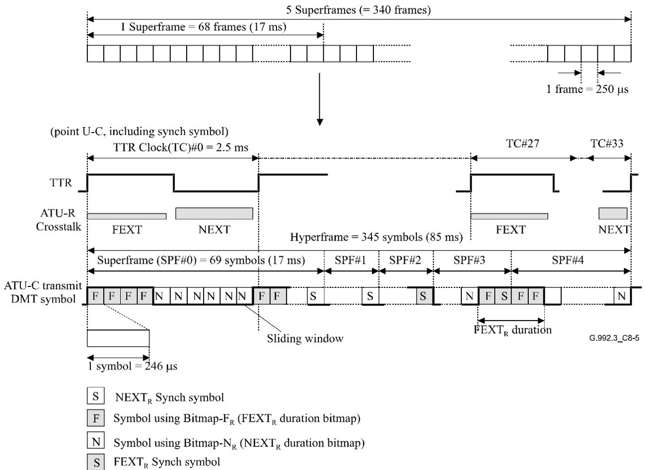
Figure C.8-5/G.992.3 – Hyperframe structure for downstream
