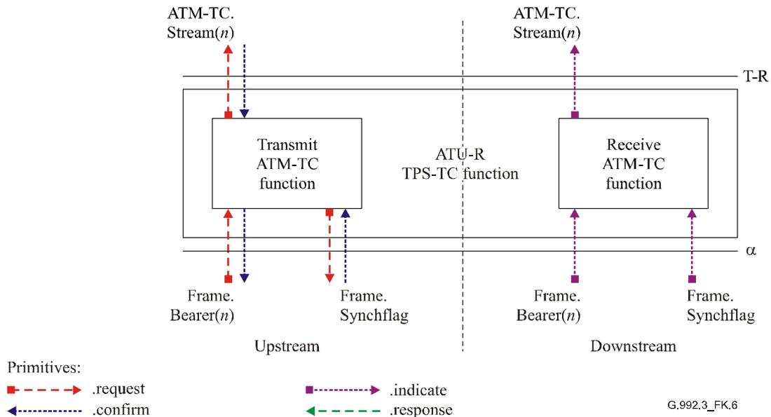
**Figure K.6/G.992.3 – Signals of the ATU-R ATM-TC function**
