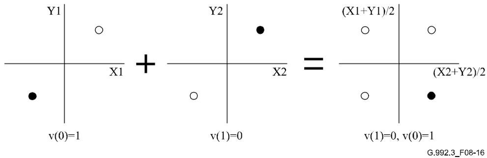
**Figure 8-16/G.992.3 – Combination of a pair of 1-bit constellations to build a 2-bit constellation**
