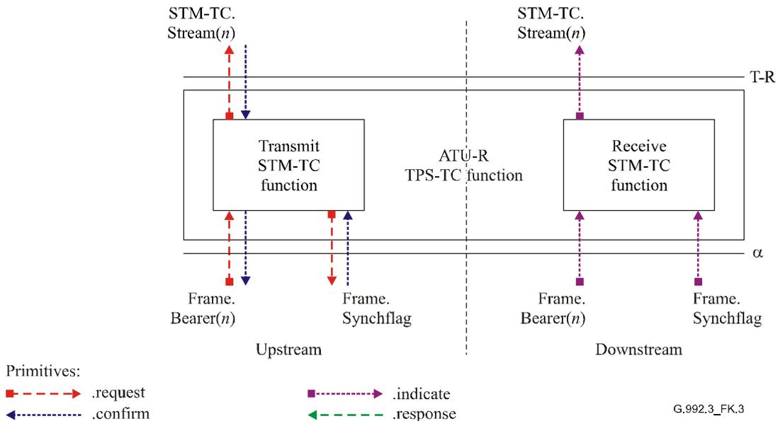
**Figure K.3/G.992.3 – Signals of the ATU-R STM-TC function**
