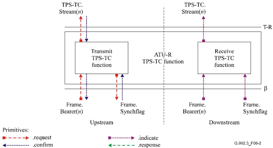
**Figure 6-2/G.992.3 – Signals of an ATU-R TPS-TC function**
