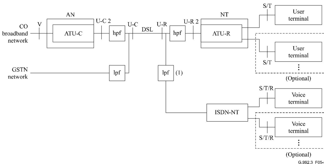
Figure 5-8/G.992.3 – Data with ISDN service application model
