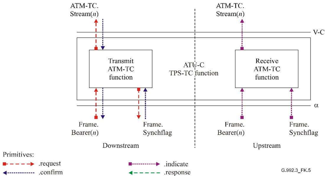
**Figure K.5/G.992.3 – Signals of the ATU-C ATM-TC function**
