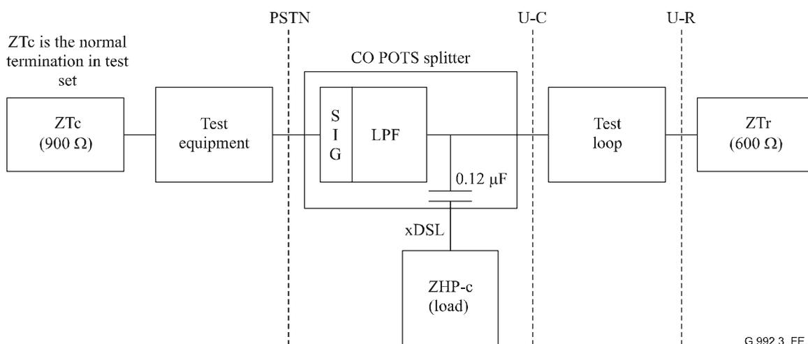
ZHP-c = the impedance presented to the POTS connection by an ATU-C through the capacitance of the POTS splitter DC blocking capacitors
