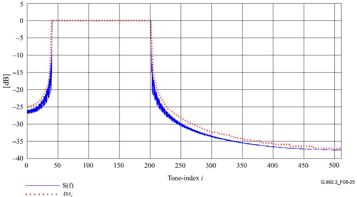
**Figure 8-25/G.992.3 – Example of the downstream  $\log_{tss_i}$  values (in dB) as a function of the subcarrier index**
