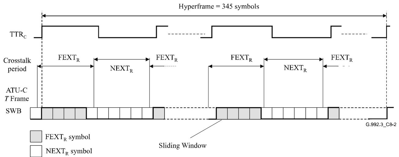
**Figure C.8-2/G.992.3 – Sliding window for downstream symbols**
