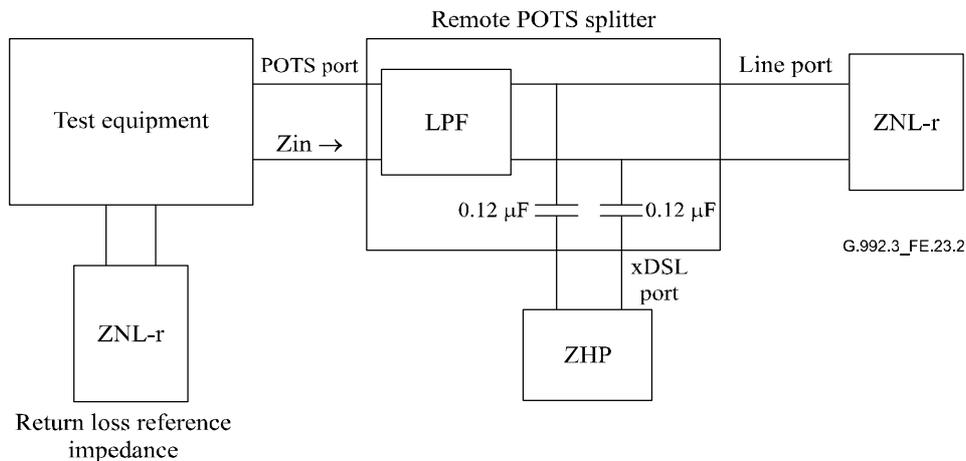
$$\text{ReturnLoss} = -20 \text{ Log} \left| \frac{\text{ZNL-r} - \text{Zin}}{\text{Zin} + \text{ZNL-r}} \right| \text{ dB}$$
