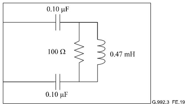
NOTE – Component Tolerances: Capacitors: 2.5%, Resistors: 1%, Coils: 5%.
