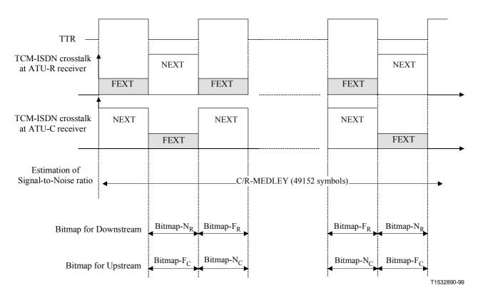
Figure C8-11/G.992.3 – Estimation of periodic Signal-to-Noise Ratio
