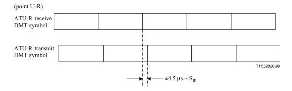
Figure C8-3/G.992.3 - Loop timing for ATU-R
