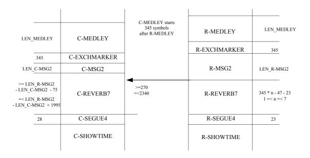
Figure C8-18/G.992.3 – Timing Diagram of the Initialization Procedure (part 2) without C-PARAMS and without R-PARAMS states
