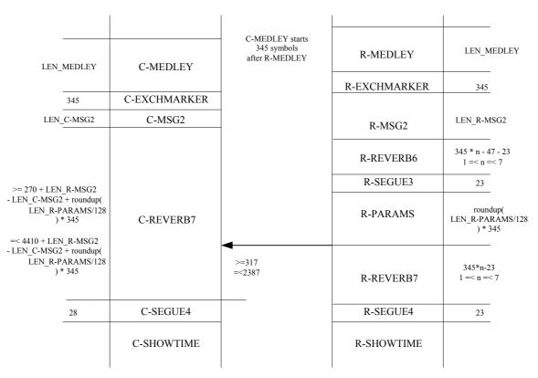
Figure C8-20/G.992.3 – Timing Diagram of the Initialization Procedure (part 2) without C-PARAMS and with R-PARAMS states
