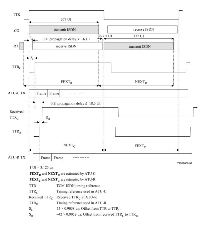
Figure C8-1/G.992.3 – Timing chart of the TCM-ISDN crosstalk
