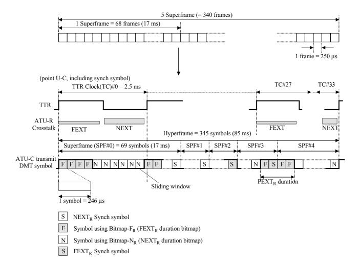
Figure C8-5/G.992.3 – Hyperframe structure for downstream
