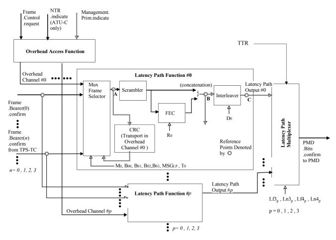
Figure C7-1/G.992.3 – Block Diagram of Transmit PMS-TC Function
