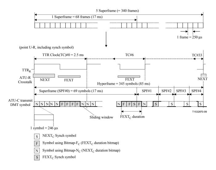
Figure C8-7/G.992.3 – Hyperframe structure for upstream
