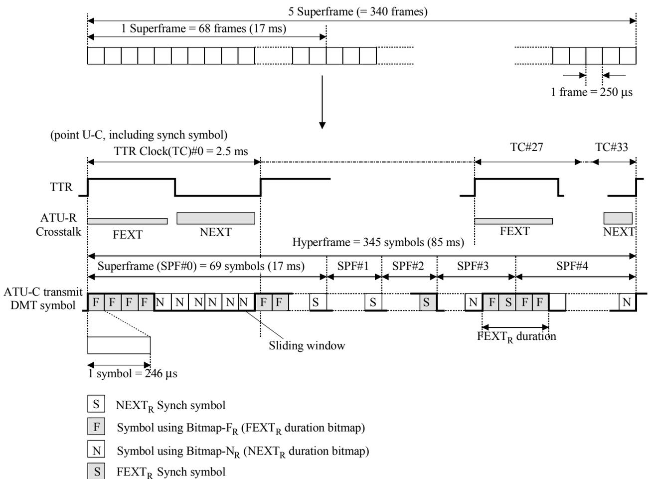
Figure C8-5/G.992.3 – Hyperframe structure for downstream
