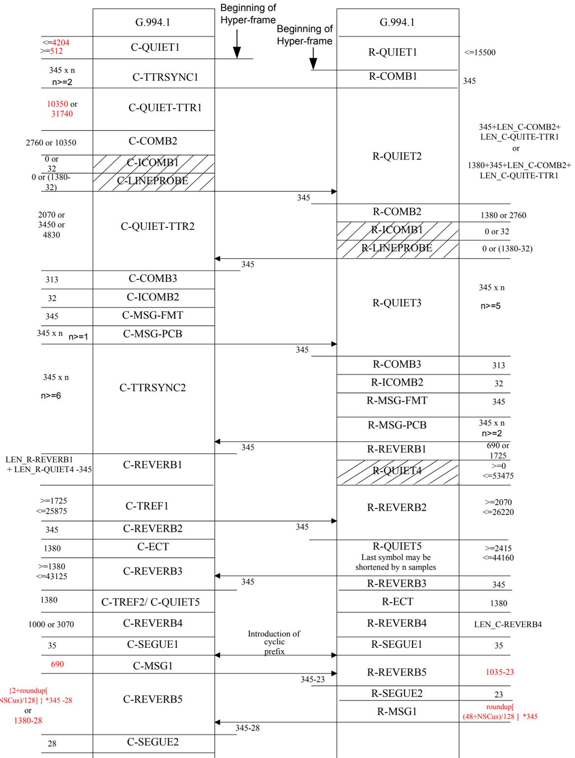
Figure C8-16/G.992.3 – Timing Diagram of the Initialization Procedure
