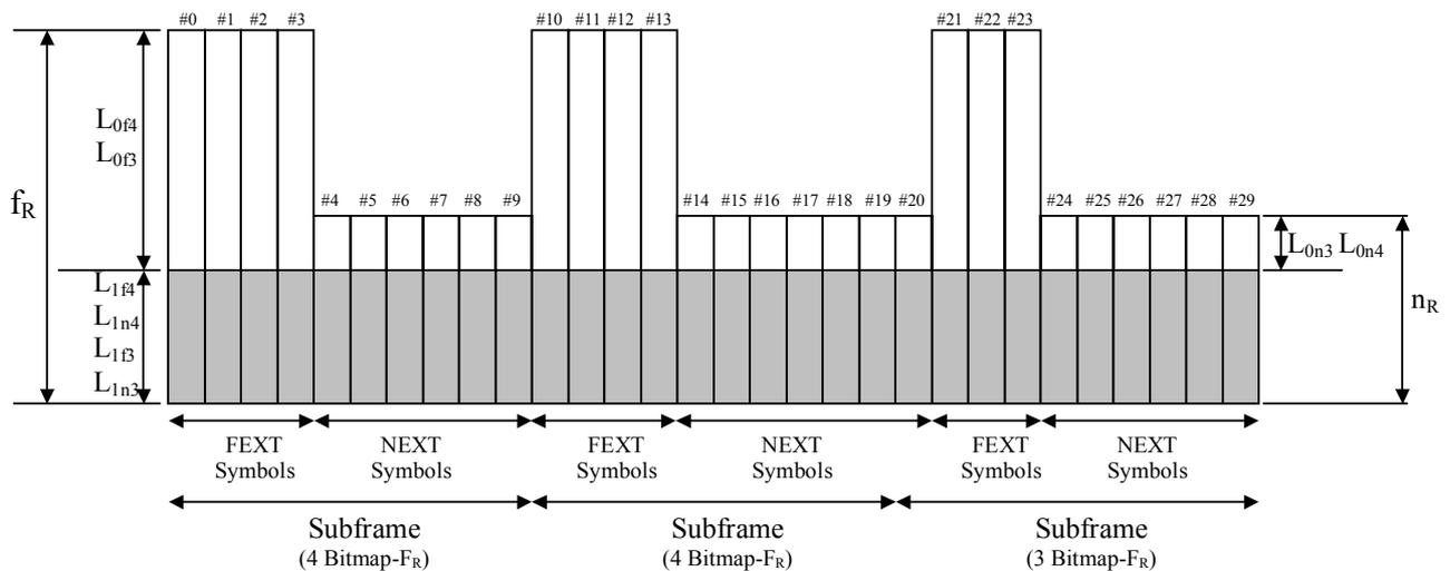
Figure C8-9/G.992.3 – First example of data rate to symbol type mapping.
