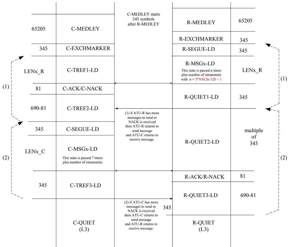
Figure C8-22/G.992.3 – Loop Diagnostics Timing Diagram (part 2)
