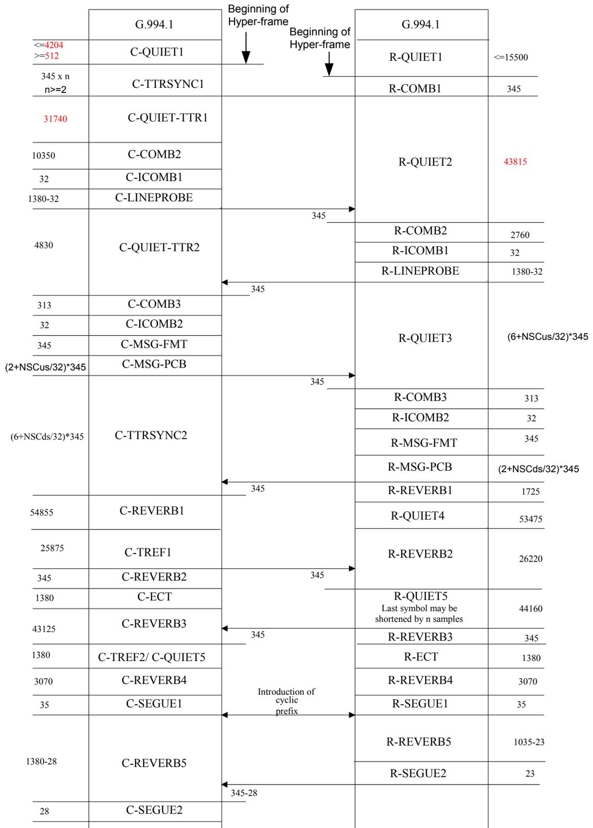
Figure C8-21/G.992.3 – Loop Diagnostics Timing Diagram (part 1)
