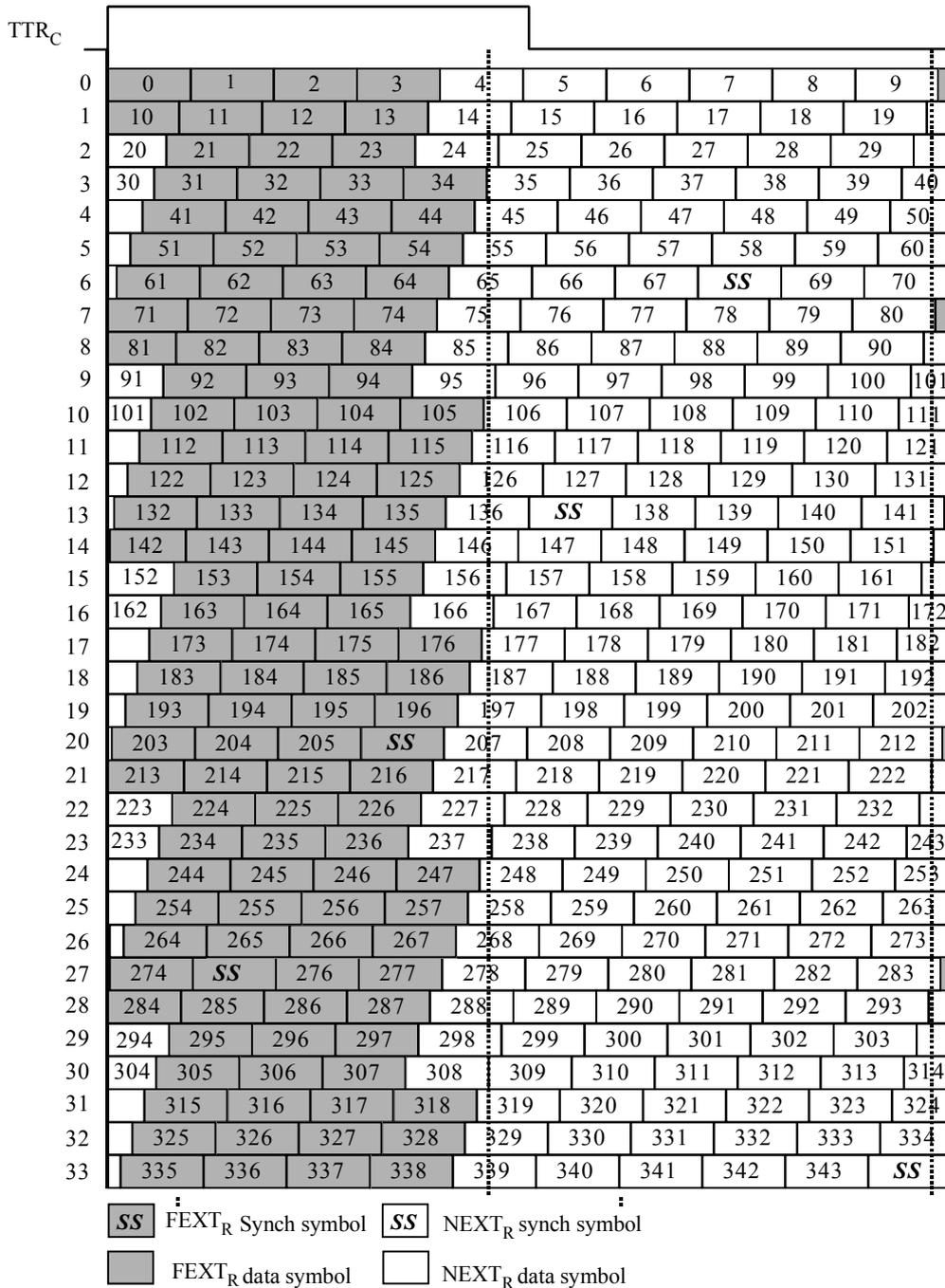
**Figure C8-6/G.992.3 – Symbol pattern in a hyperframe with cyclic prefix – Downstream**
