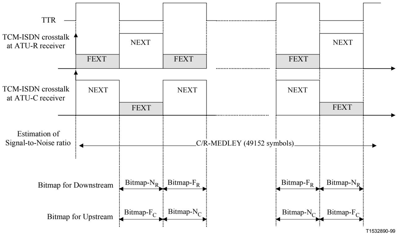
**Figure C8-11/G.992.3 – Estimation of periodic Signal-to-Noise Ratio**
