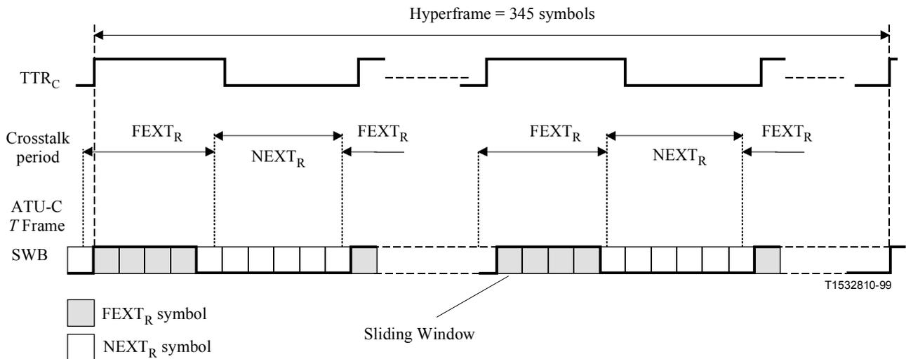
**Figure C8-2/G.992.3 – Sliding window for downstream symbols**
