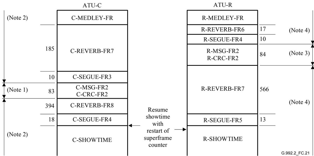
**Figure C.21/G.992.2 – Timing diagram of the Fast Retrain procedure, ATU-C initiated from SHOWTIME (part 2)**
