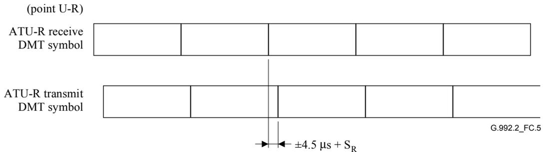
**Figure C.5/G.992.2 – Loop timing for ATU-R**
