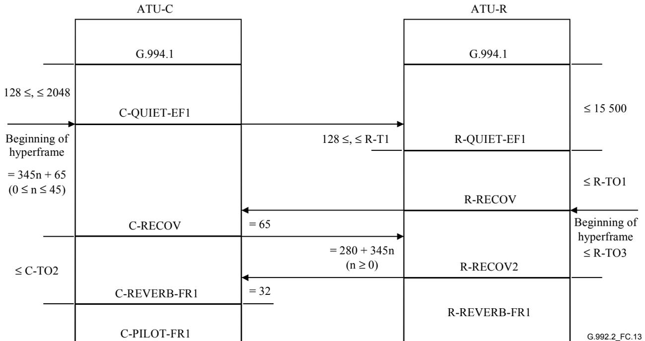
Figure C.13/G.992.2 – Timing diagram of Escape to Fast Retrain
