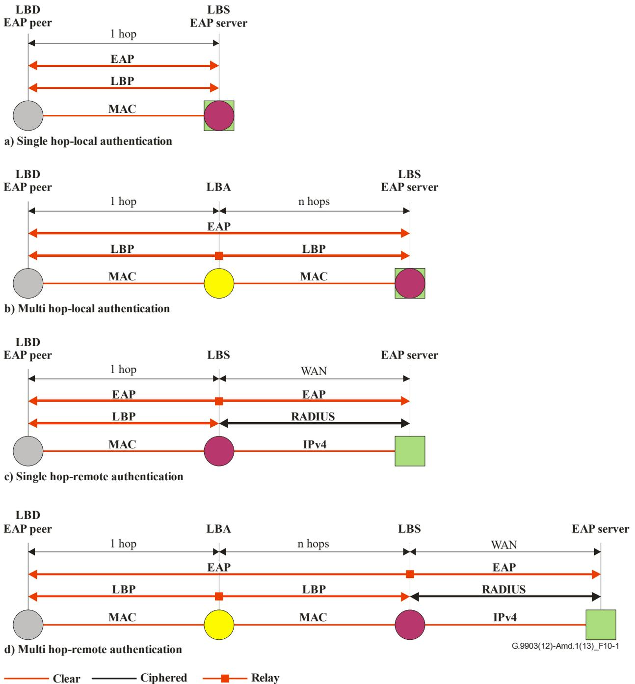
**Figure 10-1 – LBP and EAP relaying capabilities**
