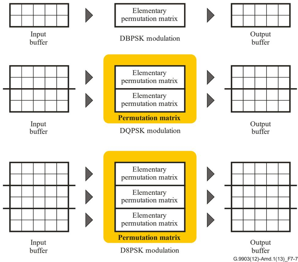
**Figure 7-7 – Permutation matrix used with different modulations**
