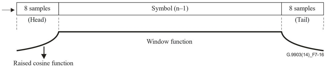
**Figure 7-16 – Windowing using a raised cosine for the shaping function**
