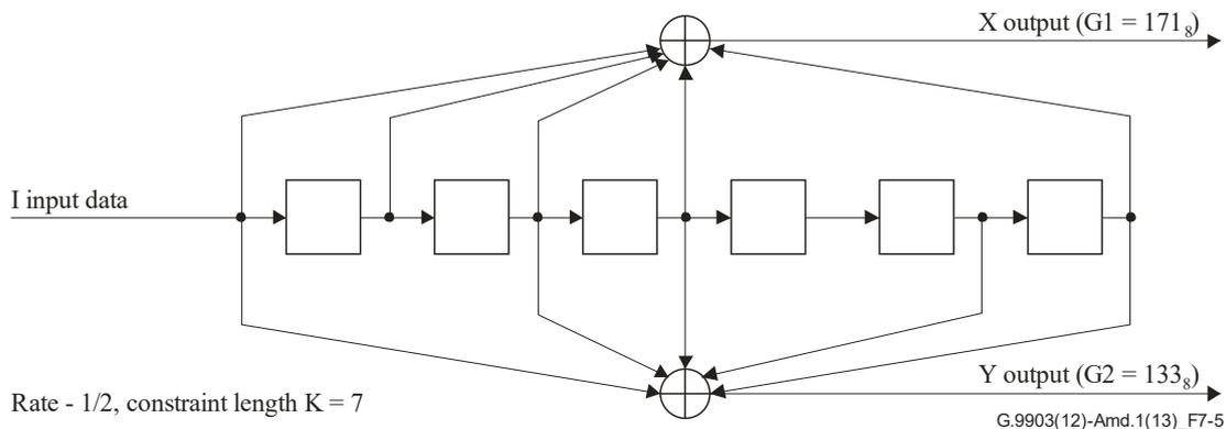
**Figure 7-5 – Convolutional encoder**
