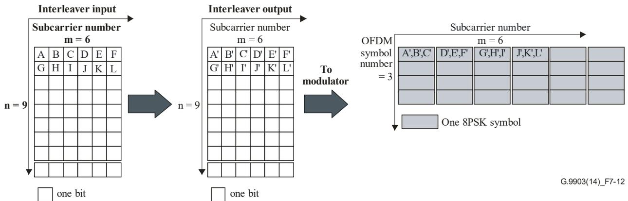
Figure 7-12 – Interleaving process for 8-PSK/D8PSK case
