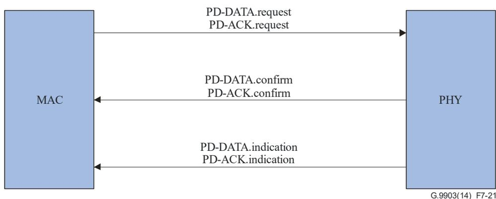
Figure 7-21 – Data or ACK primitive flow
