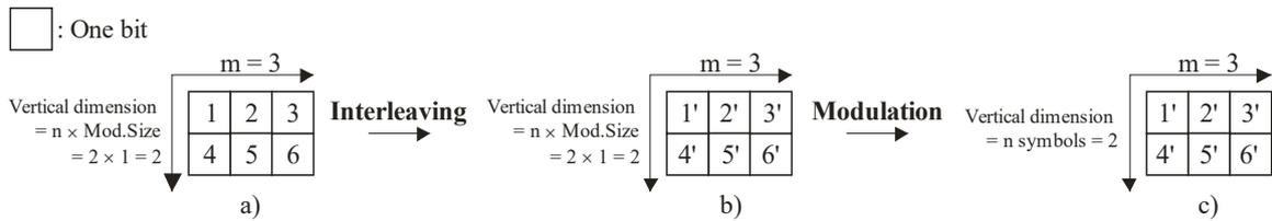
**Figure 7-9 – Example of interleaving with DBPSK**
