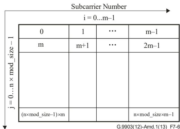
**Figure 7-6 – Bit order input into the input buffer**
