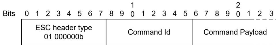
**Figure 9-12 – Command frame header format**
