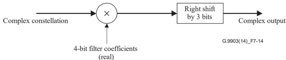
**Figure 7-14 – Block diagram of the pre-emphasis filter**
