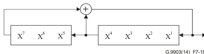
**Figure 7-18 – PN sequence generator using linear feedback shift register (LFSR)**
