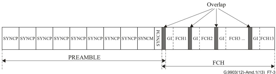
Figure 7-3 – ACK/NACK frame structure
