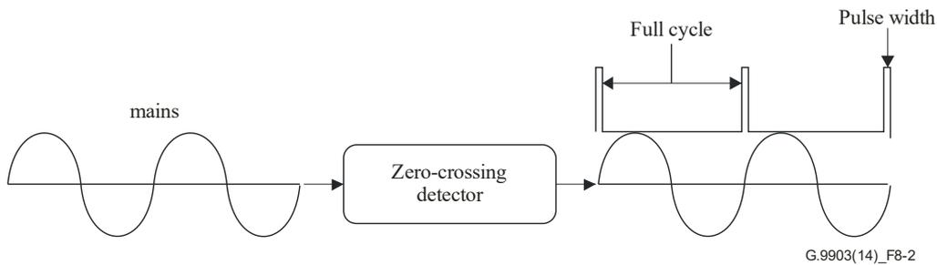
**Figure 8-2 – Zero-crossing detector**
