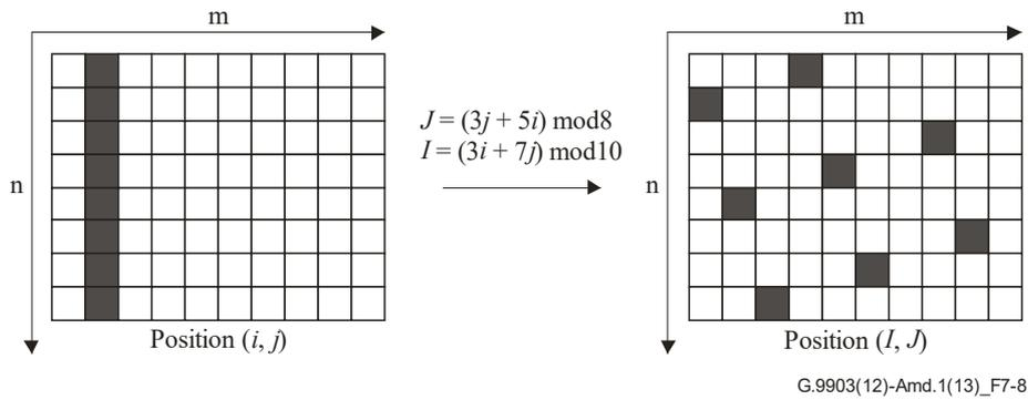
**Figure 7-8 – Example of spreading behaviour**
