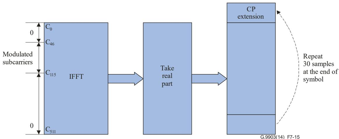
**Figure 7-15 – IFFT input/output and CP addition**
