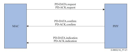
Figure 7-21 – Data or ACK primitive flow
