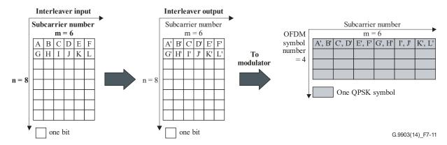
Figure 7-11 – Interleaving process for QPSK/DQPSK case
