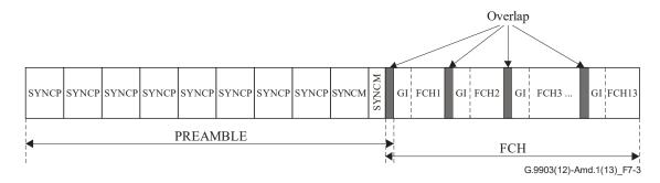
Figure 7-3 – ACK/NACK frame structure
