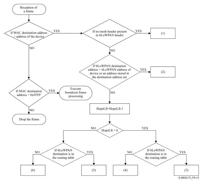
Figure 9-13 – Unicast packet routing processing
