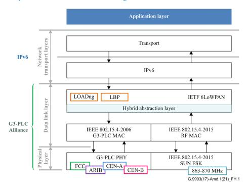
Figure H.1 – G3-PLC Hybrid PLC & RF protocol stack
