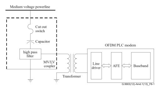
Figure 8-1 – Proposed coupling circuit
