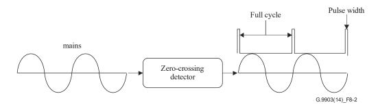
Figure 8-2 – Zero-crossing detector
