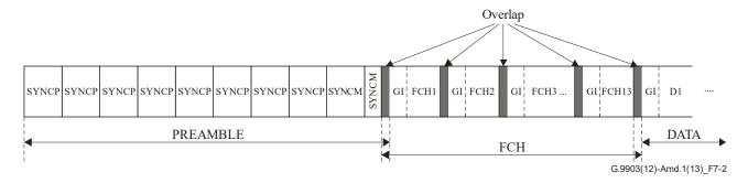
Figure 7-2 – Typical data frame structure
