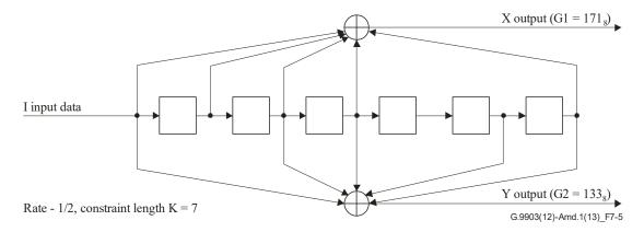
Figure 7-5 – Convolutional encoder
