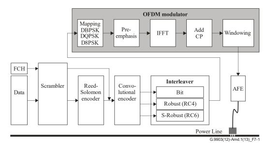
Figure 7-1 – Block diagram of an OFDM transceiver
