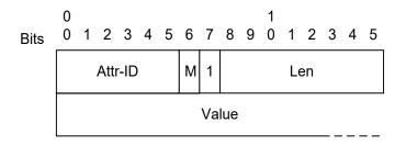
Figure 9-24 – Configuration parameter format
