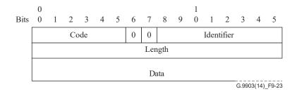
Figure 9-23 – Embedded EAP message format (generic)
