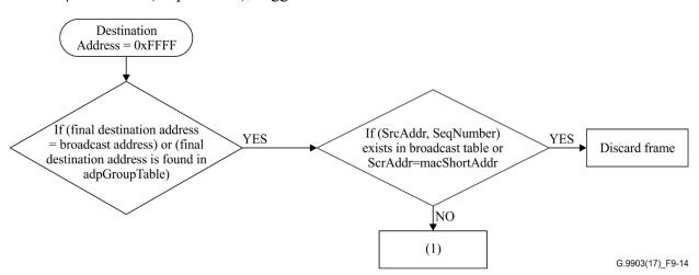
Figure 9-14 – Broadcast frame routing processing
