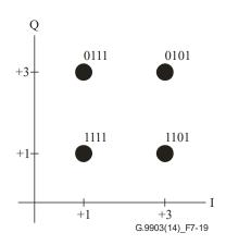
Figure 7-19 – 16-QAM constellation diagram
