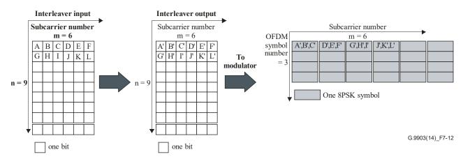
Figure 7-12 – Interleaving process for 8-PSK/D8PSK case
