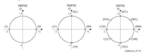
Figure 7-13 – Constellation encoding
