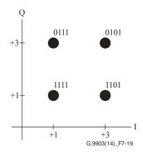
Figure 7-19 – 16-QAM constellation diagram
