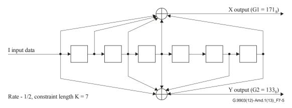
Figure 7-5 – Convolutional encoder
