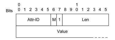
Figure 9-24 – Configuration parameter format
