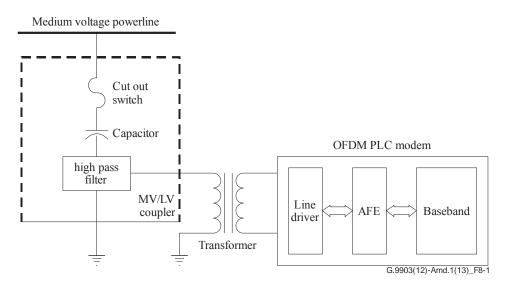
Figure 8-1 – Proposed coupling circuit
