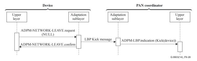
Figure 9-28 – Message sequence chart during the removal of a device by itself
