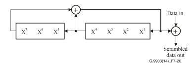
Figure 7-20 – LFSR used to generate the data bits that are used to modulate the pilot tones
