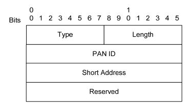
Figure E.7 – Target link-layer address option field
