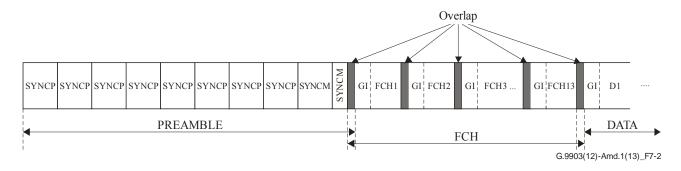
Figure 7-2 – Typical data frame structure
