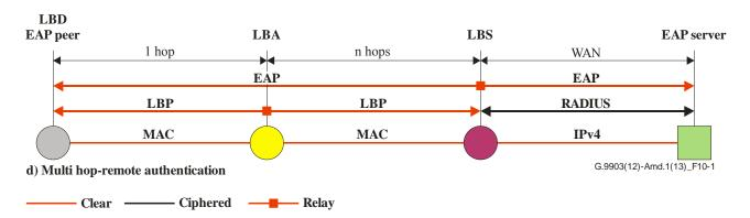
Figure 10-1 – LBP and EAP relaying capabilities
