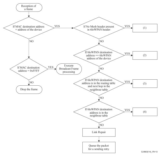
Figure 9-13 – Unicast packet routing processing
