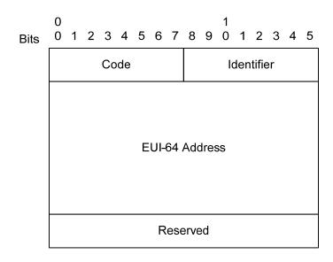
Figure E.6 – Source link-layer address option field
