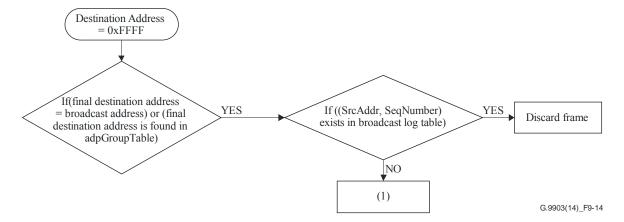
Figure 9-14 – Broadcast frame routing processing
