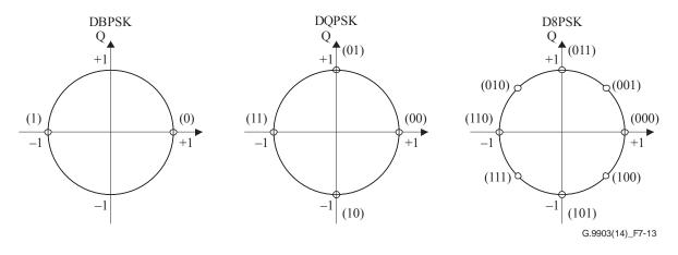
Figure 7-13 – Constellation encoding
