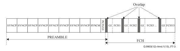
Figure 7-3 – ACK/NACK frame structure
