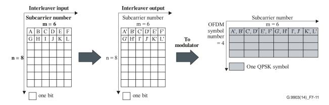
Figure 7-11 – Interleaving process for QPSK/DQPSK case
