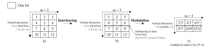
Figure 7-10 – Example of interleaving with DQPSK
