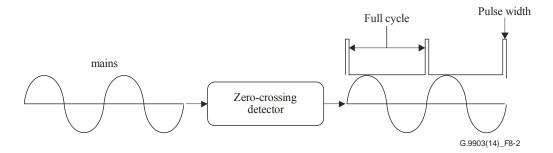
Figure 8-2 – Zero-crossing detector
