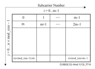
Figure 7-6 – Bit order input into the input buffer
