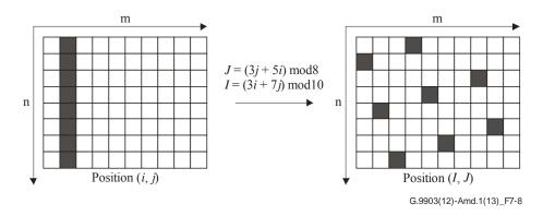
Figure 7-8 – Example of spreading behaviour
