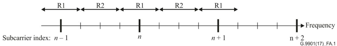
Figure A.1 – Frequency notching
