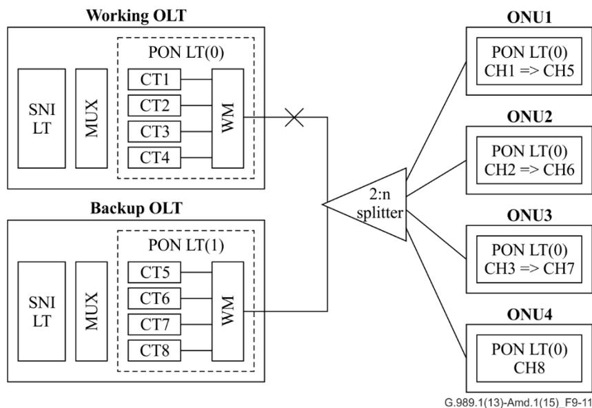
**Figure 9-11 – Type W protection – 2n:n model with dual parenting**
