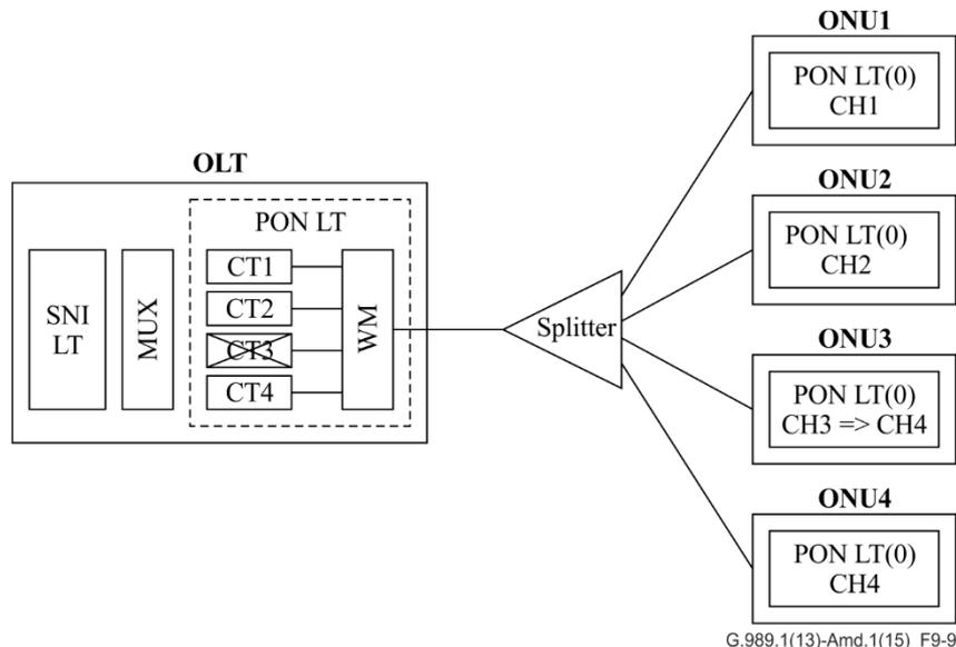
**Figure 9-9 – Type W protection – 1:n model with all active OLT CTs**
