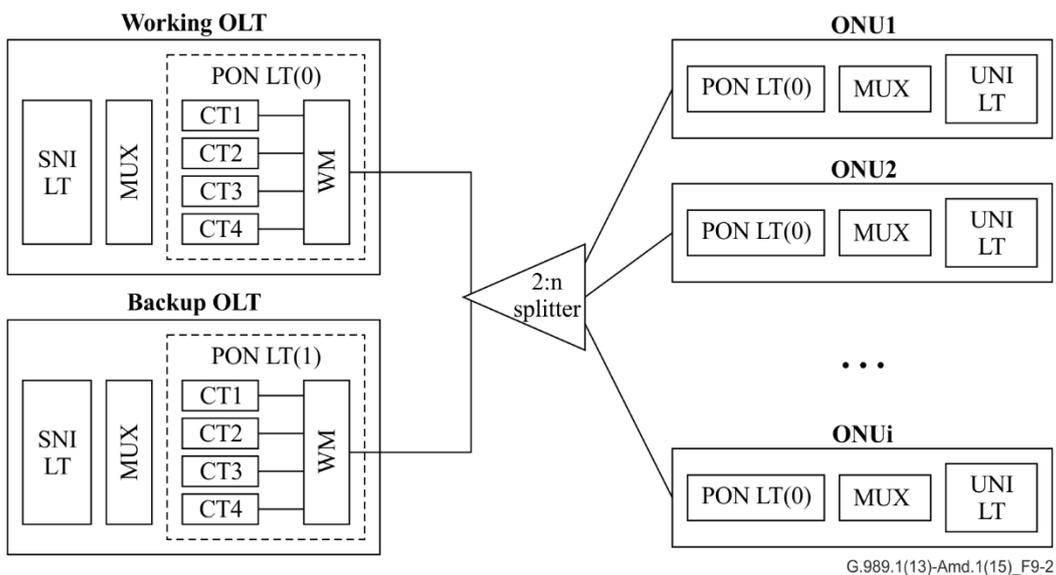
**Figure 9-2 – Type B protection – 1:1 model with dual homing**
