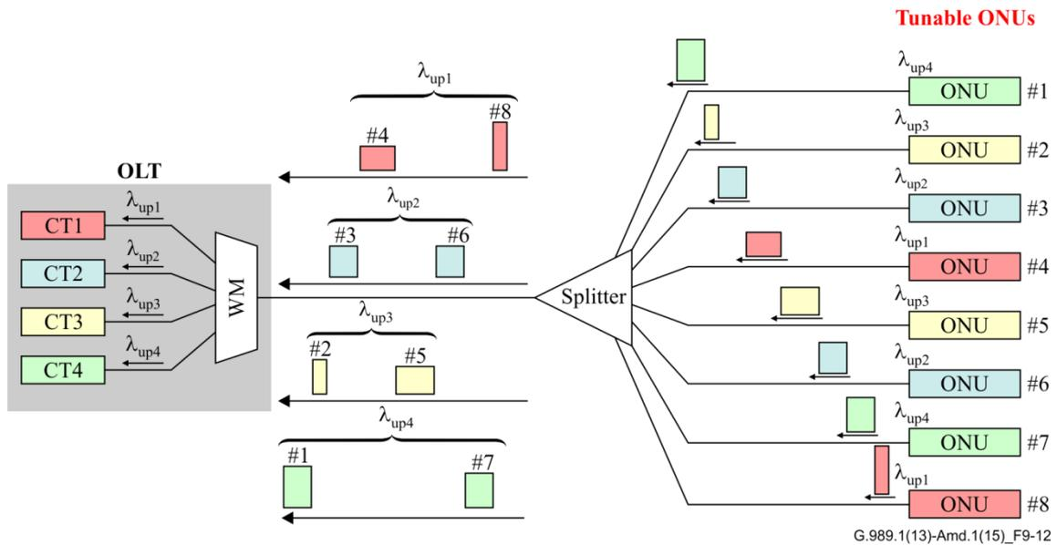
**Figure 9-12 – Example of OLT-port sleep mode (before starting sleep mode)**
