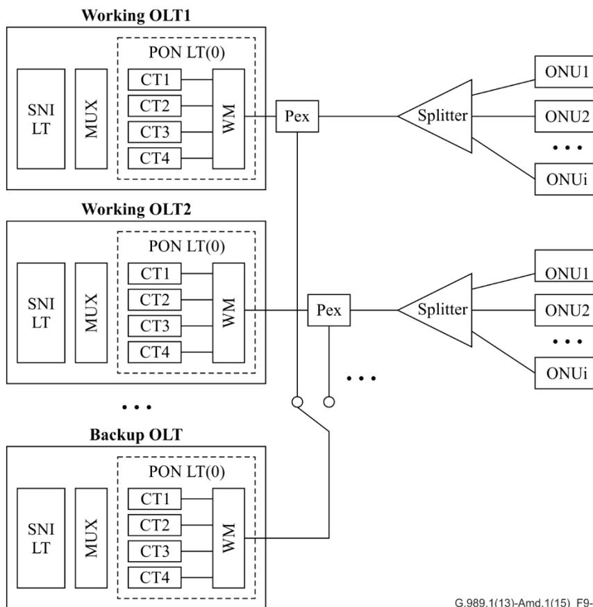
**Figure 9-5 – Type B protection – 1:n model with dual parenting**
