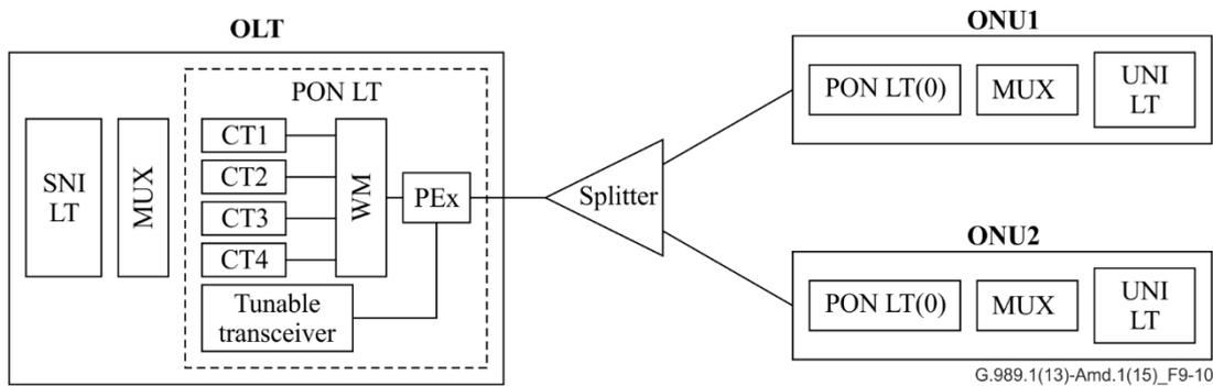
**Figure 9-10 – Type W protection – (n+1):n model**
