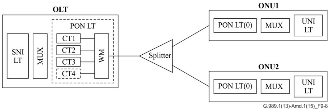
**Figure 9-8 – Type W protection - 1:n model with backup OLT CT**
