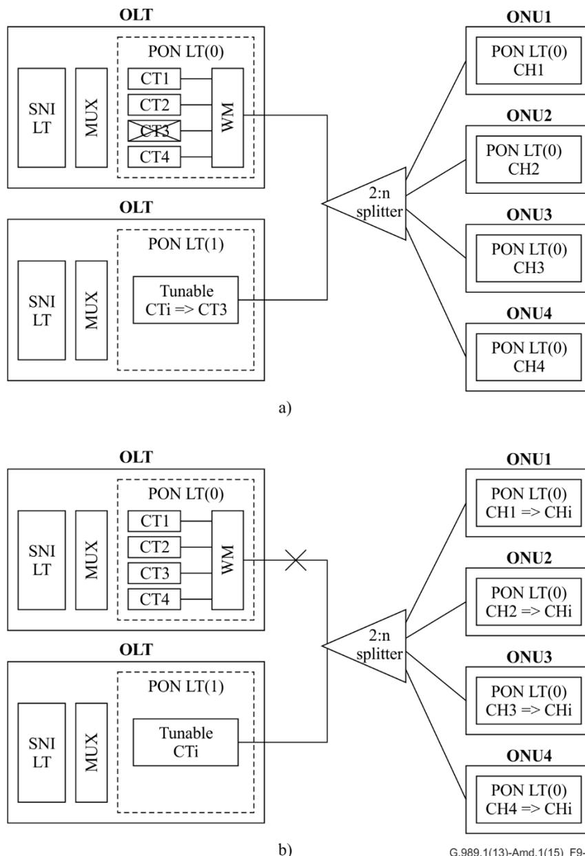
**Figure 9-4 – Type B protection – 1:n model (a) CT failure, (b) feeder fibre failure**
