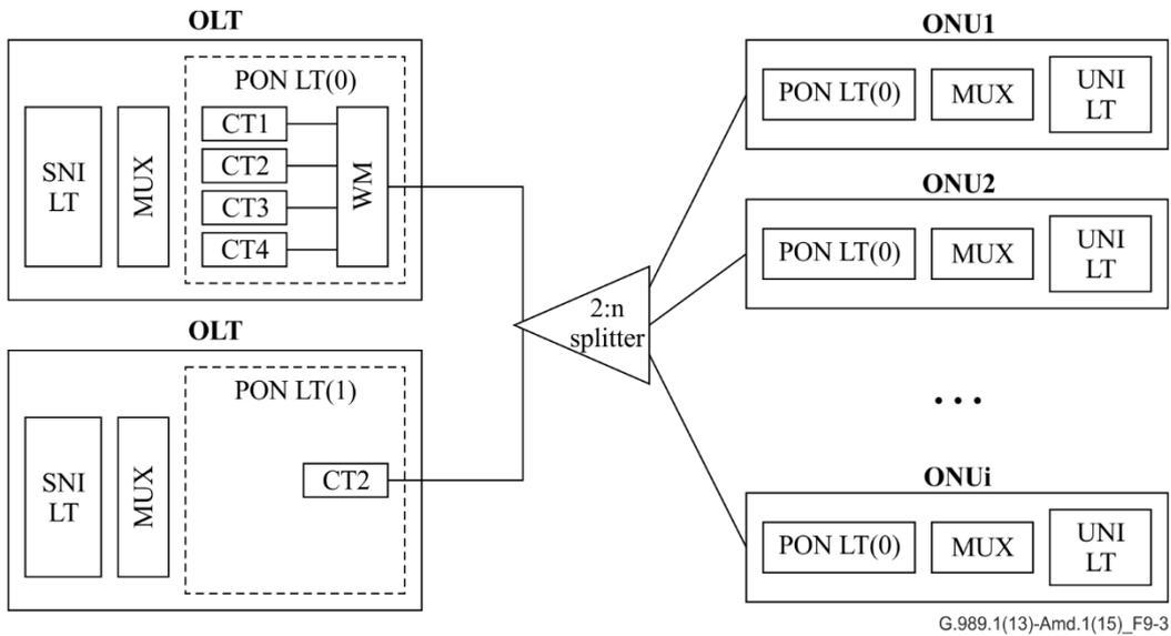
**Figure 9-3 – Type B protection – 1:1 model with single backup CT**
