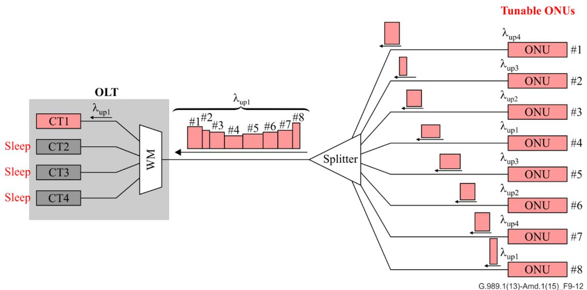
**Figure 9-13 – Example of the OLT-port sleep (CT 2, CT 3 and CT 4 are in the sleep mode)**
