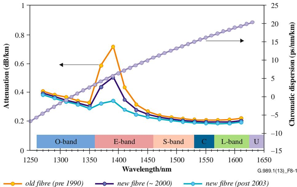
**Figure 8-1 – Single mode fibre attenuation and chromatic dispersion**
