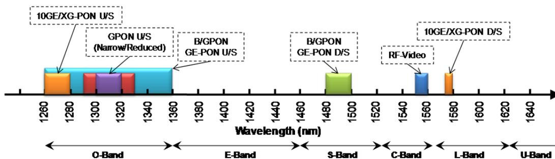
**Figure 8-2 – Wavelength plans of legacy PON systems**
