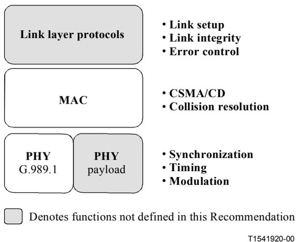
**Figure 2/G.989.1 – Functional view of reference model**
