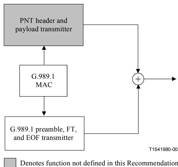
**Figure 9/G.989.1 – Basic structure of a G.989.1 transmitter**
