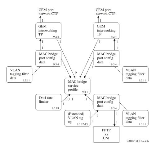
Figure 8.2.2-5 – Illustration of 1:P filtering
