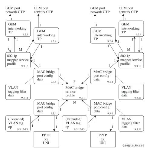
Figure 8.2.2-9 – Illustration of N:MP bridge-map-filtering
