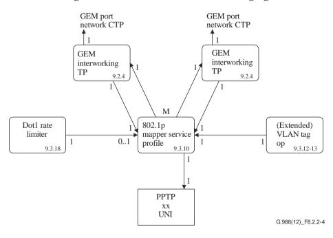
Figure 8.2.2-4 – Illustration of 1:M mapping
