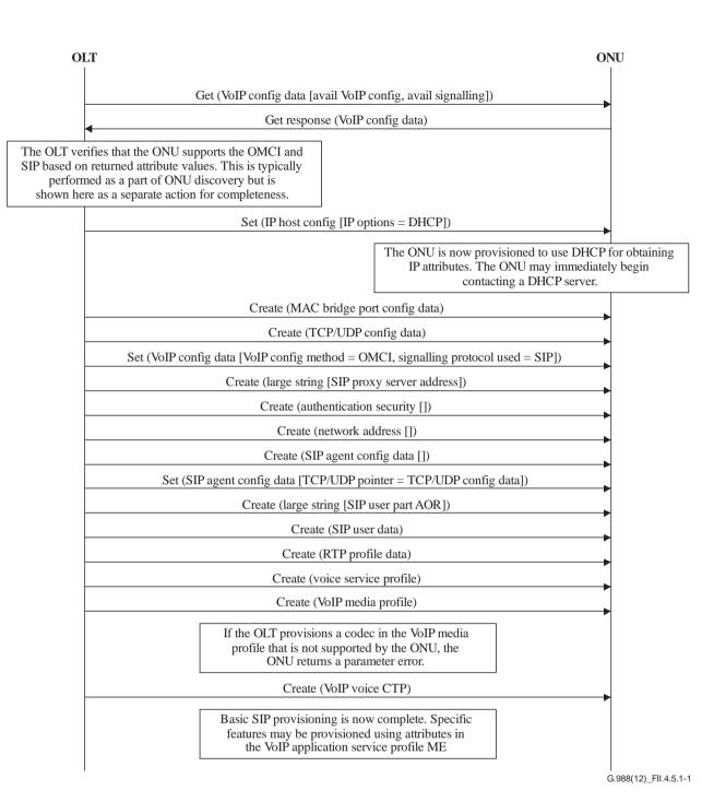
Figure II.4.5.1-1 – SIP provisioning flow
