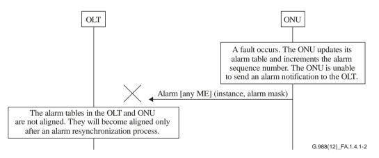
Figure A.1.4.1-2 – Alarm sequence number fails to stay in sync
