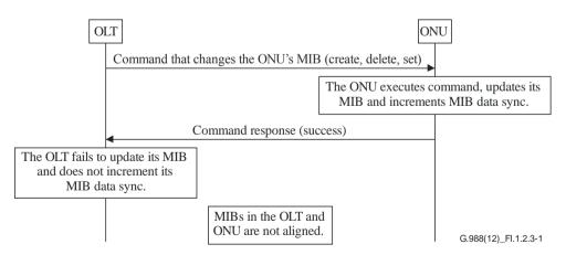
Figure I.1.2.3-1 – Mismatch of MIBs at the ONU and OLT under OLT command
