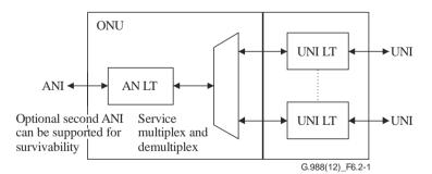
Figure 6.2-1 – ONU functional block diagram
