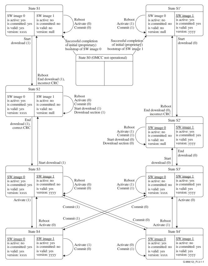
NOTE – In Figure I.3.1-1, states S1 and S2 (and S1' and S2') are distinguished only for convenience in understanding the flow. Upon receipt of a start download message, and particularly when the ONU re-boots, any partial downloads in progress are discarded.
