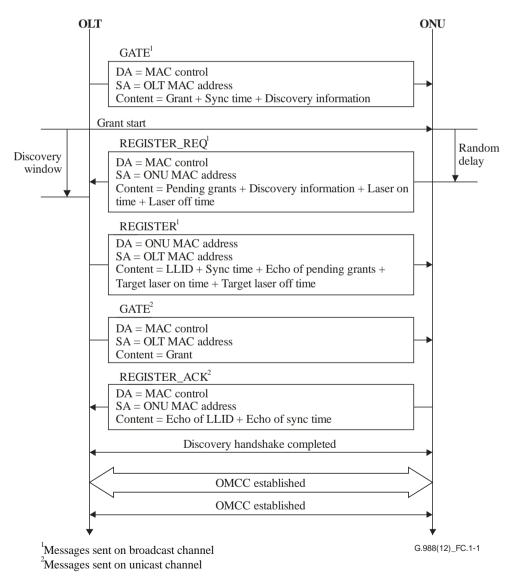
Figure C.1-1 – OMCC establishment process, Ethernet PON
