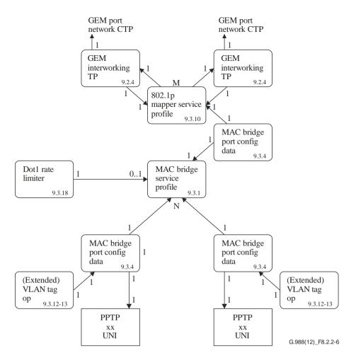
Figure 8.2.2-6 – Illustration of N:M bridge-mapping
