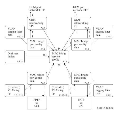
Figure 8.2.2-8 – Illustration of N:P bridge-filtering
