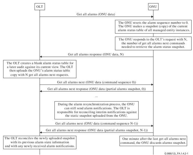
Figure A.1.4.2-1 – Alarm resynchronization
