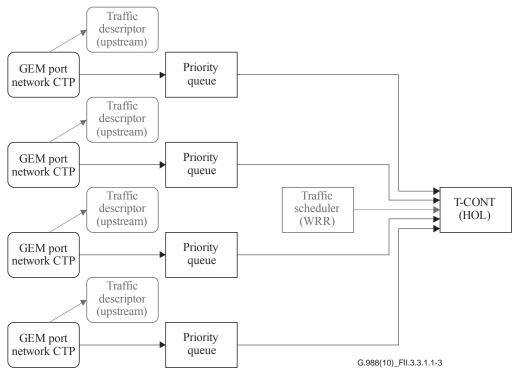
NOTE – The traffic scheduler performs no function in this example. It is shown to illustrate components that may be present as inbuilt features of the ONU architecture.
