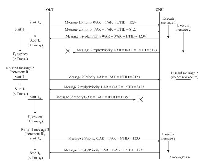
Figure B.2.1-1 - Concurrent message exchange with error recovery
