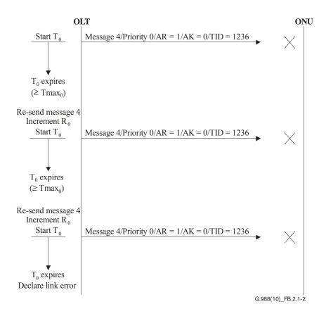
Figure B.2.1-2 – OMCC link error detection
