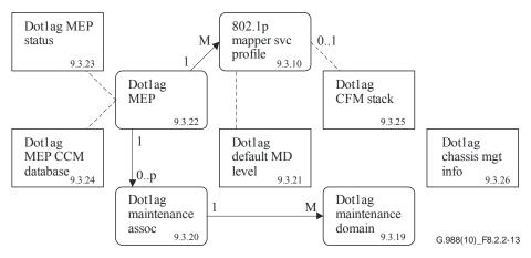
NOTE – If a mapper is associated with ports of a bridge, the 802.1ag entities should be associated with the bridge and its ports, rather than with the mapper.
