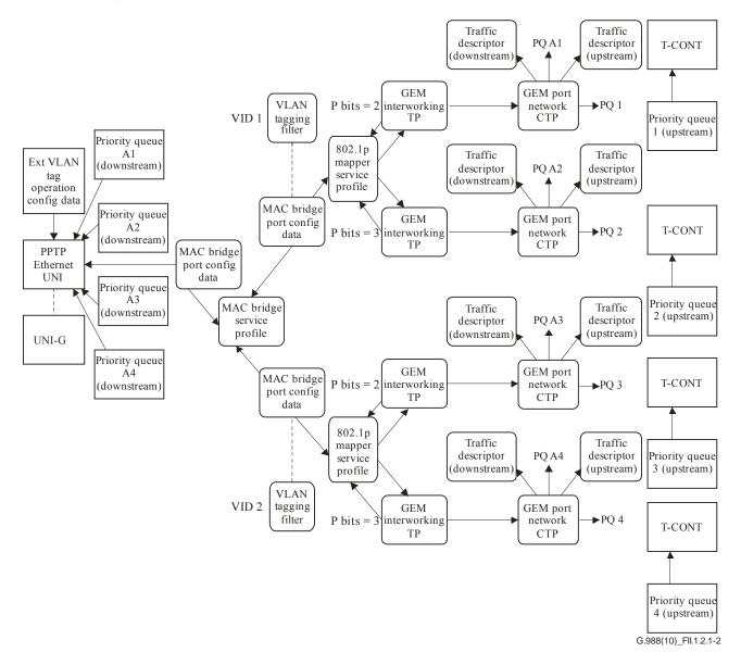
Figure II.1.2.1-2 – Single UNI, two VLANs, VID-based priorities
