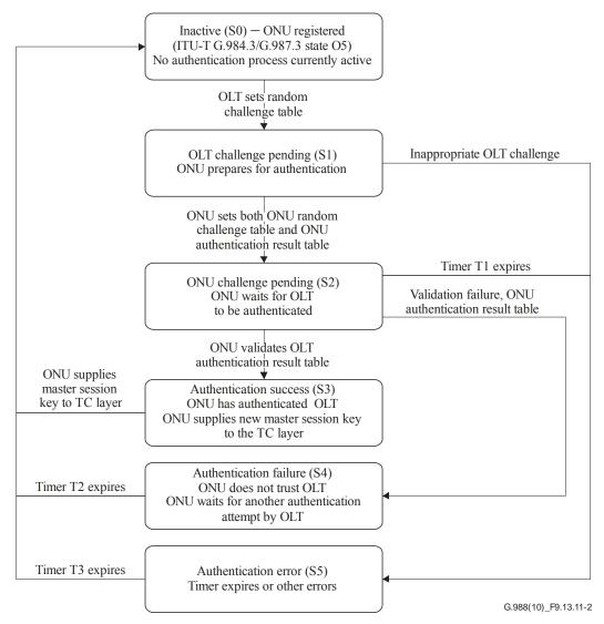
NOTE 1-Timer T1: ONU challenge pending timer. Timer T1 is used to abort an unsuccessful OLT authentication attempt by limiting the overall time an ONU can remain in state S2. The recommended value of T1 is 3 seconds.
