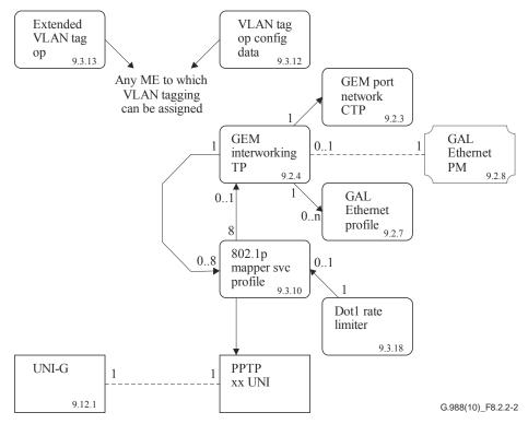
NOTE – A mapper service profile may be associated with any IEEE 802.3 UNI, such as Ethernet or xDSL, or another IEEE 802.3 function such as an IP host config data ME.
