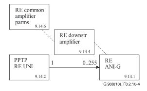
Figure 8.2.10-4 – Mid-span downstream PON reach extender core (hybrid)
