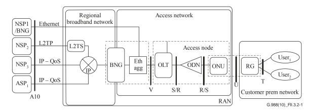
Figure II.3.2-1 – High-level architecture
