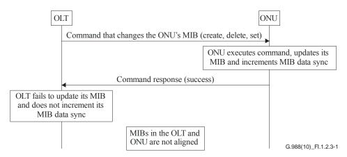
Figure I.1.2.3-1 – Mismatch of MIBs at ONU and OLT under OLT command
