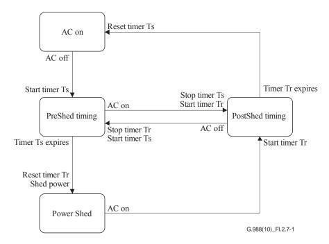
Figure I.2.7-1 – Power shedding state diagram
