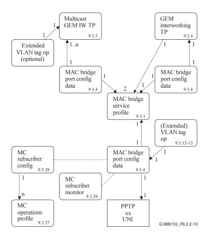
Figure 8.2.2-10 – Illustration of multicast service
