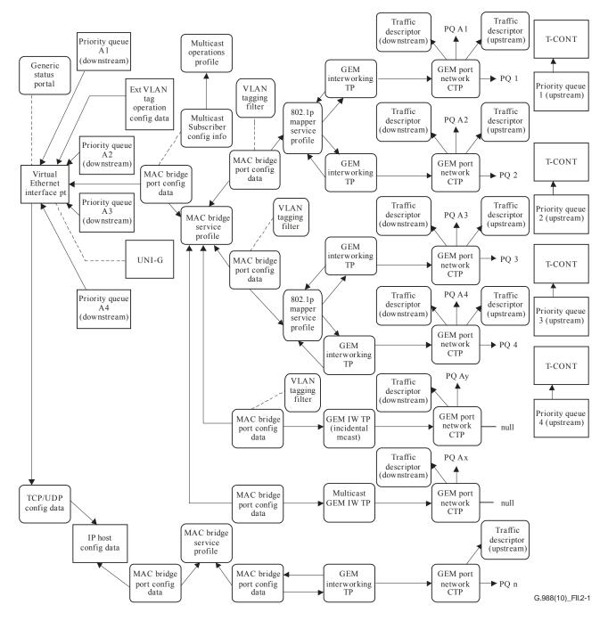
Figure II.2-1 – Dual-managed ONU model
