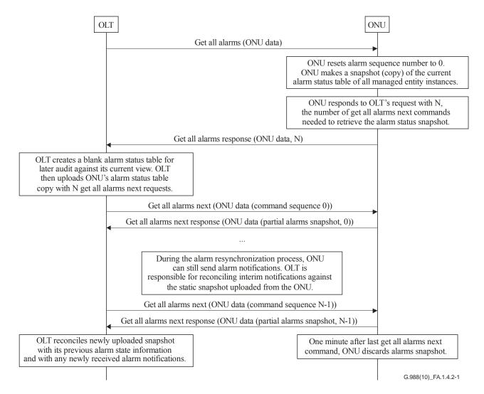
Figure A.1.4.2-1 – Alarm resynchronization
