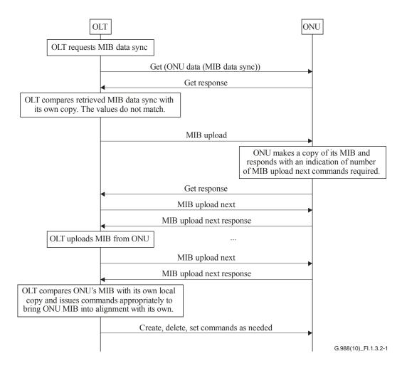
Figure I.1.3.2-1 – MIB resynchronization
