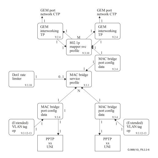
Figure 8.2.2-6 – Illustration of N:M bridge-mapping
