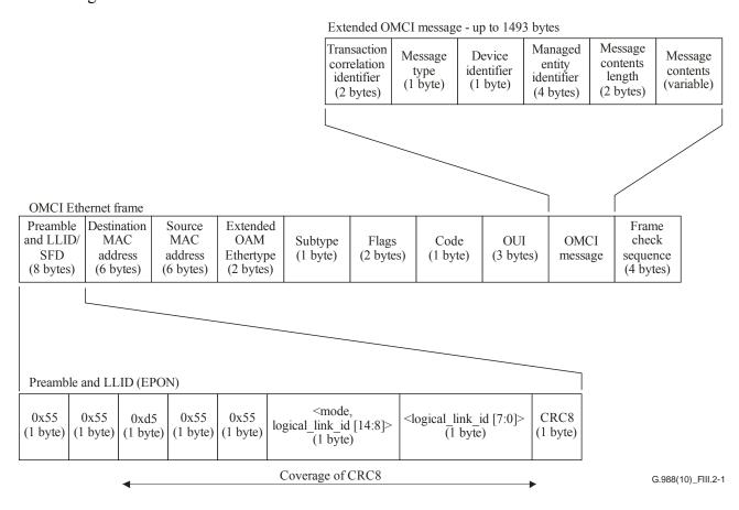
Figure III.2-1 – Extended OAM frame structure for EPON OMCI
