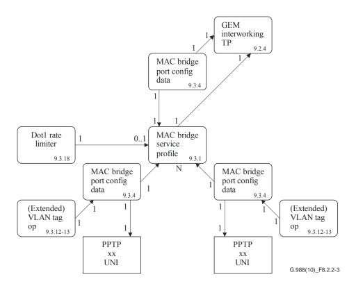
Figure 8.2.2-3 – Illustration of N:1 bridging
