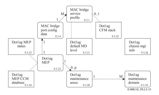
Figure 8.2.2-12 – Illustration of [IEEE 802.1ag] in MAC bridge model
