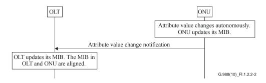
Figure I.1.2.2-2 – No increment of MIB data sync at ONU and OLT
