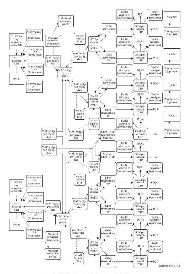
Figure II.1.3.1.2-1 - Multi-UNI L2-OCM with multicast
