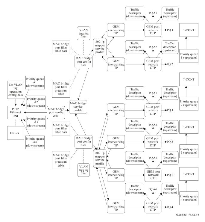
Figure II.1.2.1-1 – Single UNI, two VLANs with common priorities
