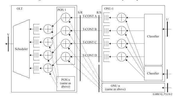
Figure II.3.2.6-2 – Upstream functionality example
