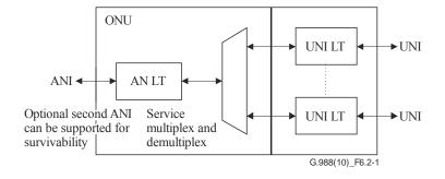
Figure 6.2-1 – ONU functional block diagram
