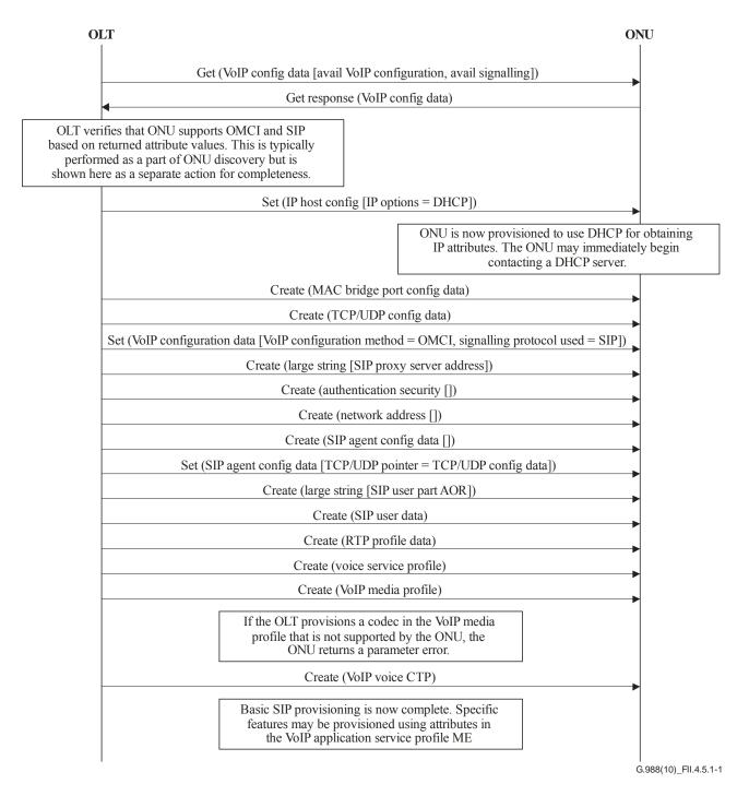
Figure II.4.5.1-1 – SIP provisioning flow
