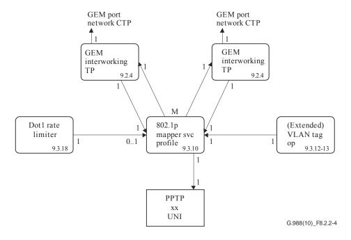
Figure 8.2.2-4 – Illustration of 1:M mapping
