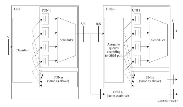
Figure II.3.2.6-1 – Downstream functionality example
