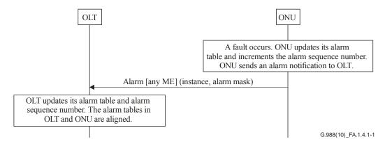
Figure A.1.4.1-1 – Increment of alarm sequence number at ONU and OLT
