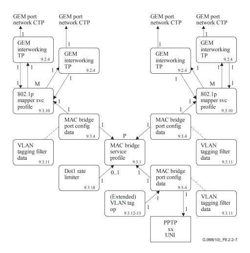
Figure 8.2.2-7 – Illustration of 1:MP map-filtering
