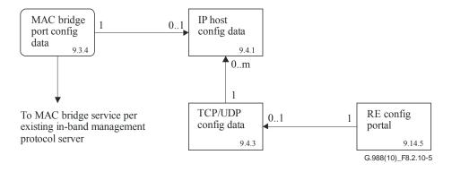
Figure 8.2.10-5 - In-band management for mid-span PON reach extender
