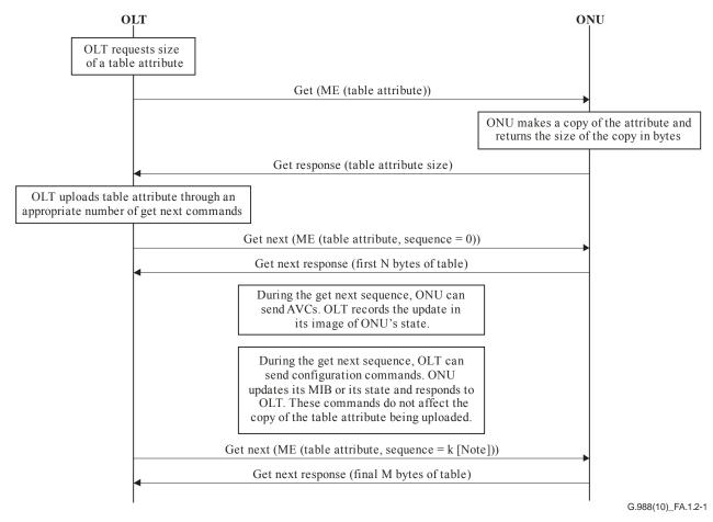
NOTE-k+1 is the number of get next commands as derived by the OLT to retrieve the complete table. For baseline OMCI messages, each get next response contains 29 bytes; for extended OMCI messages, up to 1966 bytes (1980 maximum PDU size – 14 bytes of OMCI header) are returned in a full-length response.
