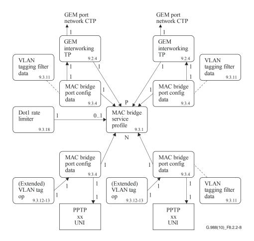
Figure 8.2.2-8 – Illustration of N:P bridge-filtering
