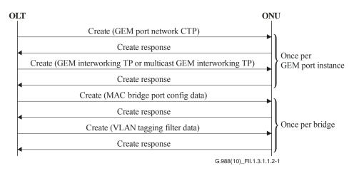
Figure II.1.3.1.1.2-1 – Data plane provisioning
