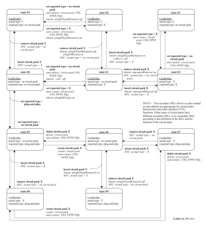
Figure 9.1.5-1 – Cardholder state diagram
