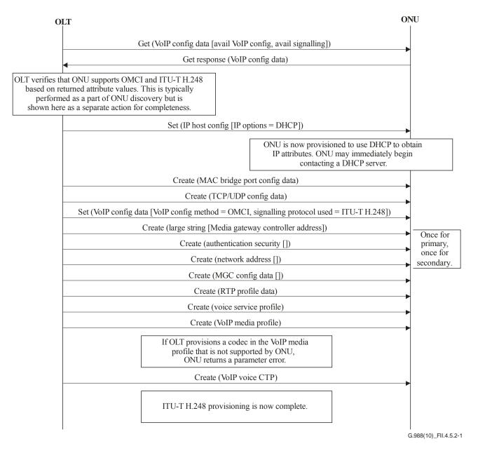
Figure II.4.5.2-1 – ITU-T H.248 provisioning flow
