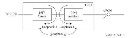
Figure 9.8.1-1 – CES loopback configuration
