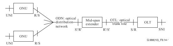
Figure 9.14.1 – Mid-span PON reach extender
