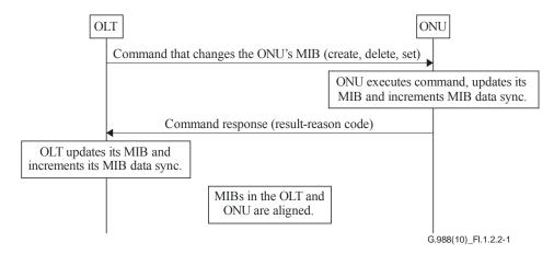
Figure I.1.2.2-1 - Increment of MIB data sync at ONU and OLT under OLT command
