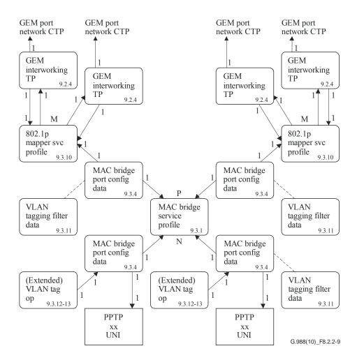
Figure 8.2.2-9 – Illustration of N:MP bridge-map-filtering
