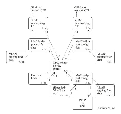
Figure 8.2.2-5 – Illustration of 1:P filtering
