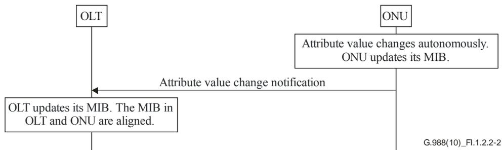
**Figure I.1.2.2-2 – No increment of MIB data sync at ONU and OLT**
