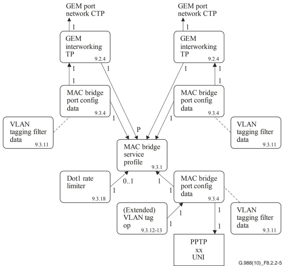
**Figure 8.2.2-5 – Illustration of 1:P filtering**
