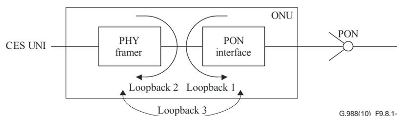
**Figure 9.8.1-1 – CES loopback configuration**
