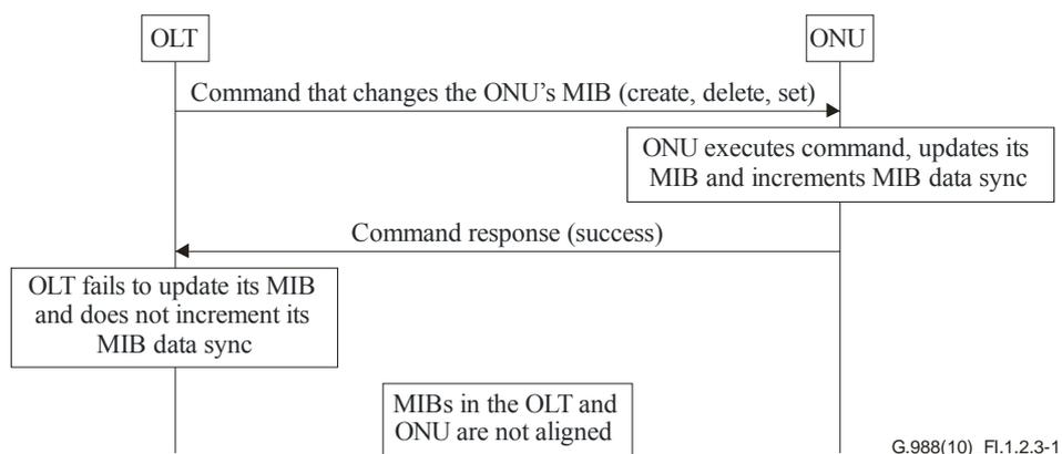
**Figure I.1.2.3-1 – Mismatch of MIBs at ONU and OLT under OLT command**
