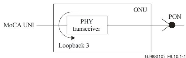
**Figure 9.10.1-1 – MoCA loopback configuration**
