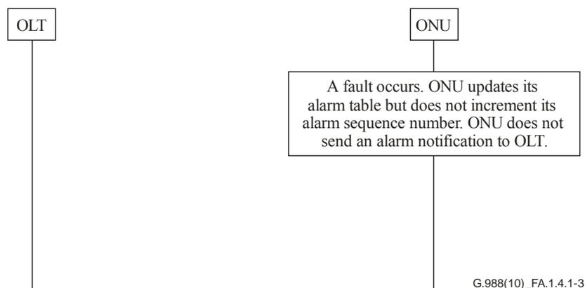
**Figure A.1.4.1-3 – No increment of alarm sequence number at ONU and OLT under ARC**
