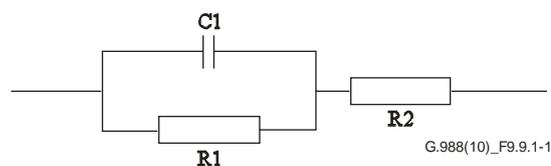
**Figure 9.9.1-1 – Impedance model for POTS UNI**
