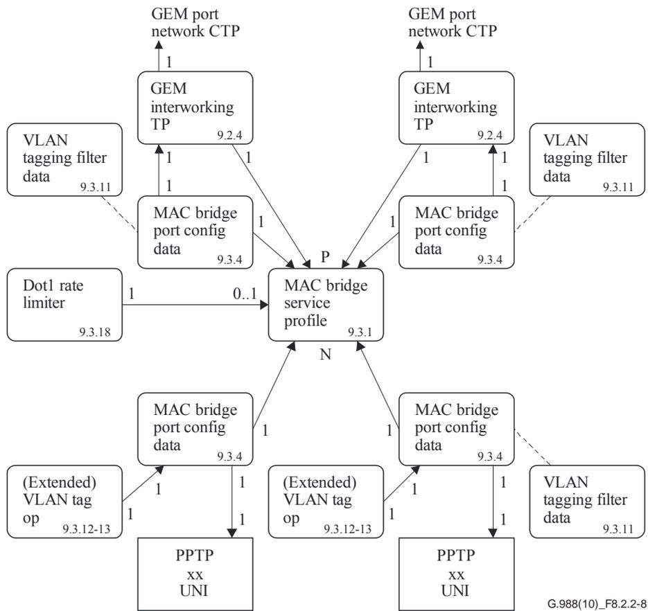
**Figure 8.2.2-8 – Illustration of N:P bridge-filtering**
