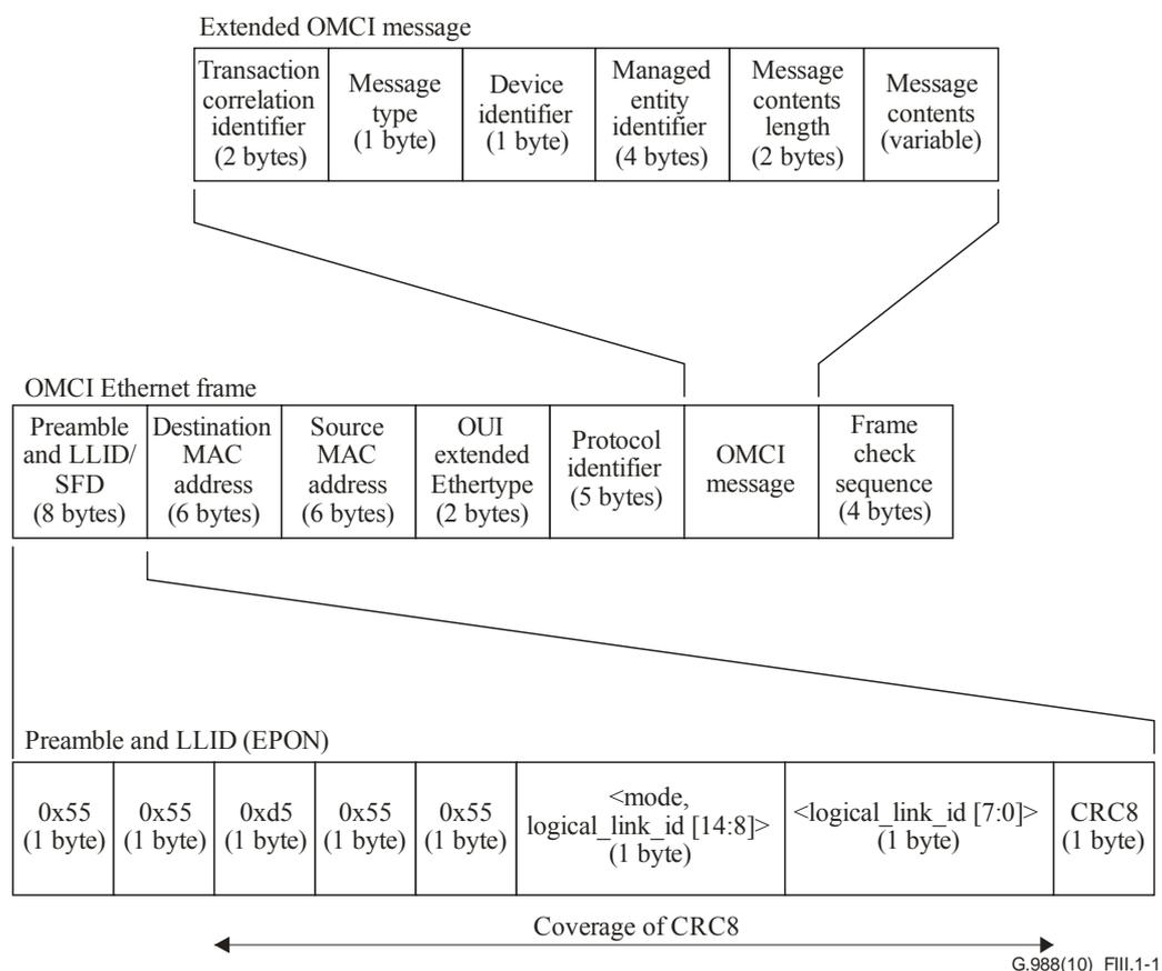
**Figure III.1-1 – OMCI Ethernet frame structure, Ethernet PON**
