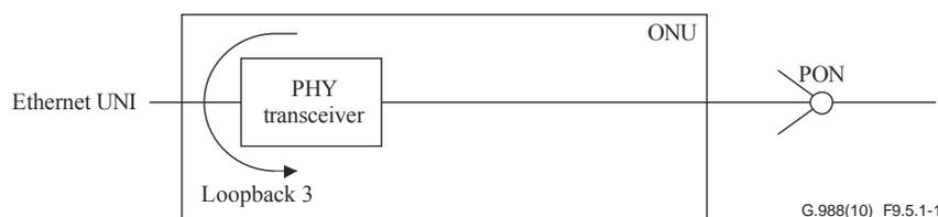
**Figure 9.5.1-1 – Ethernet loopback configuration**
