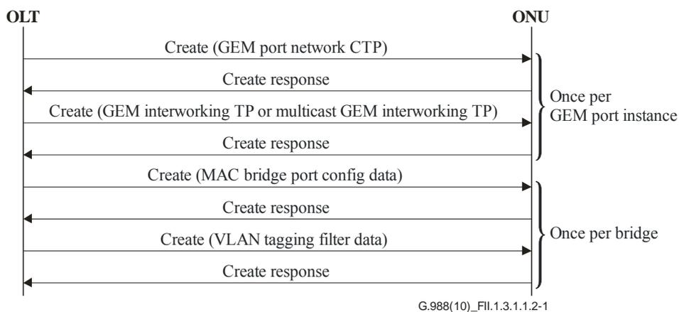
**Figure II.1.3.1.1.2-1 – Data plane provisioning**
