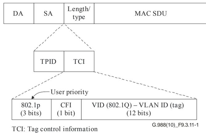
**Figure 9.3.11-1 – Format of an Ethernet frame for VLAN services**
