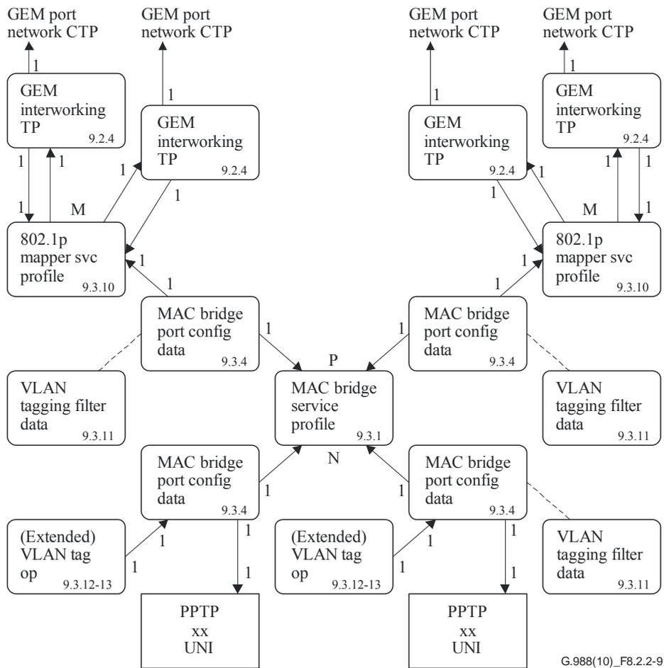
**Figure 8.2.2-9 – Illustration of N:MP bridge-map-filtering**
