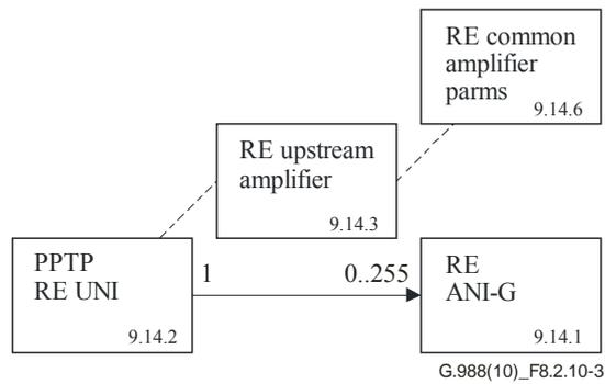
**Figure 8.2.10-3 – Mid-span upstream PON reach extender core (hybrid)**
