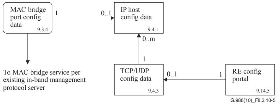
**Figure 8.2.10-5 – In-band management for mid-span PON reach extender**
