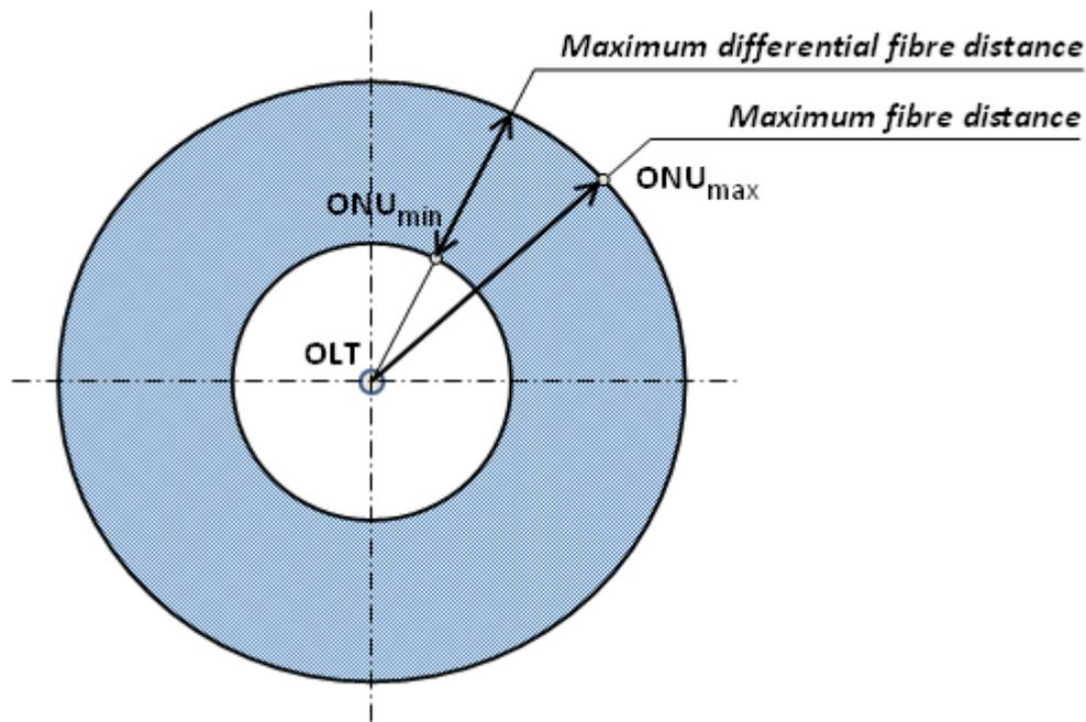
**Figure 5-4 – Fibre distance concepts**
