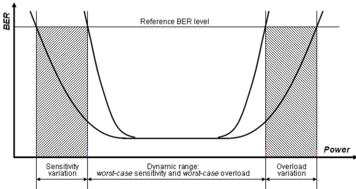
**Figure 5-3 – Rx output BER as a function of received optical power, and the definition of dynamic range**
