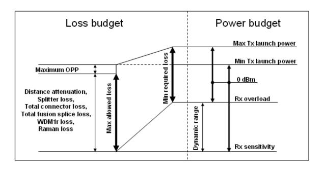
Figure 5-2 – Relationship between the power and loss budget parameters
