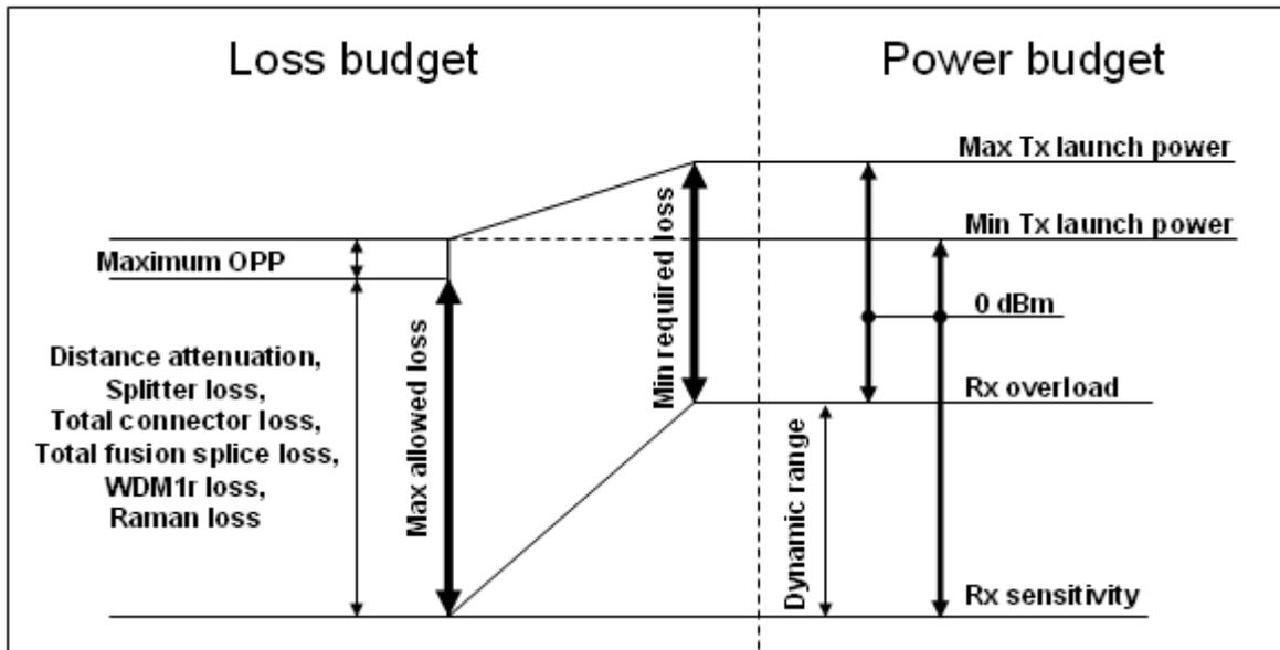
**Figure 5-2 – Relationship between the power and loss budget parameters**
