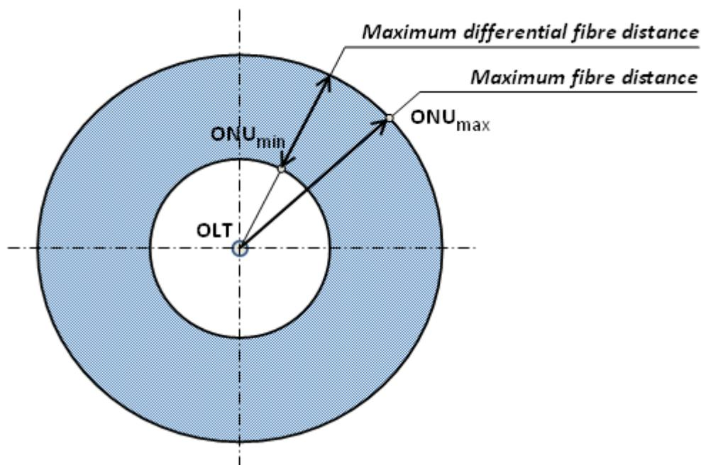
Figure 5-4 – Fibre distance concepts
