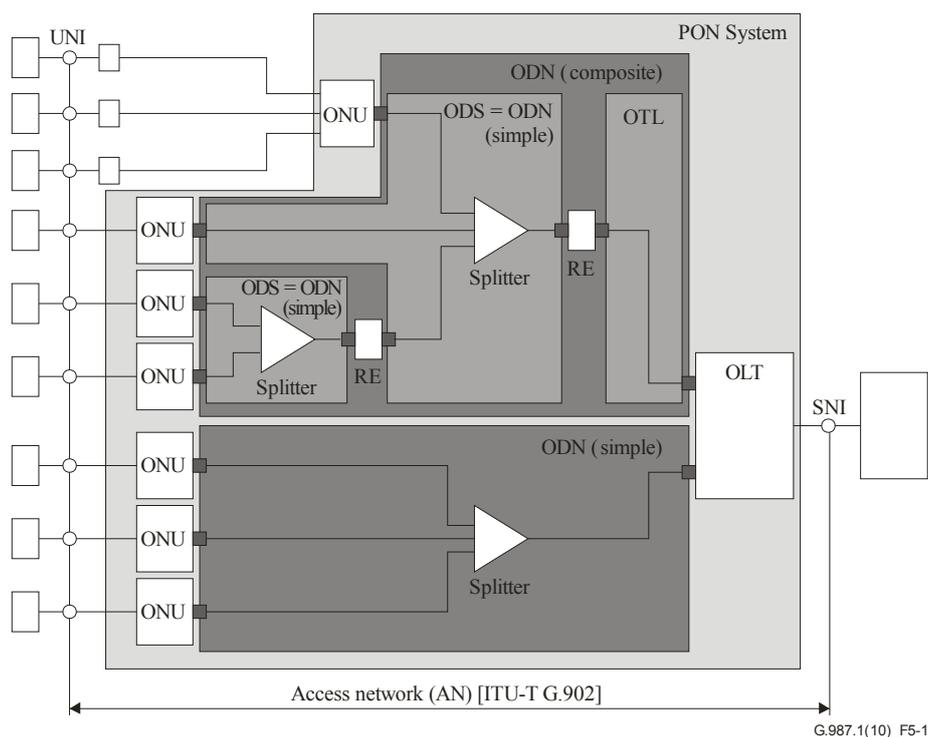
**Figure 5-1 – Reference access network architecture**
