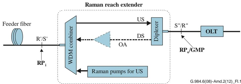
**Figure I.1 – Reverse pumped distributed Raman amplifier for Raman RE**
