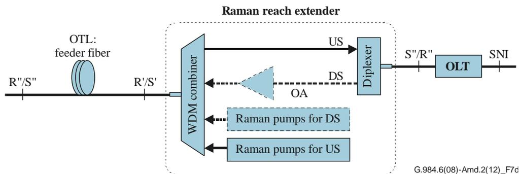
**Figure 7d – Example configuration for Raman RE; OA and Raman pumps for DS are optional**
