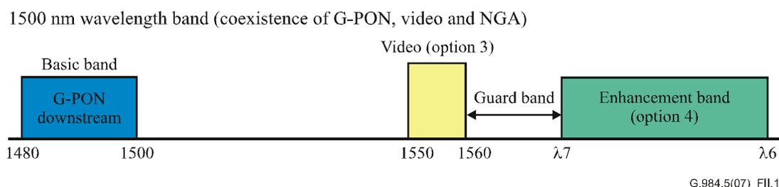
Figure II.1 – Wavelength allocation
