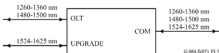
**Figure I.1 – Reference diagram of WDM1**
