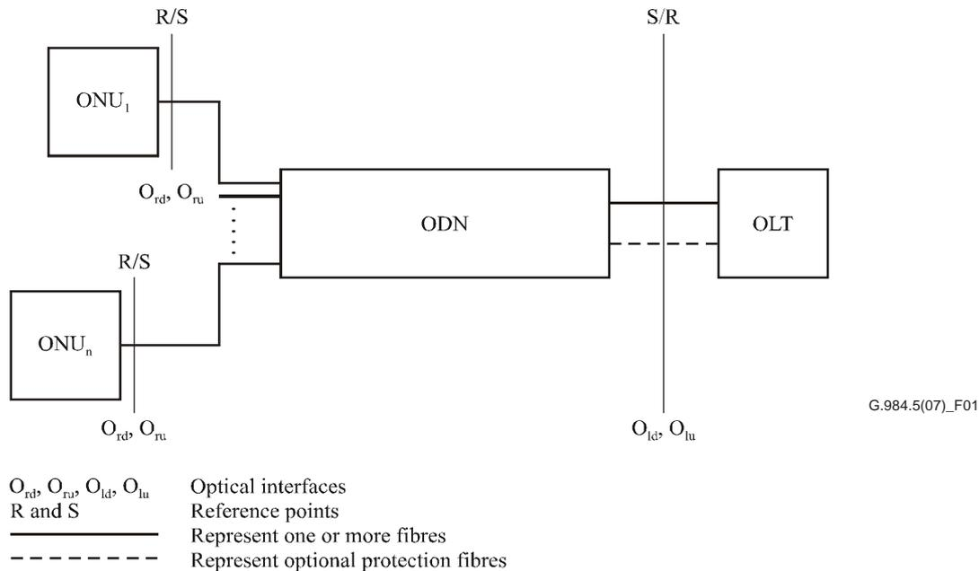
**Figure 1 – Generic physical configuration of the optical distribution network (reproduced from Figure 5 of [ITU-T G.983.1])**
