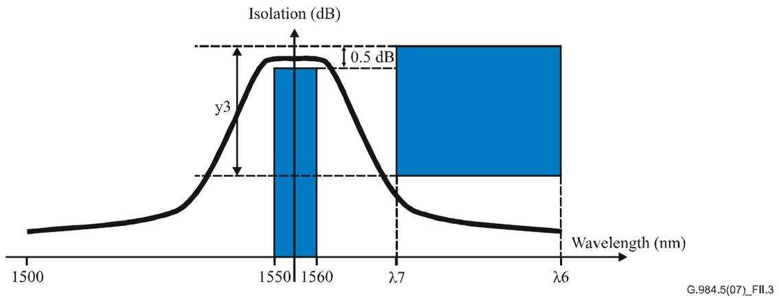
**Figure II.3 – Example of integrated filter characteristics for video**
