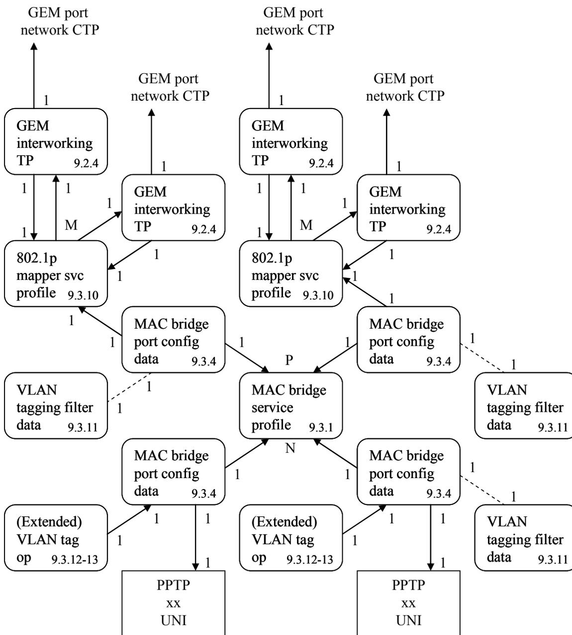
**Figure 8.2.2-9 – Illustration of N:MP bridge-map-filtering**
