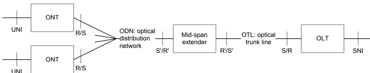
Figure 9.14-1 – Mid-span PON reach extender
