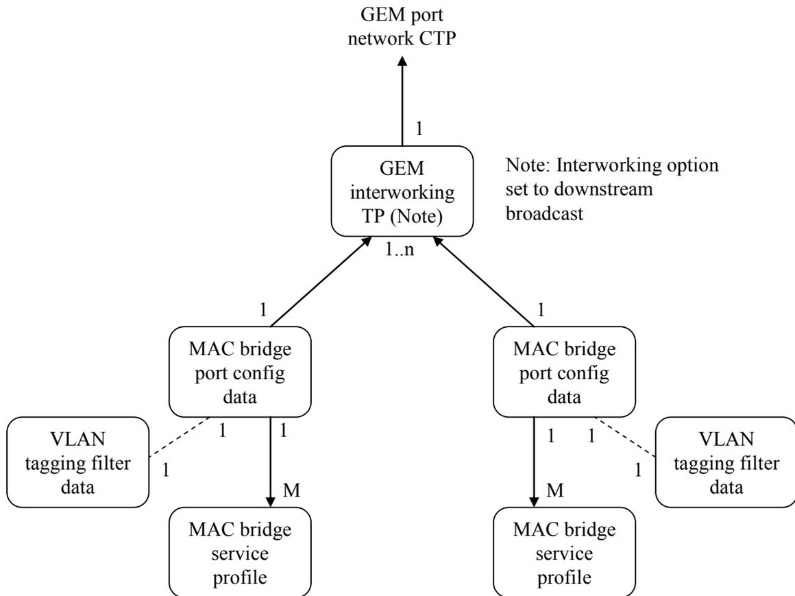
Figure 8.2.2-11 – Illustration of downstream broadcast configuration
