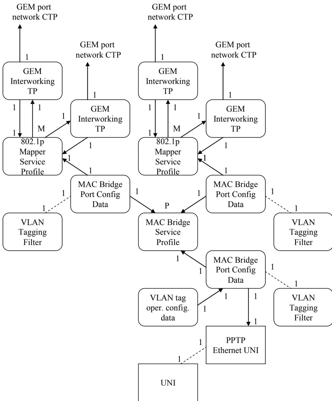
**Figure 8.2.2-7 – Illustration of 1:MP map-filtering**
