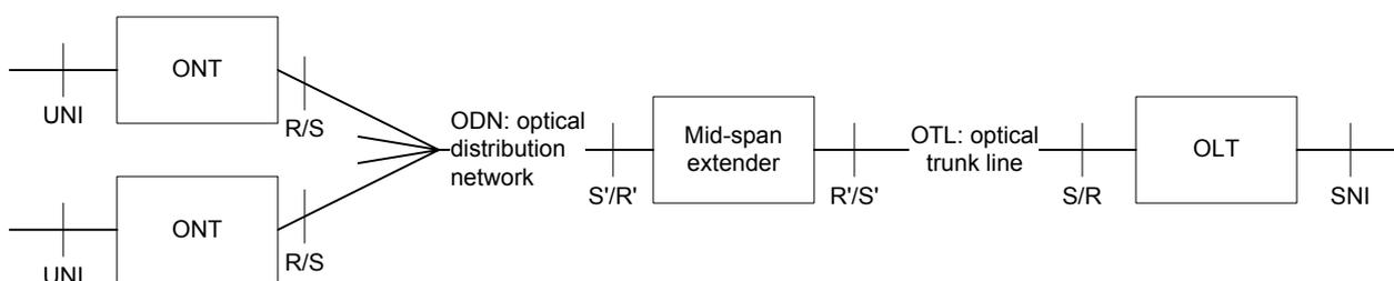
**Figure 9.14-1 – Mid-span PON reach extender**
