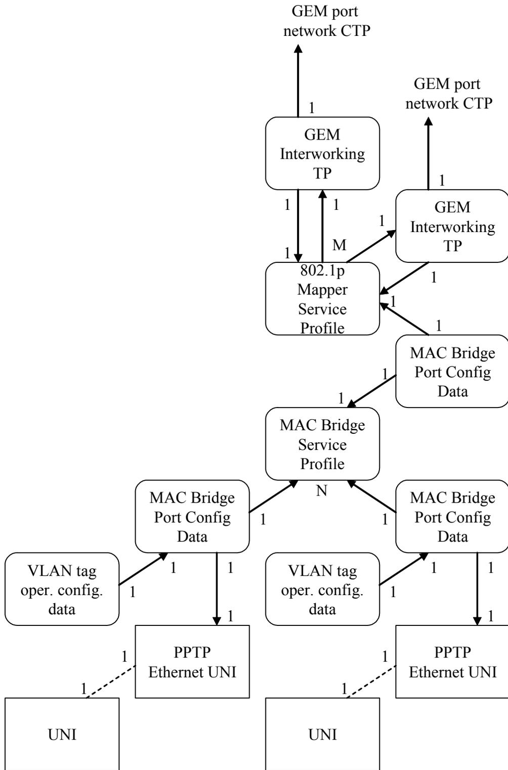
**Figure 8.2.2-6 – Illustration of N:M bridge-mapping**
