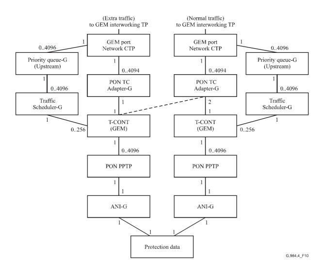
Figure 10/G.984.4 – Part of ME relation diagram for 1:1 protection
