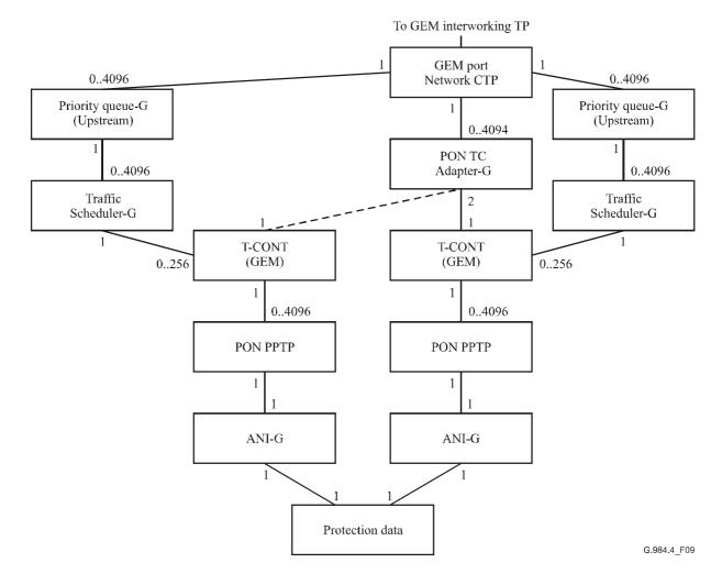
Figure 9/G.984.4 – Part of ME relation diagram for 1+1 protection
