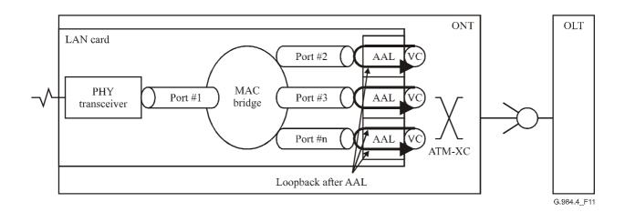
Figure 11/G.984.4 – Schematic diagram of loopback after AAL
