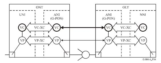
Figure 4/G.984.4 – ATM VC cross-connection termination model
