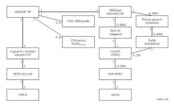
Figure 8/G.984.4 – ME relation diagram for structured CES
