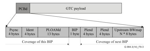
Figure 8-3 – GTC physical control block downstream (PCBd)
