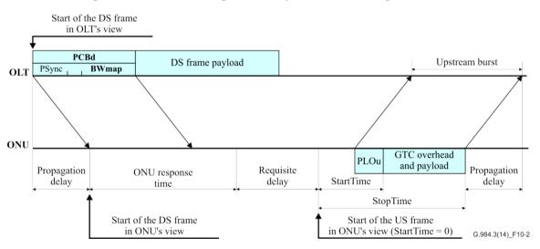
Figure 10-2 – ONU timing diagram – General case
