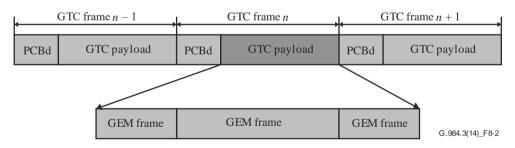
Figure 8-2 – Downstream GTC frame
