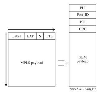
Label: Label value, EXP: Experimental use, S: Bottom of stack
