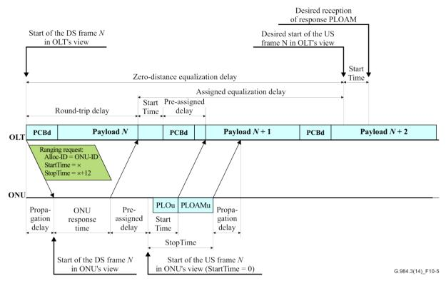
Figure 10-5 – Equalization delay measurements
