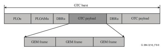
Figure 8-9 – Upstream GTC burst
