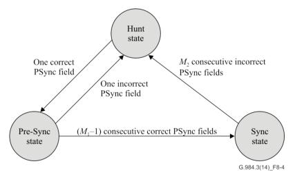
Figure 8-4 – GTC downstream ONU synchronization state machine
