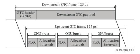
Figure 8-1 – GTC layer framing
