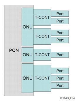
Figure 5-2 – Upstream multiplexing
