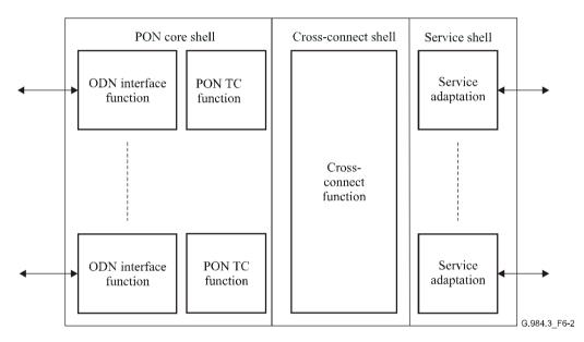
Figure 6-1 – OLT functional block diagram
