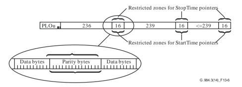
Figure 13-6 – Pointer restrictions in the case of contiguous allocations with FEC
