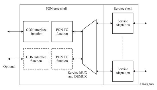
Figure 6-2 – ONU functional block diagram
