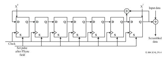
Figure A.4 – Scrambler block diagram
