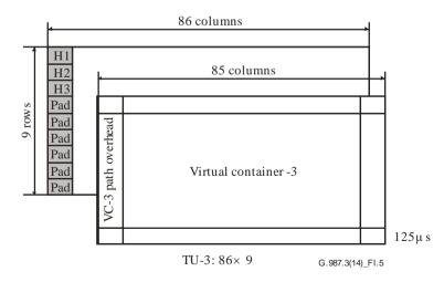
Figure I.5 – The TU-3 frame structure
