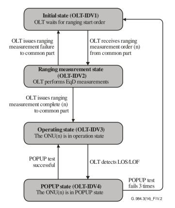
Figure IV.2 – ONU-specific part state diagram
