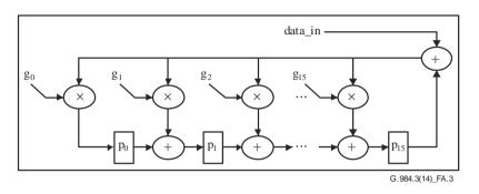
Figure A.3 – IIR model for FEC encoder
