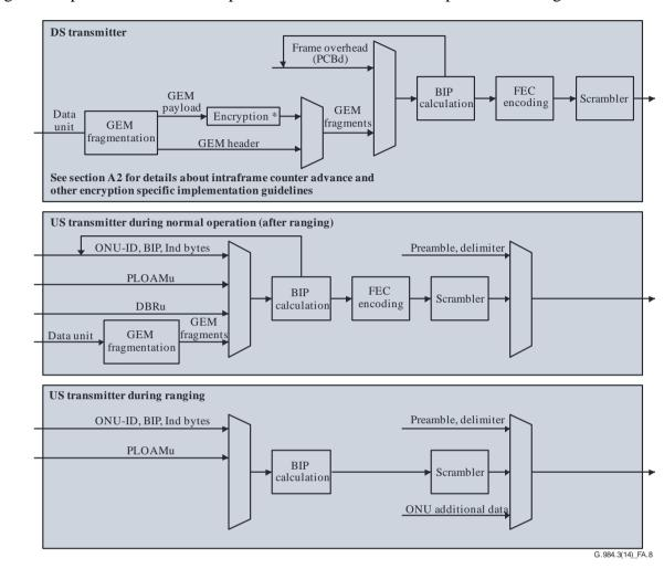
Figure A.8 presents the order of operations in downstream and upstream framing.
