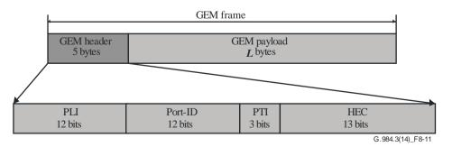
Figure 8-11 – GEM header and frame structure
