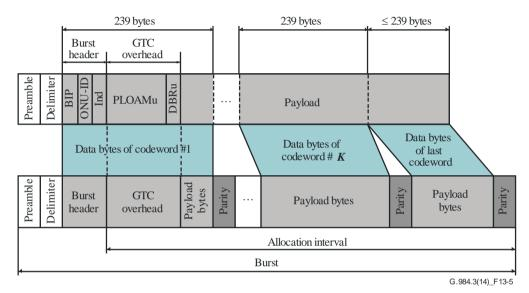
Figure 13-5 – US transmission with FEC parity bytes insertion
