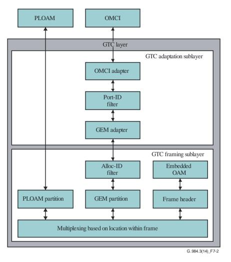
Figure 7-2 – Functional blocks in the C/M-plane
