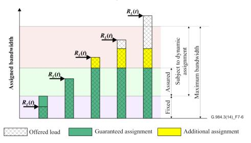
Figure 7-6 – Variants of bandwidth assignment for different offered loads
