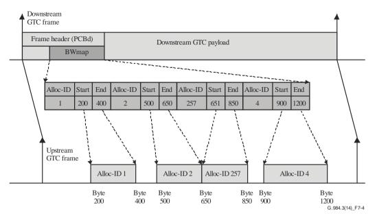
Figure 7-4 – GTC media access control concept
