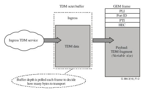
Figure I.2 – TDM mapping over GEM
