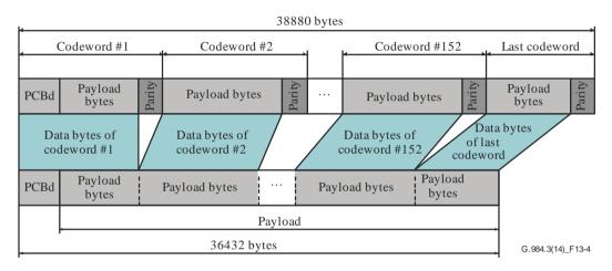
Figure 13-4 – Payload reconstruction at the FEC decoder
