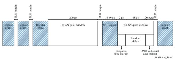
Figure A.6 – Serial number request example
