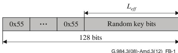
**Figure B.1 – Format of a data encryption key with reduced effective length**
