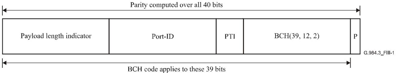
**Figure III.1 – The GEM header structure, showing detail of the 13-bit header error control field**
