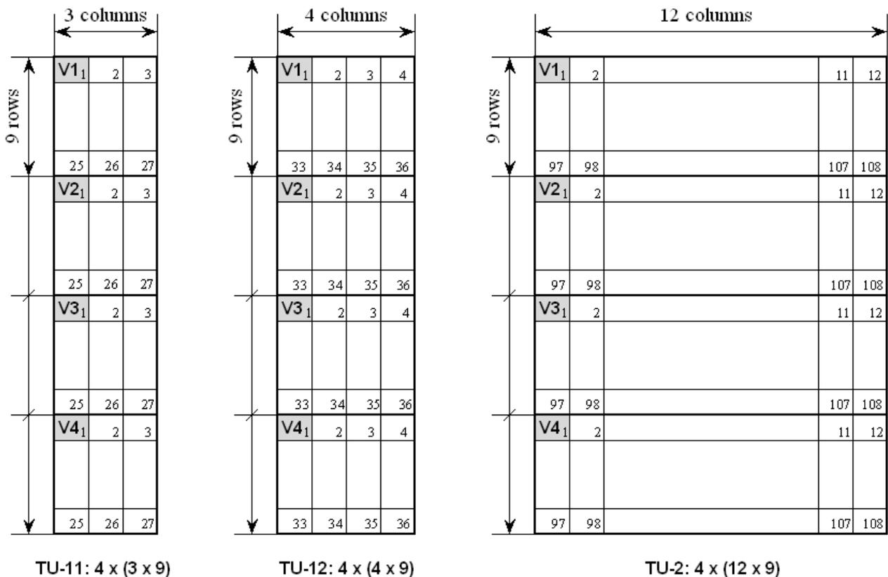
Figure I.4 – The TU-11, TU-12 and TU-2 four-frame multiframe Structures
