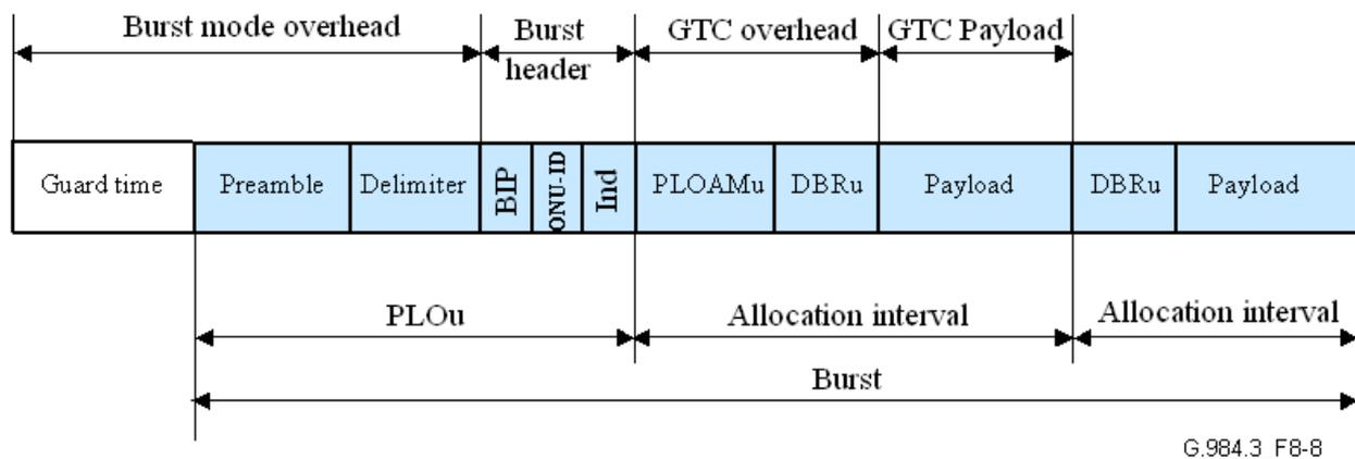
**Figure 8-8 – Details of physical and GTC layer upstream overhead**
