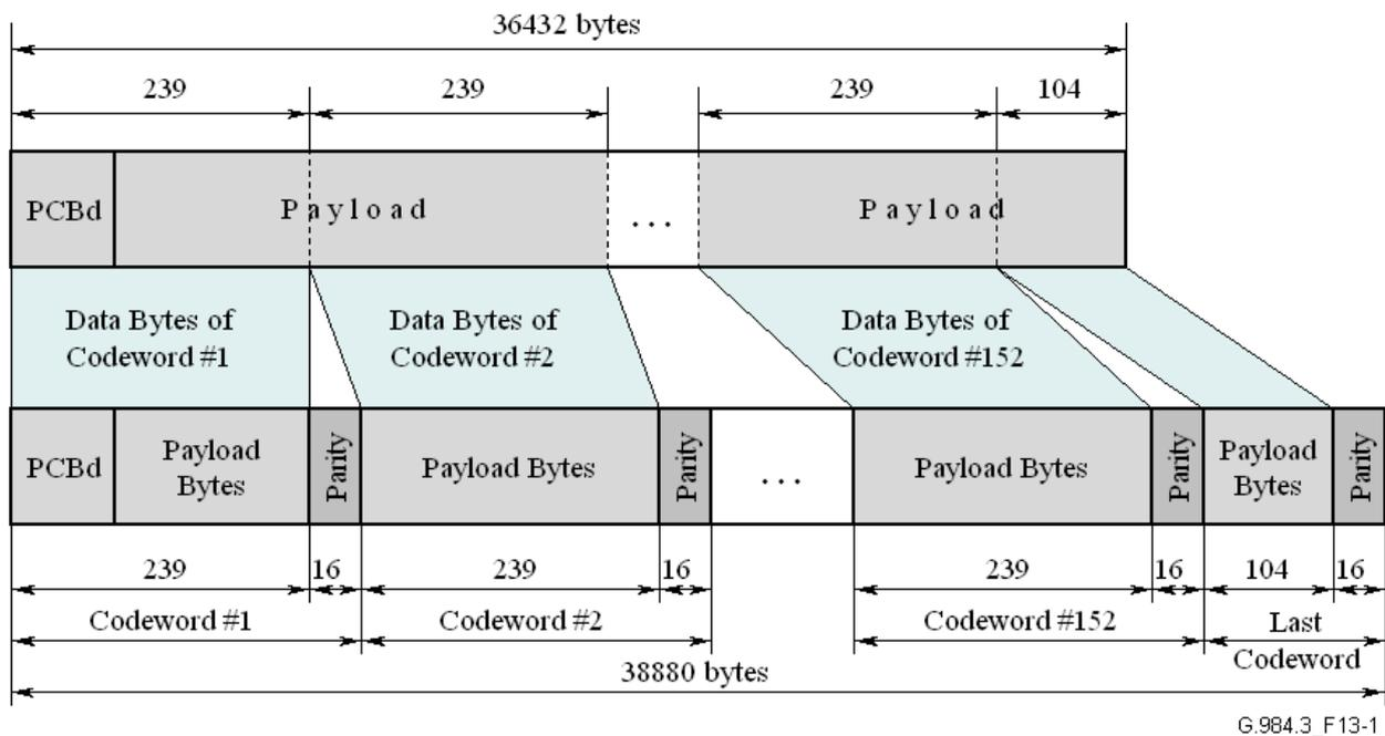
**Figure 13-1 – DS transmission with FEC parity bytes insertion**
