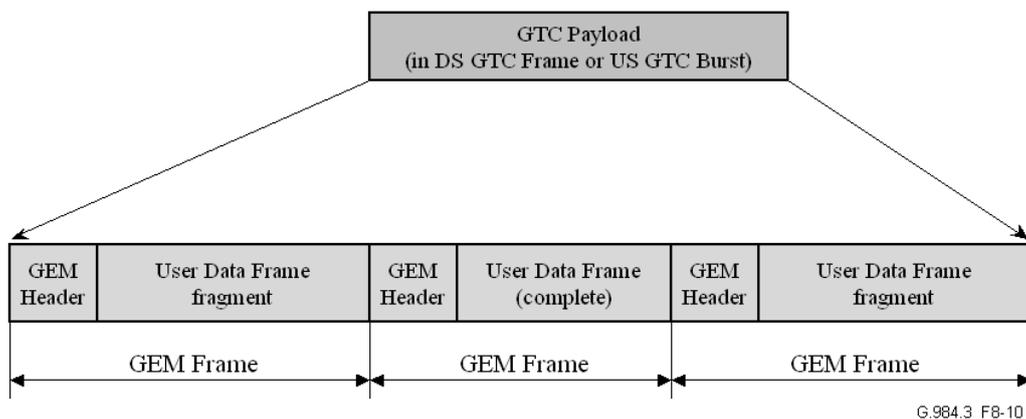
Figure 8-10 – Mapping of GEM frames into GTC payload
