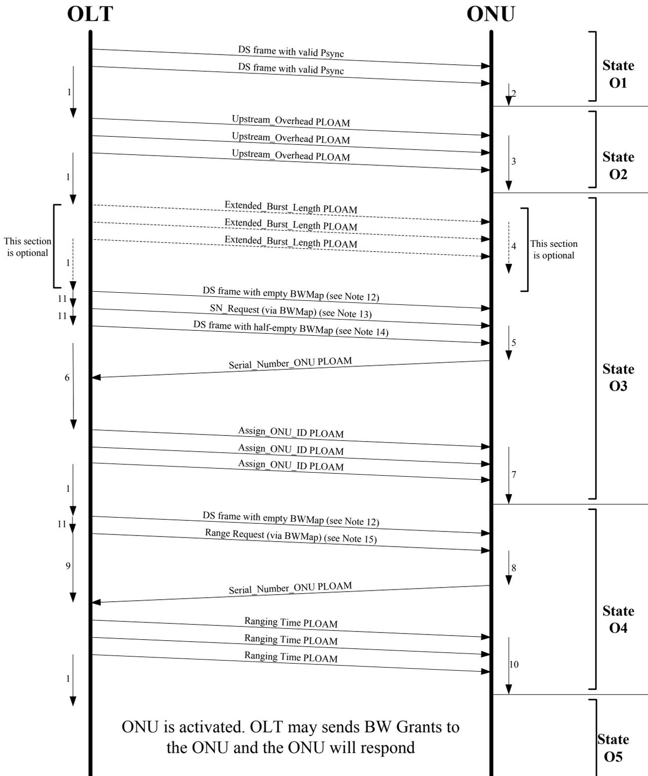
**Figure A.6-1 – Activation process flow**
