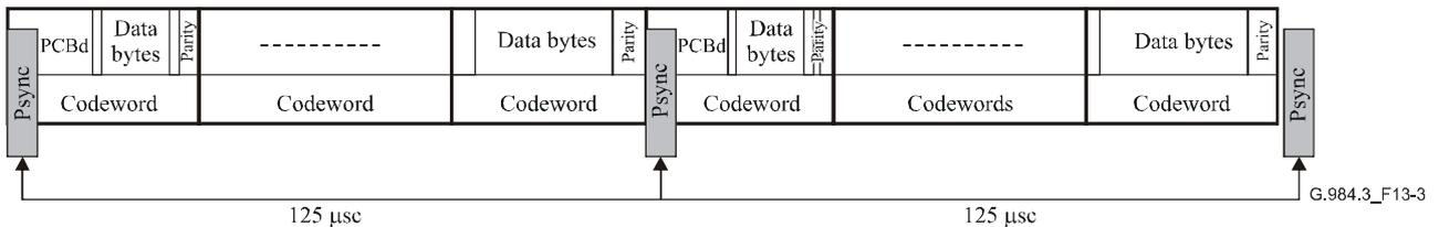
**Figure 13-3 – DS frame synchronization**
