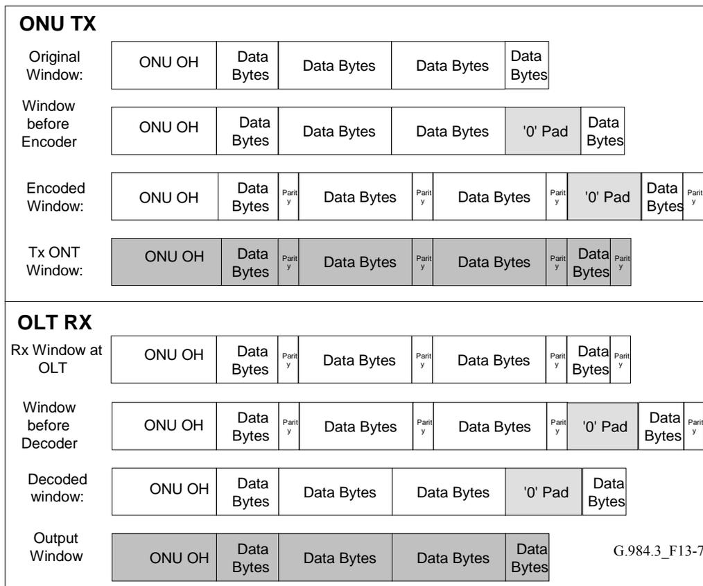
**Figure 13-7 – US transmission with FEC structure**
