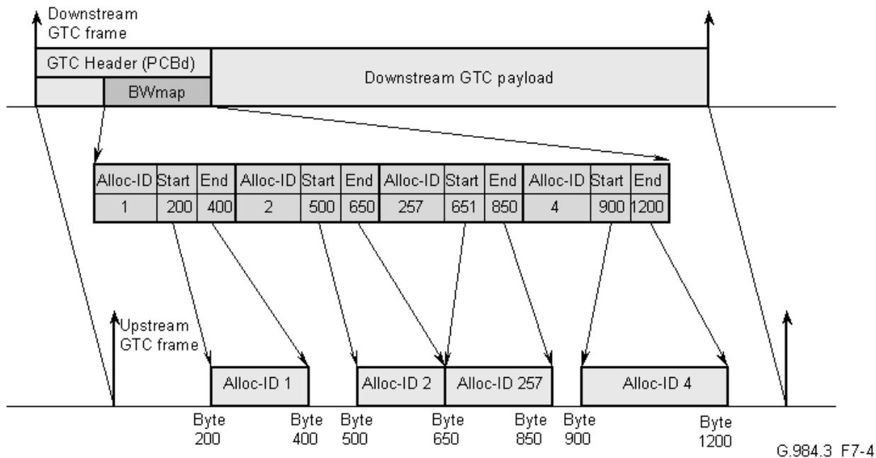
**Figure 7-4 – GTC media access control concept**
