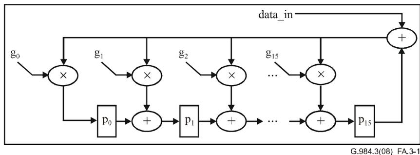
**Figure A.3-1 – IIR model for FEC encoder**
