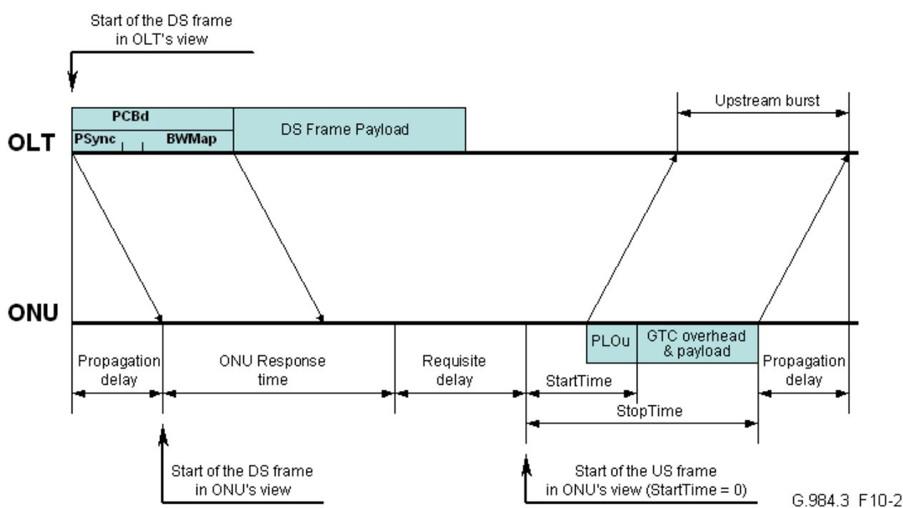
**Figure 10-2 – ONU timing diagram – General case**
