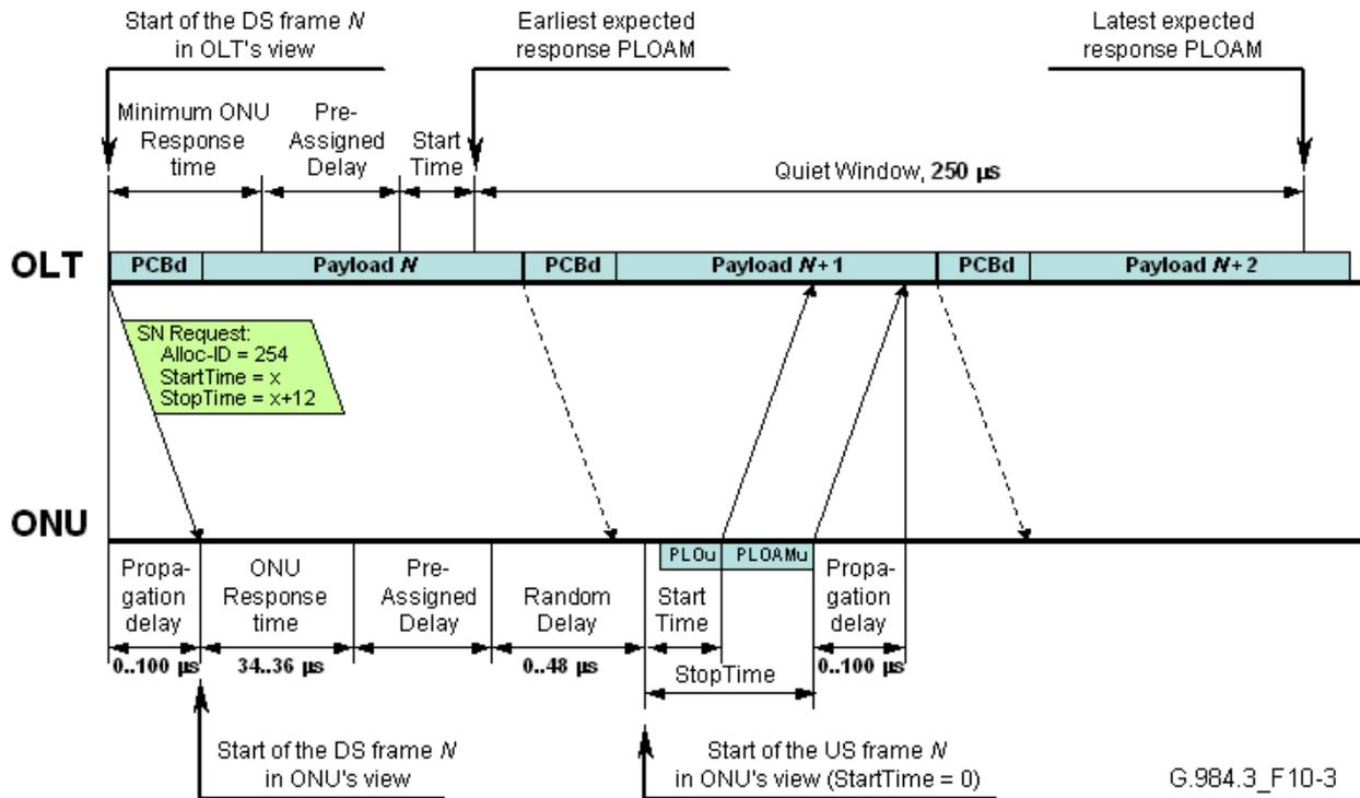
Figure 10-3 – Timing relationships during serial number acquisition
