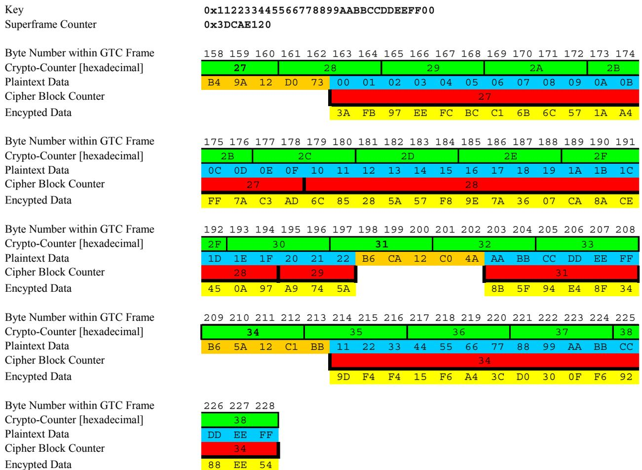
Figure A.2-1 – Relationship between data and crypto-counter; no FEC
