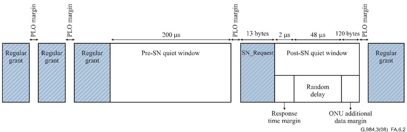
Figure A.6-2 – Serial number request example
