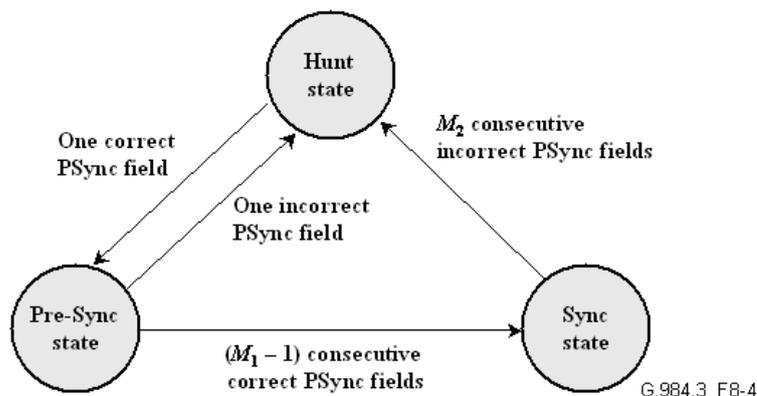
**Figure 8-4 – GTC downstream ONU synchronization state machine**
