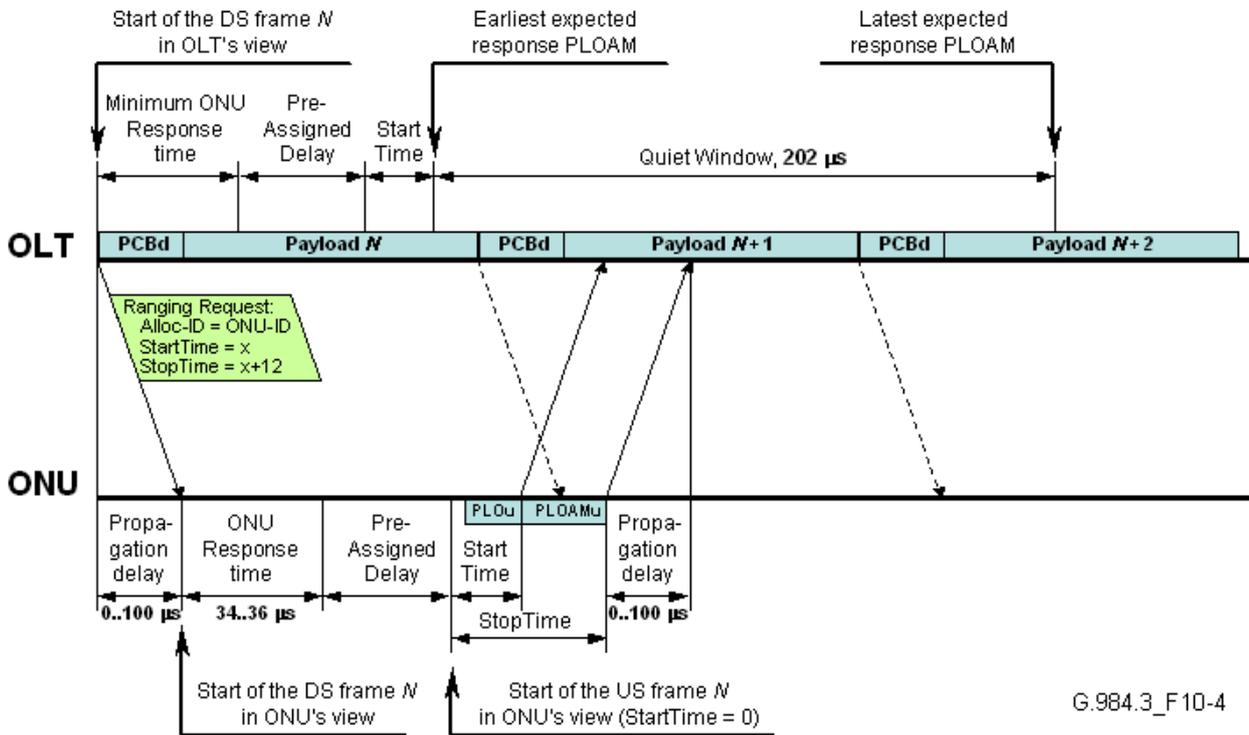
Figure 10-4 – Timing relationships during ranging
