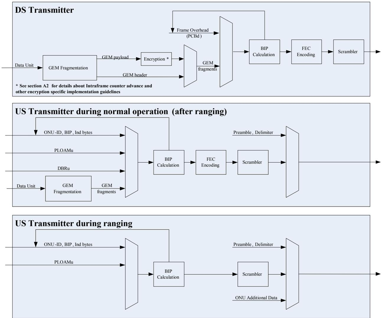
Figure A.8-1 – Transmitter block diagram
