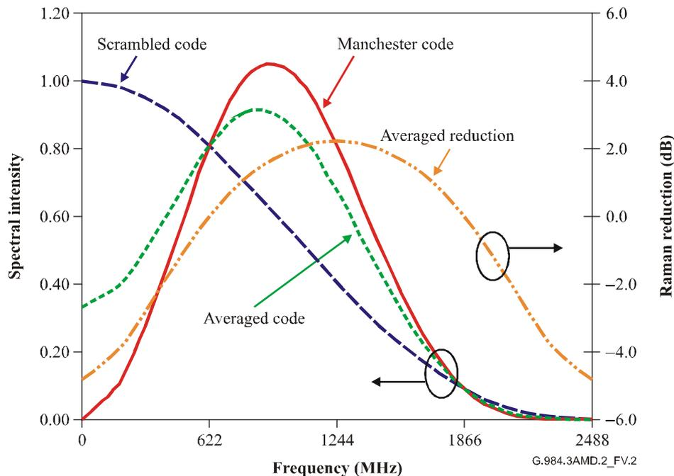
**Figure V.2/G.984.3 – Spectra of ordinary scrambled pattern, Manchester-coded pattern, the average code, and the average reduction in spectral intensity**
