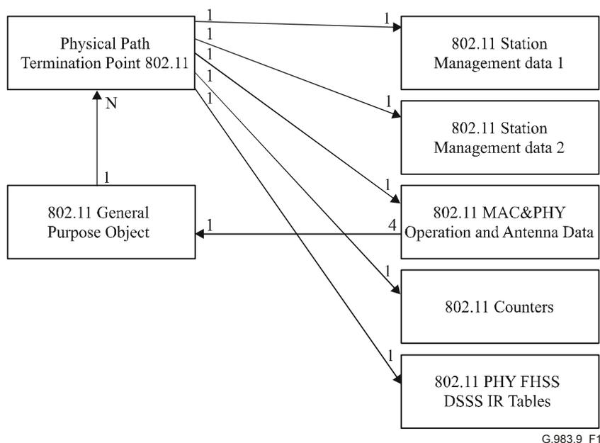
**Figure 1/G.983.9 – Managed entity relation diagram for IEEE 802.11 interface support**
