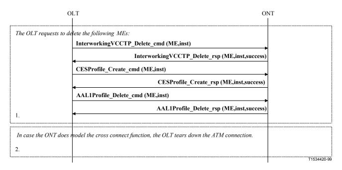
Figure I.21/G.983.2 – Connection tear-down of an unstructured CES
