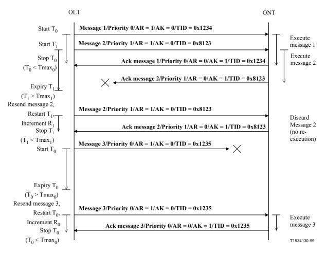
Figure 14/G.983.2 – Concurrent Message Exchange with Error Recovery
