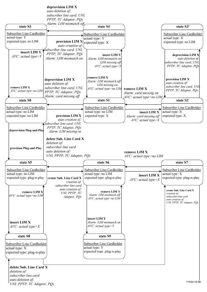
Figure 10/G.983.2 - Subscriber Line Cardholder state diagram
