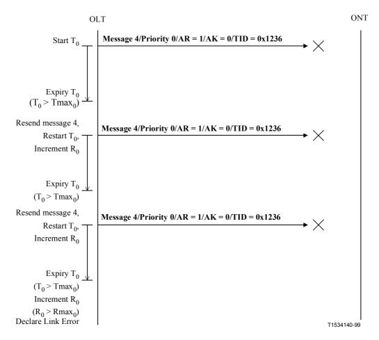
Figure 15/G.983.2 – OMCC Link Error Detection
