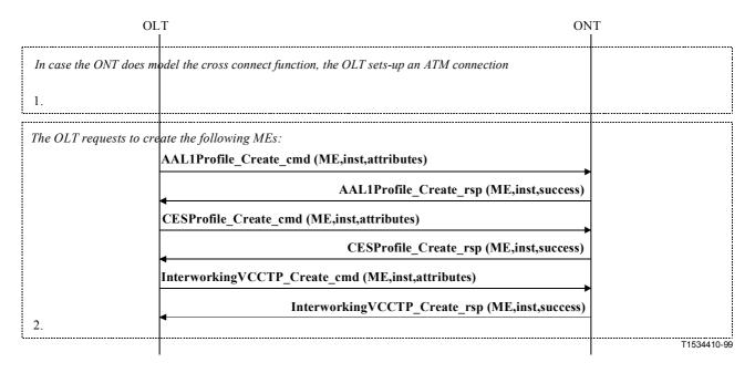
Figure I.20/G.983.2 – Connection set-up of an unstructured CES
