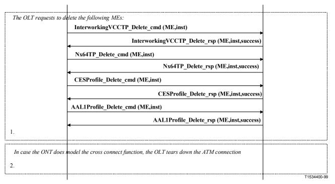
Figure I.19/G.983.2 – Connection tear-down of a structured CES
