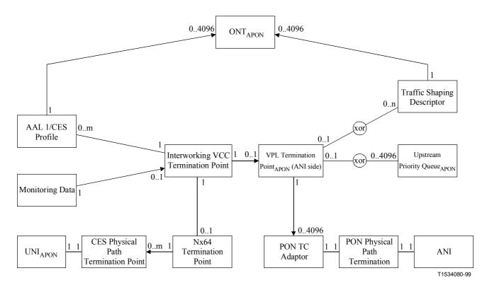
Figure 7/G.983.2 – Managed Entity relation diagram, structured CES service in the ONT that does not model VP Cross-connect function
