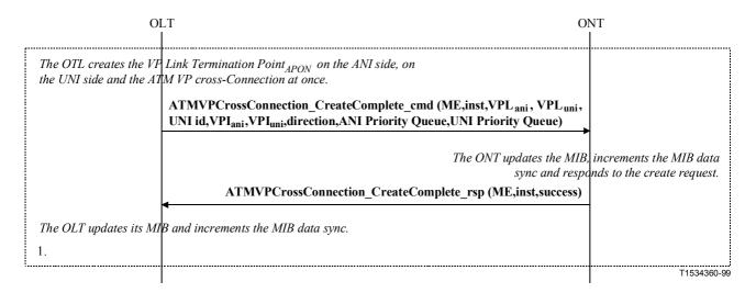
Figure I.15/G.983.2 – VP Cross-Connection set-up (alternative 2)
