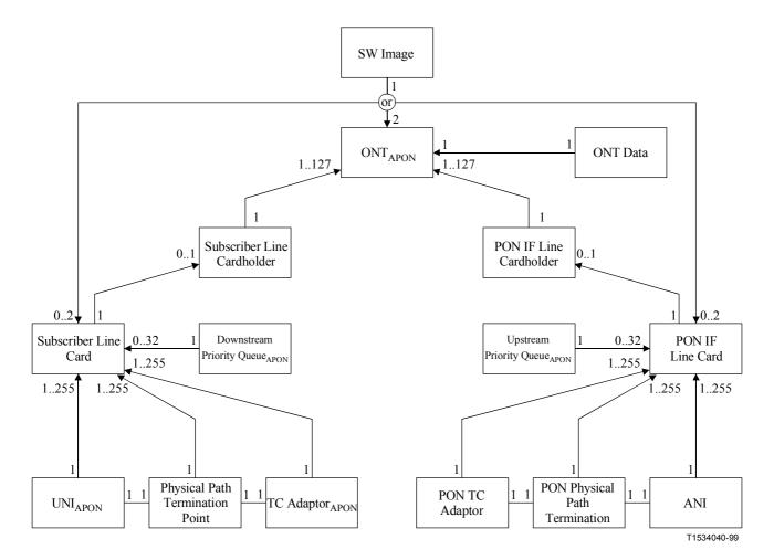
Figure 3/G.983.2 – Managed Entity relation diagram for non-integrated interfaces
