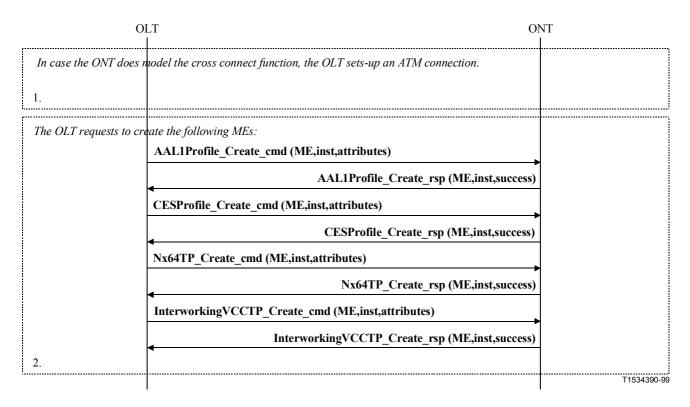
Figure I.18/G.983.2 – Connection set-up of a structured CES
