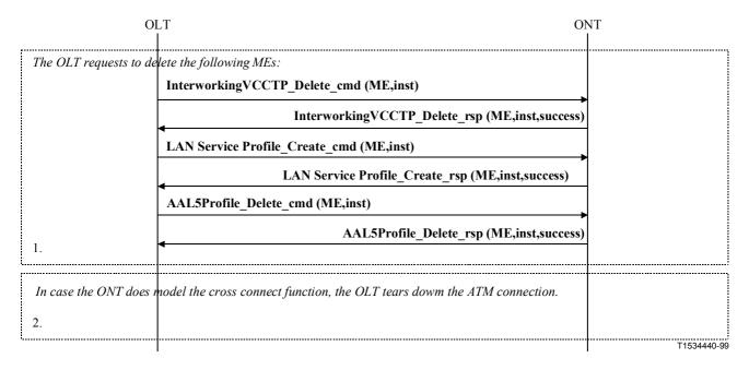
Figure I.23/G.983.2 – Connection tear-down Native LAN connection
