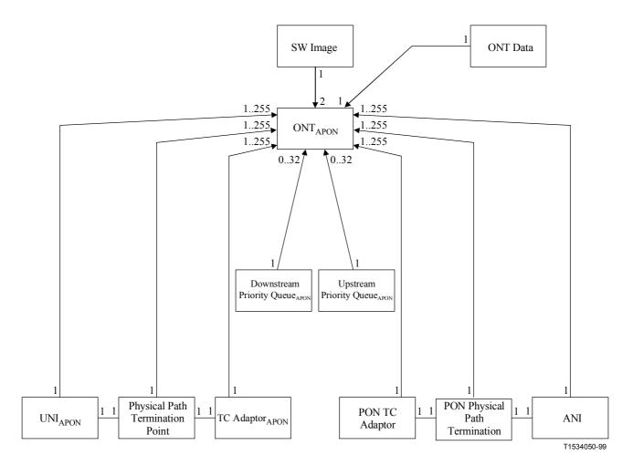
Figure 4/G.983.2 - Managed Entity relation diagram for integrated interfaces
