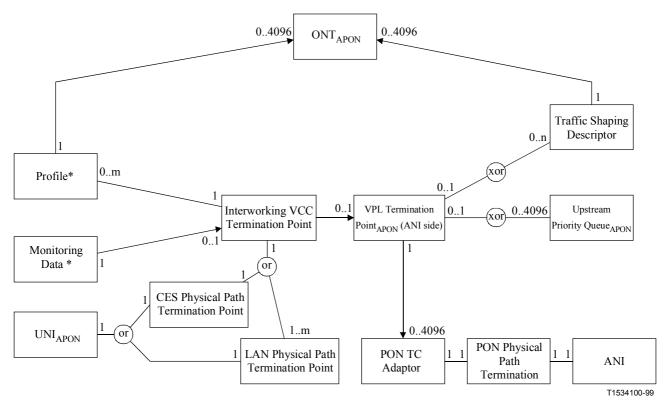
Figure 9/G.983.2 – Managed Entity relation diagram, unstructured CES and LAN service in the ONT that does not model VP Cross-connect function
