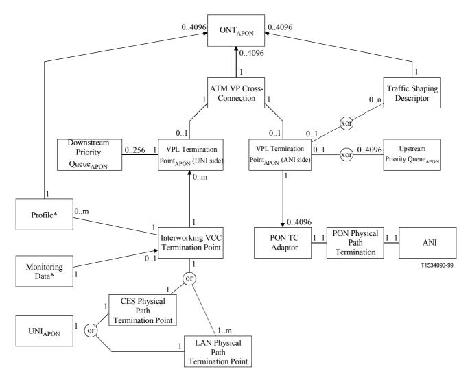
Figure 8/G.983.2 – Managed Entity relation diagram, unstructured CES and LAN service in the ONT that models VP Cross-connect function
