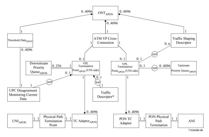
Figure 5/G.983.2 – Managed Entity relation diagram, ATM service
