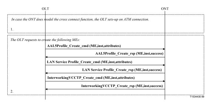
Figure I.22/G.983.2 – Connection set-up Native LAN connection
