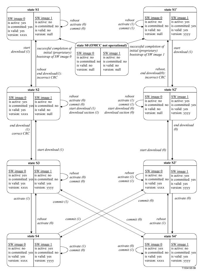
Figure 11/G.983.2 – Software Image State diagram
