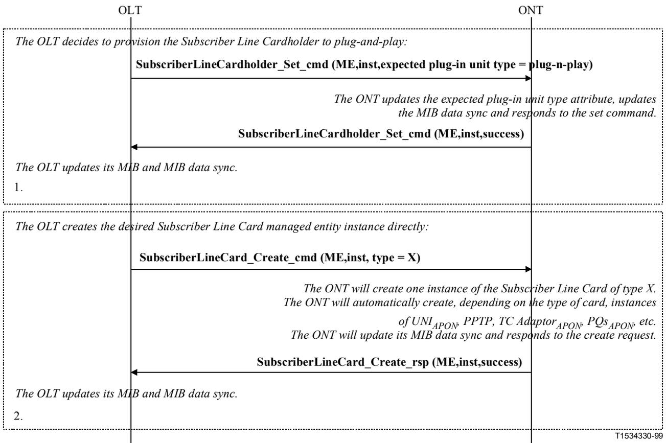
**Figure I.12/G.983.2 – Plug-and-play Subscriber Line Card provisioning**
