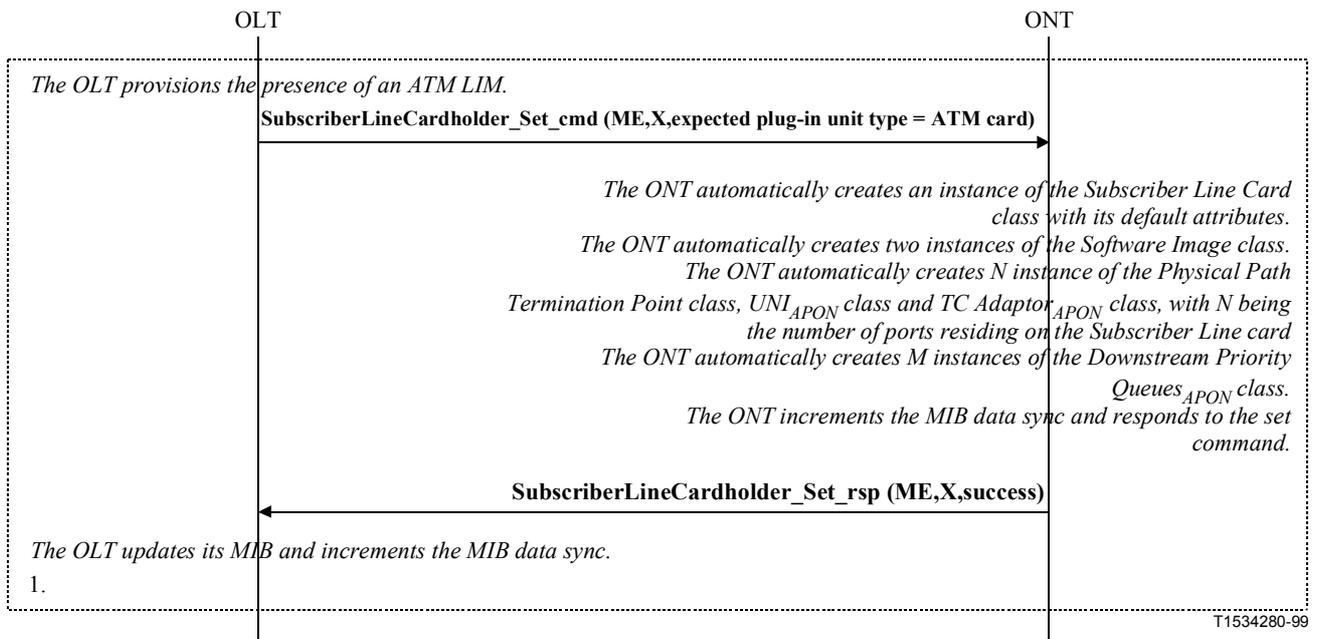
**Figure I.9/G.983.2 – ATM Subscriber Line Card provisioning**
