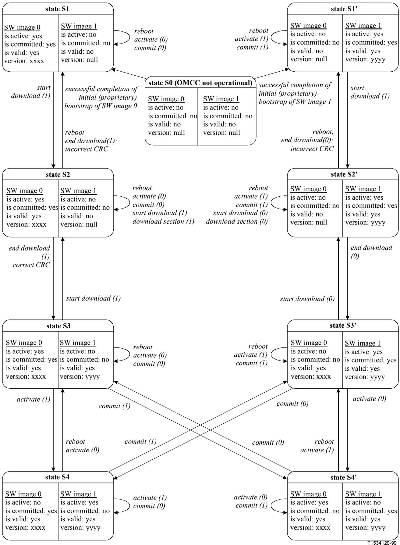
Figure 11/G.983.2 – Software Image State diagram
