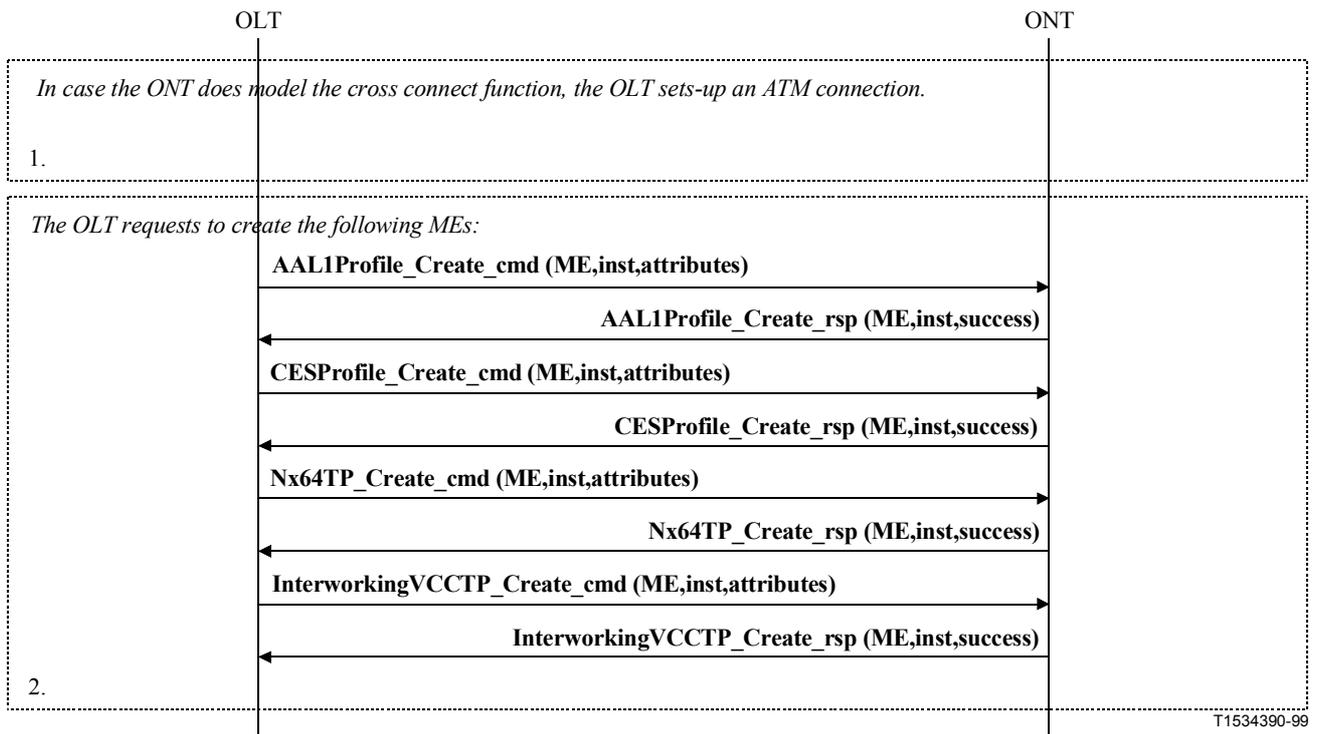
Figure I.18/G.983.2 – Connection set-up of a structured CES
