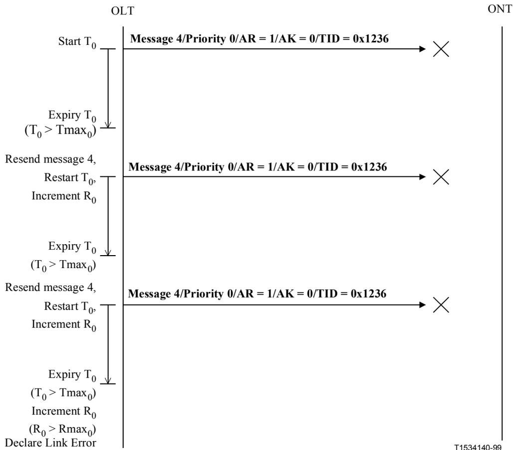
**Figure 15/G.983.2 – OMCC Link Error Detection**
