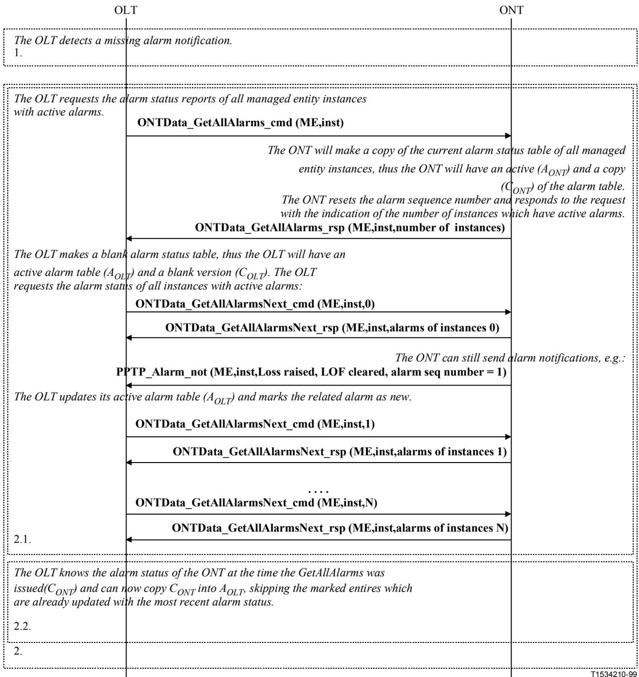
**Figure I.5/G.983.2 – Audit and alarm resynchronization**
