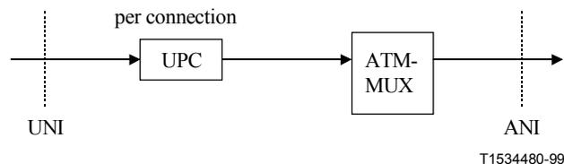
**Figure IV.1/G.983.2 – Policing per connection**
