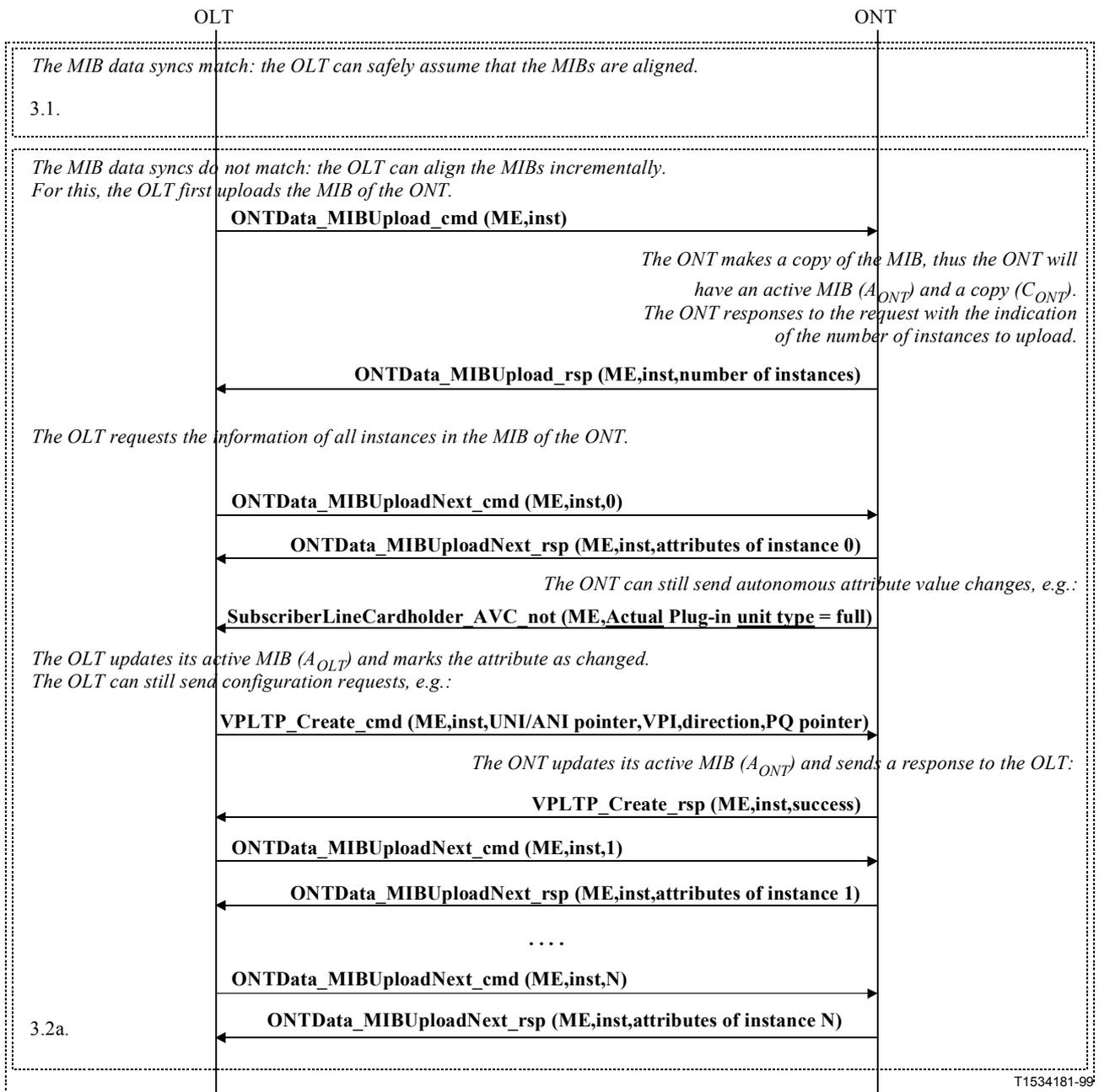
Figure I.3/G.983.2 – Audit and MIB resynchronization
