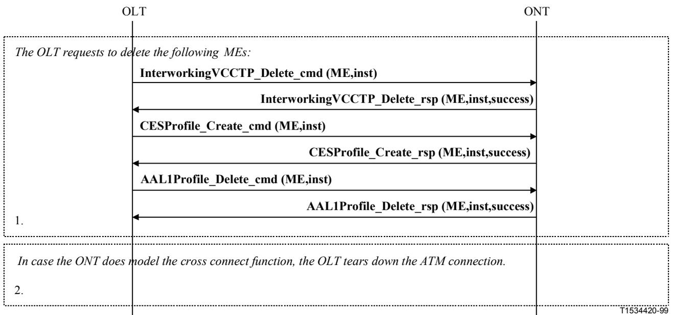
**Figure I.21/G.983.2 – Connection tear-down of an unstructured CES**
