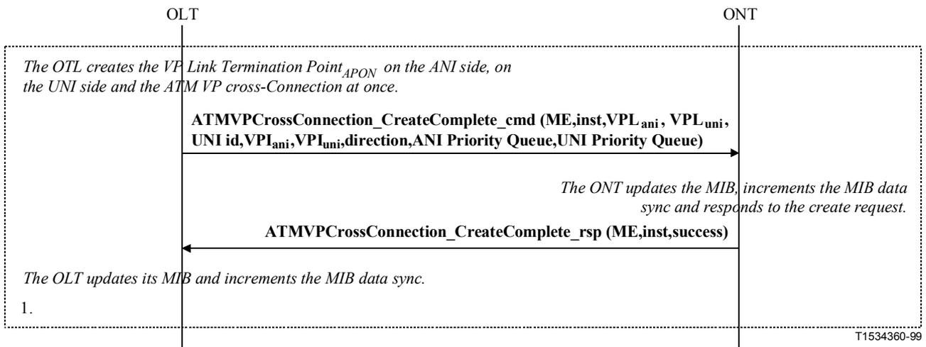
**Figure I.15/G.983.2 – VP Cross-Connection set-up (alternative 2)**
