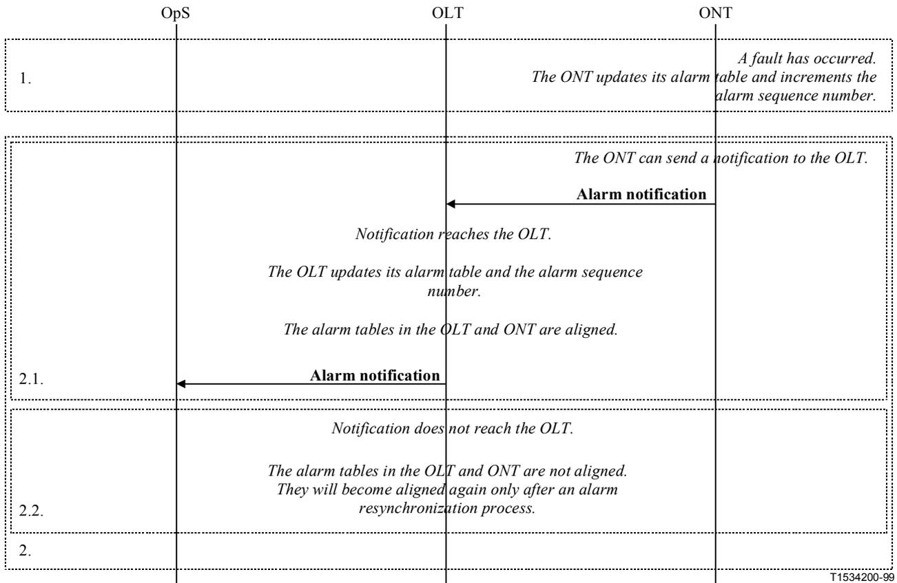
**Figure I.4/G.983.2 – Increment of alarm sequence number at ONT and OLT**
