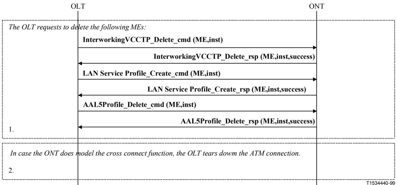
**Figure I.23/G.983.2 – Connection tear-down Native LAN connection**
