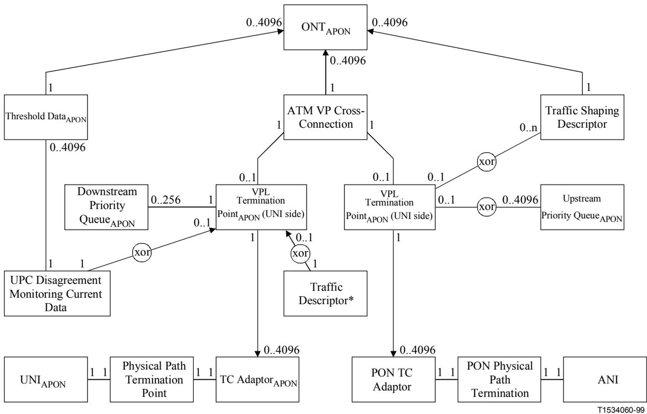
**Figure 5/G.983.2 – Managed Entity relation diagram, ATM service**
