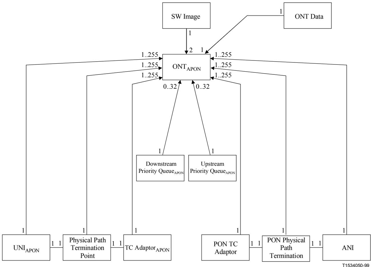
**Figure 4/G.983.2 – Managed Entity relation diagram for integrated interfaces**
