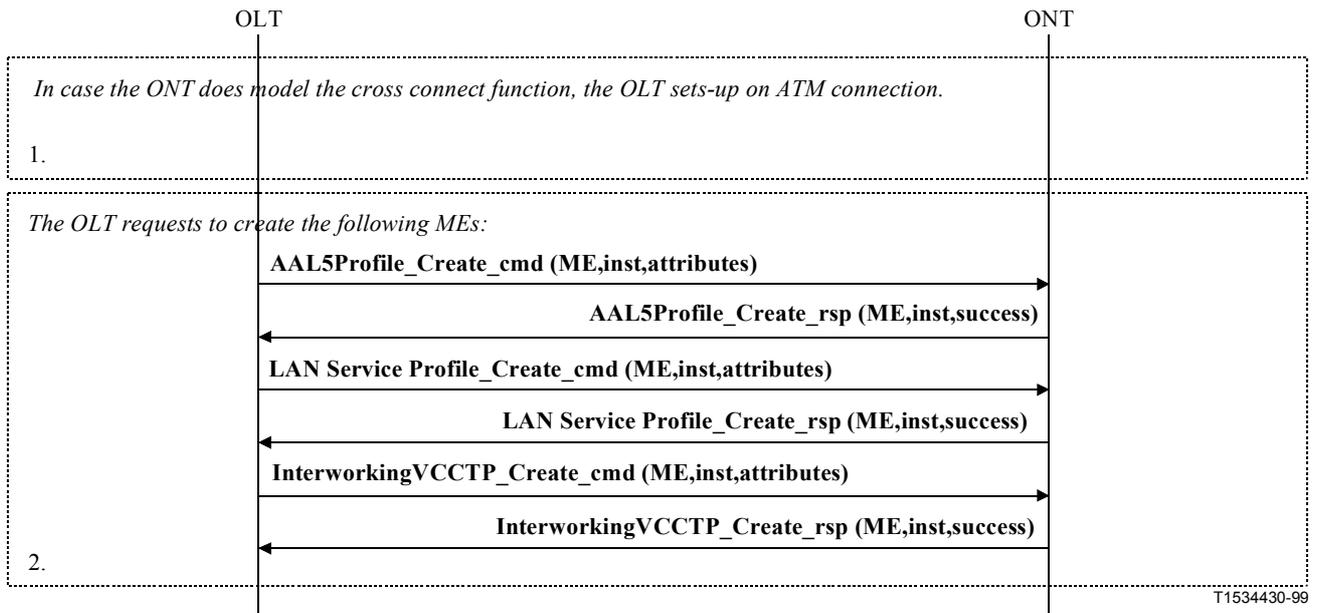
**Figure I.22/G.983.2 – Connection set-up Native LAN connection**
