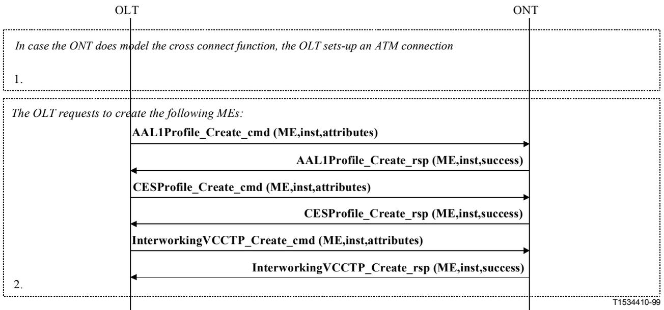
**Figure I.20/G.983.2 – Connection set-up of an unstructured CES**
