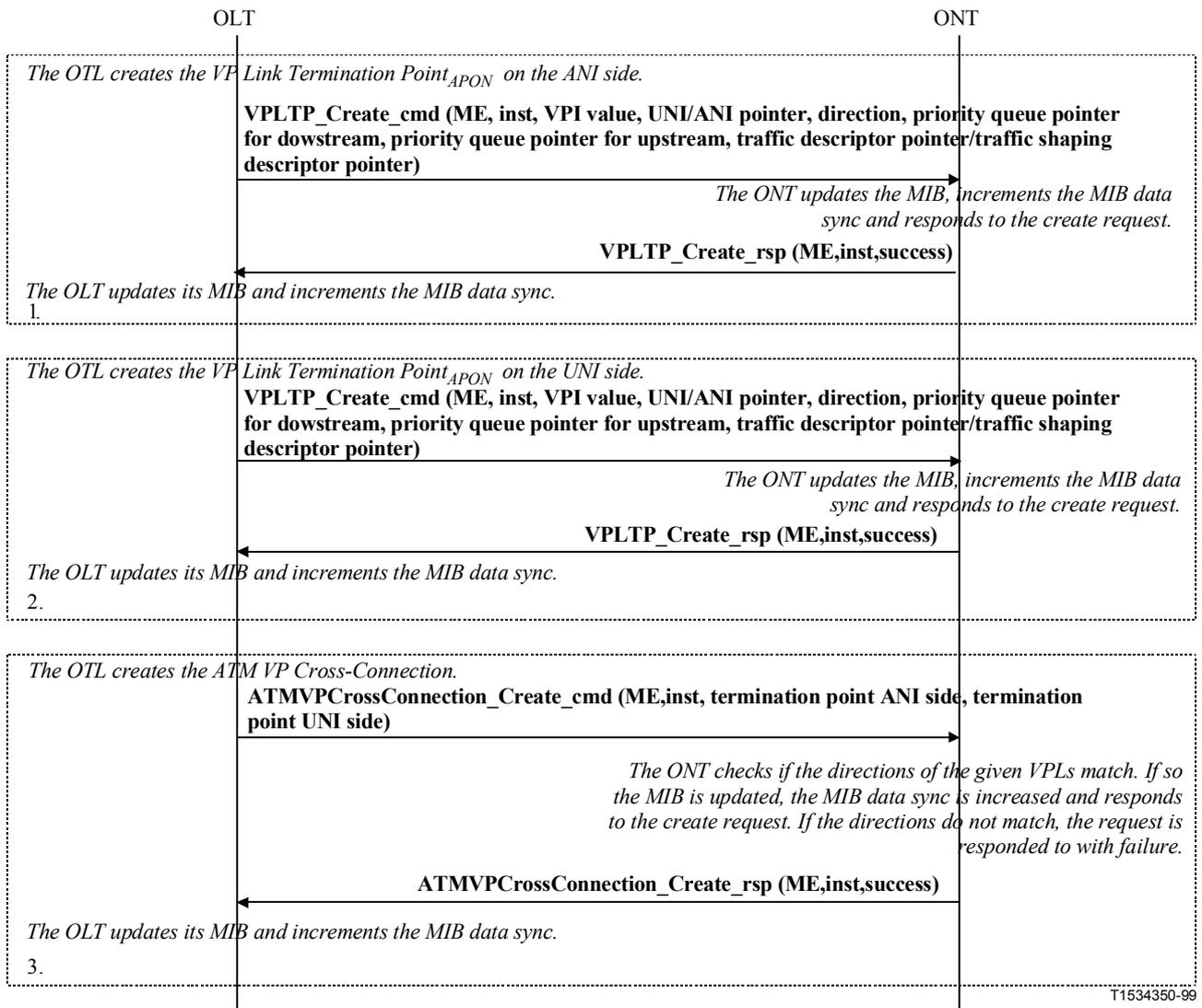
Figure I.14/G.983.2 – VP Cross-Connection set-up (alternative 1)
