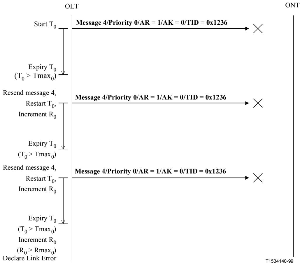
**Figure 15/G.983.2 – OMCC Link Error Detection**
