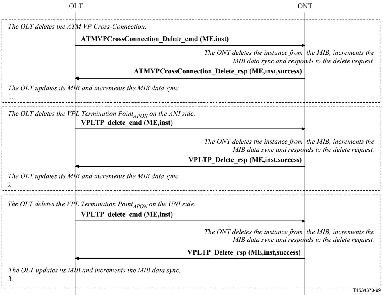
**Figure I.16/G.983.2 – VP Cross-Connection deletion (alternative 1)**
