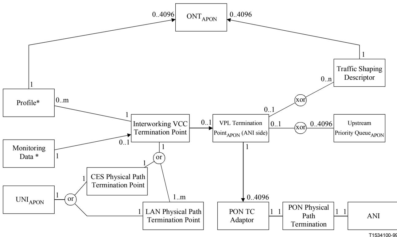
**Figure 9/G.983.2 – Managed Entity relation diagram, unstructured CES and LAN service in the ONT that does not model VP Cross-connect function**
