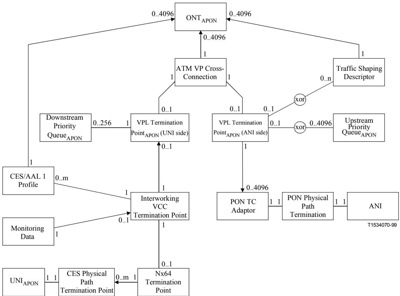
**Figure 6/G.983.2 – Managed Entity relation diagram, structured CES service in the ONT that models VP Cross-connect function**
