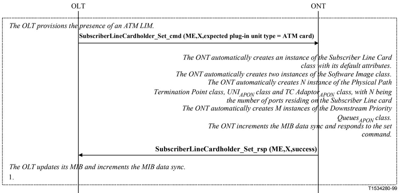
**Figure I.9/G.983.2 – ATM Subscriber Line Card provisioning**
