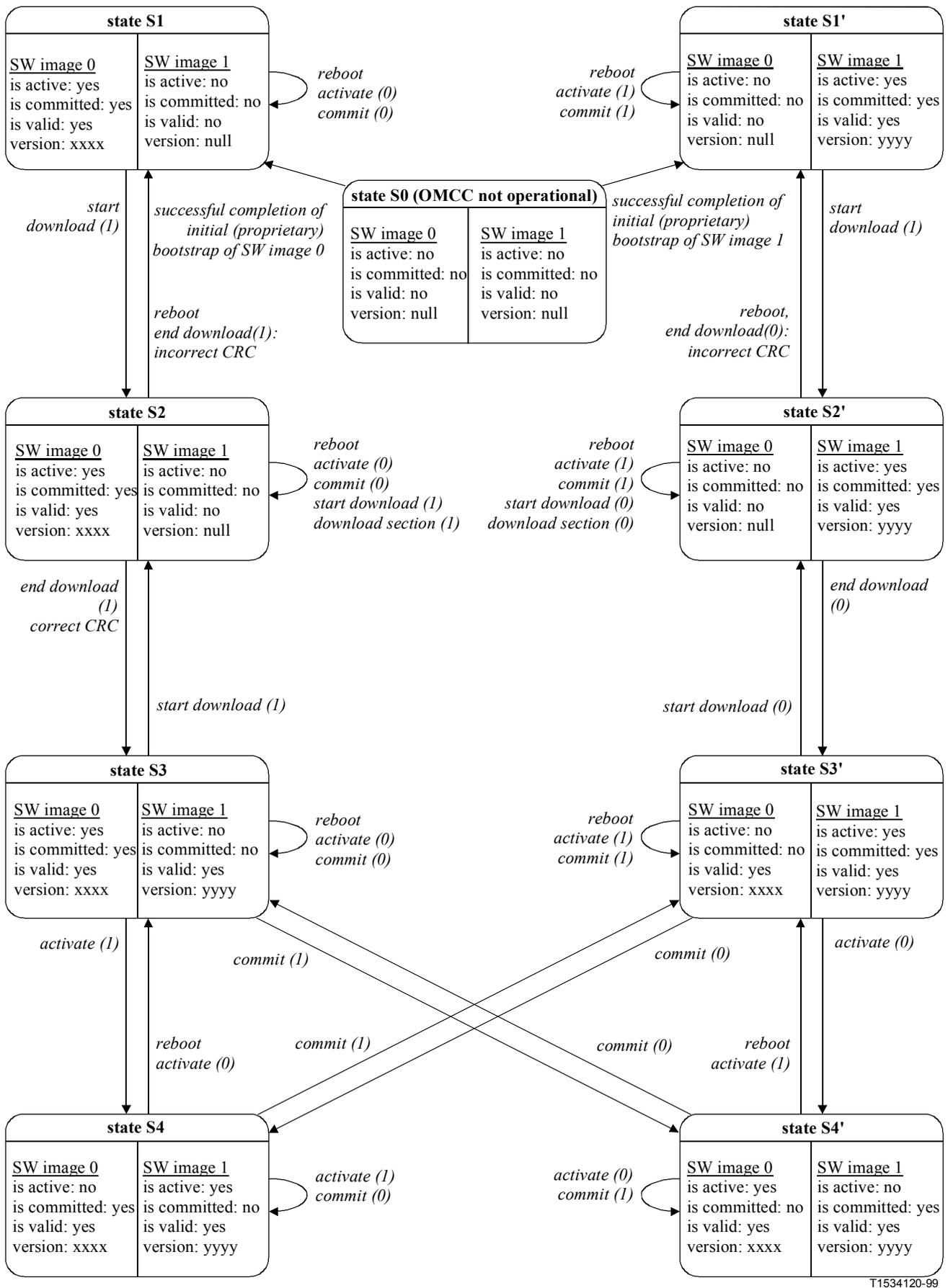
Figure 11/G.983.2 – Software Image State diagram
