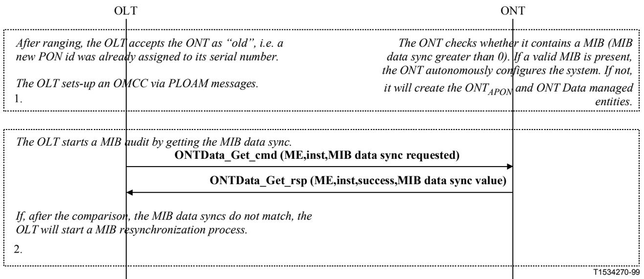
**Figure I.8/G.983.2 – Start-up phase of an "old" ONT**
