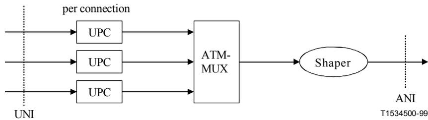
**Figure IV.3/G.983.2 – Policing and shaping per connection or per multiple connections**
