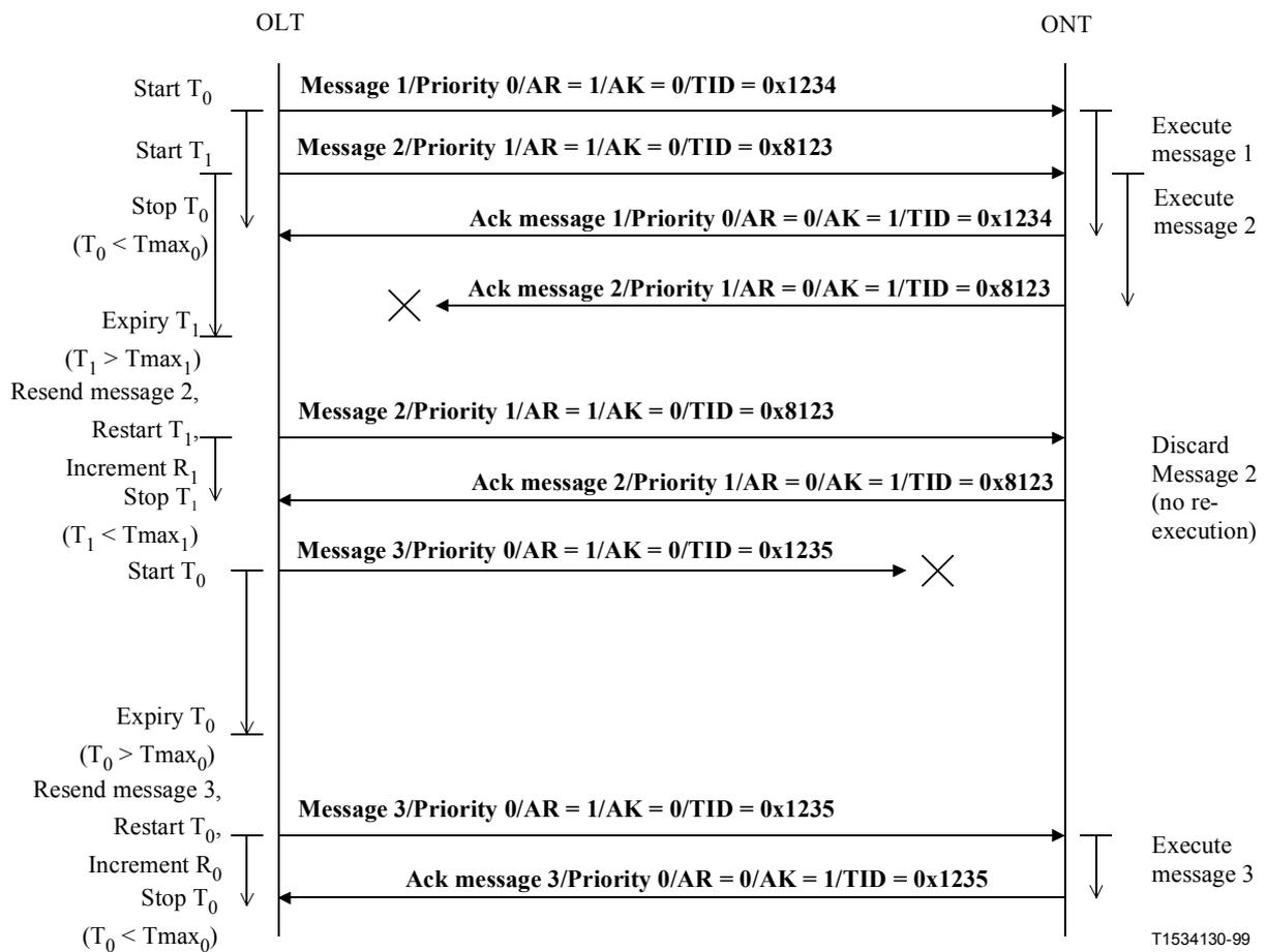
**Figure 14/G.983.2 – Concurrent Message Exchange with Error Recovery**
