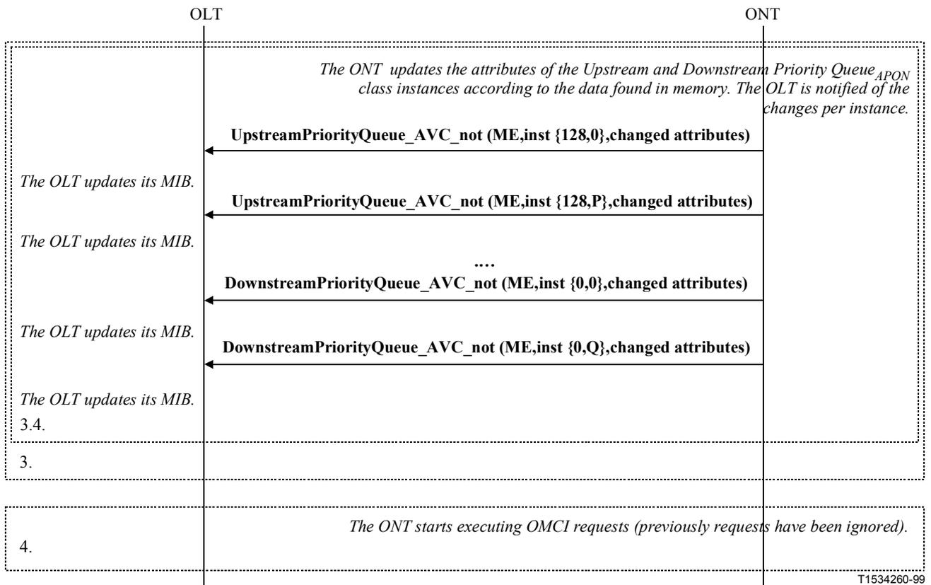
**Figure I.7/G.983.2 – Start-up phase of a "new" ONT with integrated interfaces on both sides (concluded)**
