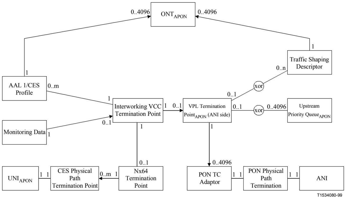
**Figure 7/G.983.2 – Managed Entity relation diagram, structured CES service in the ONT that does not model VP Cross-connect function**
