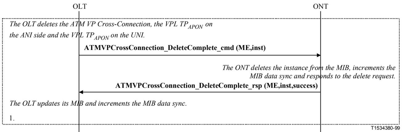
**Figure I.17/G.983.2 – VP Cross-Connection deletion (alternative 2)**
