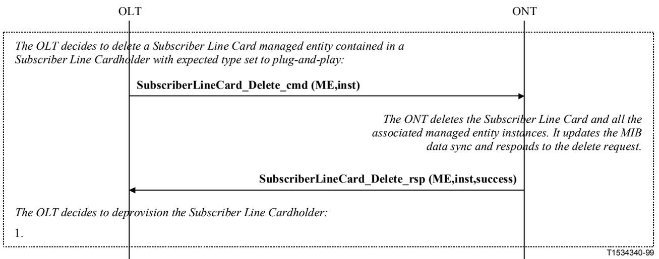
**Figure I.13/G.983.2 – Plug-and-play Subscriber Line Card de-provisioning**
