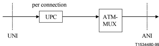
**Figure IV.1/G.983.2 – Policing per connection**
