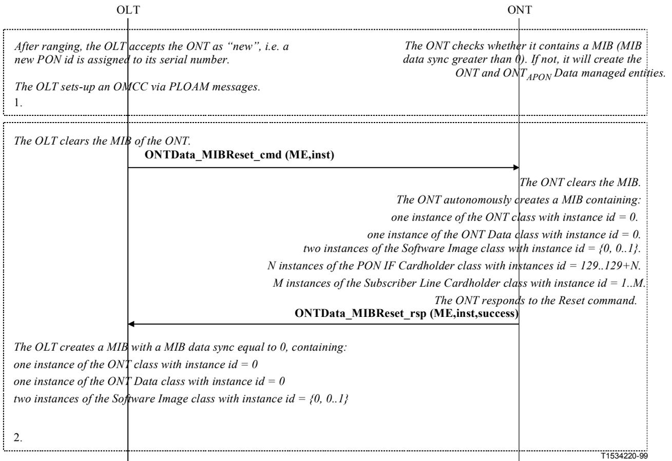
**Figure I.6/G.983.2 – Start-up of a "new" ONT with Cardholders on both sides**
