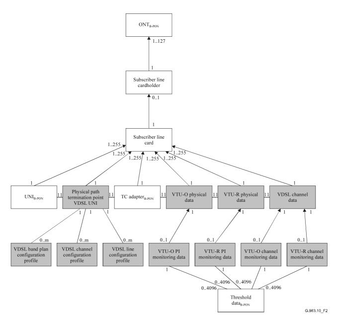
Figure 2/G.983.10 – Managed entity relation diagram for VDSL interfaces
