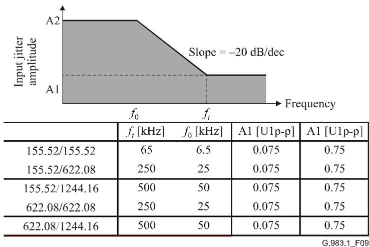
**Figure 9/G.983.1 – Jitter tolerance mask for ONU**
