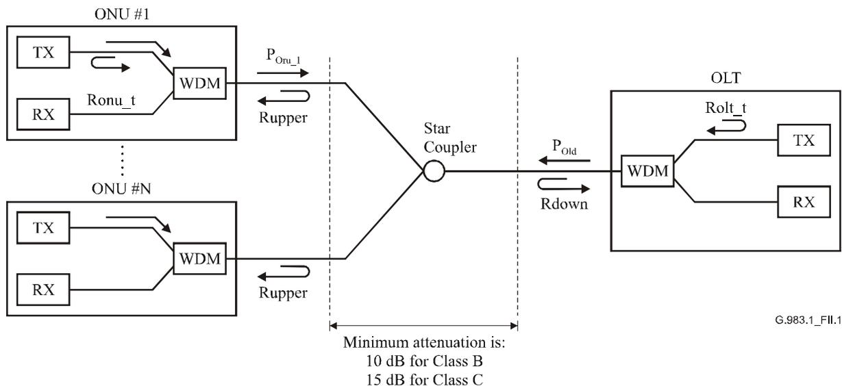
**Figure II.1/G.983.1 – Reflectance model to be considered**
