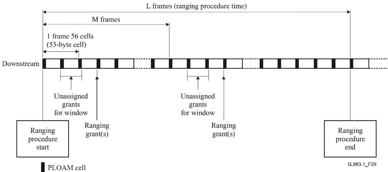
**Figure 29/G.983.1 – Repeated opening of the ranging window**
