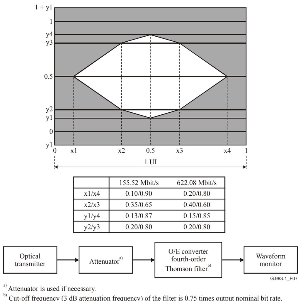
**Figure 7/G.983.1 – Mask of the eye diagram for the upstream transmission signal**
