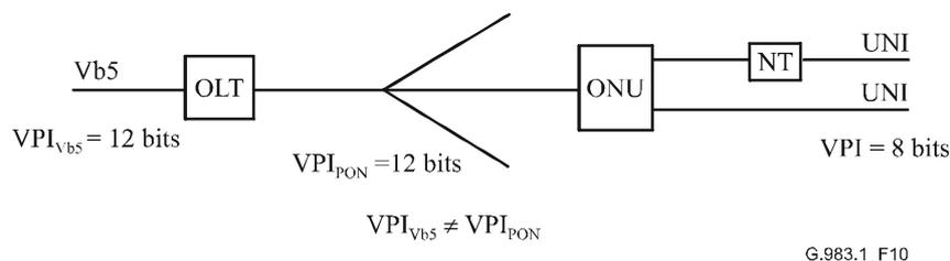
**Figure 10/G.983.1 – VP usage on the PON**
