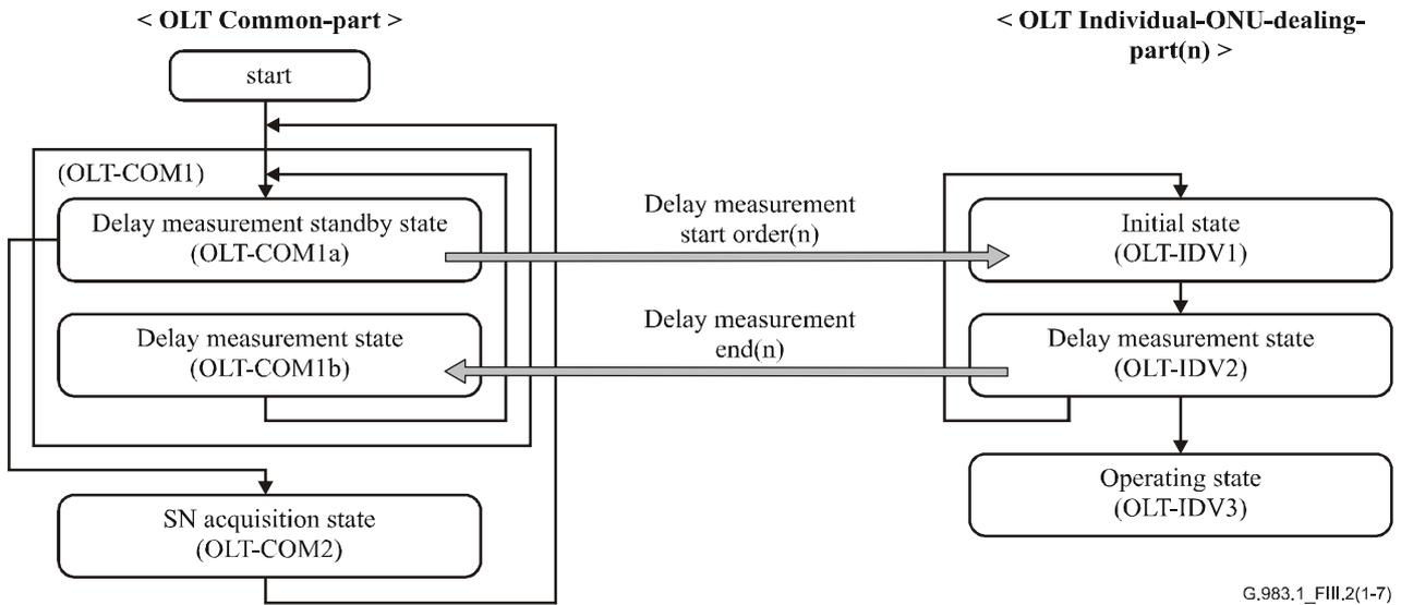
**Figure III.2/G.983.1 – Ranging flow [OLT] (example) (sheet 1 of 7)**
