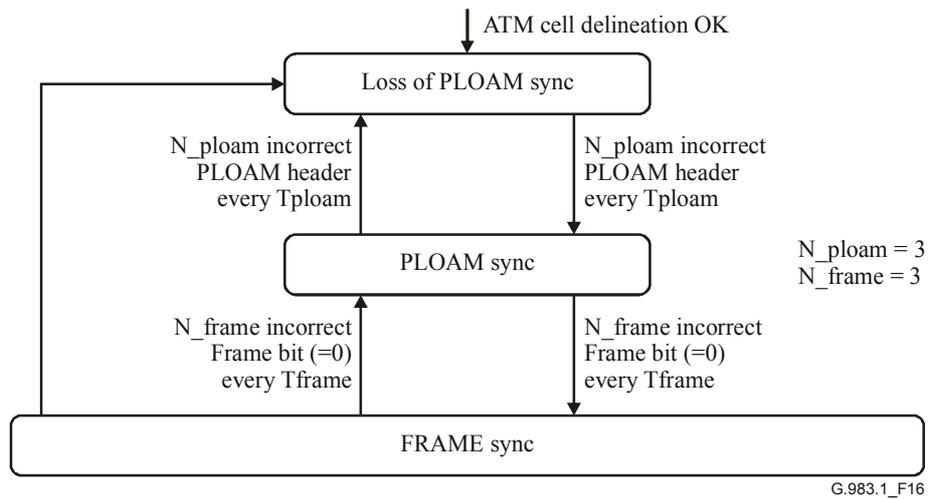
**Figure 16/G.983.1 – Frame synchronization flow**
