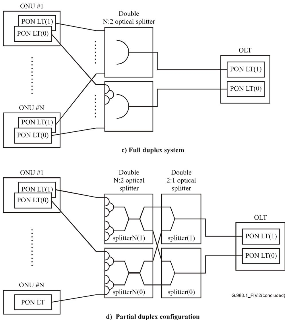
**Figure IV.2/G.983.1 – Duplex ATM-PON system (concluded)**
