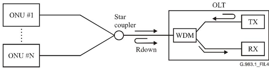
**Figure II.4/G.983.1 – Model 2 incidence into OLT receiver**
