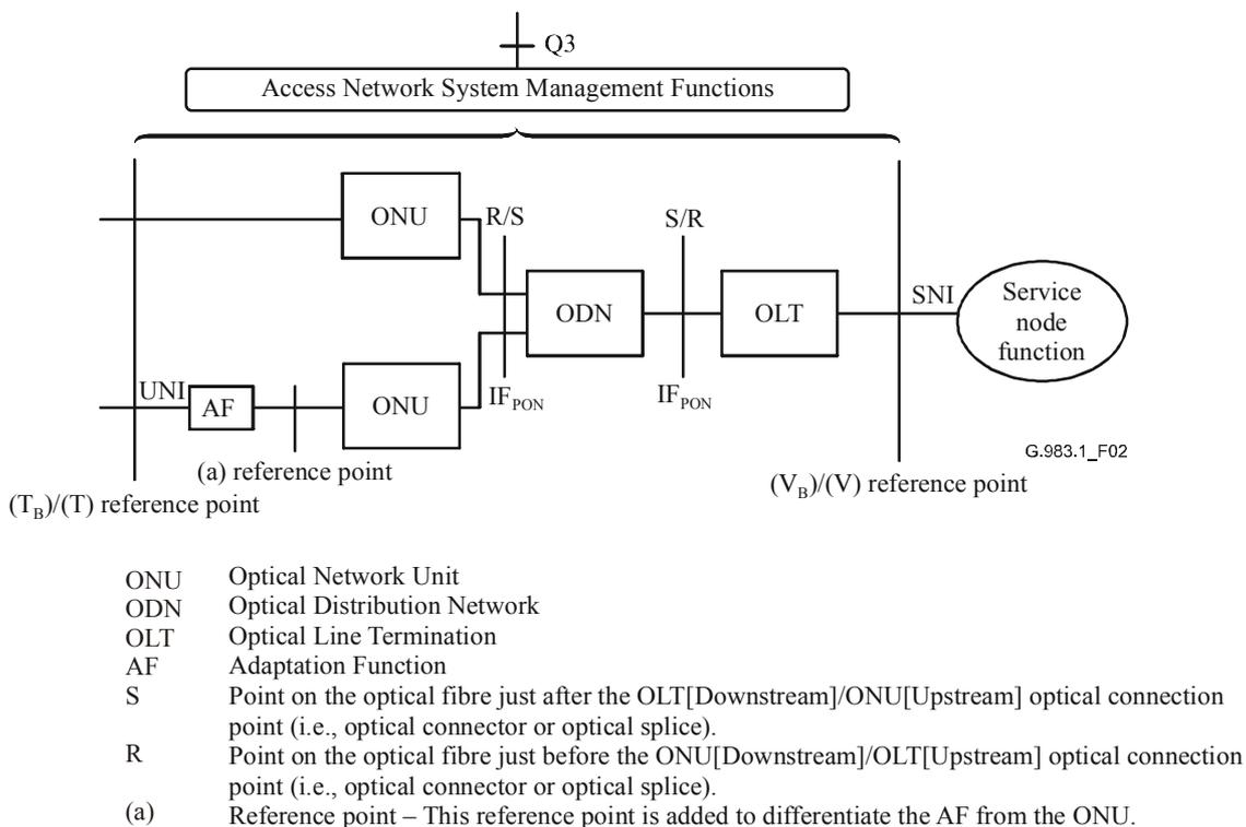
**Figure 2/G.983.1 – Reference configuration for an ATM based PON**
