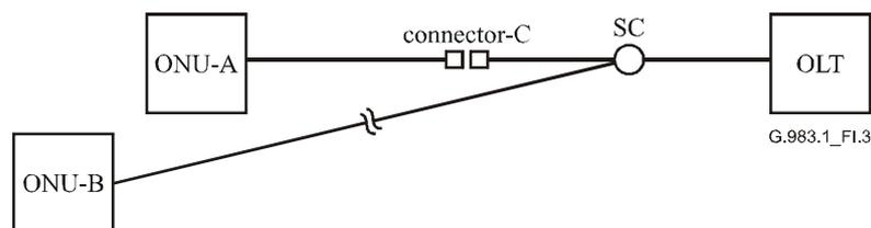
**Figure I.3/G.983.1 – Effect of disconnecting a connector near ONU**
