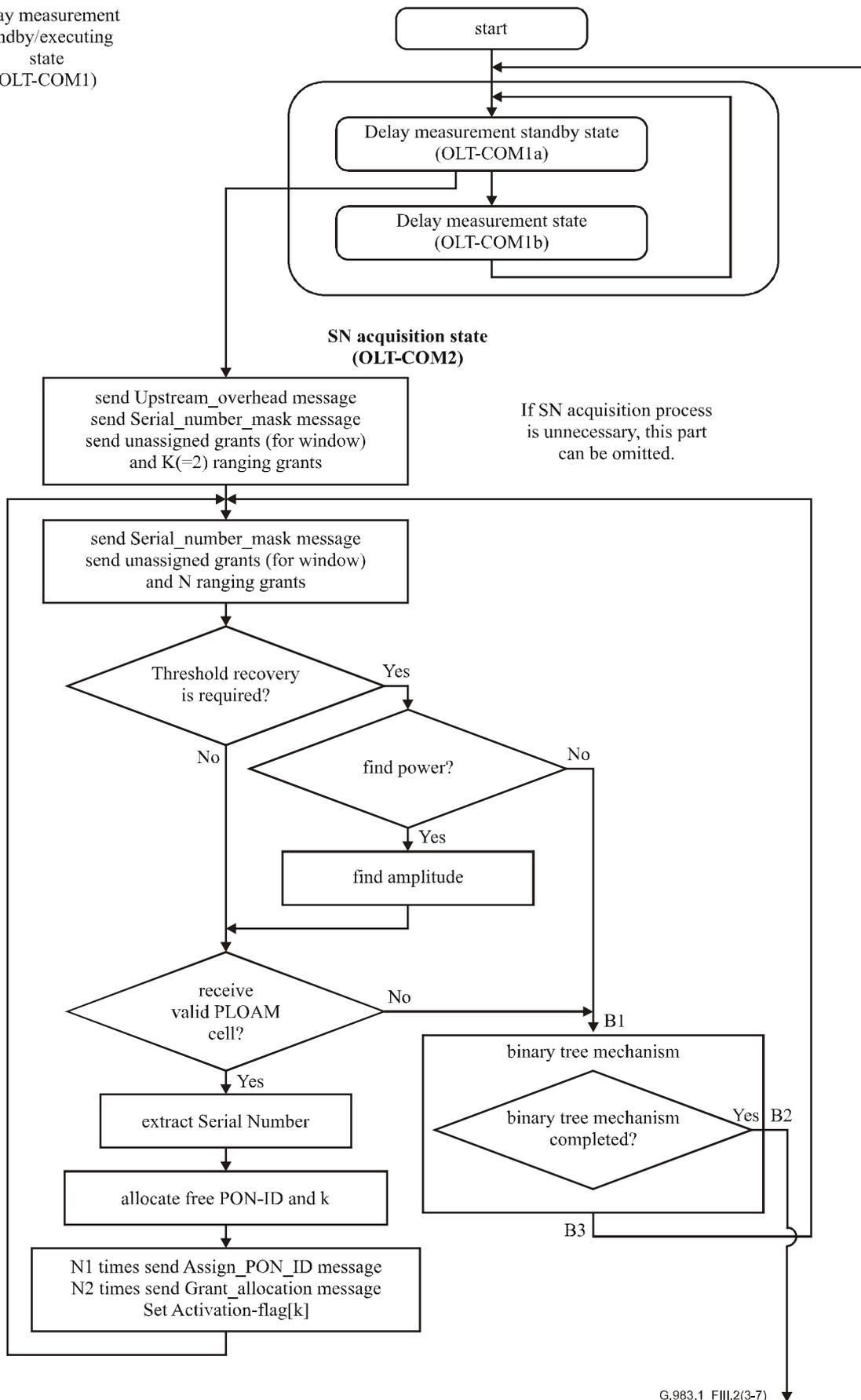
Figure III.2/G.983.1 – Ranging flow [OLT] (example) (sheet 3 of 7)
