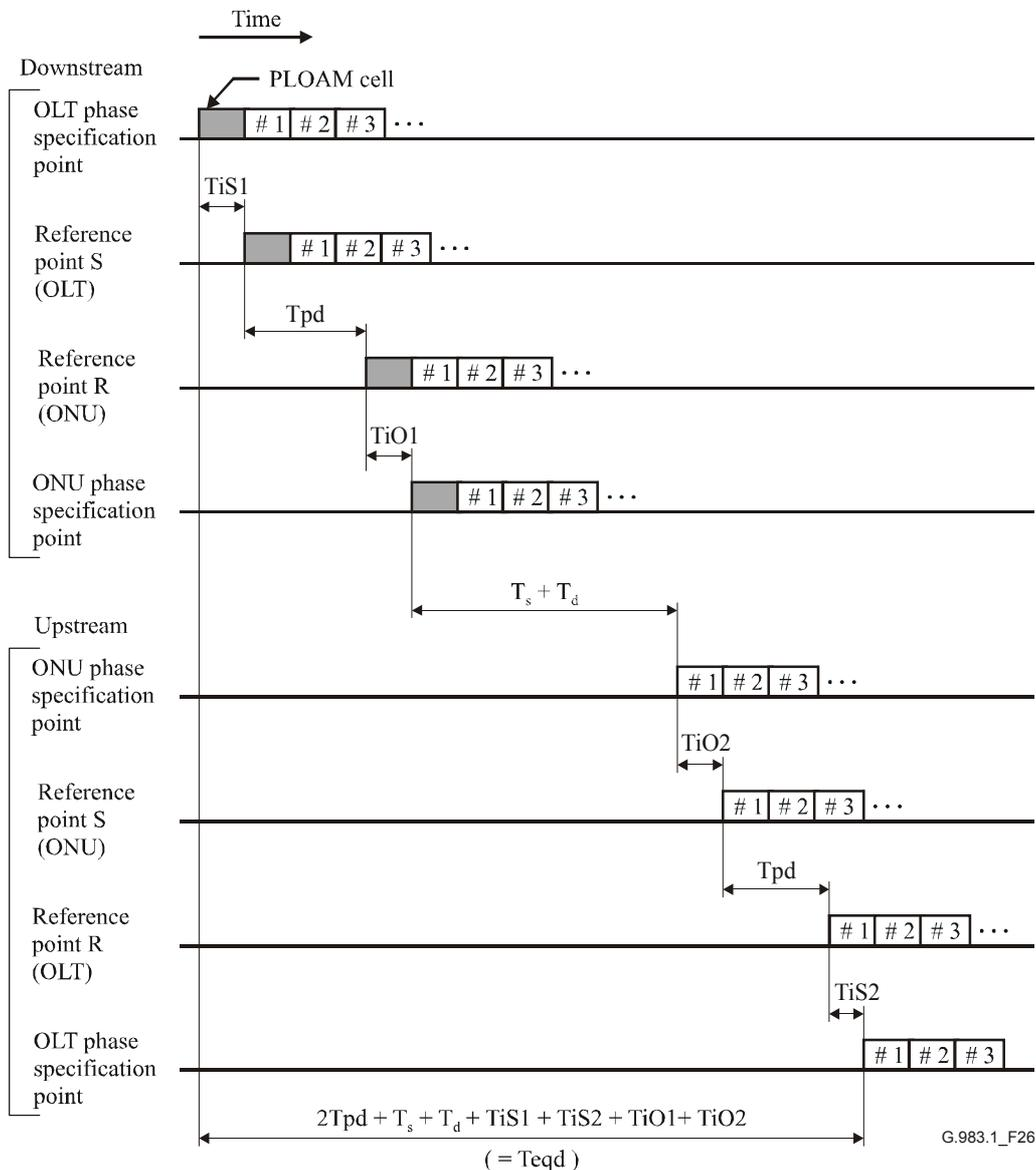
**Figure 26/G.983.1 – Phase relationship between downstream and upstream**
