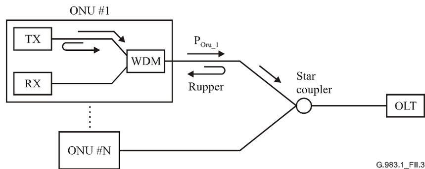
Figure II.3/G.983.1 – Model 1 for incidence into OLT receiver
