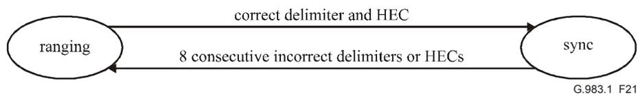
**Figure 21/G.983.1 – Cell delineation state diagram**
