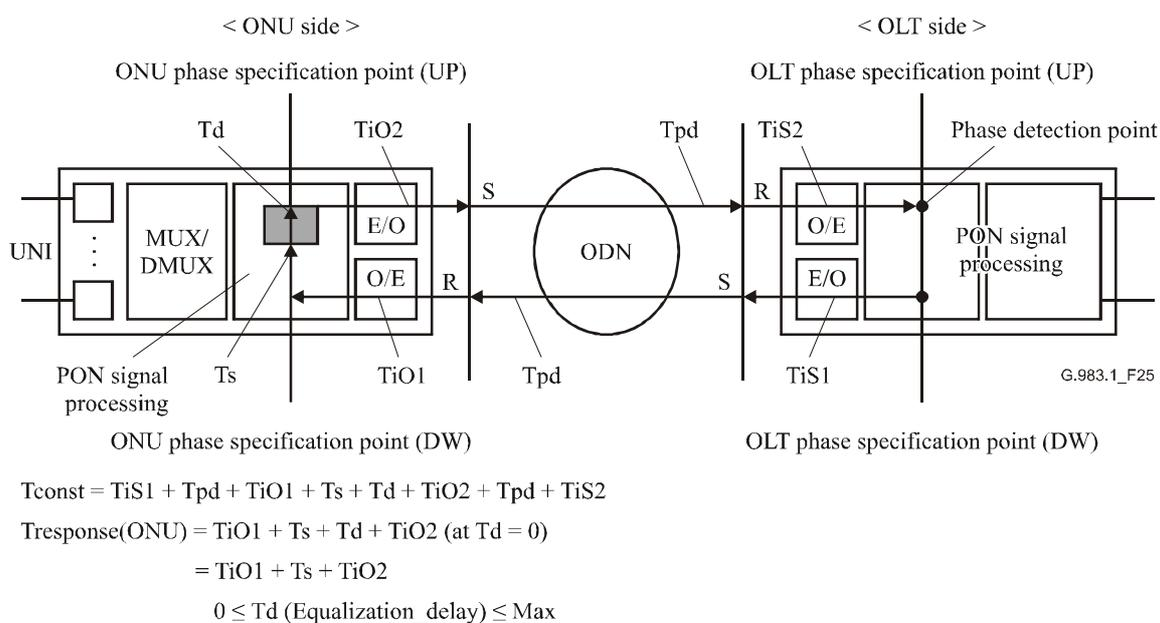
Figure 25/G.983.1 – Configuration of the specification points
