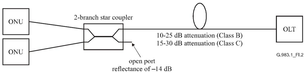
**Figure I.2/G.983.1 – Effect of open connectors located at OLT side of star coupler**
