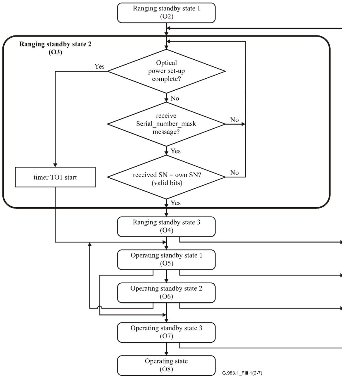
**Figure III.1/G.983.1 – Ranging flow [ONU] (example) (sheet 2 of 7)**
