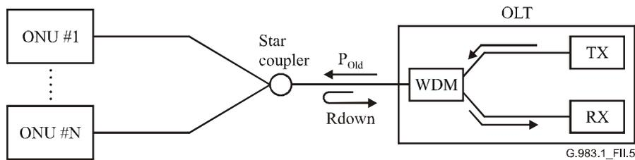
**Figure II.5/G.983.1 – Model 3 for incidence into OLT receiver**
