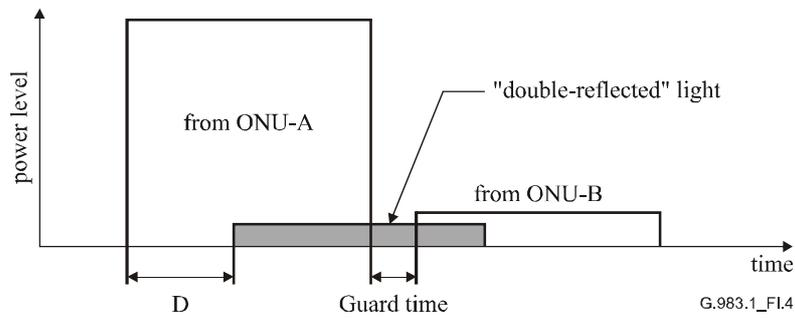
D Round-trip time between ONU-A and connector-C.
