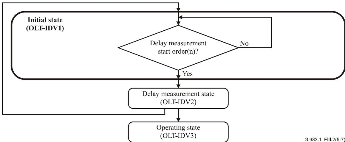
**Figure III.2/G.983.1 – Ranging flow [OLT] (example) (sheet 5 of 7)**
