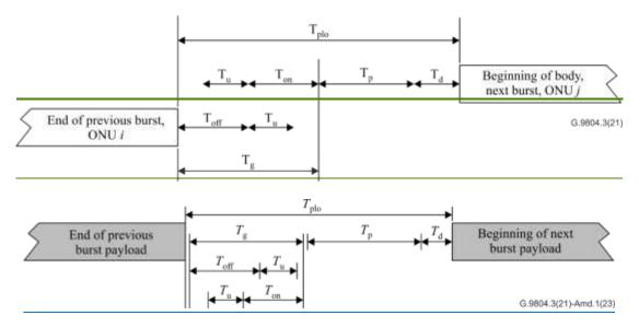
Figure III.1 – Timing relationship- between the various physical layer overhead times
