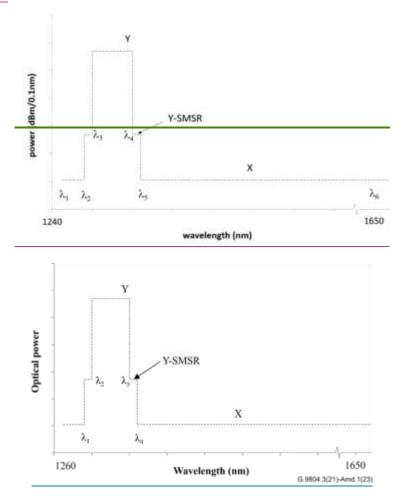
Figure 9-1a – ONU transmitter OOB-PSD mask definition
