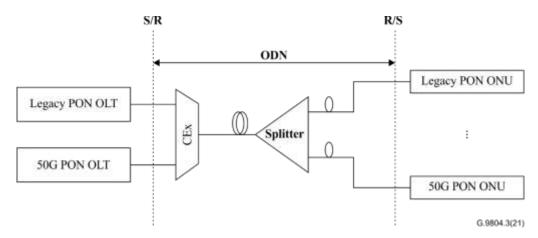
Figure 6-2 – General architectural reference diagram of 50G-PON coexisting with legacy PON using the external CEx method
