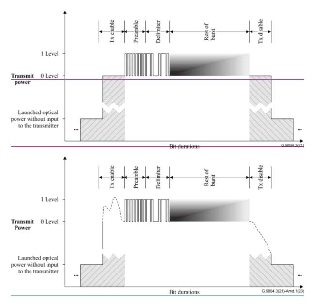
Figure 9-2 – Relationship between ONU power levels and burst times
