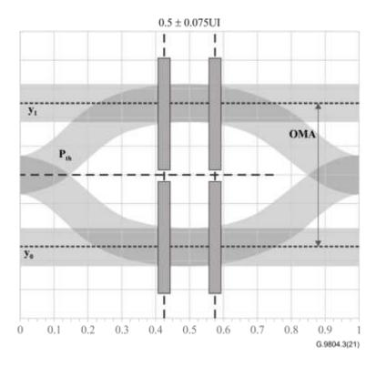
Figure 9-9 - Illustration of the TDEC measurement
