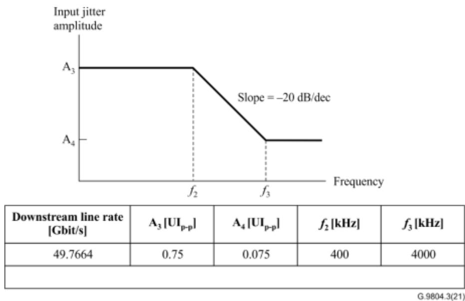
**Figure 9-11 – Sinusoidal jitter mask for jitter transfer evaluation**
