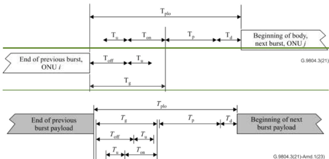
**Figure III.1 – Timing relationship between the various physical layer overhead times**
