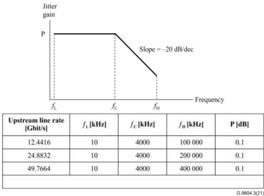
**Figure 9-10 – Jitter transfer mask for ONU**
