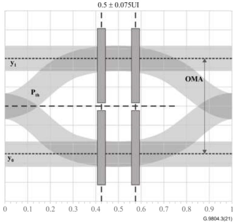
**Figure 9-9 – Illustration of the TDEC measurement**
