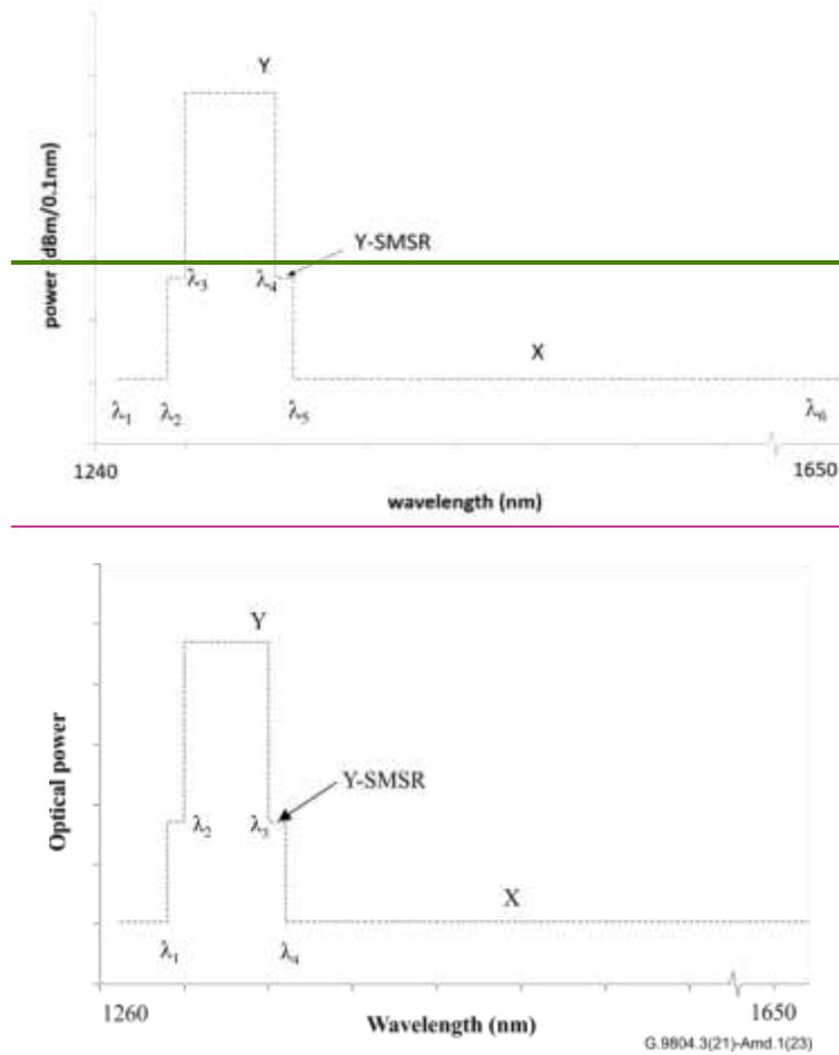
**Figure 9-1a – ONU transmitter OOB-PSD mask definition**
