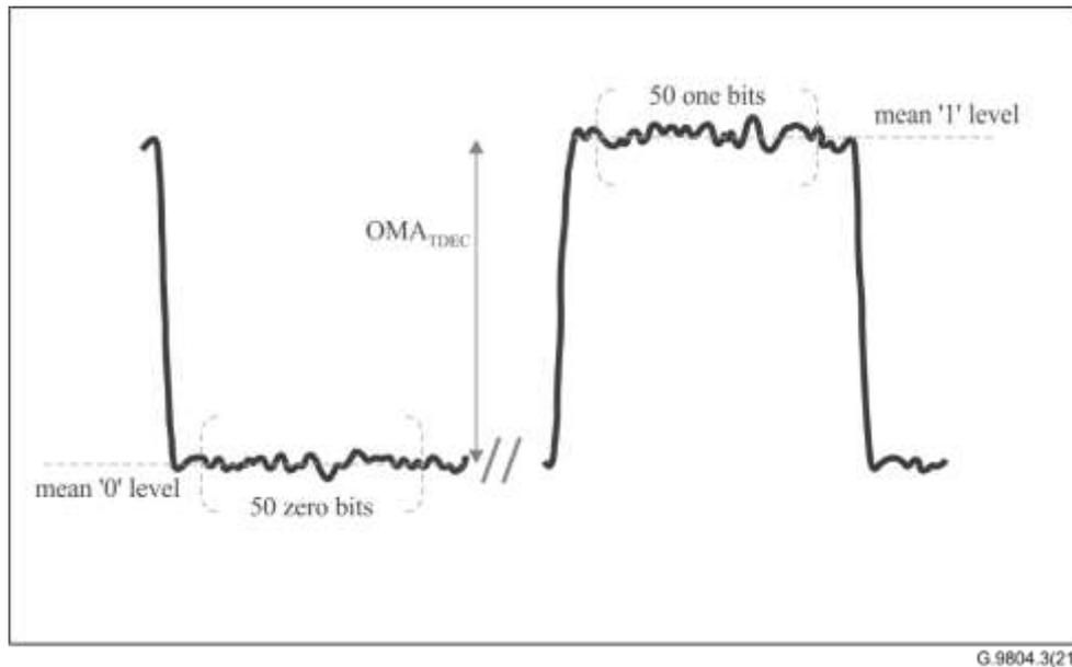
**Figure 9-8 – Illustration of the OMA measurement**
