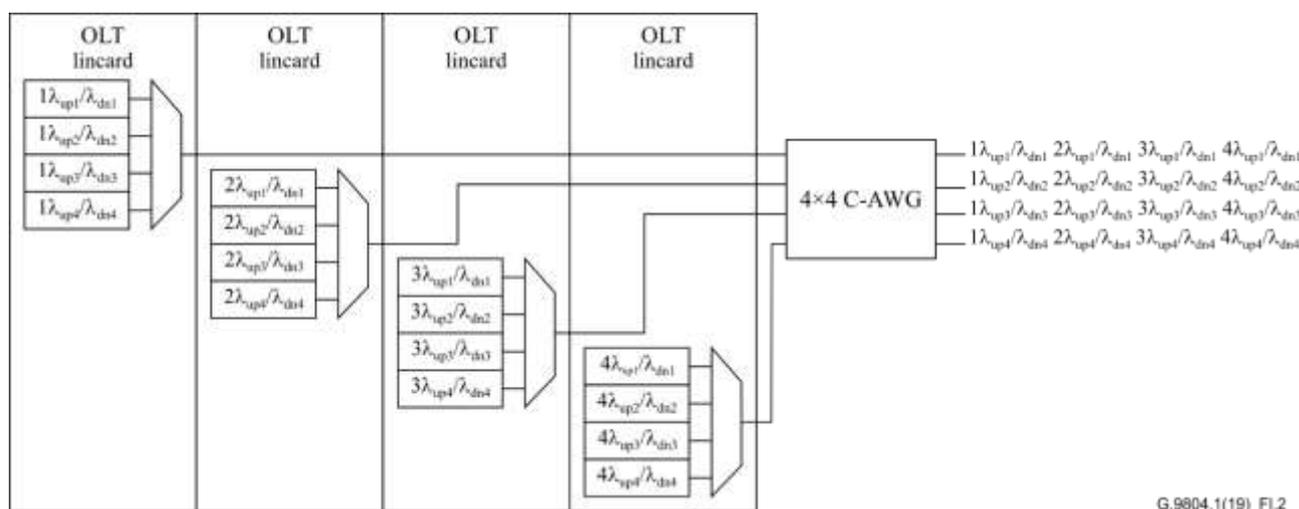
**Figure I.2 – OLT resilience configuration with integrated port design**
