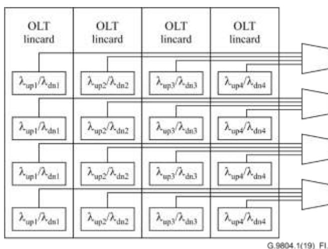
**Figure I.1 – OLT resilience configuration with individual port design**
