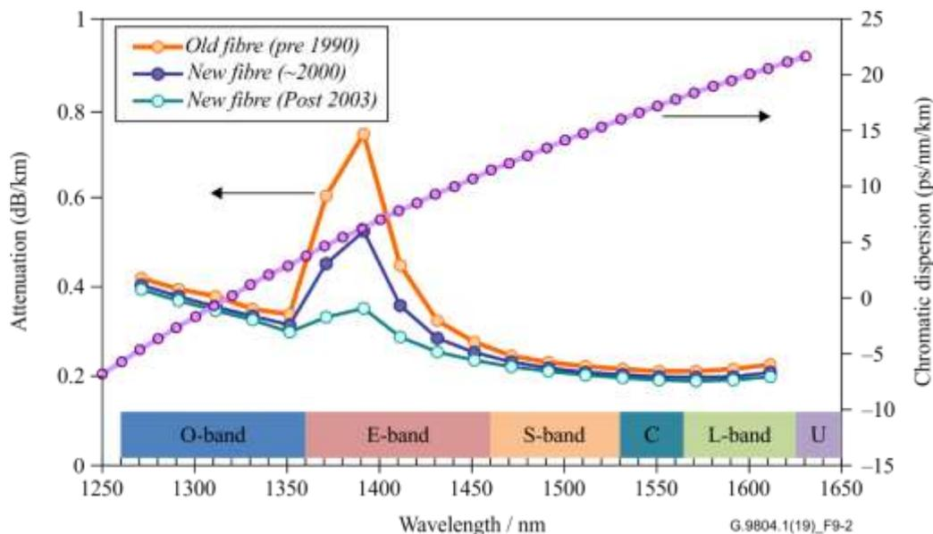
Figure 9-2 – Single mode fibre attenuation and chromatic dispersion
