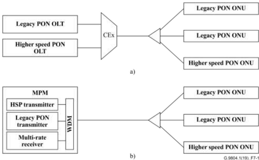
**Figure 7-1 – ODN co-existence scenario (a) with CEx device,
