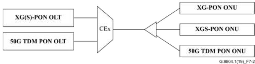
**Figure 7-2 – Coexistence of XG(S)-PON and 50G TDM PON by independent CEx device**
