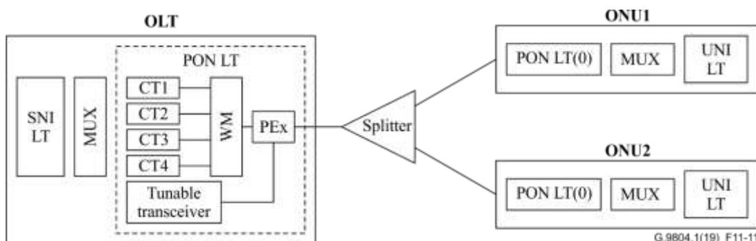
**Figure 11-11 – Type W protection – (n+1):n model**
