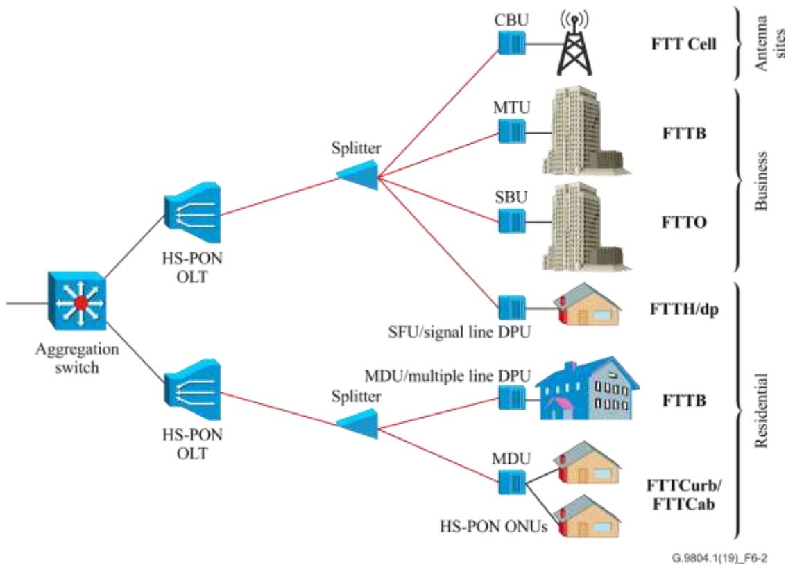
**Figure 6-2 – Deployment scenarios of higher speed PON**
