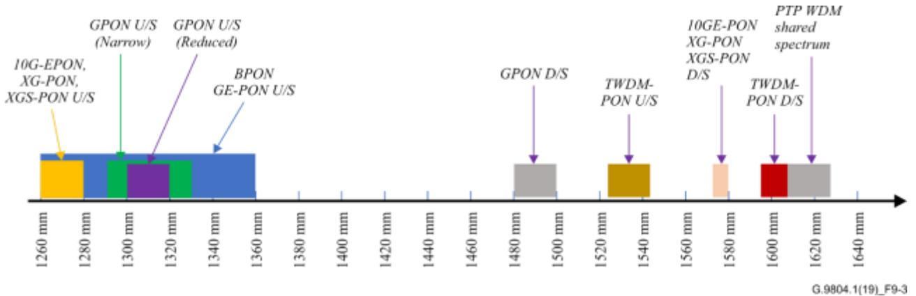
**Figure 9-3 – Wavelength plans of legacy PON systems**
