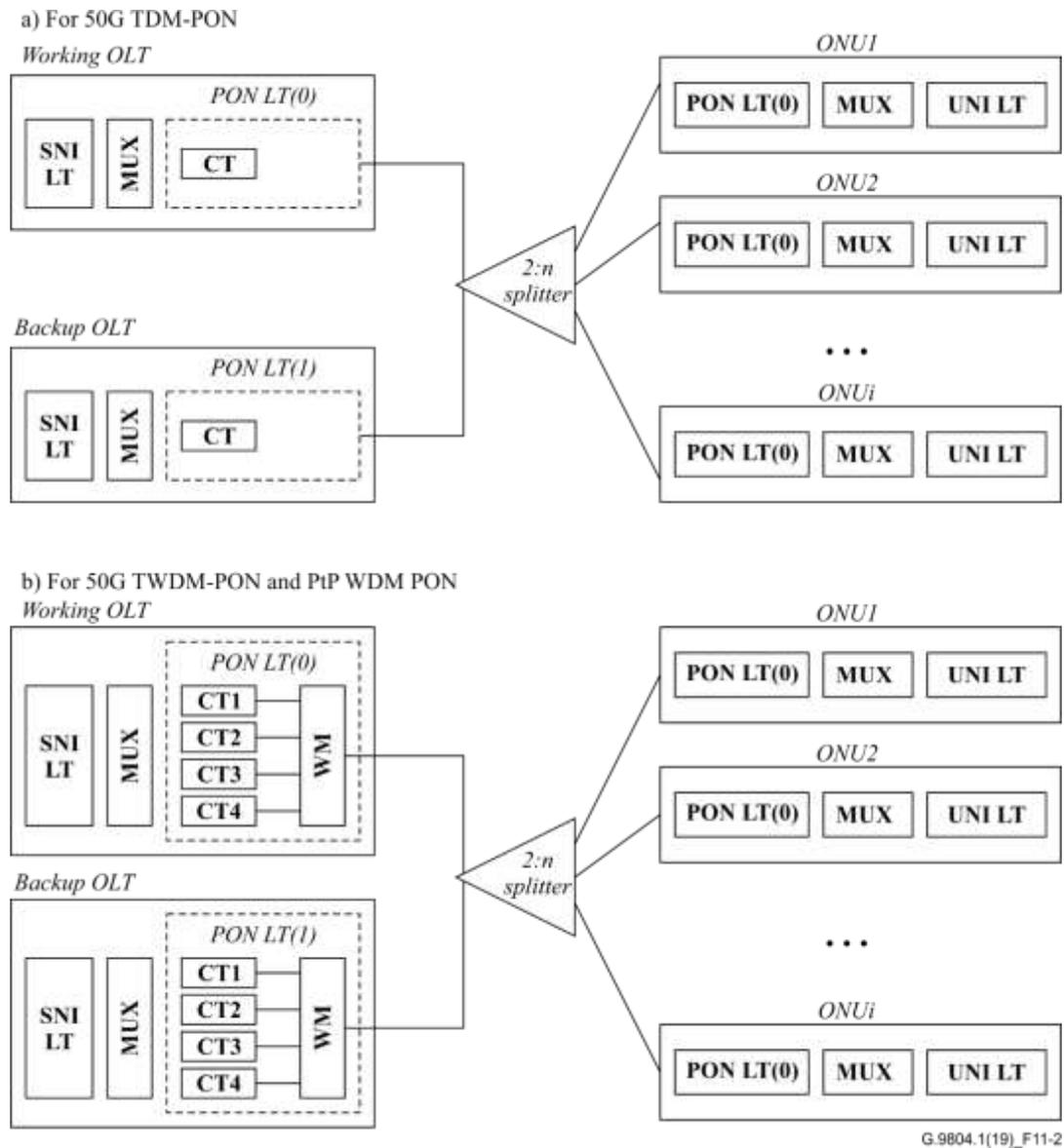
**Figure 11-2 – Type B protection – 1:1 model with dual parenting**
