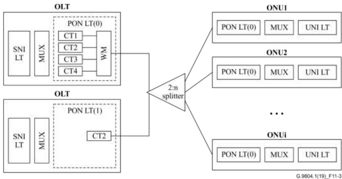
**Figure 11-3 – Type B protection – 1:1 model with single backup CT**
