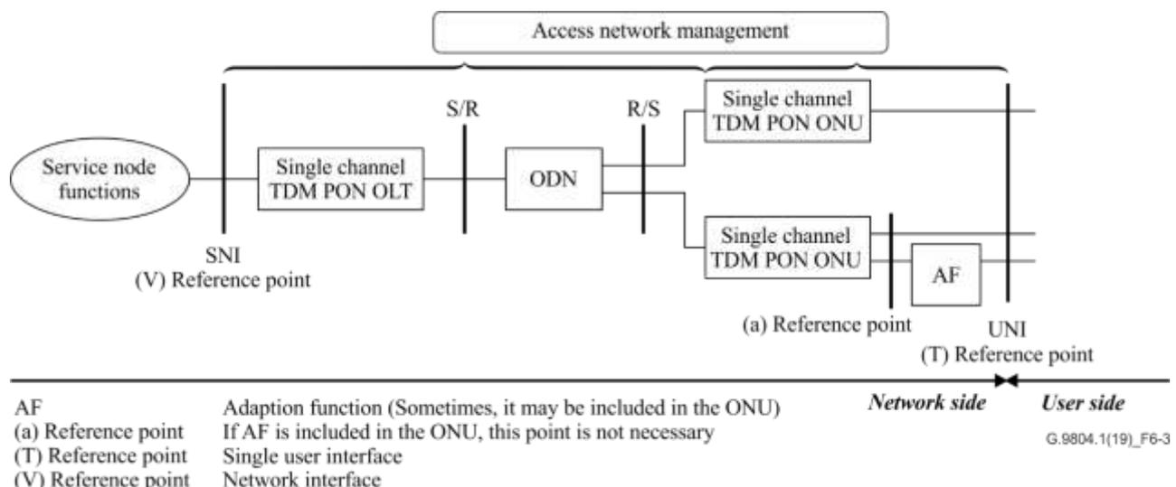
**Figure 6-3 – High-level reference configuration of single channel TDM PON**
