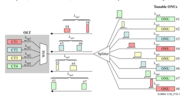
Figure 10-1 – Example of TWDM PON OLT-port sleep mode (before starting sleep mode)
