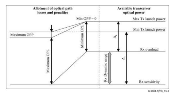
Figure 5-3 – Relationship between optical power and loss parameters
