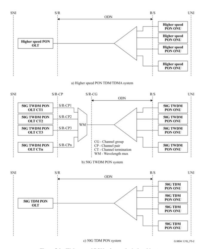
Figure 5-2 – Higher speed PON reference logical architecture
