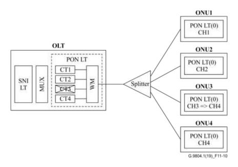
Figure 11-10 – Type W protection – 1:n model with all active OLT CTs
