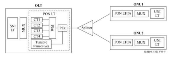
Figure 11-11 – Type W protection – (n+1):n model
