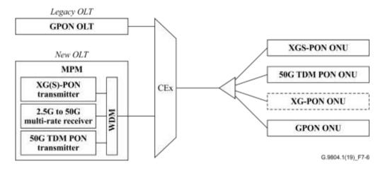
Figure 7-6 – Co-existence scenario of three generation PON systems by mixing WDM and multi-rate receiver
