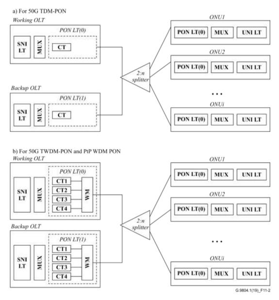
Figure 11-2 – Type B protection – 1:1 model with dual parenting
