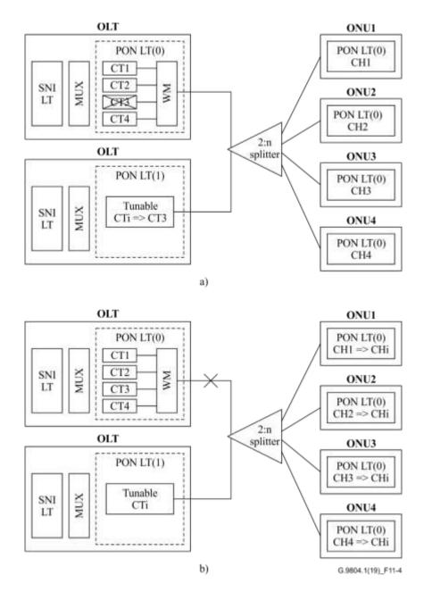
Figure 11-4 – Type B protection – 1:n model (a) CT failure, (b) feeder fibre failure
