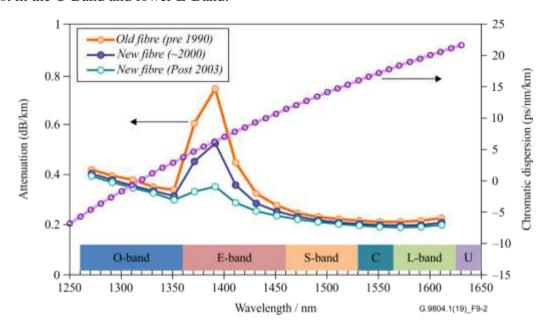
Figure 9-2 – Single mode fibre attenuation and chromatic dispersion
