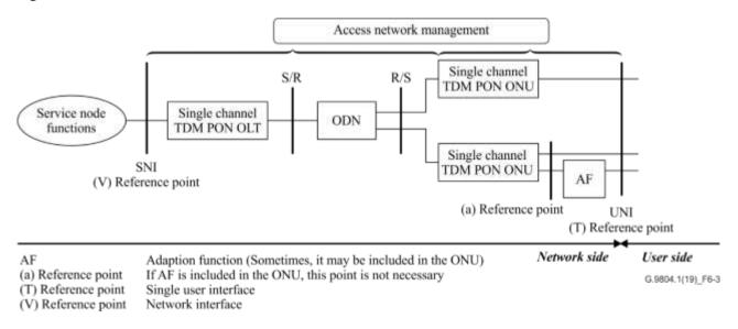
Figure 6-3 – High-level reference configuration of single channel TDM PON
