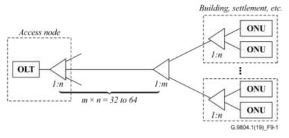
Figure 9-1 – 50G TDM PON splitter architecture options
