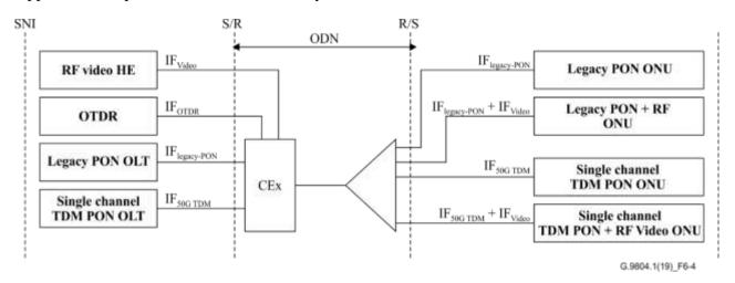
Figure 6-4 – Functional reference architecture and points for single channel TDM PON system coexistence with legacy systems
