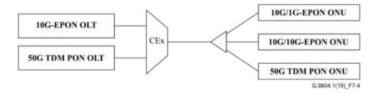
Figure 7-4 – Coexistence of 10G-EPON and 50G TDM PON by independent CEx device
