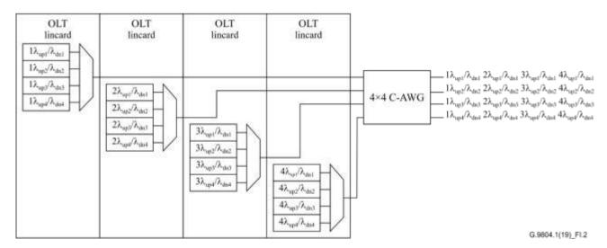
Figure I.2 – OLT resilience configuration with integrated port design
