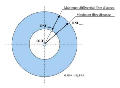
Figure 5-5 – Fibre distance concepts
