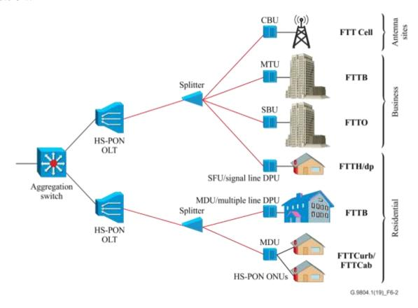
Figure 6-2 – Deployment scenarios of higher speed PON
