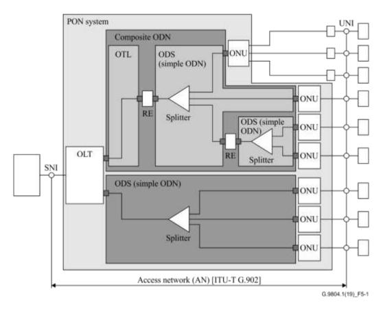
Figure 5-1 – Reference access network architecture
