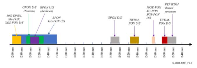
Figure 9-3 – Wavelength plans of legacy PON systems
