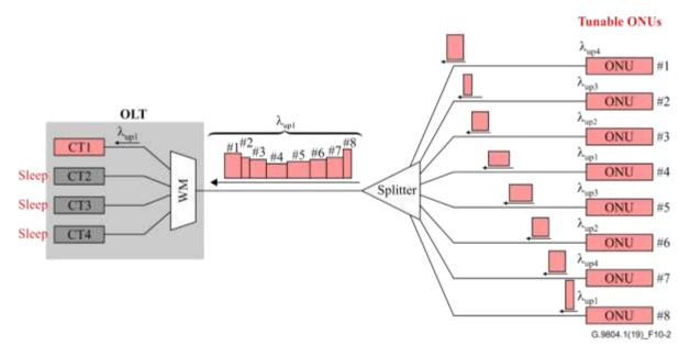
Figure 10-2 – Example of the TWDM PON OLT-port sleep (CT 2, CT 3 and CT 4 are in sleep mode)
