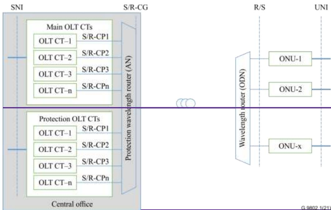
**Figure 11-1 Example of full CT protection**
