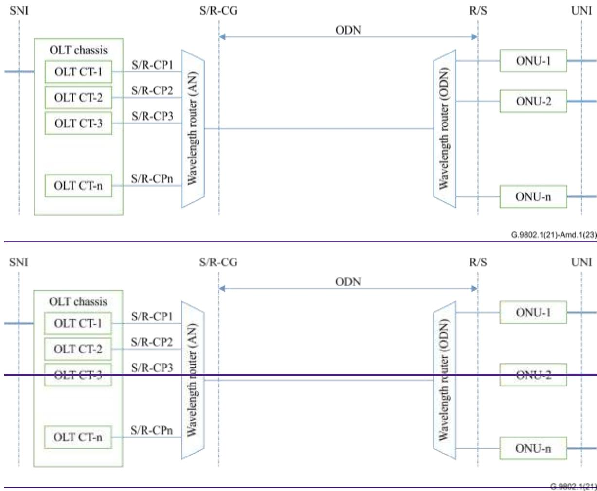
**Figure 6-1 – Functional architecture and reference points for WRP**
