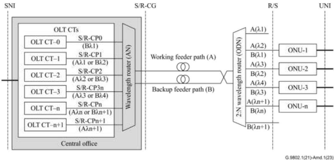
**Figure 11-9 – Example of individual CT and feeder protection using tuneable CTs, dual 2:n WRs, and tuneable ONUs**
