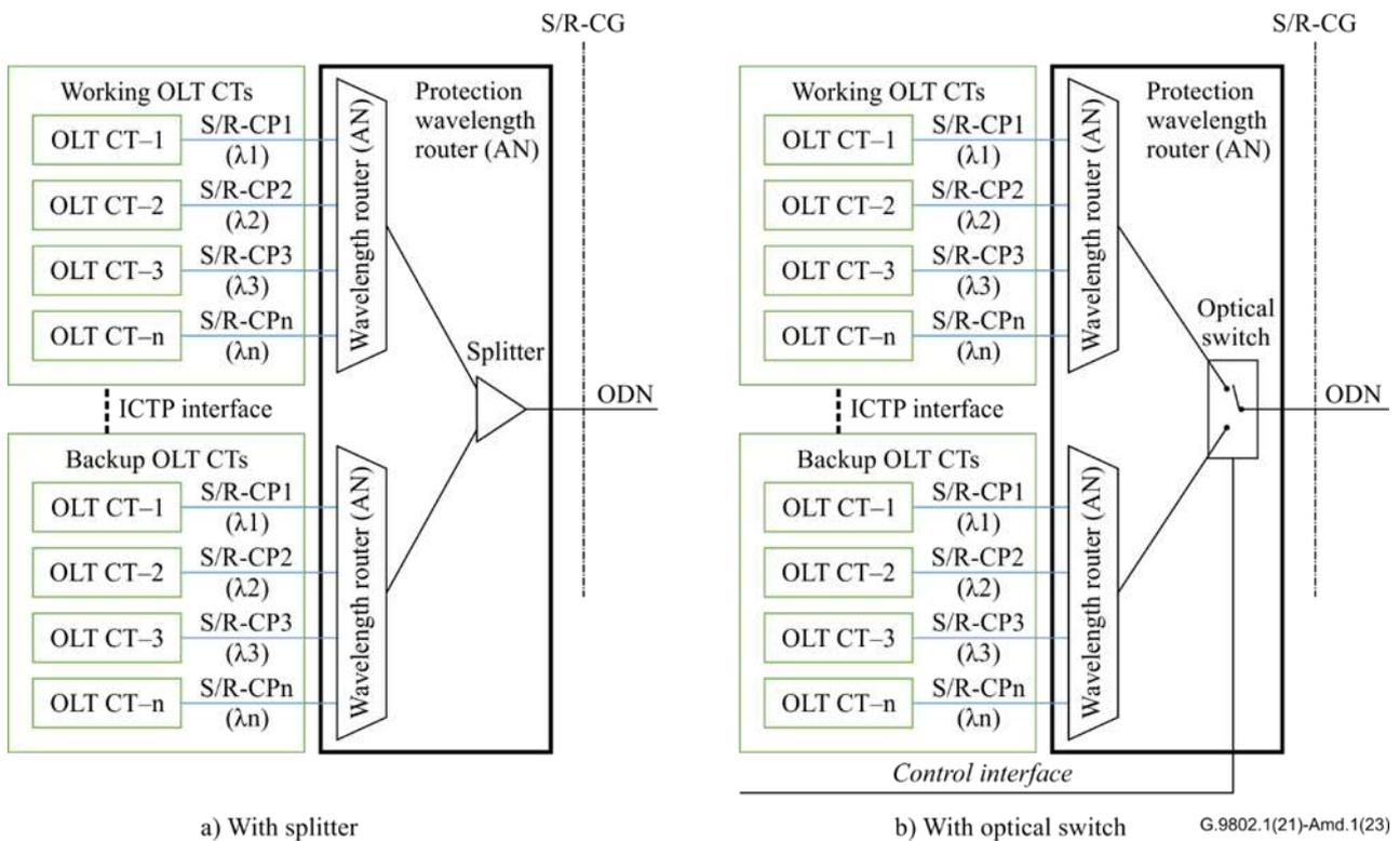
**Figure 11-2 – Reference architectures of protection wavelength router (AN) in full CT protection scenario**
