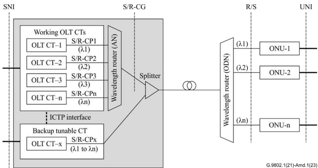
**Figure 11-3 – Example of individual CT protection through a splitter and a tunable CT**
