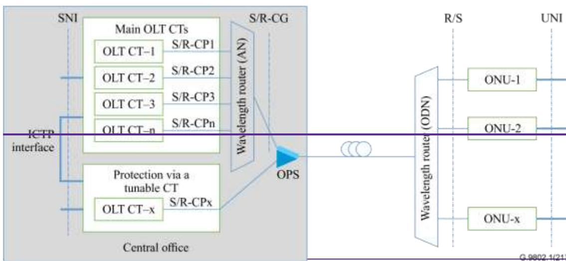
**Figure 11-2 Example of individual CT protection through an OPS and a tunable CT**
