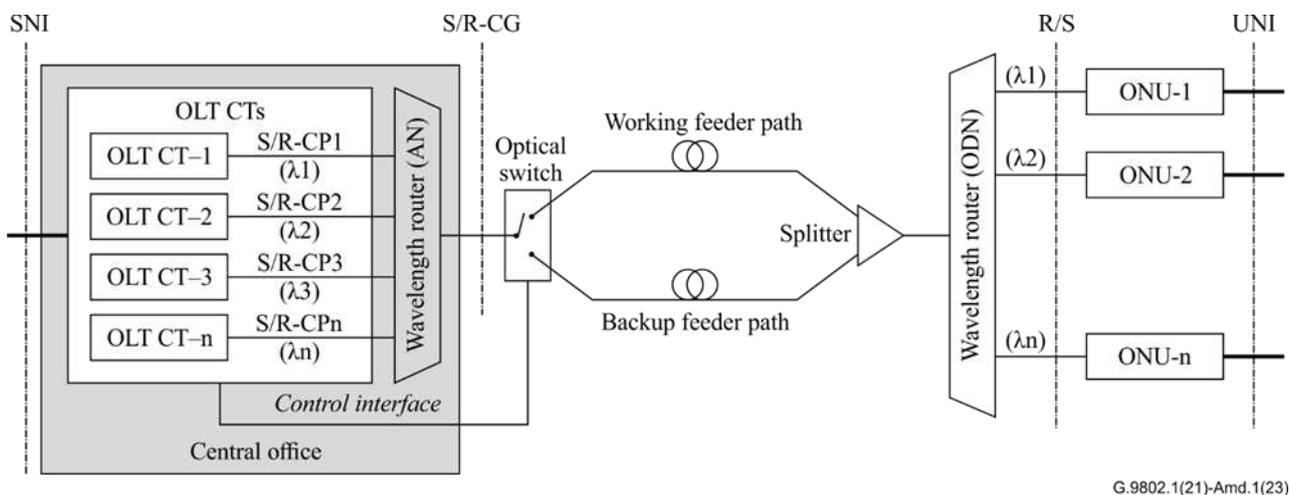
**Figure 11-5 – Example of feeder protection through single OLT with an external optical switch**
