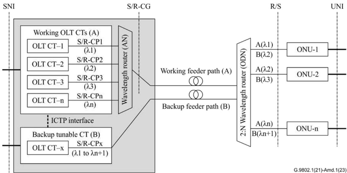
**Figure 11-4 – Example of individual CT and ODN protection using a 2:n wavelength router and a tuneable CT**
