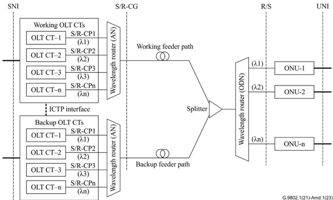
**Figure 11-7 – Example of feeder protection through dual OLT**
