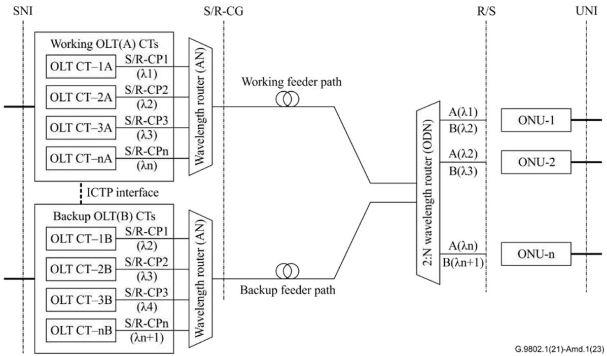
**Figure 11-8 – Example of CT and feeder protection using dual OLTs, 2:n wavelength router, and tuneable ONUs.**
