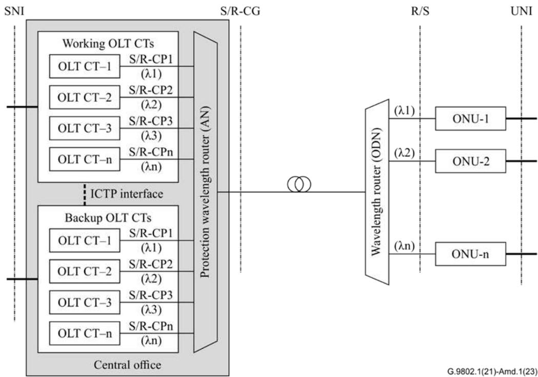
**Figure 11-1 – Example of full CT protection scenario**
