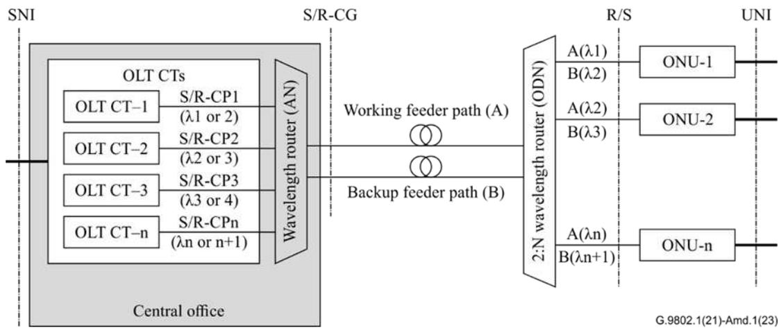
**Figure 11-6 – Example of feeder protection using a single OLT with adjacent channel tuneable CTs, 2:n wavelength routers, and tuneable ONUs**
